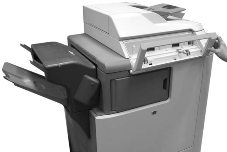
Figure 6-8 Remove the control panel (3 of 3)
