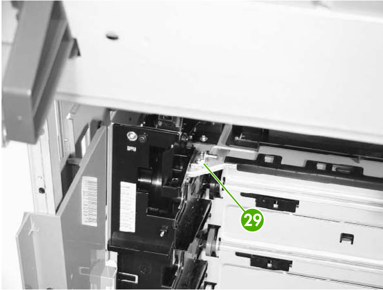
Figure 6-192 Remove the delivery assembly (13 of 15)
