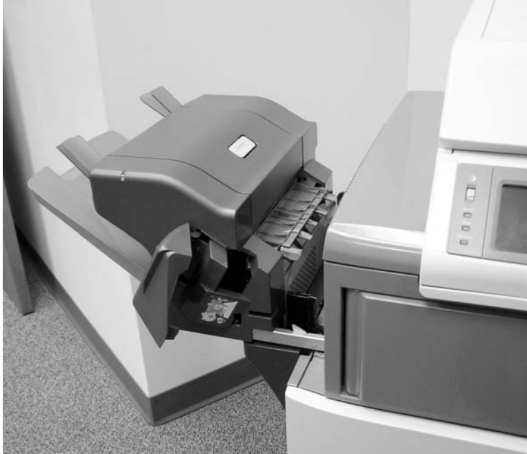
Figure 6-19 Replace the staple cartridge (3 of 3)
