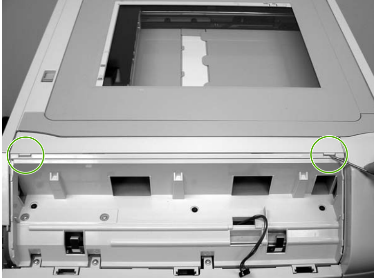
Figure 6-275 Remove the top covers (1 of 2)
