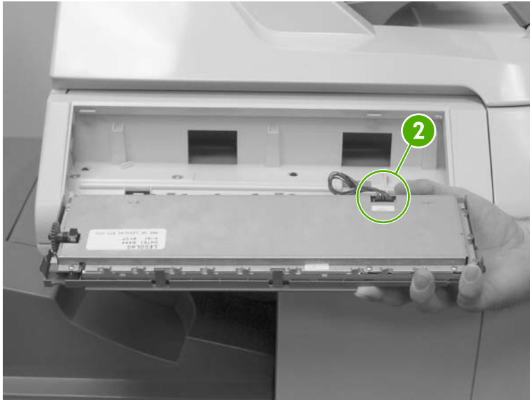
Figure 6-7 Remove the control panel (2 of 3)
