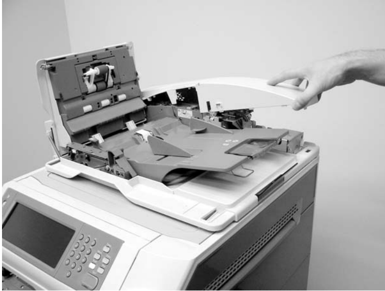
Figure 6-317 Remove the ADF rear cover (3 of 3)
