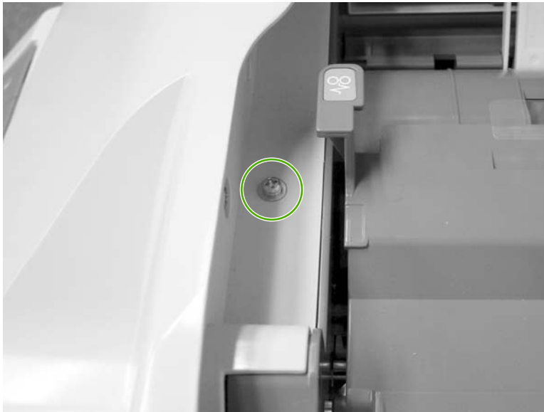
Figure 6-313 Remove the ADF front cover (1 of 2)
