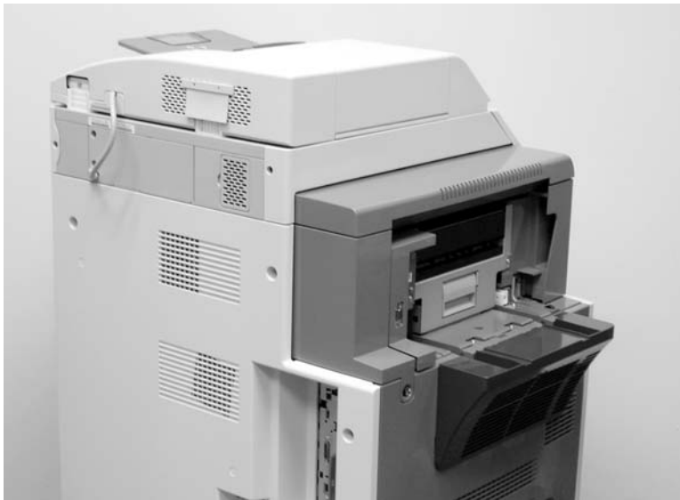
Figure 6-16 Remove the stapler/stacker (5 of 5)
