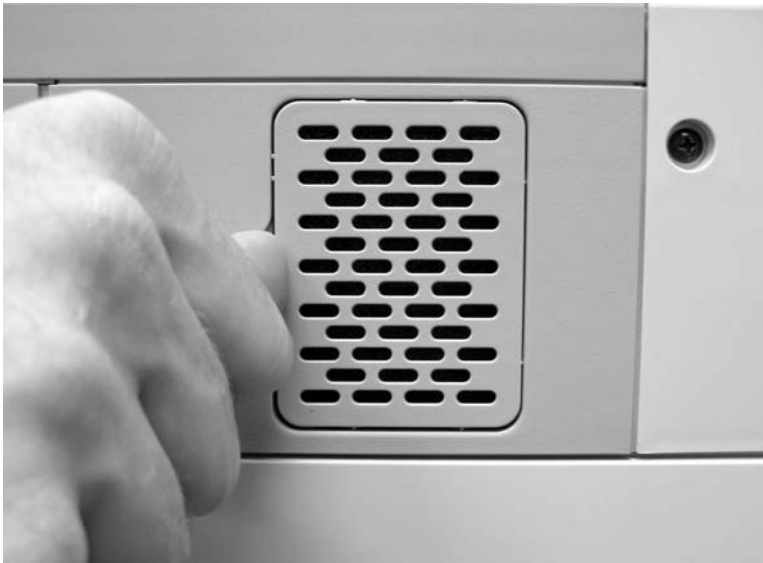
Figure 6-58 Remove the scanner filter (1 of 2)
