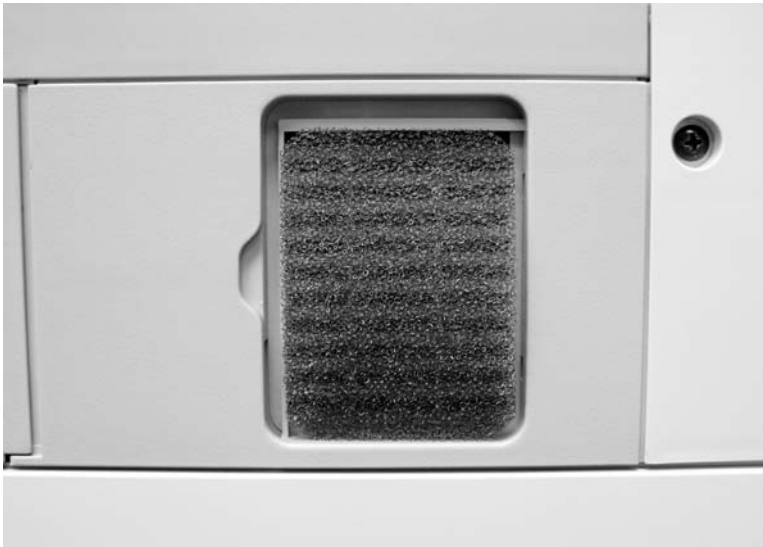
Figure 6-59 Remove the scanner filter (2 of 2)
