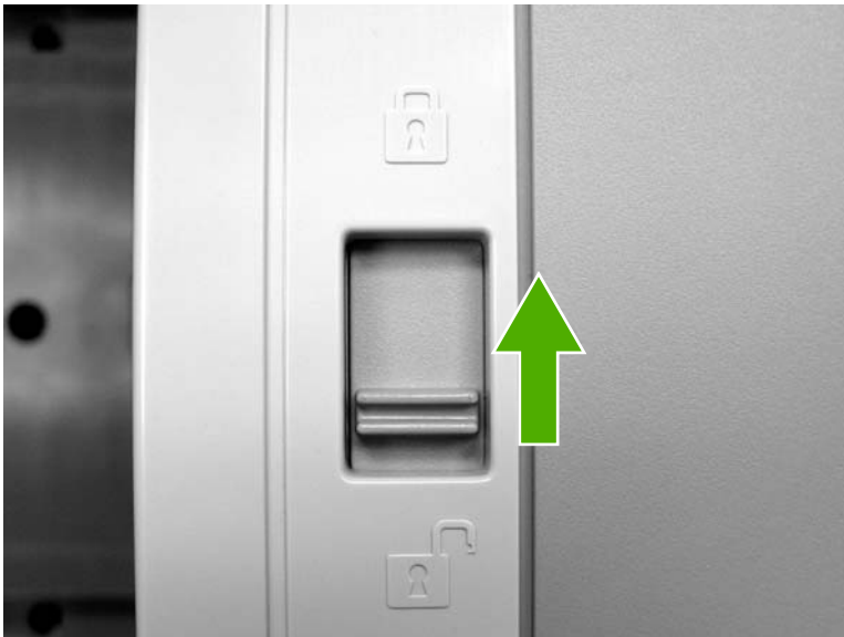
Figure 6-282 Remove the scanner left cover (1 of 2)
