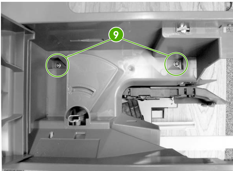
Figure 6-373 Remove the IPTU front cover and front door (5 of 6)
