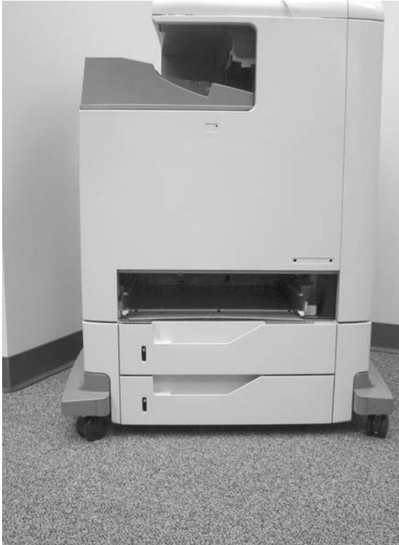
Figure 6-46 Remove the tray 2, 3, or 4 pickup and feed rollers (1 of 2)
