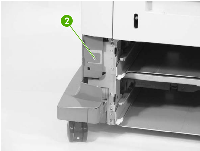
Figure 6-337 Remove the left cover (2 of 3)
