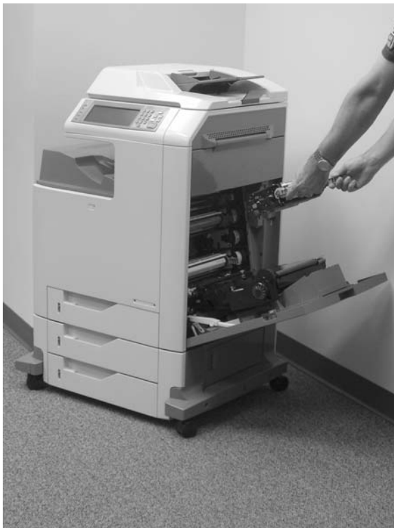
Figure 6-4 Remove the print cartridges (3 of 3)
