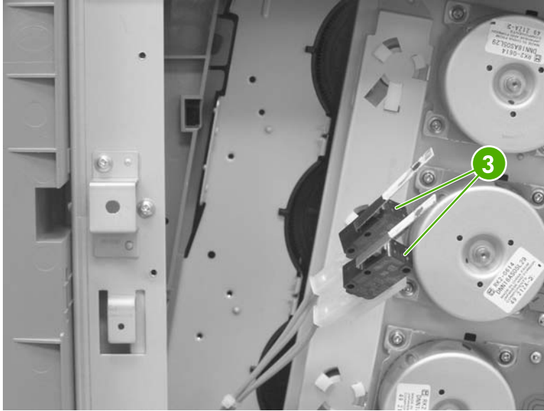
Figure 6-270 Remove the door-open switch assembly (3 of 3)
