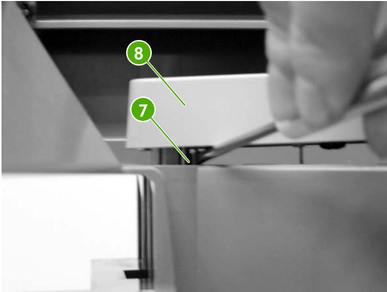
Figure 6-372 Remove the IPTU front cover and front door (4 of 6)
