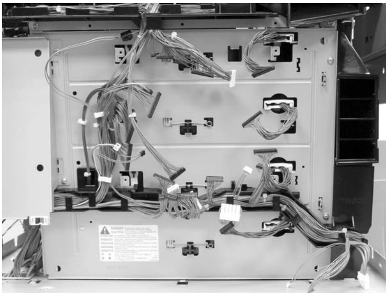
Figure 6-235 Remove the DC controller (2 of 2)
