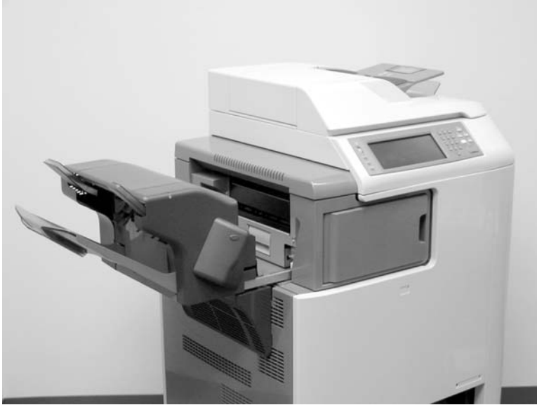
Figure 6-13 Remove the stapler/stacker (2 of 5)
