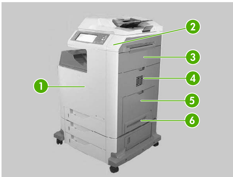
Figure 6-75 Cover, door, and panel locations (1 of 2)
