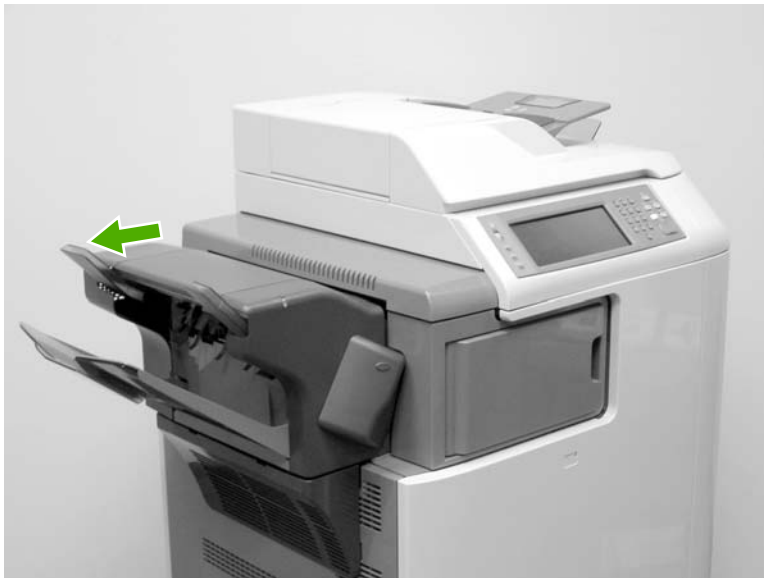
Figure 6-12 Remove the stapler/stacker (1 of 5)
