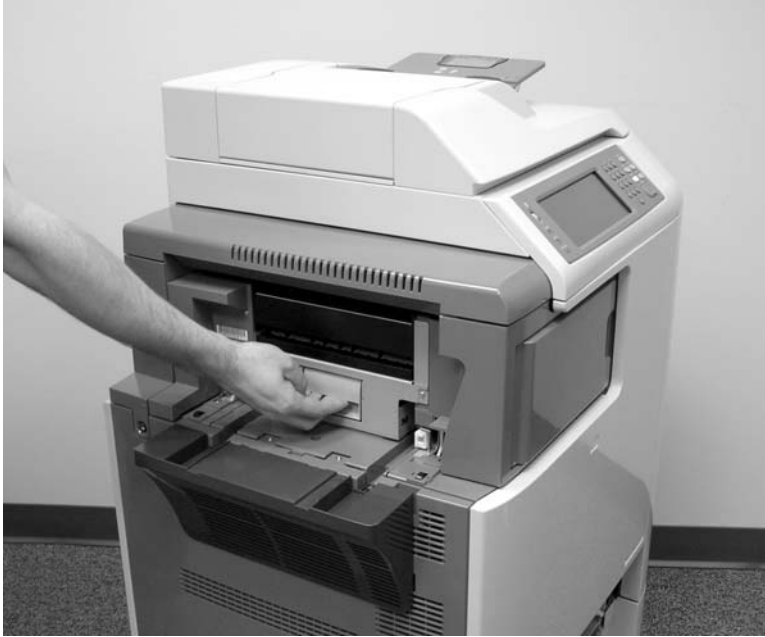
Figure 6-9 Remove the IPTU (1 of 3)
