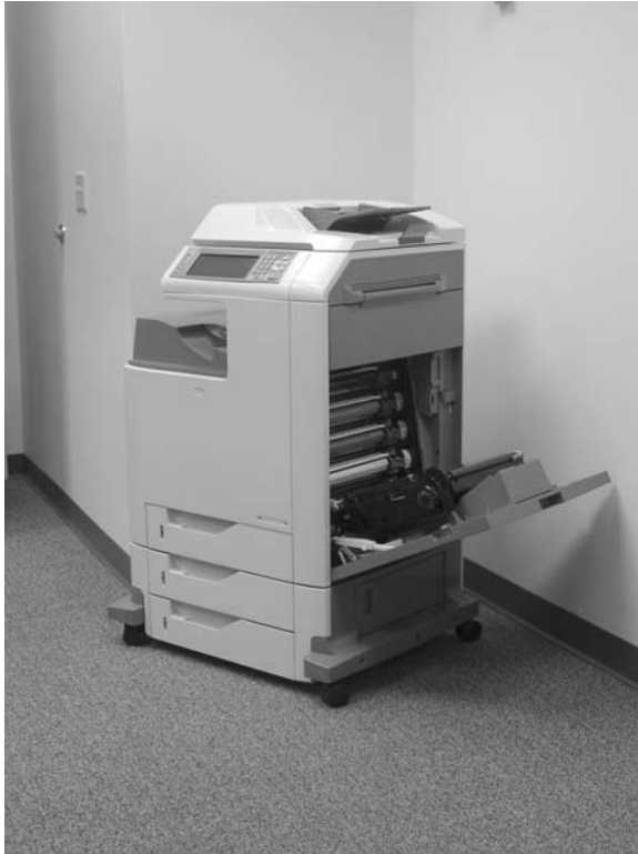
Figure 6-23 Remove the ETB assembly (1 of 4)
