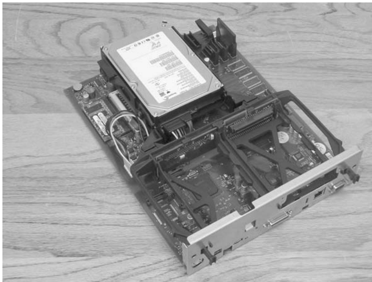
Figure 6-62 Remove the formatter (2 of 2)
