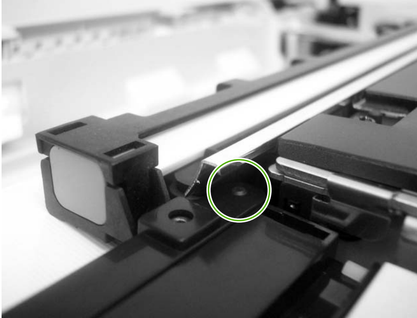
Figure 6-293 Remove the optical assembly (7 of 10)
