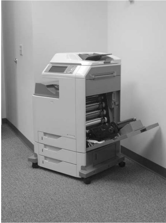
Figure 6-3 Remove the print cartridges (2 of 3)
