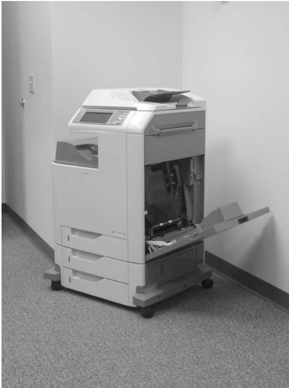
Figure 6-2 Remove the print cartridges (1 of 3)
