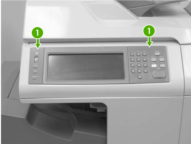
Figure 6-5 Remove the control panel overlays
