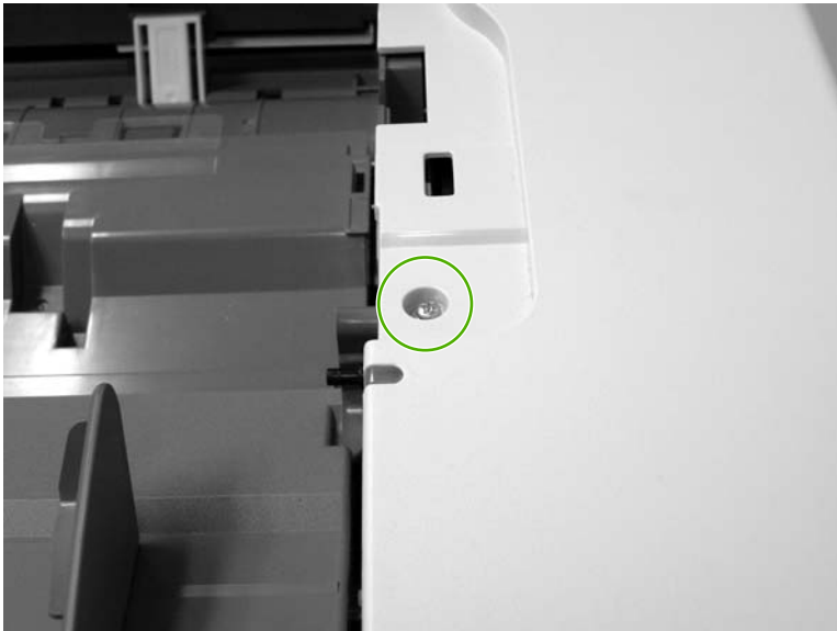
Figure 6-316 Remove the ADF rear cover (2 of 3)
