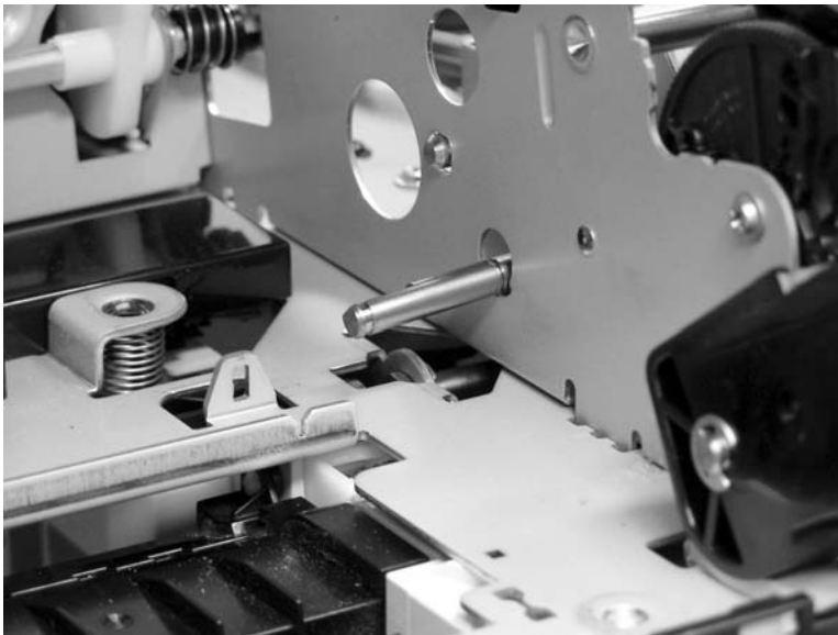
Figure 6-209 Remove the pickup motor assembly (2 of 3)
