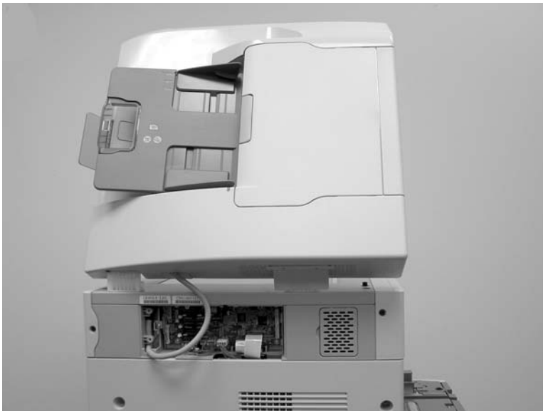
Figure 6-274 Remove the ADF assembly (3 of 3)
