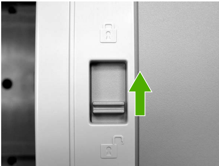
Figure 6-284 Remove the scanner right cover (1 of 2)
