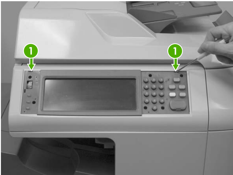
Figure 6-6 Remove the control panel (1 of 3)
