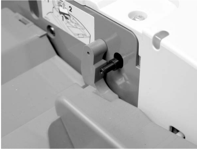
Figure 6-31 Remove the ADF input tray (3 of 3)
