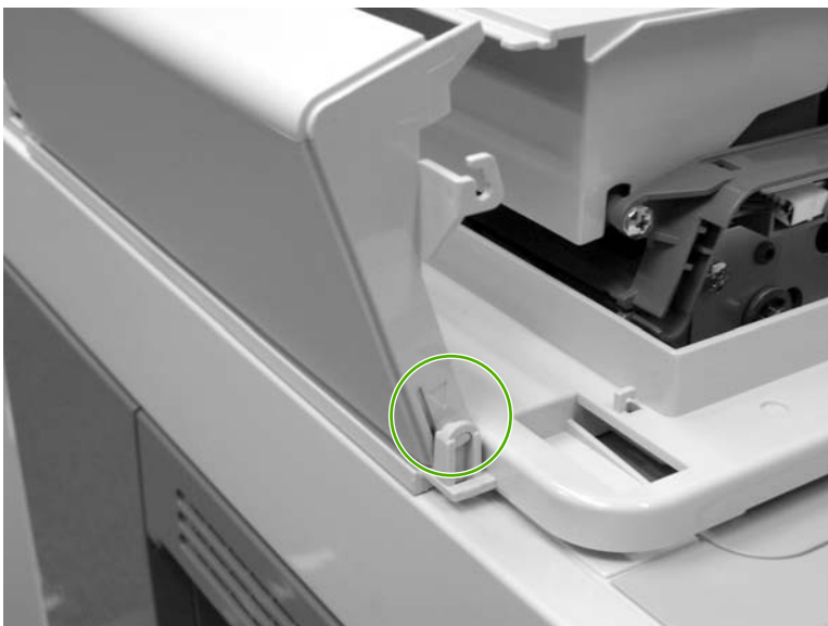
Figure 6-319 Remove the ADF left cover (2 of 2)
