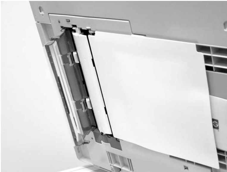
Figure 6-309 Remove the ADF white mylar backing (2 of 3)
