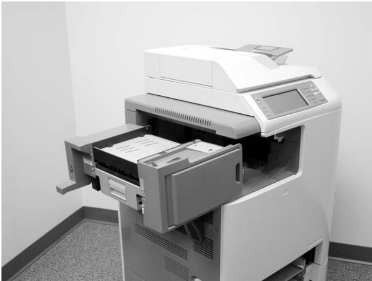
Figure 6-10 Remove the IPTU (2 of 3)
