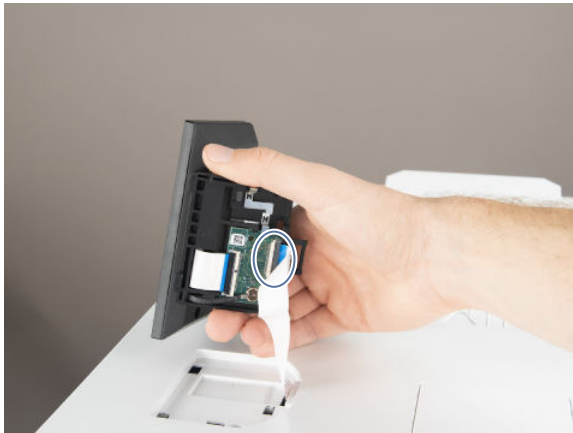
Figure 5-258 Remove the control panel
