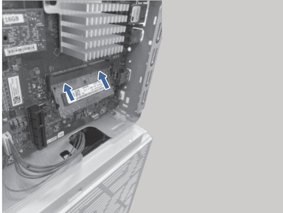
Figure 5-62 Insert the top edge into the formatter
