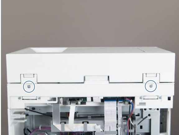
Figure 5-142 Remove two screws
