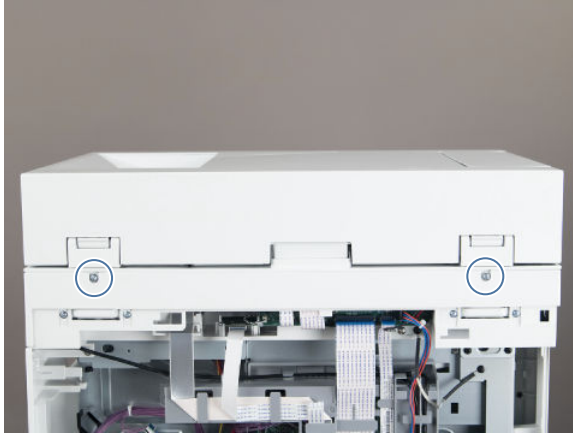
Figure 5-132 Remove two screws
