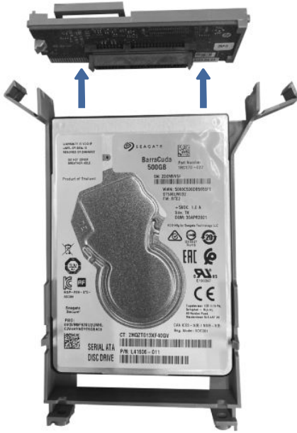
Figure 5-97 Remove the PCA cradle
