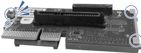
Figure 5-85 Verify PCA installation
