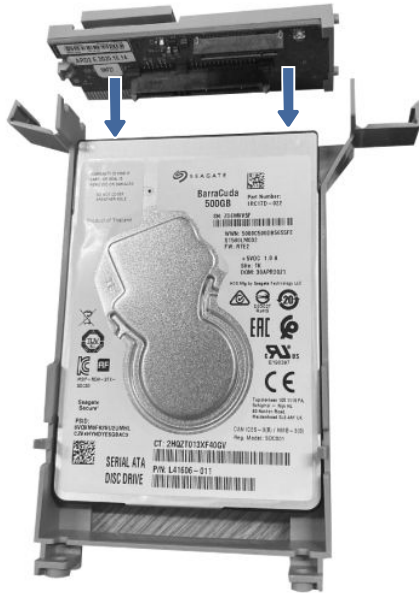
Figure 5-103 Align the SSD card
