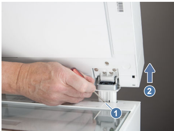
Figure 5-151 Release two tabs
