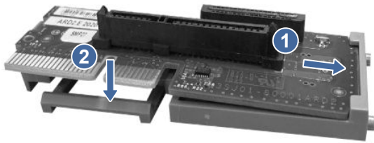
Figure 5-84 Install PCA in cradle
