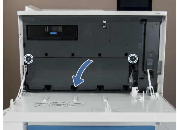
Figure 2-4 Remove two screws, open the cover
