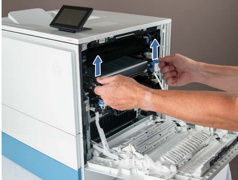
Figure 5-508 Disengage the ITB
