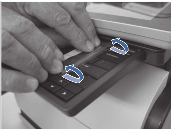
Figure 5-27 Apply the keyboard overlay
