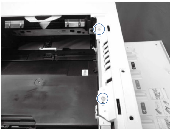
Figure 5-596 Remove two screws
