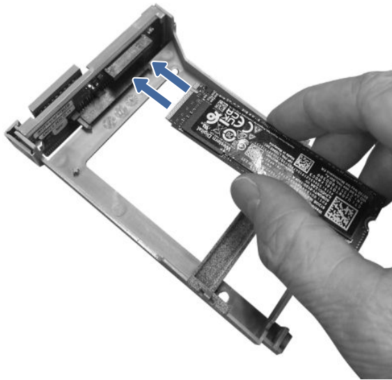
Figure 5-89 Align the SSD card
