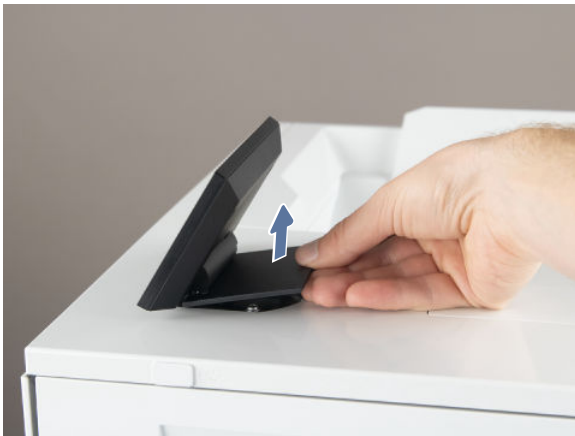
Figure 5-255 Remove the control panel cover
