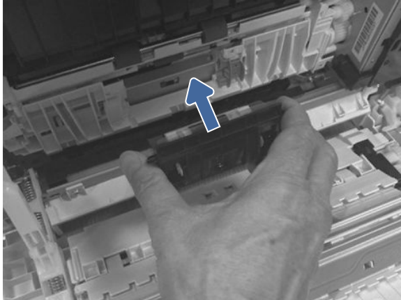
Figure 5-40 Install the separation roller assembly
