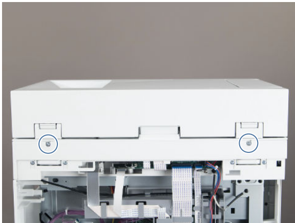
Figure 5-149 Remove two screws
