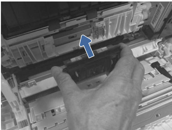
Figure 2-17 Install the separation roller assembly
