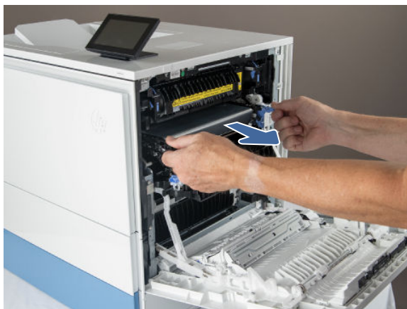
Figure 5-12 Release the ITB
