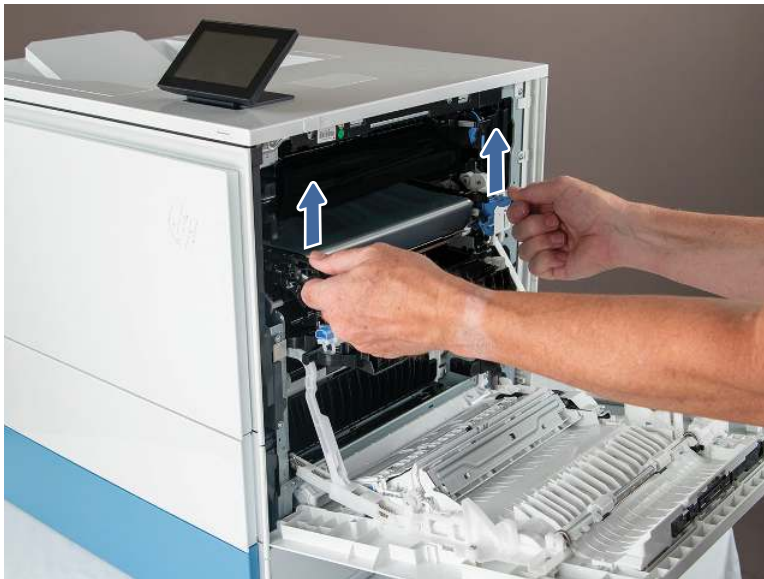
Figure 5-543 Disengage the ITB
