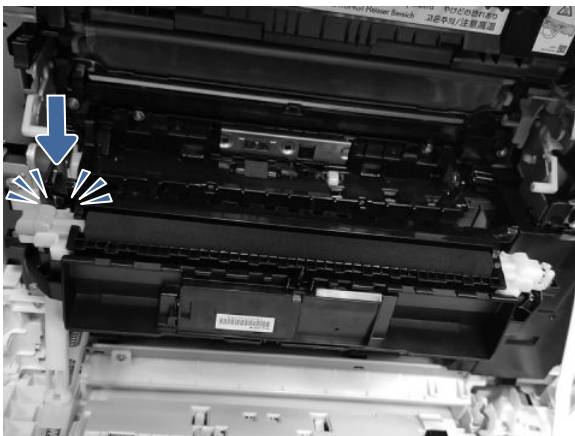
Figure 5-17 Secure the secondary transfer roller
