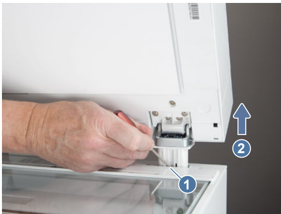
Figure 5-134 Release two tabs
