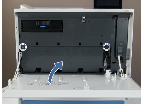
Figure 5-5 Close the cover, install two screws
