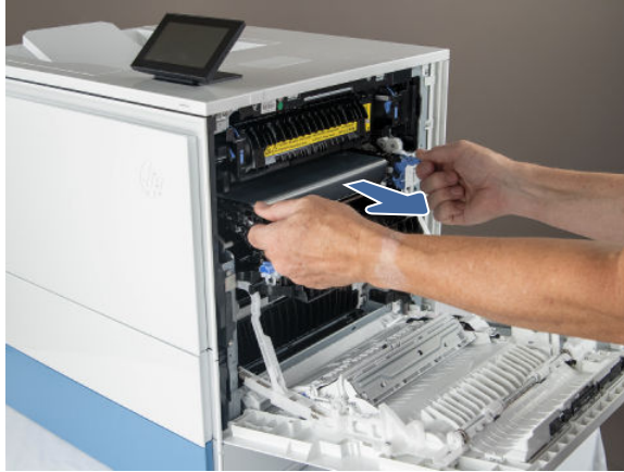
Figure 5-272 Release the ITB
