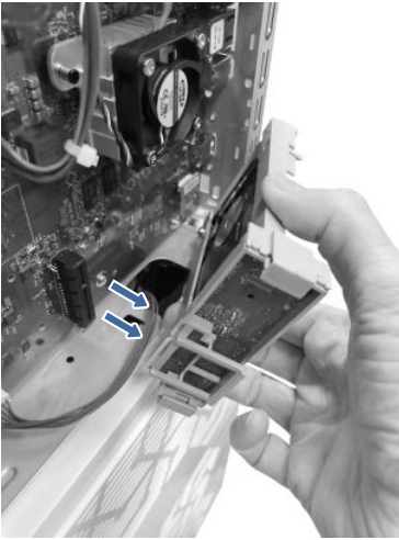
Figure 5-95 Remove the HDD
