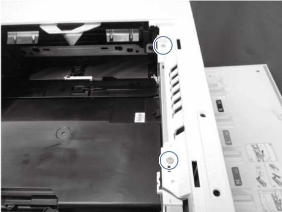
Figure 5-234 Remove two screws
