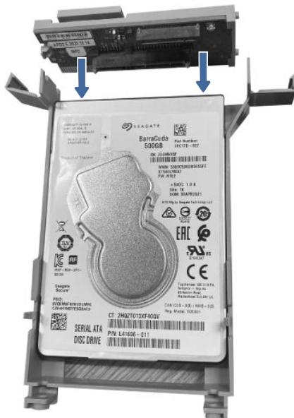
Figure 5-100 Align the PCA cradle
