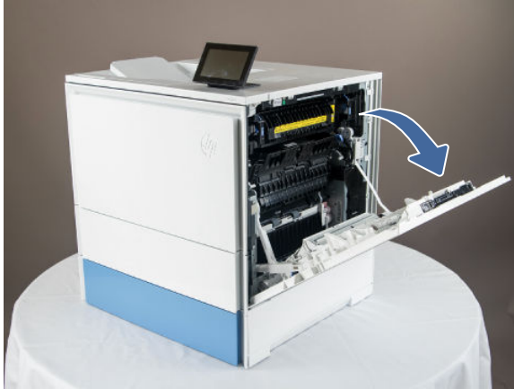
Figure 5-420 Open the right door
