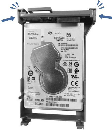
Figure 5-100 Close two clips
