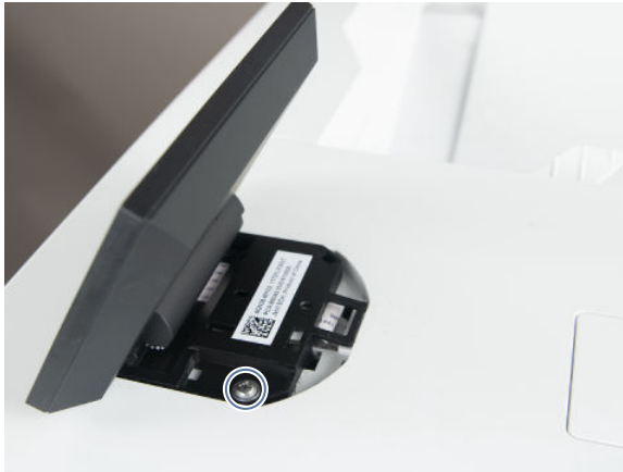
Figure 5-253 Remove one screw
