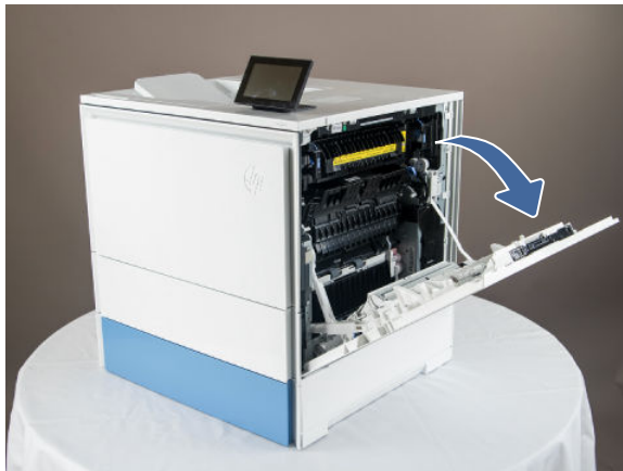
Figure 5-303 Open the right door
