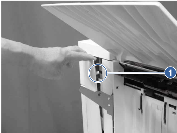
Figure 5-1409 Release one boss
