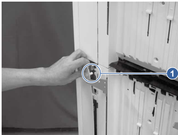
Figure 5-1170 Release one boss
