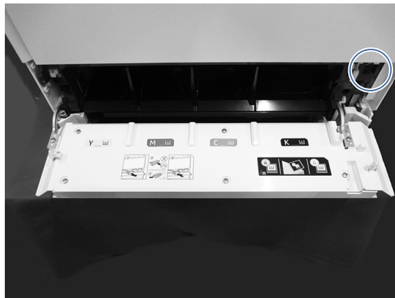
Figure 4-51 Defeat the toner supply door interlock (X654/X677 models)
