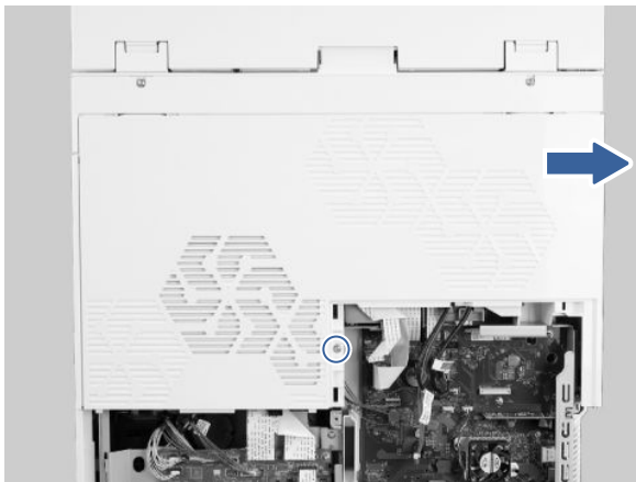
Figure 5-140 Remove the cover
