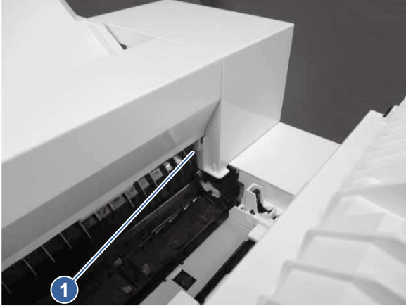
Figure 5-1090 Release one tab
