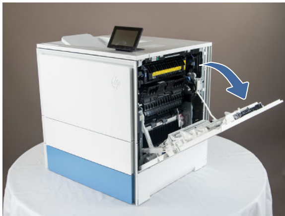
Figure 5-630 Open the right door
