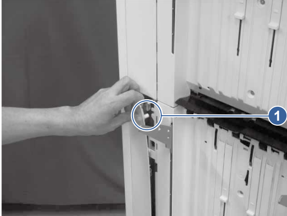
Figure 5-1416 Release one boss
