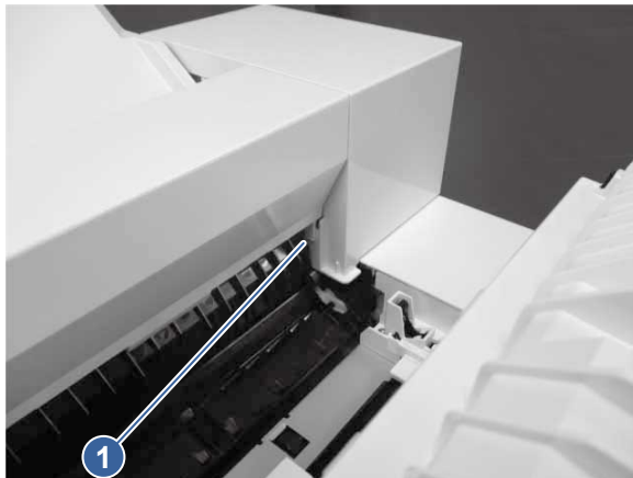
Figure 5-1289 Release one tab
