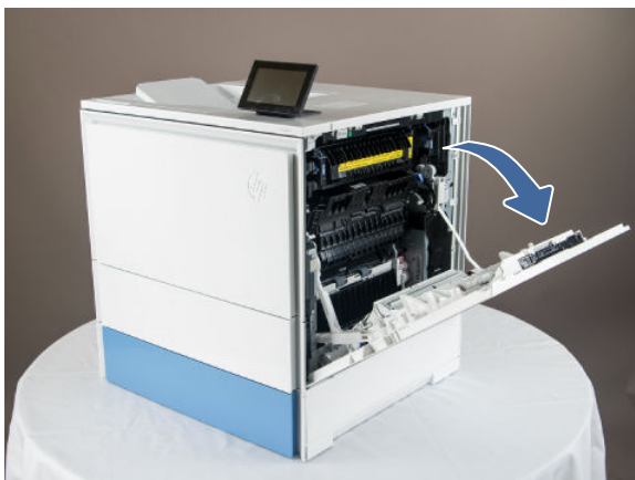
Figure 5-785 Open the right door
