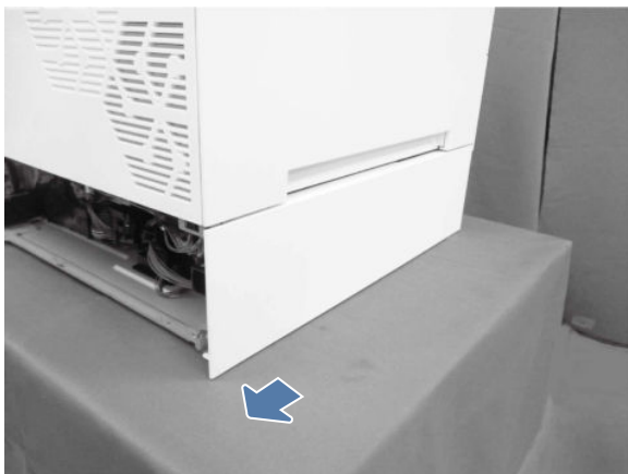
Figure 5-209 Remove the left lower cover
