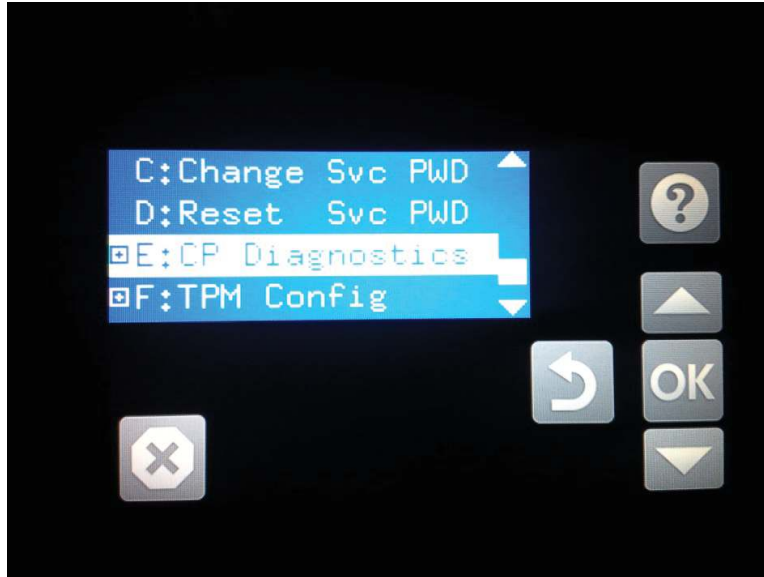
Figure 4-116 Access the diagnostics menu
