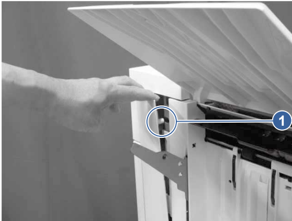
Figure 5-1070 Release one boss
