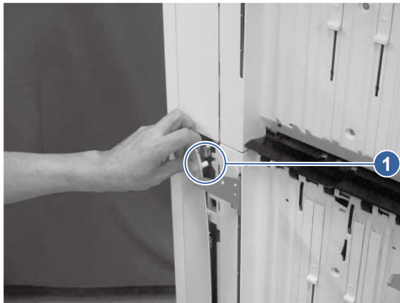
Figure 5-1331 Release one boss
