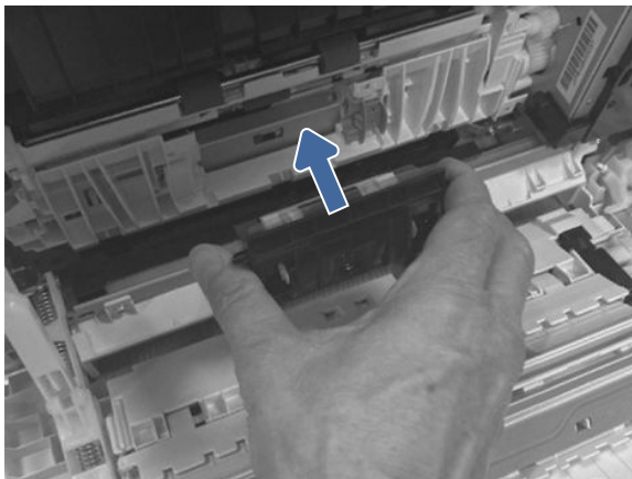
Figure 2-17 Install the separation roller assembly
