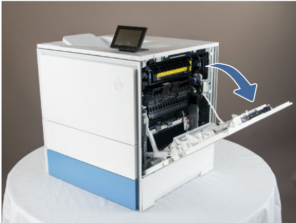
Figure 5-287 Open the right door
