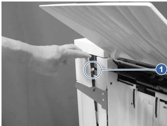
Figure 5-1058 Release one boss
