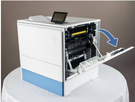
Figure 5-278 Open the right door
