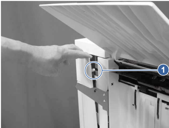
Figure 5-1195 Release one boss
