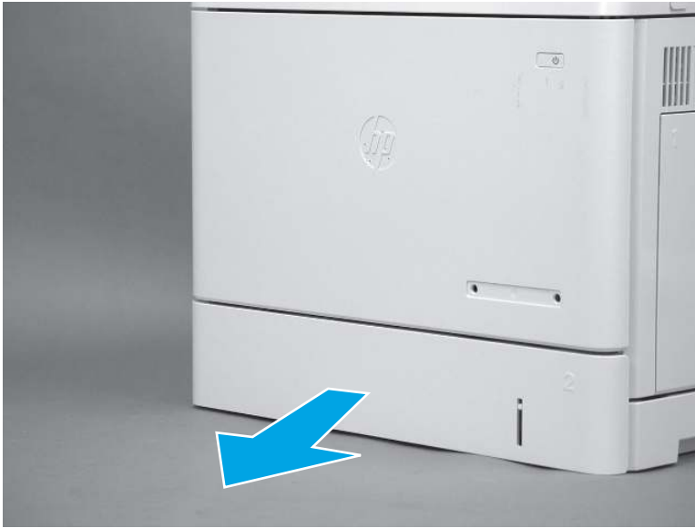
Figure 5-159 Pull the tray out
