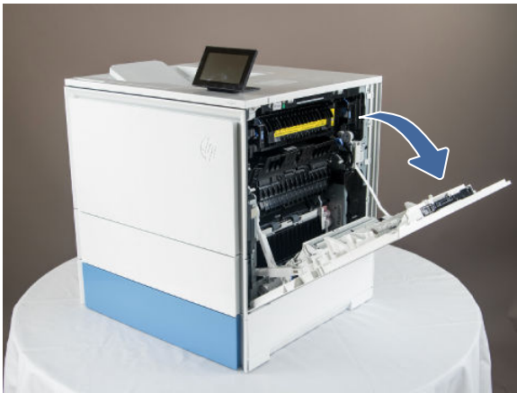
Figure 5-467 Open the right door
