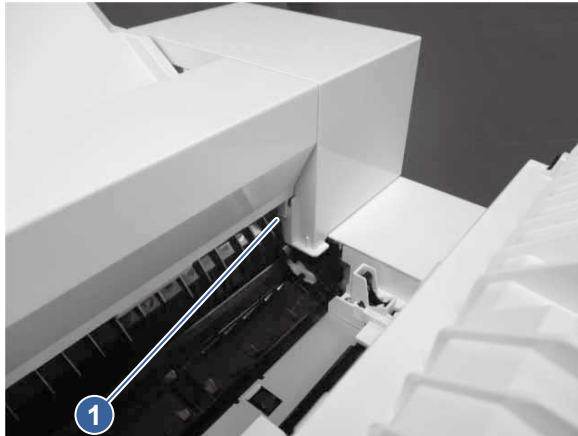
Figure 5-1411 Release one tab
