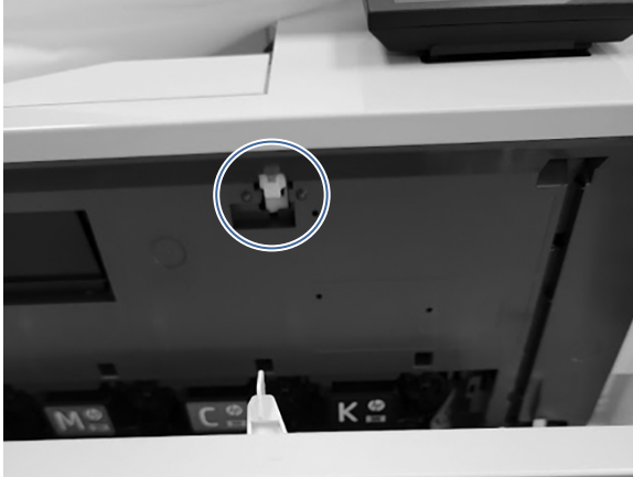
Figure 4-110 Defeat the front door interlock
