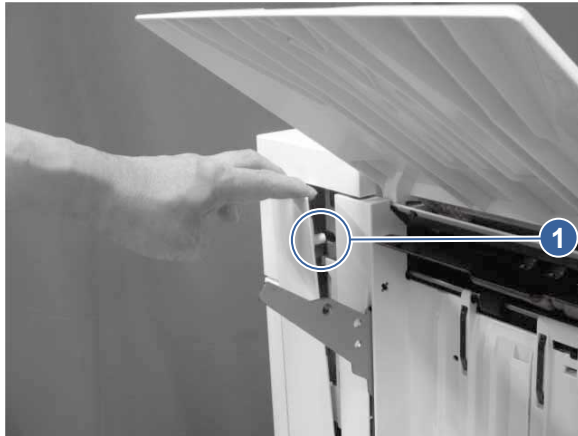
Figure 5-1236 Release one boss
