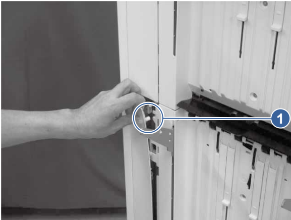
Figure 5-1198 Release one boss
