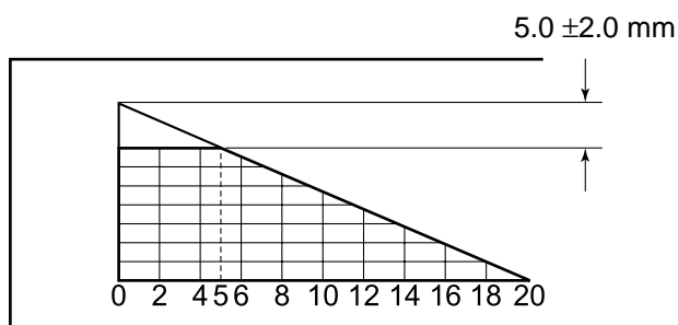
Figure 26. Image and non-image width of the leading edge
