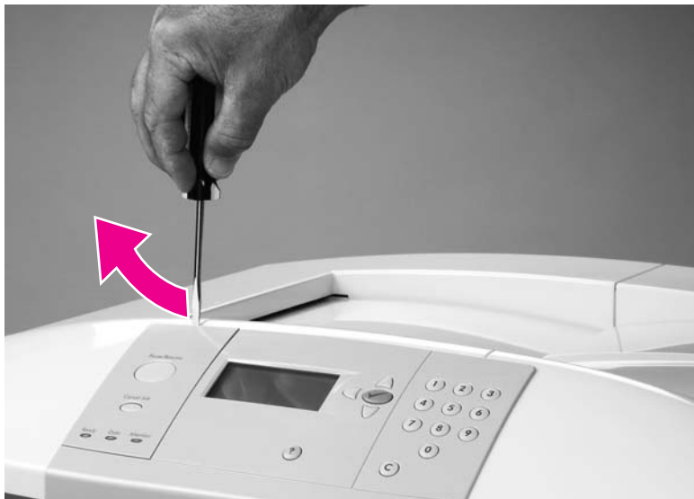
Figure 86. Remove the control panel overlay
