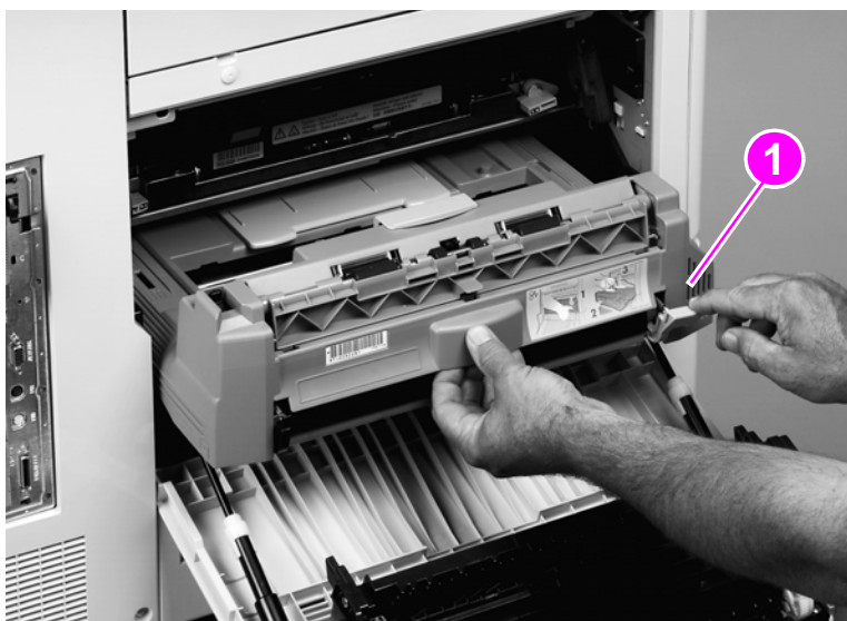
Figure 160. Remove the duplexer
