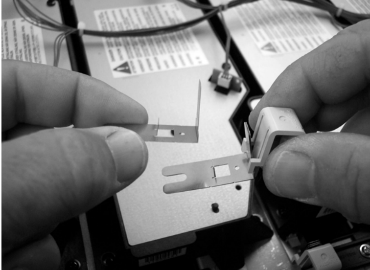
Figure 140. Add or remove the laser/scanner adjustment shims
