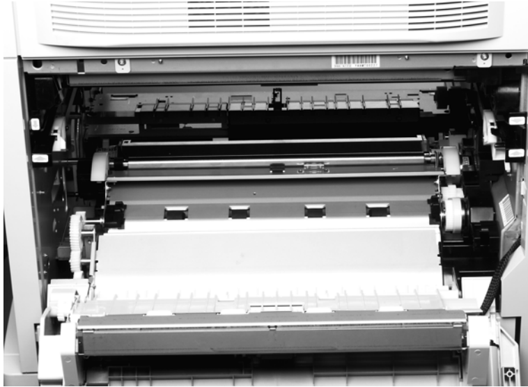
Figure 182. Remove the T2 assembly
