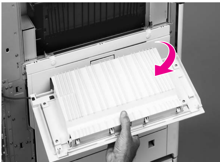
Figure 153. Remove the paper path access door
