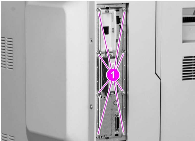
Figure 233. Remove the formatter PCB mounting screws
