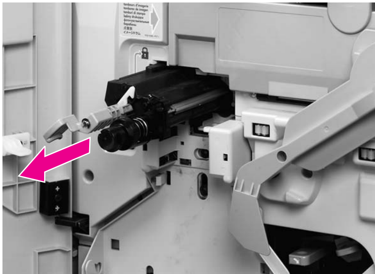
Figure 83. Remove the transfer cleaner
