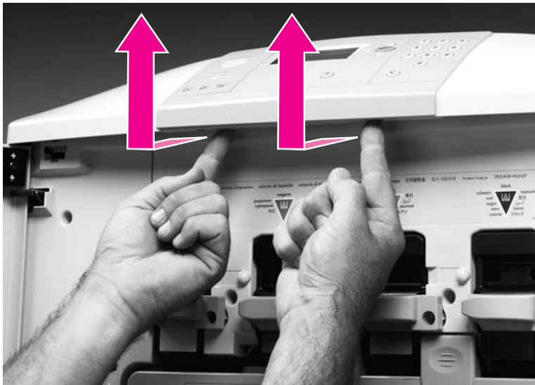
Figure 87. Release the control panel
