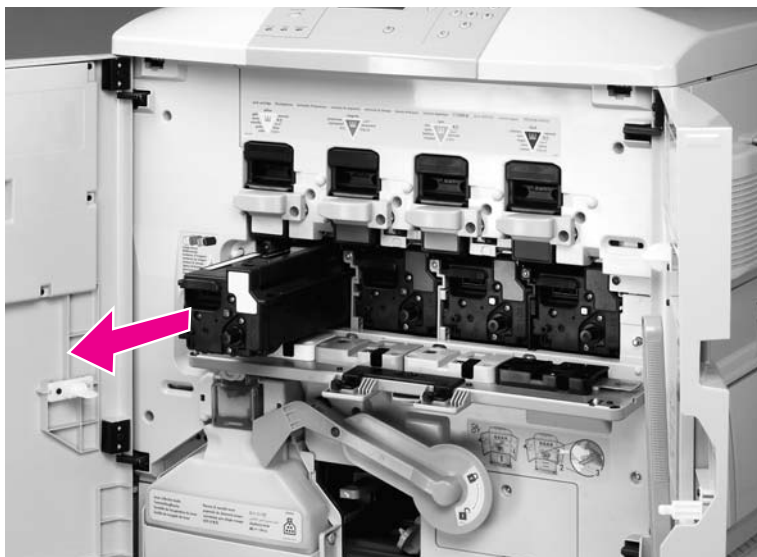
Figure 80. Remove the process cartridges
