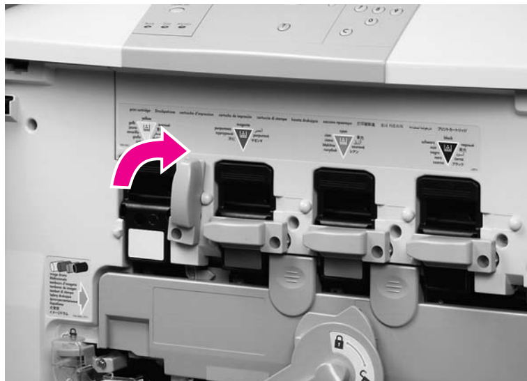
Figure 75. Rotate the toner cartridge lever
