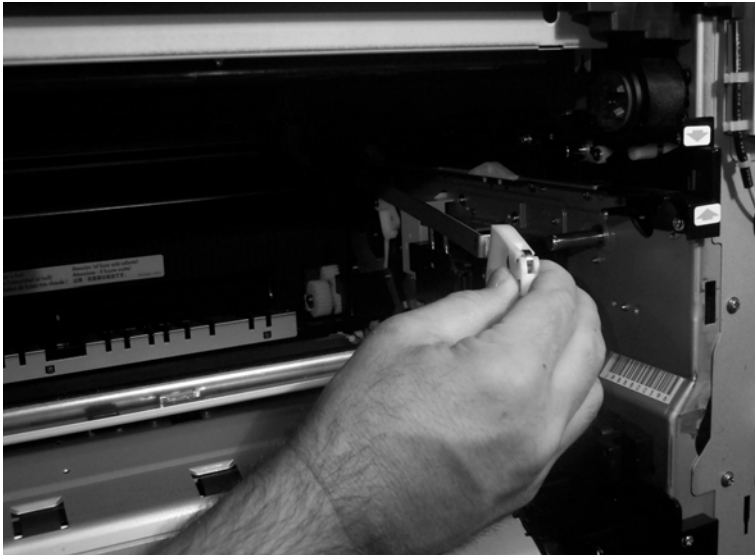
Figure 210. Remove the right back ITB lifting link
