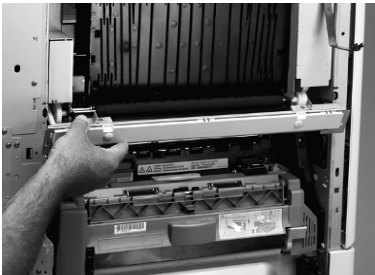
Figure 152. Remove the left side middle cover mounting bracket
