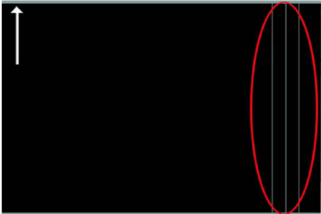
Figure 268. Lines, streaks, or scratches appear parallel to feed direction (2 of 2)
