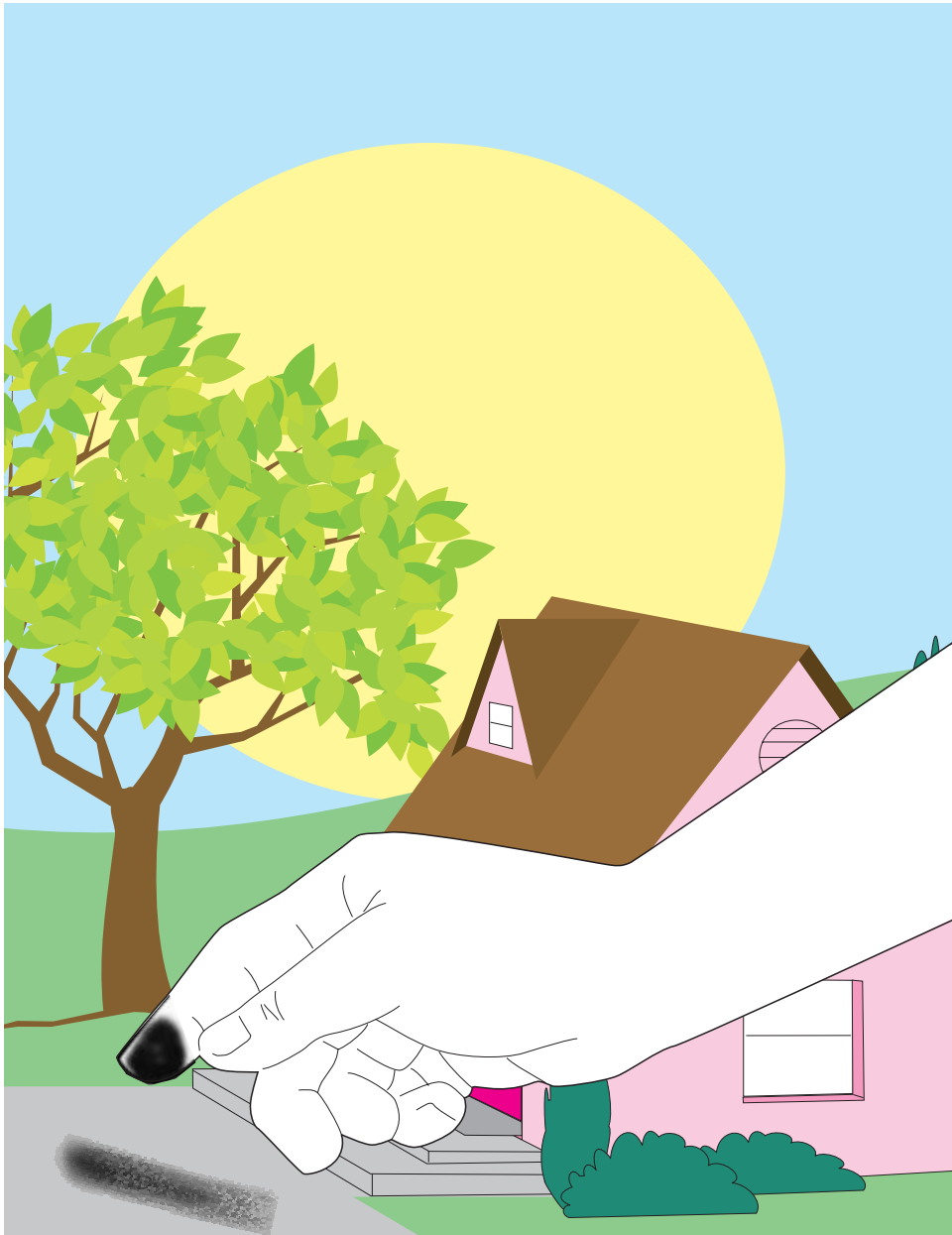
Figure 278. Poorly fused image (2 of 2)
