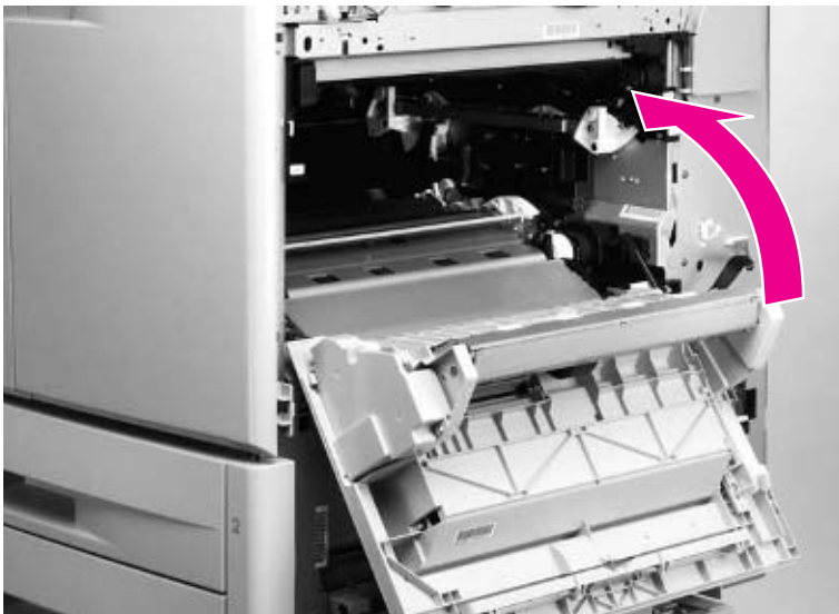
Figure 106. Gain access to the ITB door mounting screws
