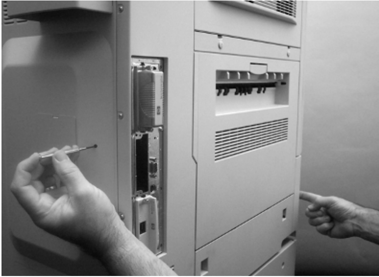
Figure 122. Prepare to print a laser/scanner adjustment page
