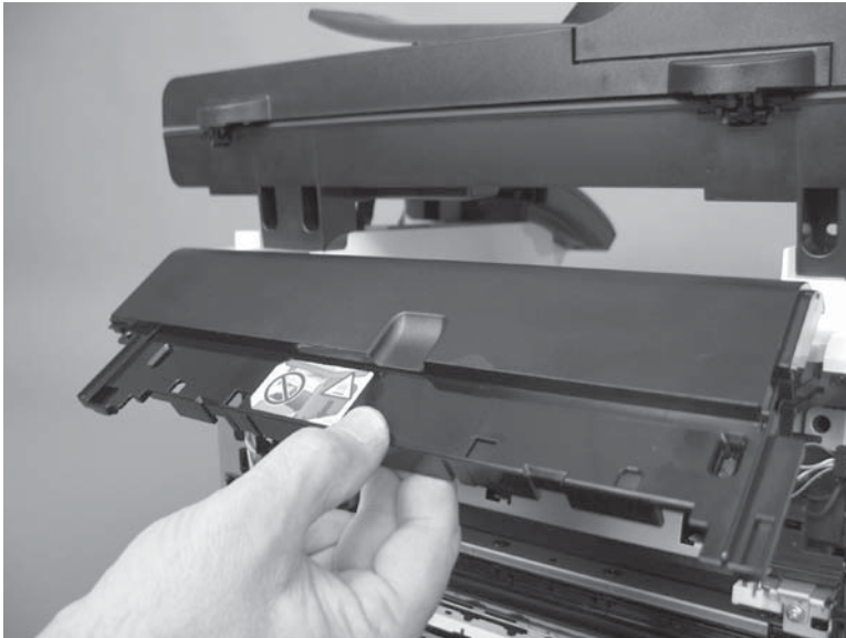
Figure 1-42 Remove the rear-upper cover (4 of 4)
