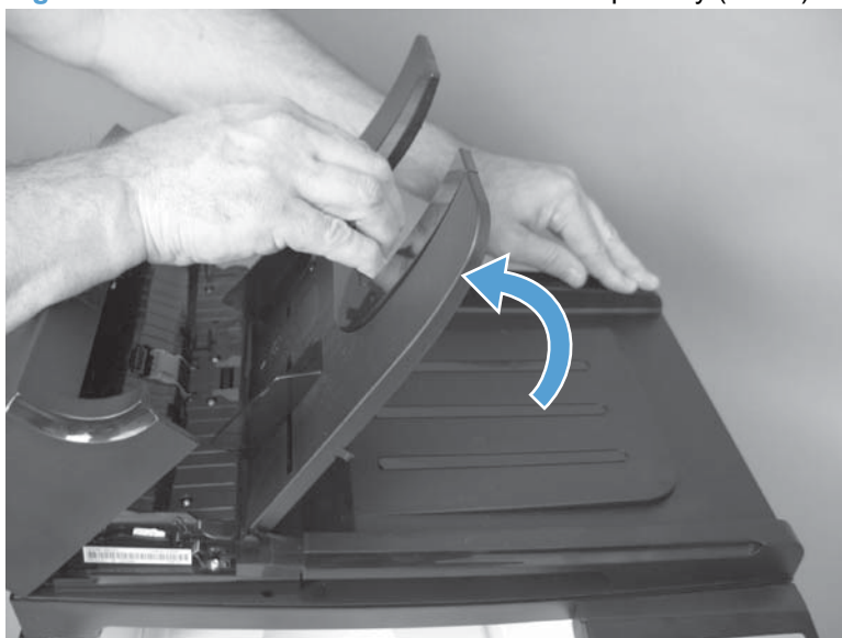
Figure 1-129 Remove the document feeder input tray (2 of 2)
