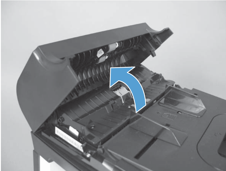
Figure 1-130 Remove the document feeder cover (1 of 3)
