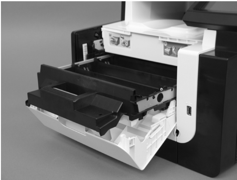
Figure 1-9 Remove the print-cartridge drawer (1 of 5)
