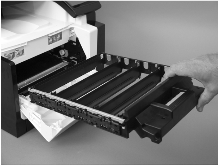
Figure 1-13 Remove the print-cartridge drawer (5 of 5)
