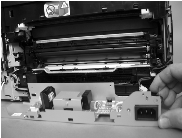
Figure 1-116 Remove the power supply (fuser; 5 of 5)
