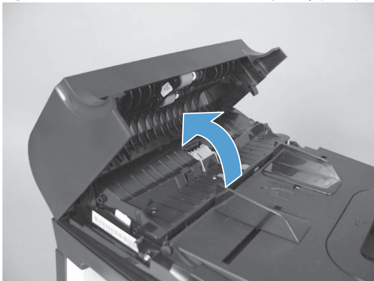
Figure 1-128 Remove the document feeder input tray (1 of 2)
