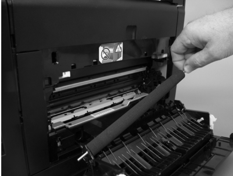
Figure 1-8 Remove the transfer roller (3 of 3)
