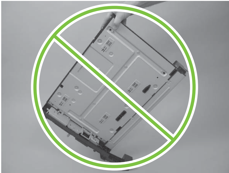
Figure 8-101 Incorrect placement of the IPTU (2 of 2)
