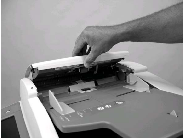
Figure 6-213 Remove the ADF separation floor assembly (1 of 4)
