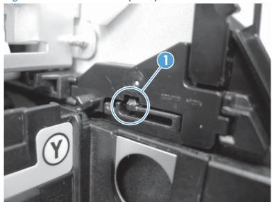
4. Rotate the cartridge-drawer retainer (callout 1) away from the chassis, and then remove it (callout 2). Repeat the previous step and this step for the left–side cartridge-drawer retainer.
