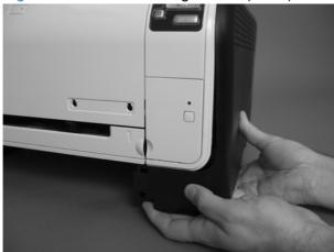
4. Use a small flatblade screwdriver to release three tabs (callout 2) at the back of the product.
