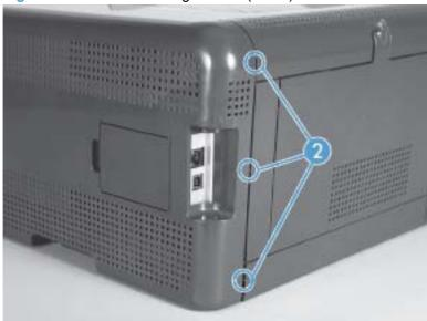
5. Rotate the bottom of the cover away from the product, and then slide it up to remove it.
