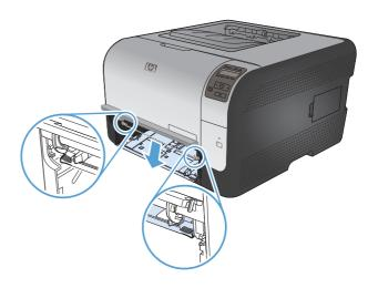
4. Remove the jammed sheet by pulling it straight out.
