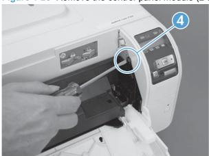
5. Rotate the top of the control-panel module away from the product to remove it.
