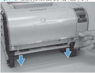
2. Carefully push the left-side Tray 1 door hinge in toward the center of the door to release it from the hinge pin.
