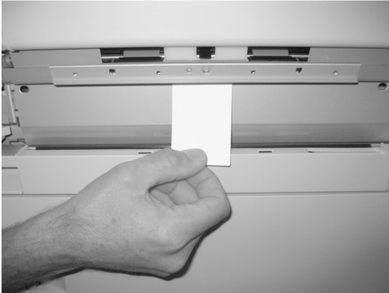
Figure 21 Test the Tray 3 feed sensor
