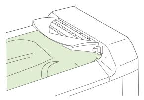
When you send print jobs to the product from a computer, the output is routed to the standard output bin or to one of the output bins on the optional 3-bin stapler/stacker or booklet maker finisher.
