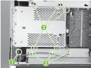
3. Rotate and lift the formatter case to remove it.
