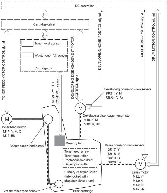
The drum motor causes the photosensitive drum to rotate. That rotation causes the primary-charging roller to rotate. The drum motor also drives the toner feed screw, the toner-feed roller, and the developing roller to transfer toner from the print cartridge into the imaging drum.
