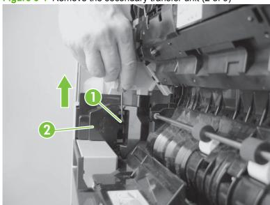
**4.** Disconnect one connector (callout 1). To disconnect, push the front of the connector toward the product, and then pull out.
