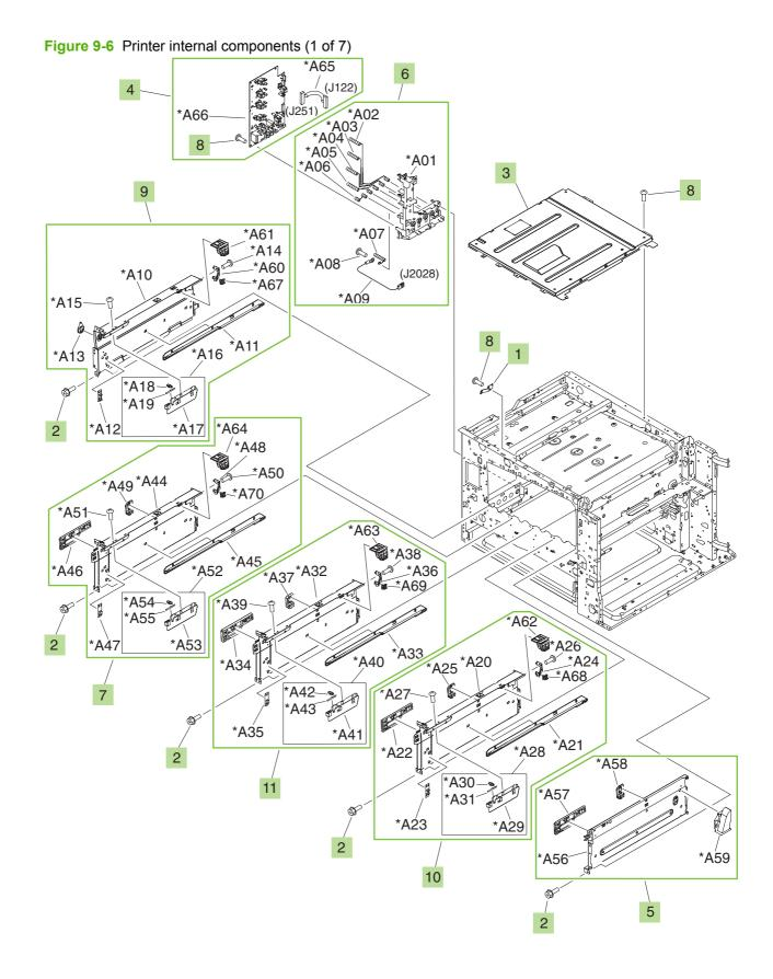
Table 9-4 Printer internal components (1 of 7)
