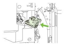
4. Push the staple cartridge unit into the stapler unit until it clicks into position.
