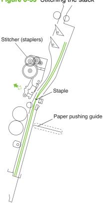
The booklet maker unit folds the stitched stack, and then feeds it to where the stapling position matches the height of the paper-pushing plate and the paper-folding roller nip. The paper-positioning plate moves the stack forward and the guide plate descends so that the paper-folding rollers directly face the stack.
