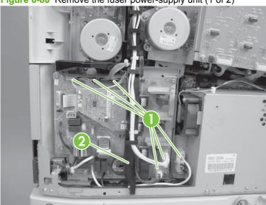
2. Remove two screws (callout 1), and then remove the fuser power-supply unit.
