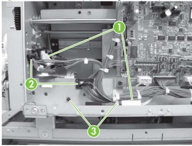
Disconnect two connectors (callout 1) and release four edge saddles (callout 2). Remove three screws (callout 3), and then remove the paper-folding/paper-pushing motor base (callout 4).
