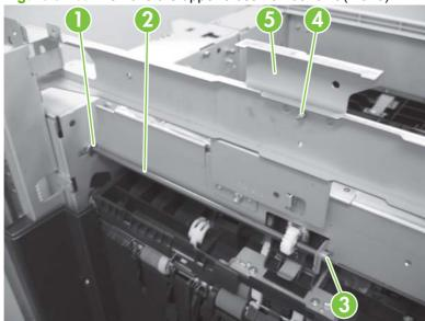
Disconnect four connectors (callout 1), and then remove the wire from the six wire retainers (callout 2).
