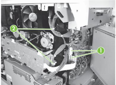
3. Remove two screws (callout 1), and then remove the laser/scanner-fan duct (callout 2).
