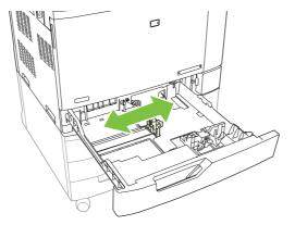
3. Adjust the paper-length guide by squeezing the adjustment latch and sliding the guide to the size of the paper being used.
