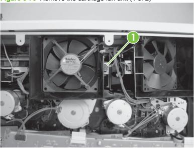
2. Release one tab (callout 1), and then remove the cartridge fan unit (callout 2).
