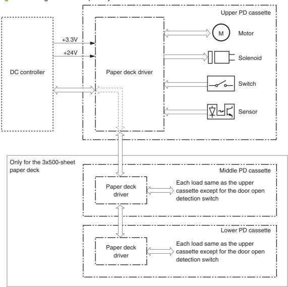
The input trays contain several motors, solenoids, sensors, and switches, as described in the following table.
