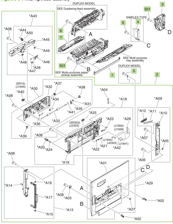
Figure 9-5 Printer right-door assembly
