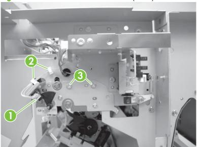
3. Remove return roller unit from the front side.
