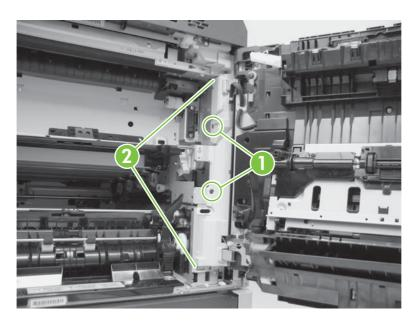
5. Remove one grounding screw (callout 1), disconnect three connectors (callout 2), and then lift the right-door assembly (callout 3) to remove it.
