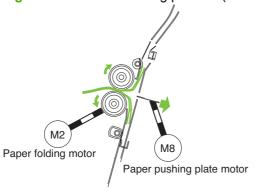
Figure 8-85 Double-folding process (5 of 5)
