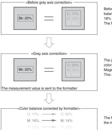
Before the gray axis correction, the process color balance equivalent to Bk 20% is; Cyan 17%, Magenta 18% and Yellow 16%.
