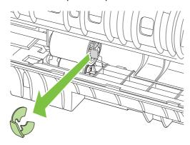
5. Remove the upper roller by sliding it to the right. Rotate the lower roller and then grasp the blue plastic tab and pull the roller off the rod.
