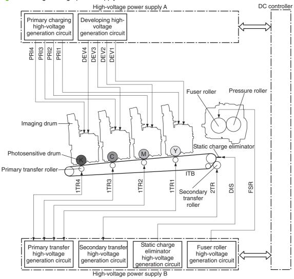
The high-voltage power supply contains several separate circuits.
