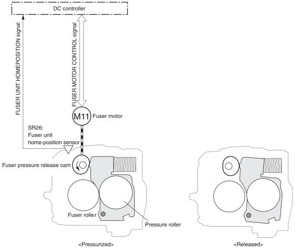
The pressure roller is depressurized under the following conditions:
