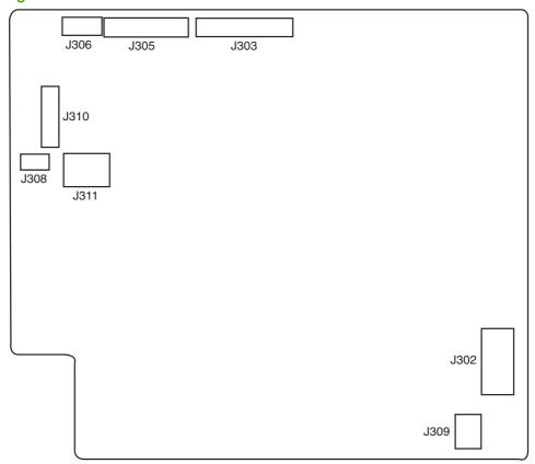
Figure 7-19 Duplexing driver PCA
