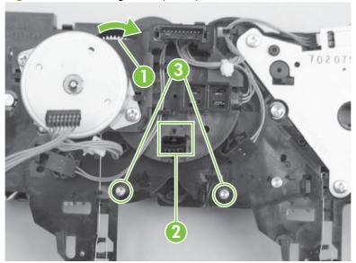
5. Install the print-cartridge drive unit over the long pins in the main drive unit. Remove all pins (callout 1), disengage locks, and reinstalled screws.
