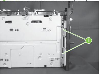
NOTE: Remove two screws (callout 1), and then remove the finisher-lock assembly (callout 2).
