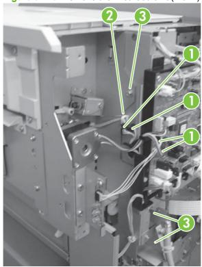
4. Remove three screws (callout 1), and then remove the support plate (callout 2).
