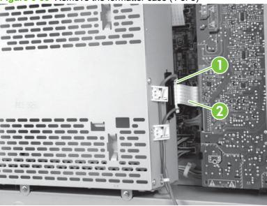
2. Disconnect one connector (callout 1), release three wire retainers (callout 2), and then remove five screws (callout 3).
