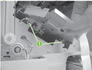
NOTE: When reinstalling, make sure the tabs are positioned correctly (callout 1).
