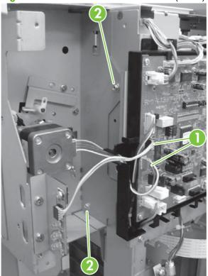
**5**. Remove the two screws from the front side of the inlet feed unit (callout 1).
