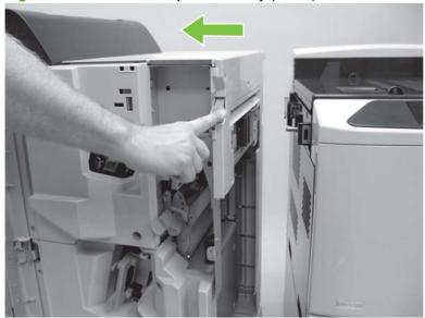
NOTE: When reassembling, adjust the wheels on the output accessory to ensure correct attachment to the printer.
