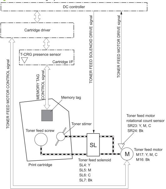
The toner-feed screw rotates, picks up the toner particles, and transports them into the imaging drum. The toner stirrer rotates at the same time as the toner-feed screw to keep the toner particles from sticking to each other.
