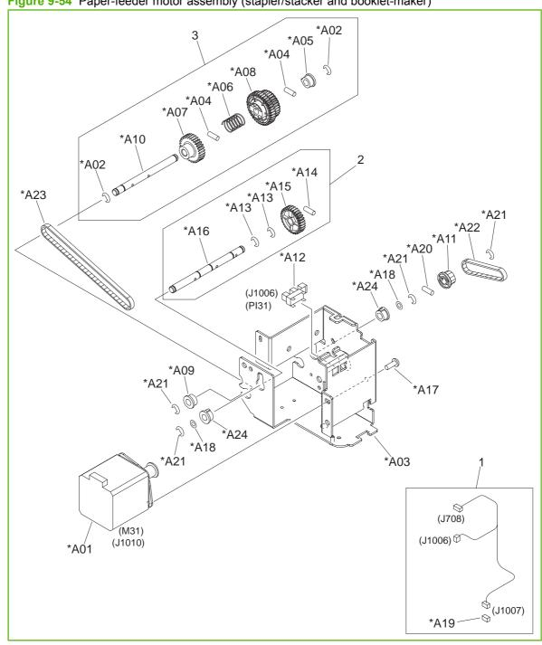
Figure 9-54 Paper-feeder motor assembly (stapler/stacker and booklet-maker)
