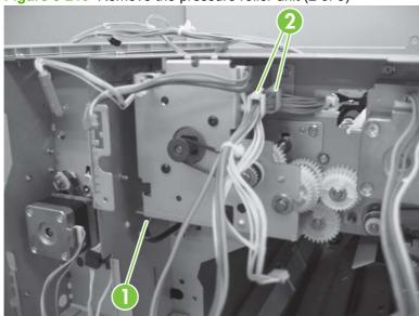
4. Remove three screws (callout 1), and then remove the drive unit (callout 2).
