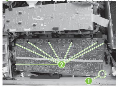
NOTE: When reassembling, set the bottom tab of the high-voltage power supply PCA (A) first. Ensure that the contact spring (callout 1) can be seen from the twelve confirmation windows.
