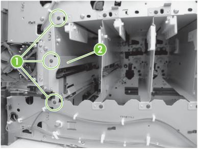
2. Disconnect the two connectors (callout 1) and lift the color-misregistration/image-density sensor unit to remove it.
