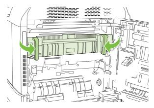
**b.** Rotate the fuser-release levers down to open them.
