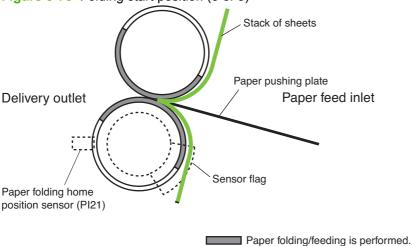
Figure 8-79 Folding start position (4 of 5)
