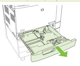
2. Adjust the paper-width guide by squeezing the adjustment latch and sliding the guide to the size of the paper being used.
