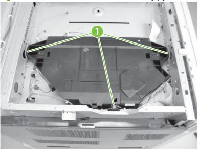
△ CAUTION: Use care when replacing the cables for the laser/scanner assemblies. The traces on the cable ends can be damaged when reinserted.
