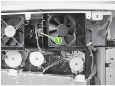
2. Release one tab (callout 1), and then remove the laser/scanner fan unit (callout 2).
