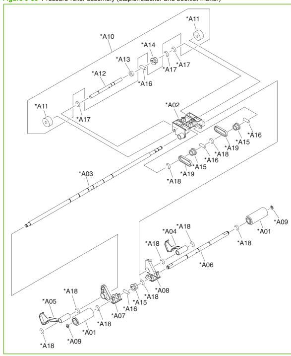
Figure 9-56 Pressure-roller assembly (stapler/stacker and booklet-maker)
