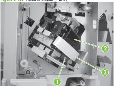
Disconnect three connectors (callout 1), release one tab (callout 2), and then remove the PCA (callout 3).
