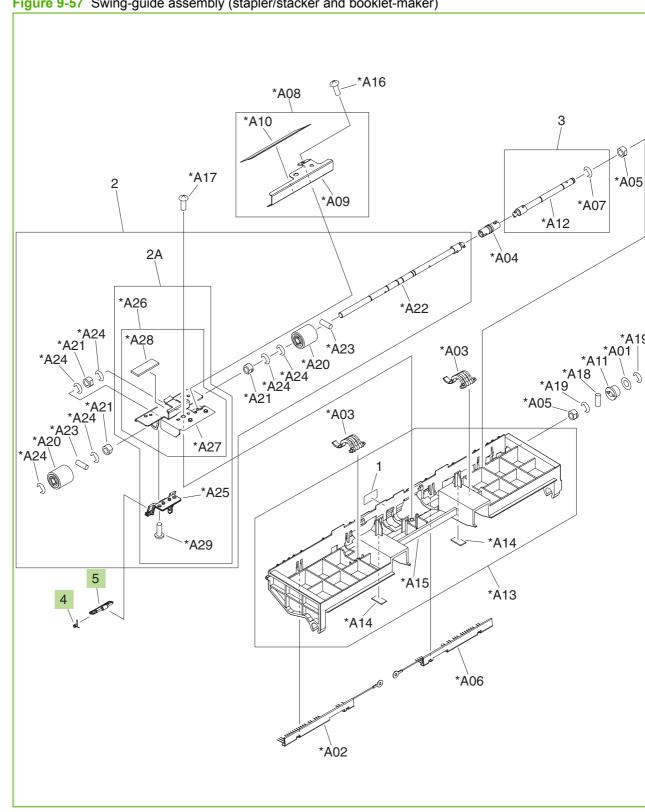
Figure 9-57 Swing-guide assembly (stapler/stacker and booklet-maker)
