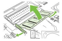
**10.** Remove the new DIMM from the antistatic package. Locate the alignment notch on the bottom edge of the DIMM.
