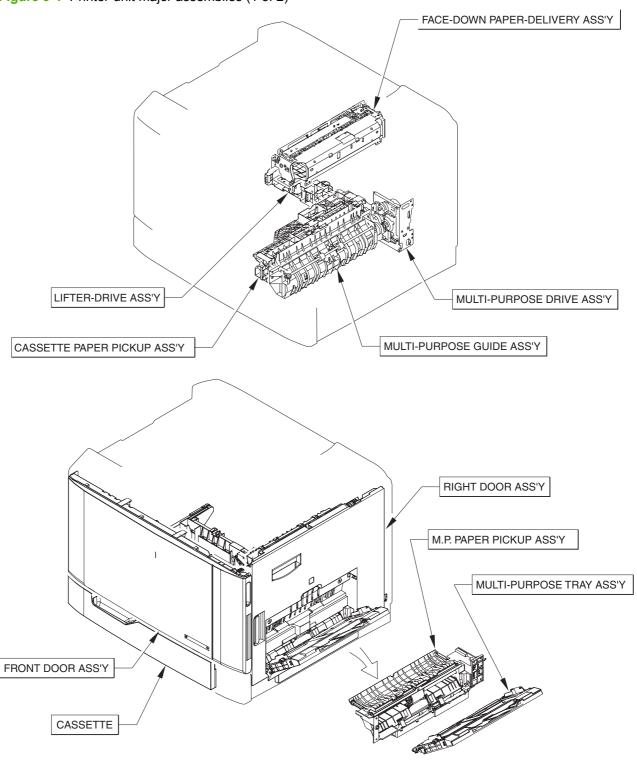
Figure 9-2 Printer-unit major assemblies (2 of 2) DUPLEX MODEL
