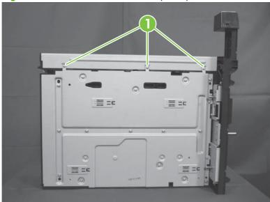
3. Remove three screws with washers (callout 1), and then release three tabs (callout 2). Release the bottom of the rear cover (callout 3) first and then lift to remove.
