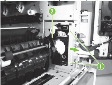
7. Remove two connectors (callout 1), one wire retainer (callout 2), and one ground screw (callout 3).
