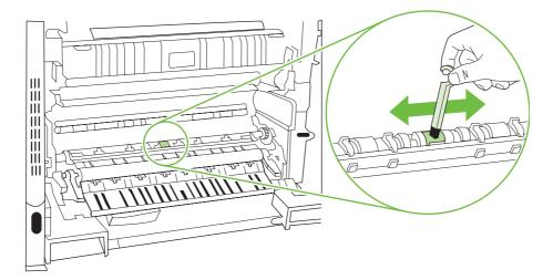
5. Close the transfer access panel, and replace the cleaning brush in its holder.
