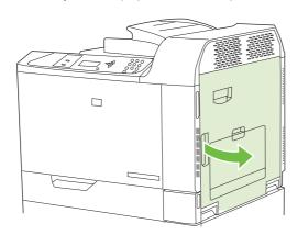
4. If paper is jammed below the duplexing unit, gently pull the paper downward to remove it.
