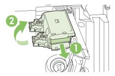
**4.** Grasp the edges of each staple cartridge and pull up firmly to remove the staple cartridges from the staple cartridge unit.
