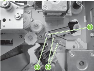
Unhook the swing pressure rack (callout 1) from the swing unit center hook. 4.
