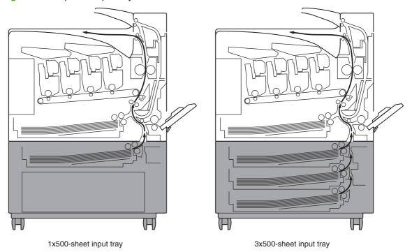
These additional trays are each controlled by paper-deck drivers, which contain a microcomputer. The paper-deck drivers receive commands from the DC controller. If the DC controller is unable to communicate with a paper-deck driver, it notifies the formatter that the optional input tray is not connected correctly.
