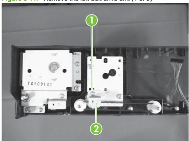
3. Remove two screws (callout 1), and then remove the left-belt drive unit (callout 2).
