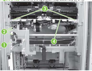
NOTE: When attaching the operation-tray assembly, do not mount the Mylar sheet (callout 1) on top of the stack trailing-edge assist guide (callout 2).
