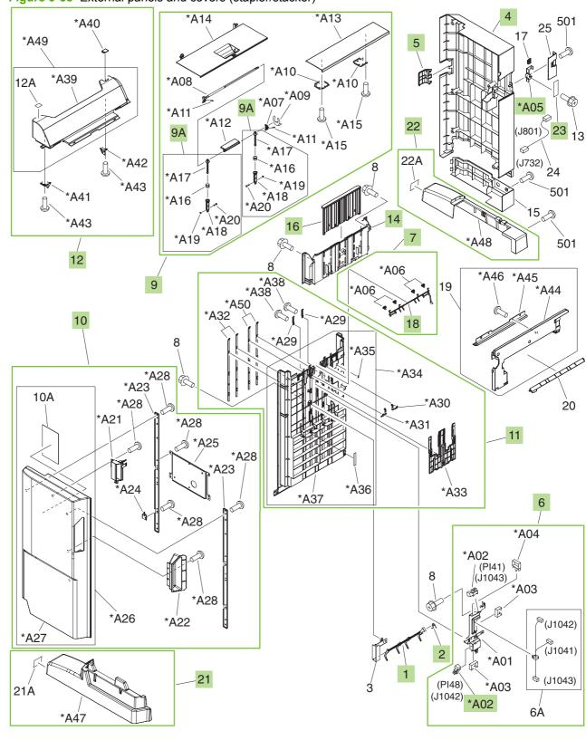
Figure 9-38 External panels and covers (stapler/stacker)
