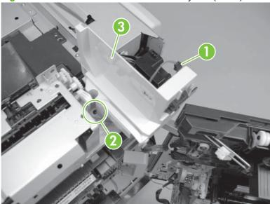
2. Remove two screws (callout 1), release one tab (callout 2), and then remove the gear cover (callout 3).
