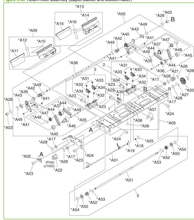
Figure 9-55 Return-roller assembly (stapler/stacker and booklet-maker)
