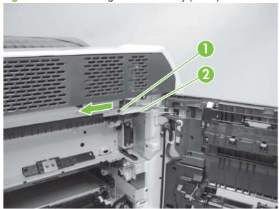
4. Remove two screws (callout 1), release the two tabs (callout 2), and then remove the right inner cover.
