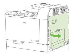
2. Lift the green handle on the transfer-access panel and open the panel.
