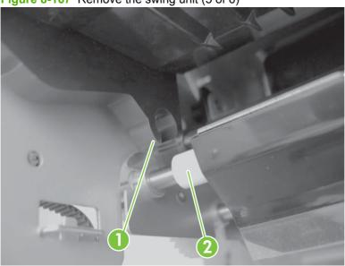
△ CAUTION: When reinstalling the swing unit, make sure the grounding plate (callout 1) is positioned so that the bottom of the grounding plate rubs against the metal plate when the swing arm moves up and down. Also make sure the pins (callout 2) are inserted correctly and the swing-pressure guide is flush (callout 3).
