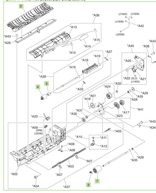
Figure 9-17 Printer multi-purpose paper-pickup assembly
