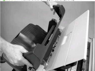
NOTE: When replacing, hook the two tabs of the left-upper cover (callout 1) under the steel plate located under the top door.
