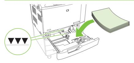
NOTE: For best performance, fill the tray completely without splitting the ream of paper. Splitting the ream can cause a multifeed problem. The capacity of the paper tray can vary. For example, if you are using 75 g/m² (20 lb) paper, the tray holds a full ream of 500 sheets. If the media is heavier, the tray will not hold a full ream. Do not overfill the tray.
