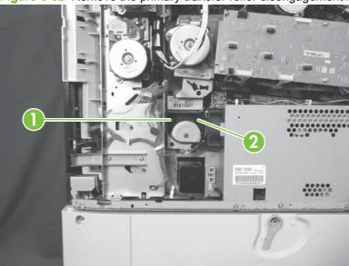
2. Disconnect one connector (callout 1). Remove three screws (callout 2), and then remove the primary-transfer roller disengagement motor (callout 3).
