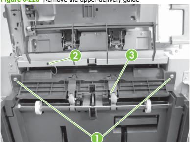
Figure 8-220 Remove the upper-delivery guide
