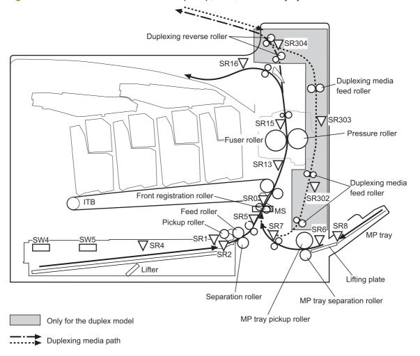
Table 5-13 Switches and sensors for the pickup, feed, and delivery system
