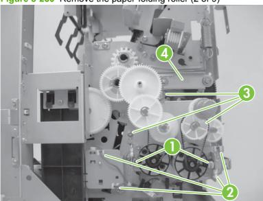
Remove one screw (callout 1), one spring retaining plate (callout 2), and two tension springs (callout
