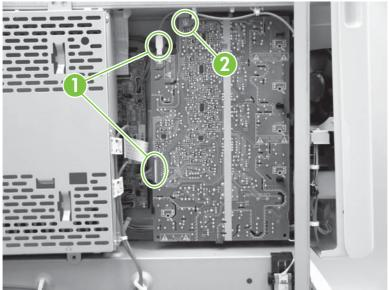
2. Release six tabs (callout 1), and then remove the high-voltage power supply PCA (B)
