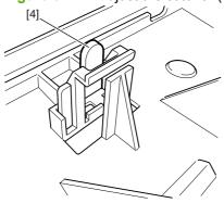
5. To adjust the front stitcher, remove the front guide plate (callout 4) and center guide plate (callout 6). To adjust the rear stitcher, remove the center guide plate (callout 6) and the rear guide plate (callout 7) (one screw each).
