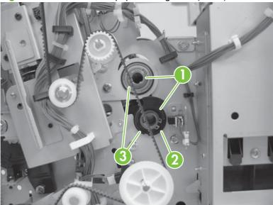
From the front, remove two c-rings (callout 1), remove two gears (callout 2), and then remove two bearings (callout 3).
