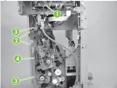
6. Remove four screws (callout 1), and then remove two brackets (callout 2).
