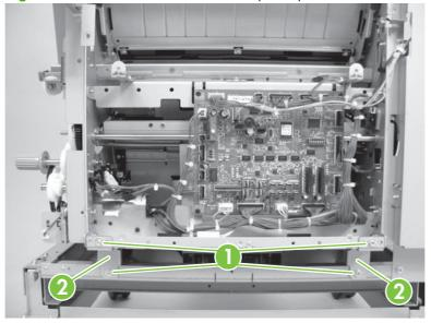
7. Remove three screws (callout 1), and then remove the saddle unit (callout 2) from the paper-feed side.
