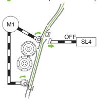
3. The solenoid turns on when the next sheet arrives, and the feed plate comes into contact.
