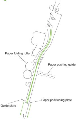
The paper-pushing plate moves the stack to the paper-folding rollers that hold the stack at its center and fold it. The paper-folding rollers and delivery roller then output the stack to the output bin.
