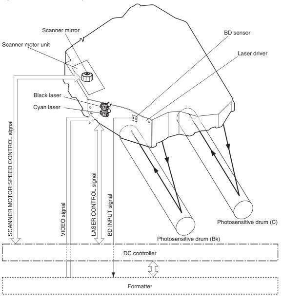
The DC controller determines that a laser/scanner has failed when any of the following conditions occurs:
