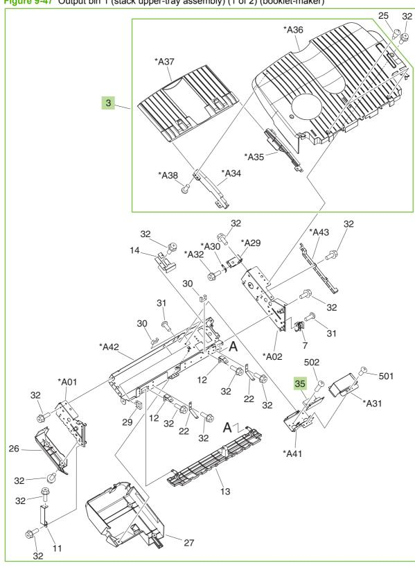
Figure 9-47 Output bin 1 (stack upper-tray assembly) (1 of 2) (booklet-maker)
