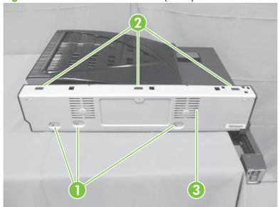
Figure 8-106 Remove the rear cover (4 of 4)
