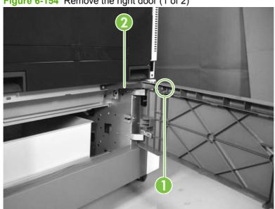
3. Release one tab (callout 1), and then remove the stopper (callout 2). Lift the right door (callout 3) to remove it.
