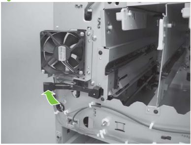
NOTE: Any time a cartridge is installed or removed while the covers are removed, the door interlock must be cycled to simulate opening and closing the top cover in order for the engine to recognize the change. When the covers are installed, the door switch and fuser interlock are automatically operated. When the covers are removed, you must perform these steps manually.
