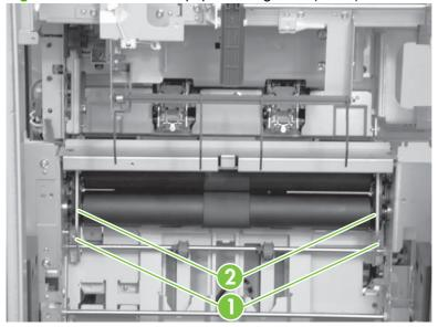
9. Slide the two paper-folding rollers to the front, and then pull them out in the delivery direction.
