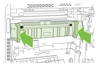
**f.** Rotate the fuser-release levers up to lock the fuser into place.
