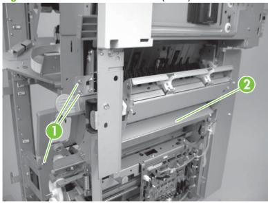
NOTE: Install the saddle unit so that the Mylar (callout 1) at the front-upper side of the saddle is on the outside of the delivery-guide plate (callout 2). A delivery fault will occur if it is on the inside.
