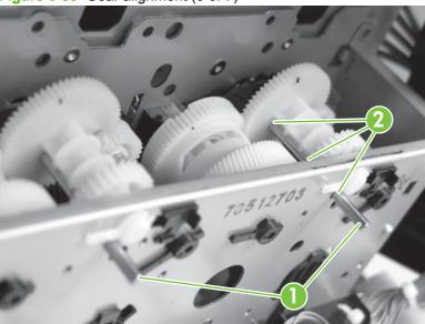
On the print-cartridge drive unit, rotate the top gear (callout 1) clockwise until the arrows align (callout 2). Insert the two short pins (callout 3).
