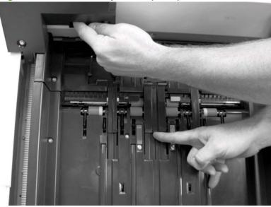
NOTE: When reinstalling, be careful not to twist the tray cable. Lift the shutter to prevent damage to the stack-delivery gate. See Move output bins 1 and 2 on page 679
