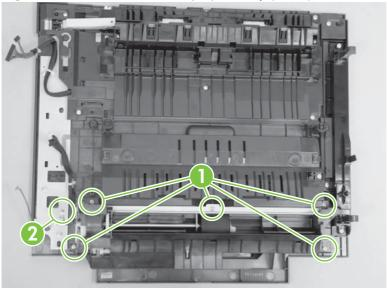
3. Remove the MP-tray pickup unit and the MP tray together.
