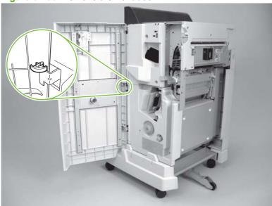
2. Lift the front door off the three hinges (callout 1) to remove.
