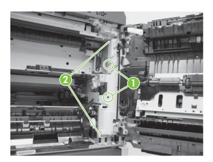
5. Lift the secondary transfer unit stopper (callout 1), and then pull it forward to remove it.
