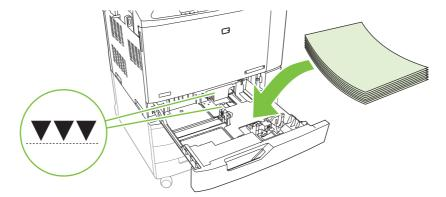
3. Slide the tray into the product. The control panel shows the tray type and size configuration. To specify custom dimensions, or if the type is not correct, press the checkmark button ✓ when the control panel prompts to change the size or type.
