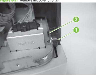
2. Release one tab (callout 1) while pulling out on the bottom left corner (callout 2). Slide the left cover (callout 3) in the direction that the arrow indicates.
