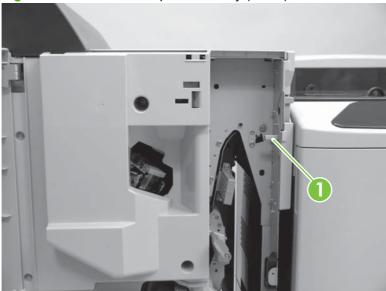
4. Press down the release button while moving the output accessory away from the printer.
