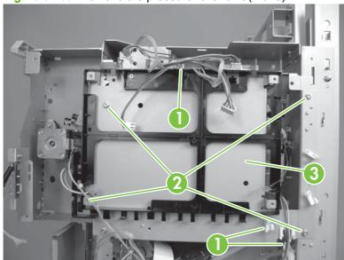
3. Disconnect one connector (callout 1) and release two wire retainers (callout 2).
