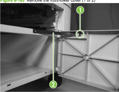
3. Clear the bottom pin (callout 1), and then lift the front-lower door (callout 2) to remove it.
