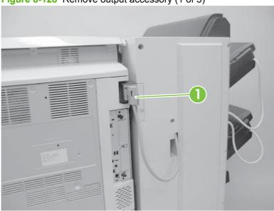
3. Open the front door to the output accessory and loosen the thumb screw (callout 1).
