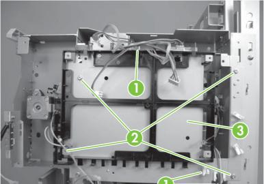
Figure 8-190 Remove the operation-tray assembly (4 of 6)
