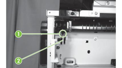
Figure 6-131 Remove the pressure-release sensor unit (2 of 2)
