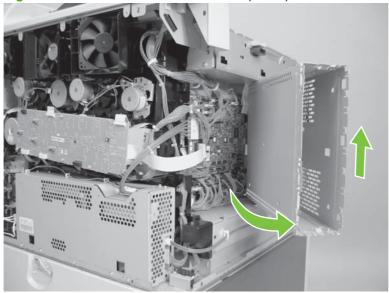
NOTE: When reassembling, insert the C-shaped hinge on the top of the formatter case into the round hole.
