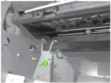
6. Slide the bushing (callout 2) to the inside and lift the swing unit (callout 1) to remove.
