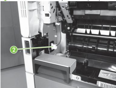
**5.** Remove one screw (callout 1), release one tab (callout 2), and then lift the left ITB guide (callout 3) to remove it.
