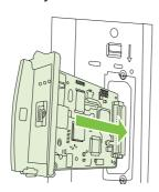
5. Insert and tighten the retaining screws that came with the print server card.
