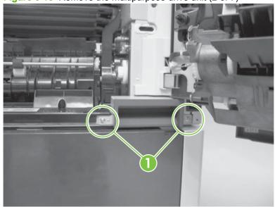
**ENWW** Removal sequence 1 215 4. Remove two screws (callout 1), release two tabs (callout 2), and then remove the right inner cover.
