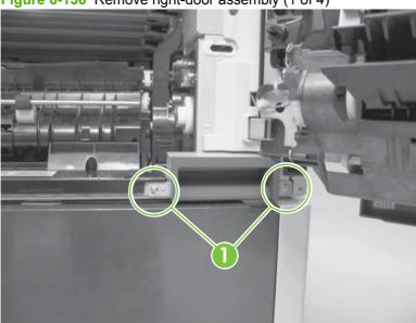
3. Remove one screw (callout 1). Slide the right door arm (callout 2) in the direction indicated to remove it.
