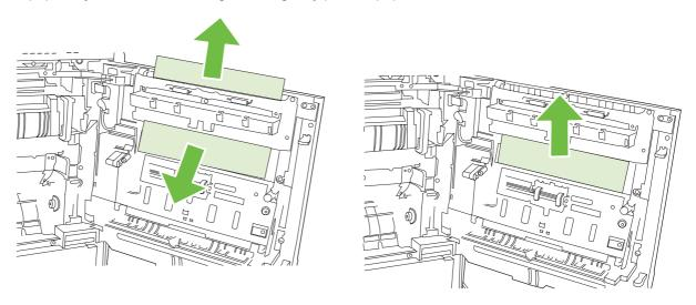
**6.** Lift the paper-feed cover on the inside of the right door. If jammed paper is present, gently pull the paper straight out to remove it.
