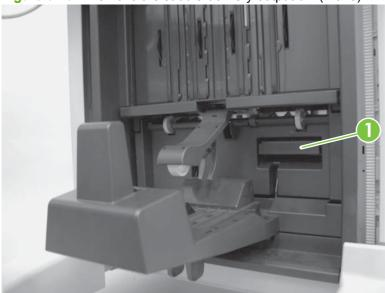
2. Remove the door pin (callout 1) to release the booklet-delivery output bin unit.
