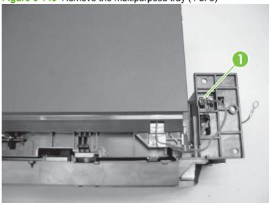
5. With the door closed, use a flat blade screw driver to pry the left side out. Pull the tray in the directions indicated to remove.
