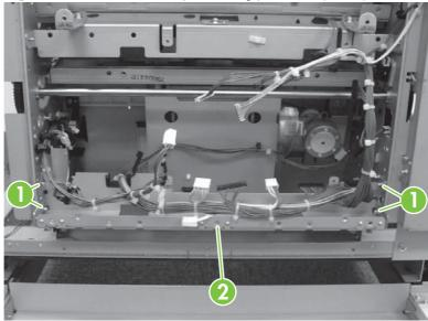
6. Disconnect two connectors (callout 1) and release two wire retainers (callout 2). Remove two screws (callout 3), shift the positioning plate unit (callout 4) forward, and then remove it from the paper-feeding side.
