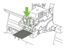
Pull the staple cartridge unit forward, and swing it downward to the original position. Push in on the handle to lock it into position.
