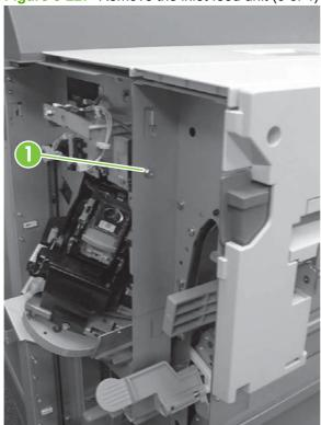
Open the top door (callout 1), and then remove the inlet feed unit (callout 2).
