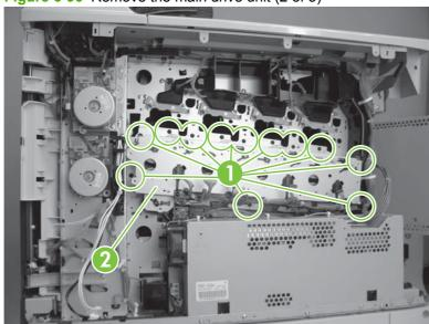
△ CAUTION: Do not remove screws that hold the main drive unit together.
