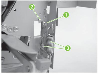
**5.** Remove one screw (callout 1), one spring-retaining plate (callout 2), and two tension springs (callout 3).
