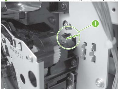
Figure 6-92 Incorrect position of print-cartridge drive unit (7 of 7)
