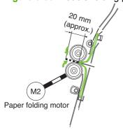
**4.** The paper-folding rollers rotate forward to push the stack forward. The paper-pushing plate returns to its home position.
