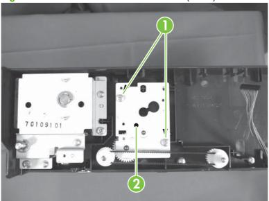
NOTE: When reassembling, be sure to attach the IPTU drive using two washers with each screw.
