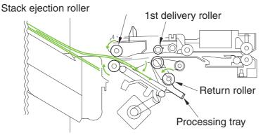
5. The first and second paper delivered to the processing output bin are aligned and then delivered to the output bin.
