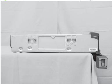
The connector can be damaged when the IPTU is placed on a table as shown below.
