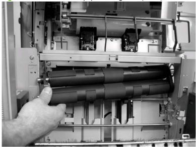
△ CAUTION: When reinstalling, attach the gears (callout 1) so that the slots (callout 2) of the paper-folding rollers face each other to ensure gear alignment.
