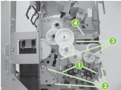
5. Remove four screws (callout 1), and then remove the stay (callout 2). Do not remove the wire retainer on the stay.
