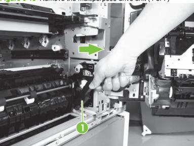
Figure 6-15 Remove the multipurpose drive unit (4 of 7)
