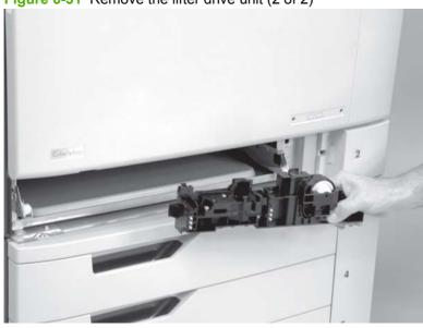
NOTE: When reassembling, ensure that the lifter drive unit is unlocked (callout 1). If the lifter is locked (callout 2), the lifter will not function correctly.
