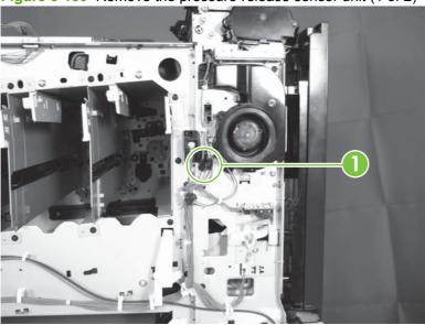
2. From the right side of the product, remove one screw (callout 1), and then the pressure-release sensor unit (callout 2).
