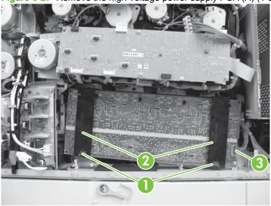
2. Remove one screw (callout 1), release seven tabs (callout 2), and then remove the high-voltage power supply PCA (A).
