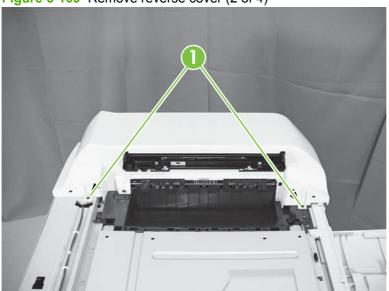
2. Push in on the lower-right corner (callout 1) and then pull out on the lower-right and upper-right tabs (callout 2). Move to the other side of the product, and then carefully move one side of the cover at a time to remove. If you feel resistance, make sure you are clearing the black plastic part on the lower-right side. Lift the cover up and over this part, and then continue to move each side of the cover to remove.
