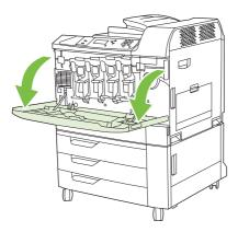
2. Grasp the handle of the used print cartridge and pull out to remove.
