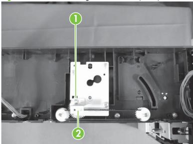
6. Remove three screws (callout 1), and then remove the right-belt drive unit (callout 2).
