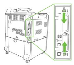
Gently pull on the black tabs to pull the formatter board from the product. Place the formatter board on a clean, flat, grounded surface.
