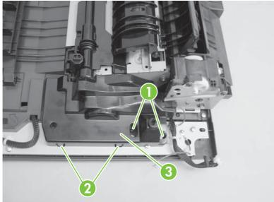
3. Remove five screws (callout 1), one wire retainer (callout 2), one connector (callout 3), and then remove the duplexing feed unit.
