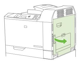
2. If paper is visible inside the right door, gently pull the paper downward to remove it.
