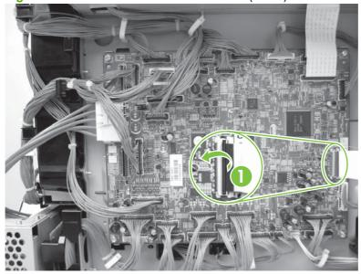
2. Remove six screws (callout 1), and then remove the DC controller PCA.
