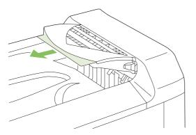
2. If no jammed paper is visible in the duplex output area, open the duplex switchback tray. Gently pull the jammed paper to remove it.
