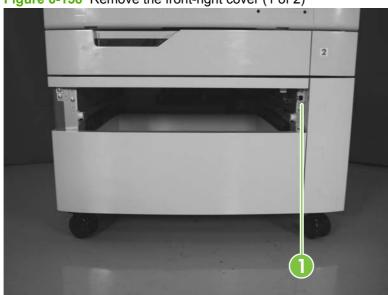
Open the right door. Remove one screw (callout 1). Lift the front-right cover (callout 2) to remove it.
