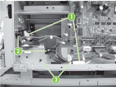
Disconnect two connectors (callout 1) and release four wire retainers (callout 2). Remove three screws (callout 3), and then remove the paper-folding/paper-pushing motor base (callout 4).
