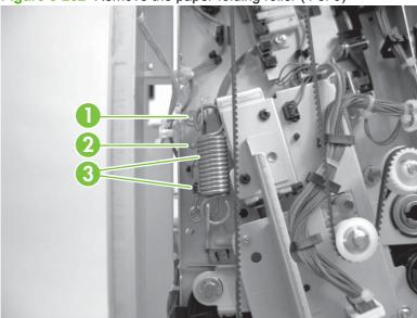
6. From the rear side, remove two c-rings (callout 1), remove one sensor flag (callout 2), and then remove two bearings (callout 3).
