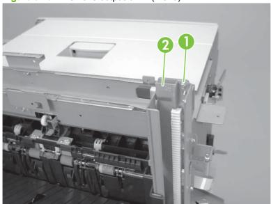
Remove two screws (callout 1), release two wire retainers (callout 2) and then disconnect two connectors (callout 3).
