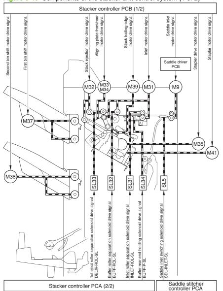
Figure 8-46 Components of the stacker unit control system (1 of 2)
