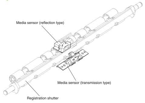
The DC controller uses the information from the media sensors to determine the paper type, and it notifies the formatter. The DC controller notifies the formatter of a paper-type mismatch if any of the following conditions exist:
