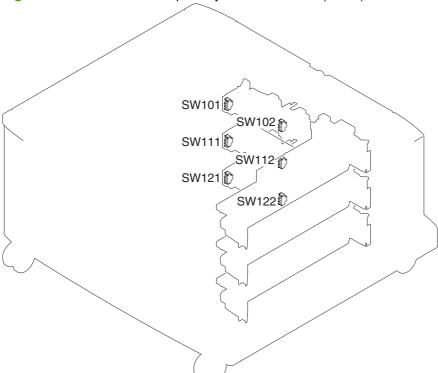
Figure 7-51 3 x 500-sheet input-tray switch locations (2 of 2)
