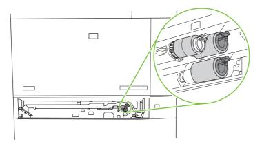
**3.** Turn the roller, and then grasp the plastic tab and pull the roller off the rod. Repeat the process for the other rollers. Recycle the used rollers.
