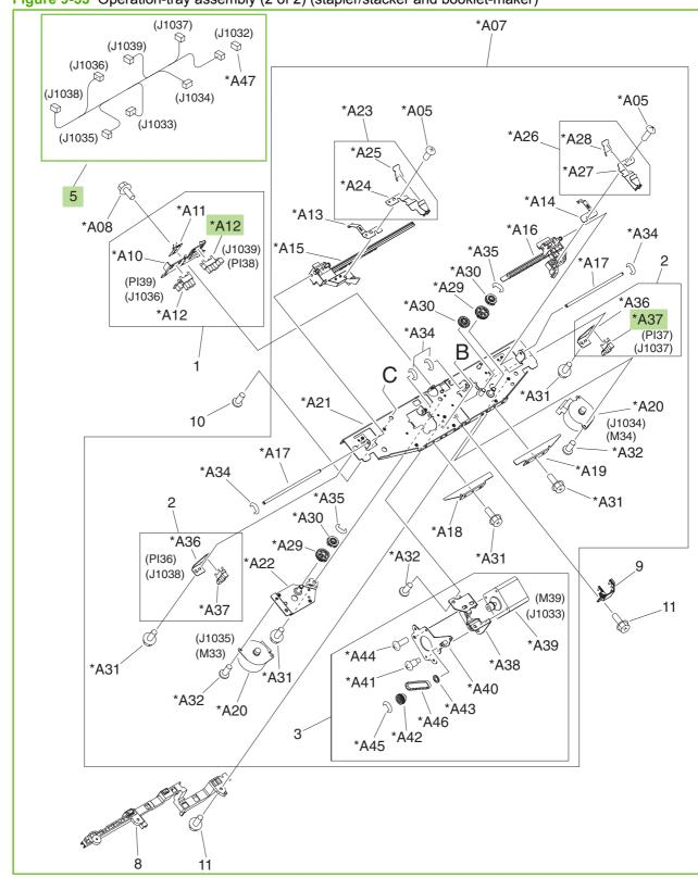
Figure 9-53 Operation-tray assembly (2 of 2) (stapler/stacker and booklet-maker)
