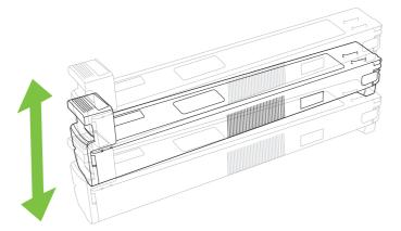
7. Align the print cartridge with its slot and insert the print cartridge until it clicks into place.
