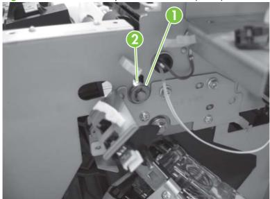
9. Slide the pressure roller unit (callout 1) to the rear side, and then remove from the front side.
