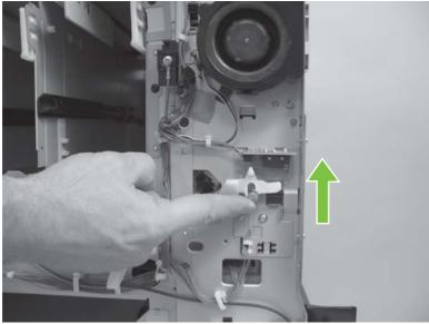
Figure 7-15 Front-door switch on the left side
