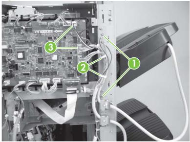
Hold output-bin 1 to prevent the bin from falling. Insert your finger in the hole at the rear side of the bin and release the lift-motor gear. Lift the shutter to prevent damage to the stack-delivery gate. Lift output-bin 1 to remove.
