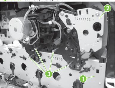
2. Reinstall the main drive unit. Push the black locks (callout 3) to the left while rotating the top gears (callout 1) on the main drive unit until they lock into position. The large holes (callout 2) should point to the right (3 o'clock position).
