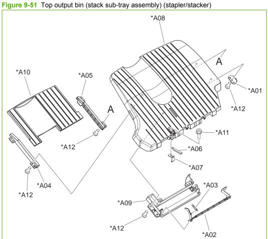
Table 9-39 Top output bin (stack sub-tray assembly) (stapler/stacker)
