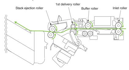
When the product sorts paper size other than A4, B5, or LTR or when set to staple and sort, copies are delivered to the processing output bin for aligning and stapling and then ejected using the stack trailing-edge assist.
