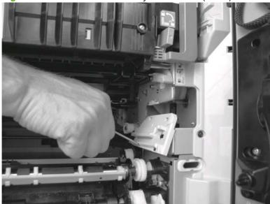
3. Close the secondary transfer unit. On the left side, release one tab (callout 1), and then lift the connector cover (callout 2) to remove it.
