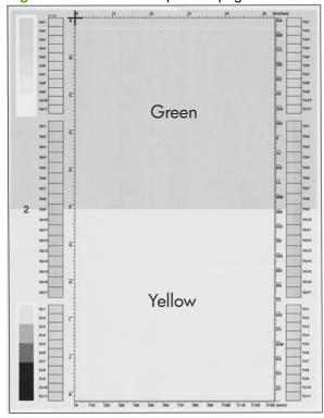
Yellow cannot be easily seen unless combined with cyan, so half of each page is yellow and the other half is an amplified version of yellow problems (green half). Compare the yellow on page one with the corresponding green on page two for defects. You can also check the cyan page for defects.
