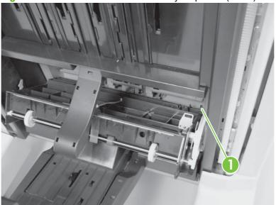
3. Release one wire retainer (callout 1) and disconnect two connectors (callout 2). Remove the booklet-delivery output bin unit.
