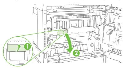
3. If paper is visible entering the bottom of the fuser, gently pull downward to remove it.
