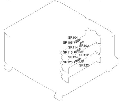
Figure 7-37 3 x 500-sheet input-tray sensor locations (2 of 2)
