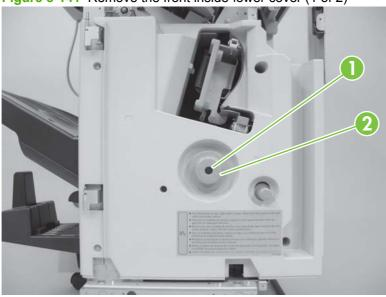
3. Remove four screws (callout 1) and remove the front inside-lower cover (callout 2).
