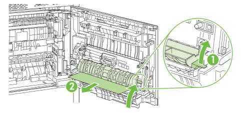
7. Lift the green handle on the transfer assembly and open the panel.
