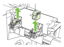
5. Unpack the new cartridges and remove the plastic packing lock from each one.
