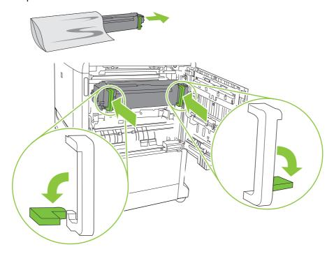
Rotate the fuser-release levers up to lock the fuser into place.
