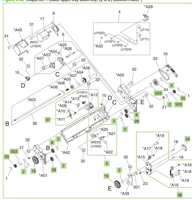
Figure 9-48 Output bin 1 (stack upper-tray assembly) (2 of 2) (booklet-maker)
