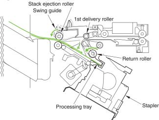
When the last sheet is aligned, the stacker controller PCA moves the aligning plate to the alignment position with the aligning motor (M33/M34) (the paper is held by the aligning plate). Then the stacker controller PCA staples at the specified staple position. After stapling, the stacker controller PCA starts the swing motor (M36) and lowers the swing guide. Then the stack is ejected by the stack-delivery roller, return roller, and stack trailing-edge assist guide.
