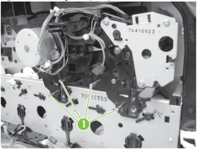
△ CAUTION: Be sure to remove all pins (callout 1). Failure to do so can damage the product.
