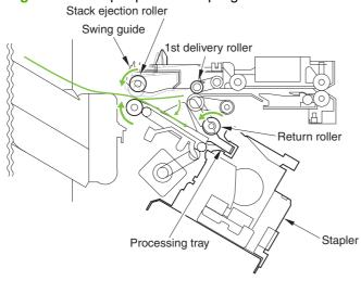
Figure 8-27 Rollers and sensors for stapling
