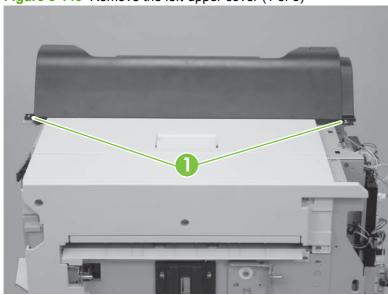
With the top door open, tilt the left-upper cover to the right, and then slide it to the left to remove.
