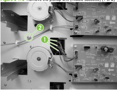
3. Remove one screw (callout 1). Grasp the pickup unit (callout 2), and then shift to the left to release the right shaft. Pull the unit forward to remove it.
