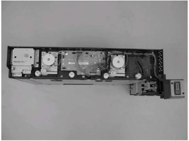
NOTE: When reassembling, tighten the screws from left to right.
