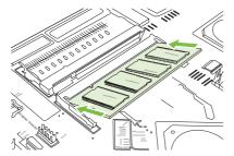
12. Push down on the DIMM until both latches engage the DIMM.
