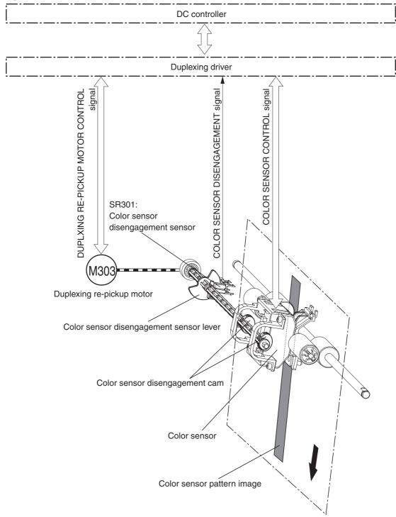
The color sensor engages or disengages based on the position of the color-sensor disengagement cam, which is driven by reversing the duplexing re-pickup motor.
