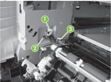
7. Slide the bushing (callout 1) out onto the rod.
