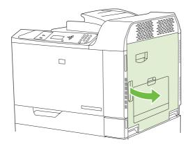
NOTE: If you are printing to very heavy banner paper, and the paper is still feeding in through Tray 1, you may need to cut the paper at the base of Tray 1 in order to open the right door and pull the paper free of the Tray 1 rollers.
