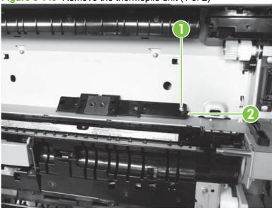
3. Disconnect two connectors (callout 1), and then remove the thermopile unit (callout 2).
