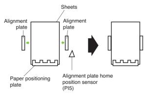
The alignment plates move away from the stack and then return (Second alignment).
