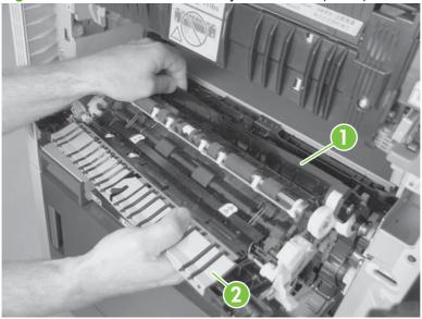
NOTE: Be sure to calibrate the media sensor from the **SERVICE** menu on the control panel after the secondary transfer unit has been replaced.
