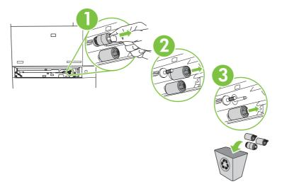
**4.** Remove each roller from its protective bag. Do not touch the rubber part of the new roller. Contaminants or scratching may result in poor print quality.
