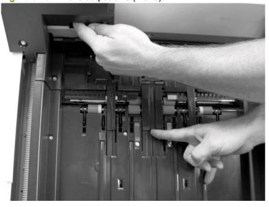
NOTE: If the stack-delivery gate (callout 1) comes off, retain the spring (callout 2) and reinstall. The spring ends (callout 3) fit in the slots provided.
