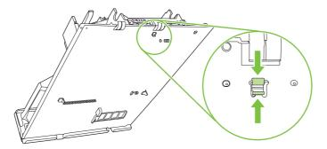
7. Rotate the end of the hard disk assembly upward until you can disengage the hinge tabs at the other end.
