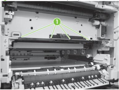
3. Remove the ITB duct.
