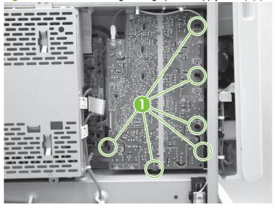
NOTE: When reassembling, ensure that the contact springs (callout 1) can be seen from the five confirmation windows. Failure to do so can cause print-quality issues.
