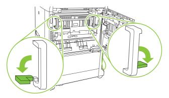
**5.** Grasp the fuser handles and pull straight out to remove the fuser. Recycle the used fuser following the instructions included with the new fuser.
