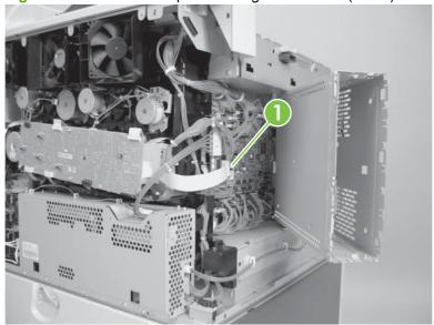
Disconnect seven connectors (callout 1), four screws (callout 2), and the print-cartridge driver PCA (callout 3).
