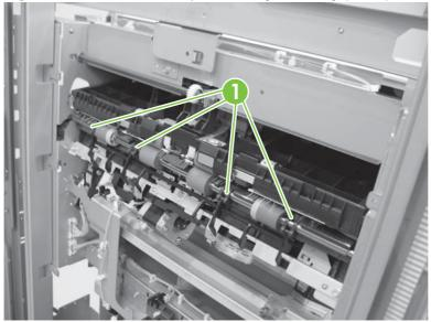
NOTE: When reinstalling, the small tab (callout 2) on each snap fastener must be inserted into a hole (callout 3). The sensor flag (callout 1) will not work properly if the tabs are not installed correctly.
