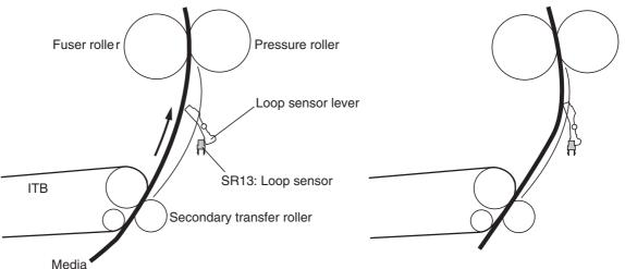
When the fuser roller and the pressure roller rotate slower than the secondary transfer roller.
