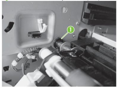
8. While tilting the feed guide (callout 1) backward, grasp the secondary transfer unit (callout 2) and slide it to the left. Release the right guide bar, and then remove the secondary transfer unit.
