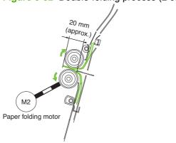
3. The paper-folding rollers rotate in reverse, pushing the stack backward 20 mm (reverse feeding).
