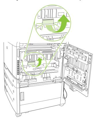
3. Remove the transfer roller, and then recycle it.
