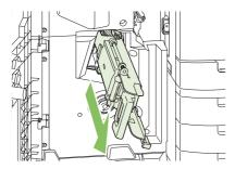
3. Grasp the small blue handle on the staple cartridge unit and pull it toward you, then swing the staple cartridge unit into an upright position.
