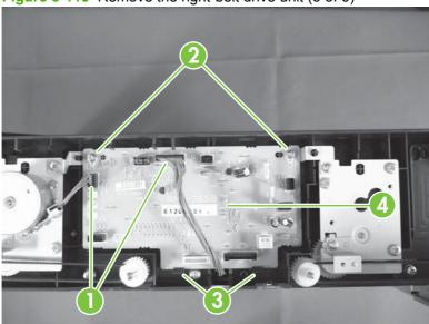
**5**. Remove one screw (callout 1), and then remove the belt cover plate (callout 2).
