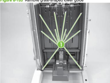
Figure 8-153 Remove grate-shaped lower guide
