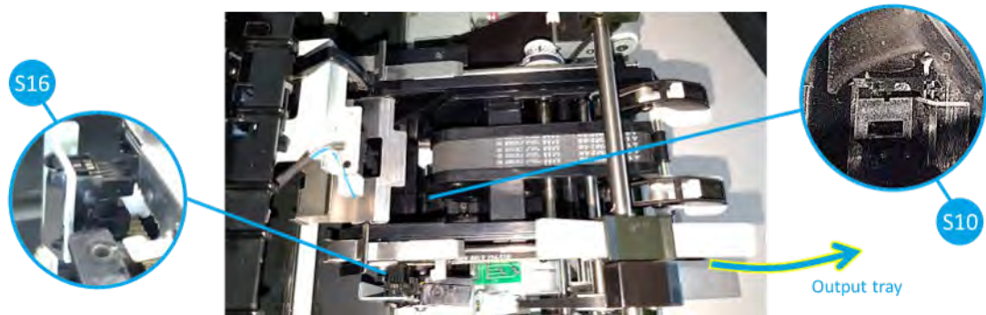
Figure 5-42 Inner finisher system - ejector unit detail view (2/3)
