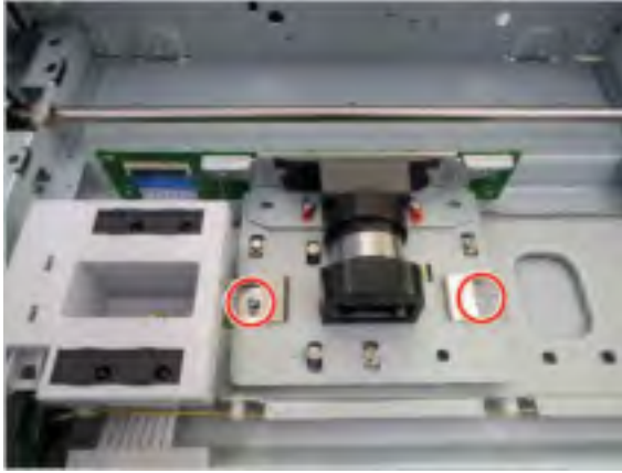
Figure 2-335 Remove screws and release scanner imaging unit
