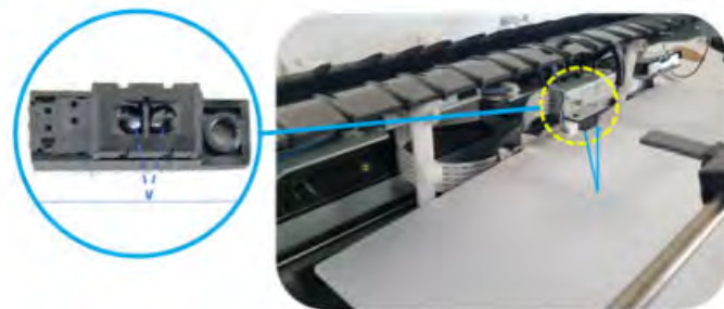
Figure 5-6 Inner finisher system - Photo emitter, detector (0604-001381)
