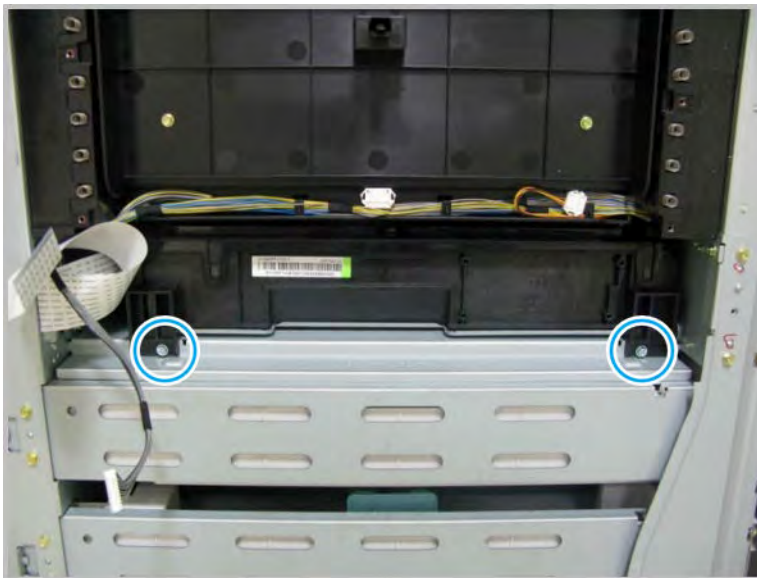
Figure 2-54 Remove the laser scanner assembly
