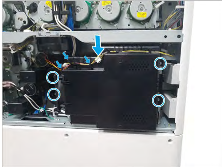
Figure 2-46 Remove the LVPS cover
