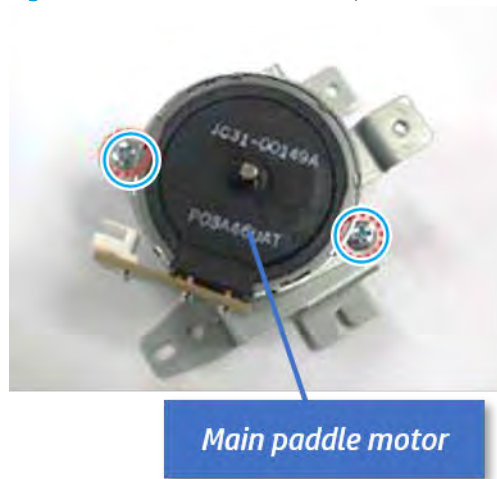
Figure 5-277 Remove the main paddle motor
