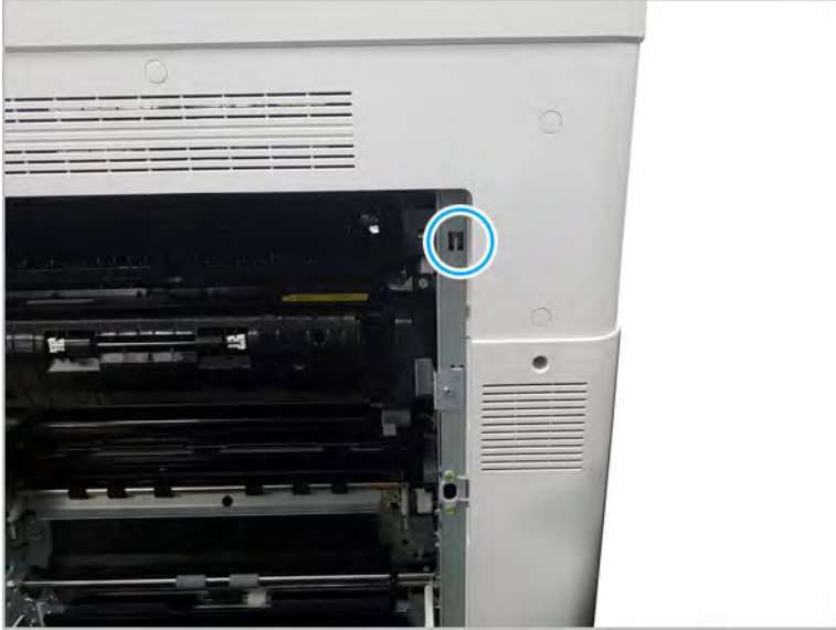
Figure 3-13 Defeat the front door interlock
