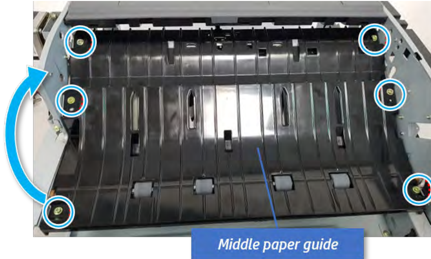
Figure 5-477 Open the middle paper guide
