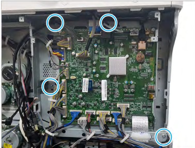
Figure 2-103 Remove the main board cage screws
