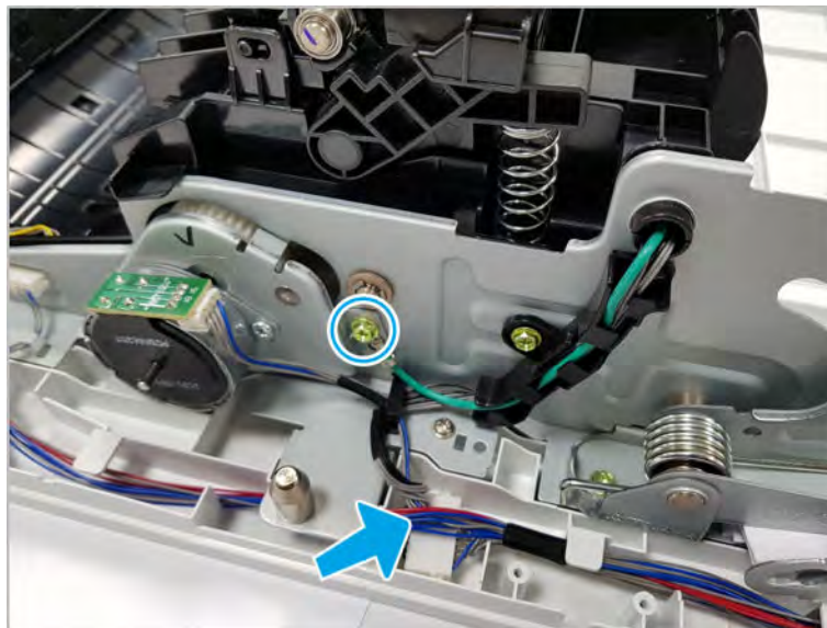
Figure 2-255 Release the wires
