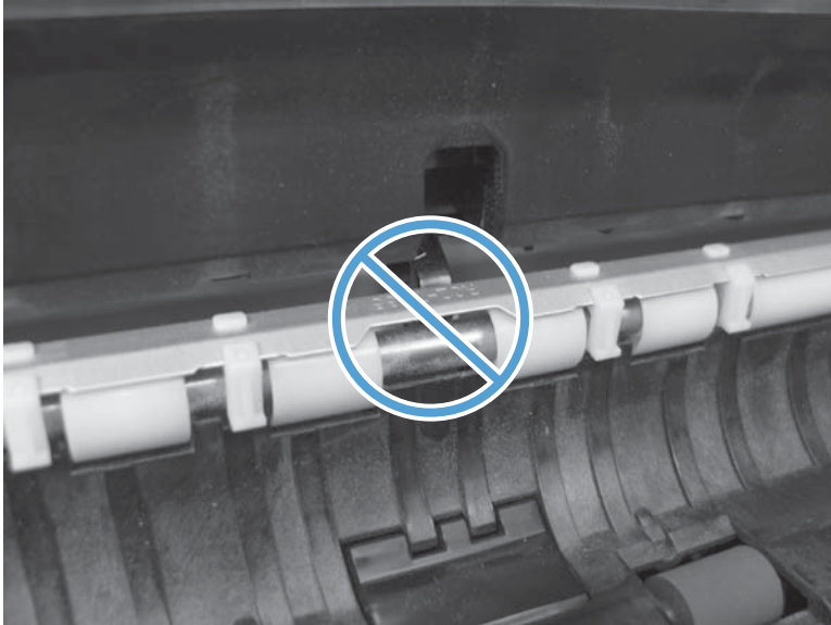
Figure 2-64 Paper pickup assembly sensor flag incorrectly installed
