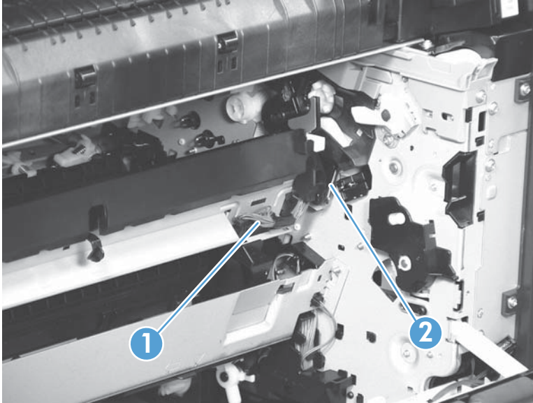
Figure 2-67 Remove the registration sensor assembly (2 of 4)
