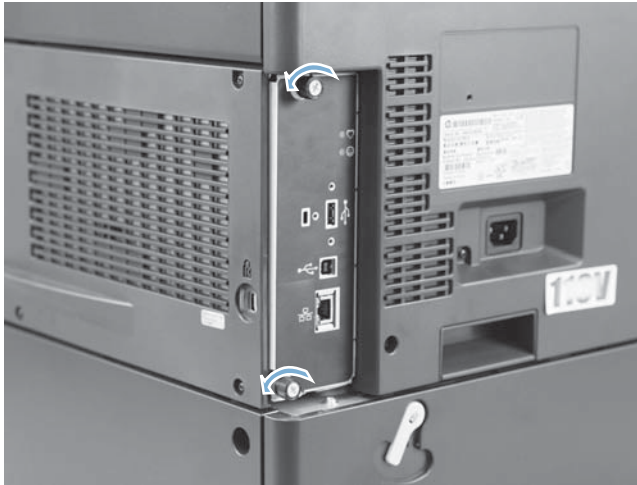
Figure 2-22 Remove the formatter (2 of 3)
