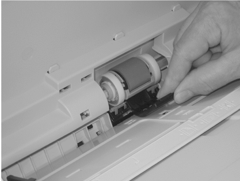
Figure 2-11 Remove the separation pad (Tray 1) (4 of 4)
