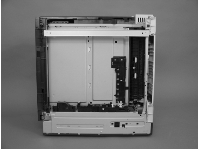
Figure 2-70 Remove the lifter-drive assembly (1 of 3)
