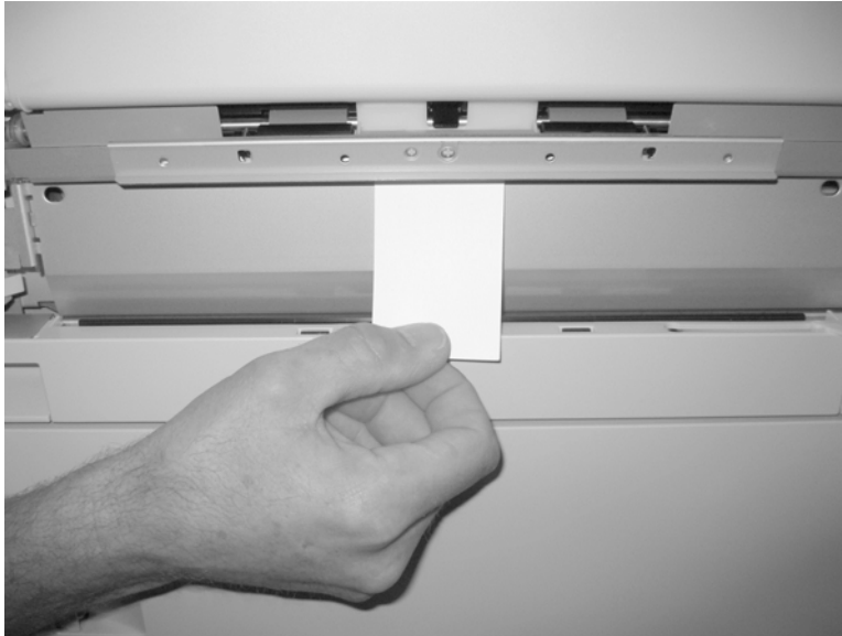
Figure 3-21 Test the Tray 3 feed sensor
