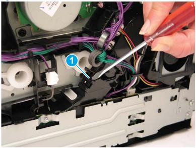
2. Release one tab (callout 1) on the rear of the fan duct cover, and then remove the fan duct cover (callout 2).
