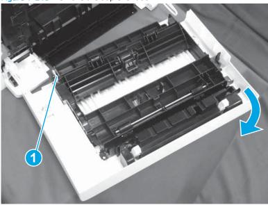
Step 9: Remove the rear door assembly (duplex models)
