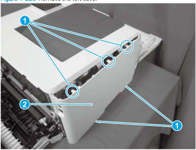
Step 5: Remove the rear cover (simplex models)
