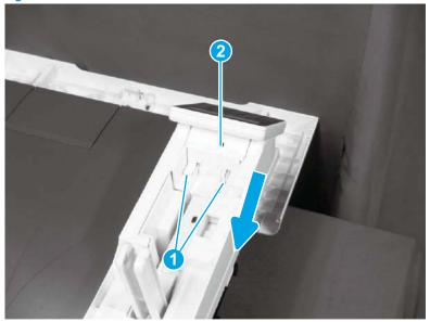
Release two tabs (callout 1), and then slide the control panel (callout 2) up to remove it.
