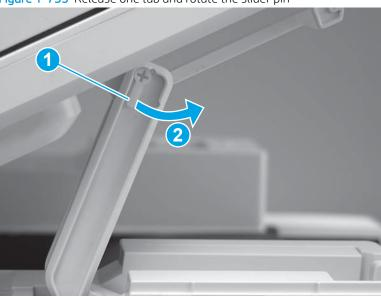
3. Remove the slider pin.
