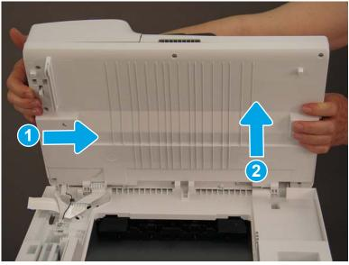
Step 5: Remove the document feeder front cover (M278-M281)
