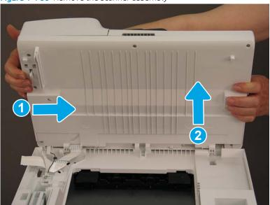
Step 9: Remove the top cover (M278-M281)
