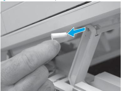
Rotate the hinge arm down.
