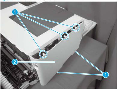
Step 4: Remove the left cover (M178-M181 and M278-M281)
