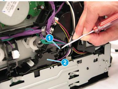
Next to the area where the duct cover was located, release the white plastic tab (callout 1). Rotate it toward the front of the printer.
