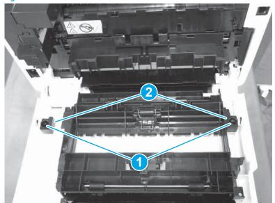
2. Rotate the shaft (callout 1) toward the printer to release it.
