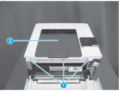
Step 17: Remove the duplex drive assembly (duplex models)
