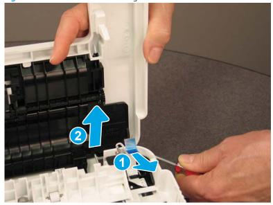
Turn the document feeder base and scanner over to rest on the top of the document feeder base with the bottom of the scanner facing up. Remove one Torx T10 screw (callout 1) on the bottom of the scanner assembly.
