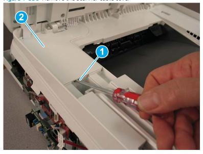
Release the flat cable (callout 1) from the guides (callout 2), and then feed the cables (callout 3) through 6. the opening in the scanner.
