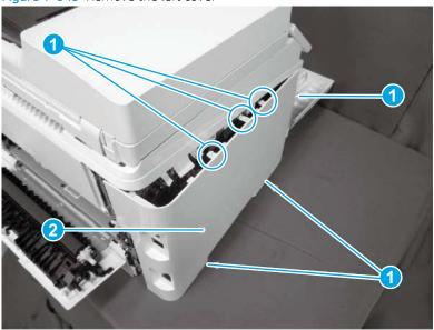
Step 7: Remove the rear cover (simplex models)
