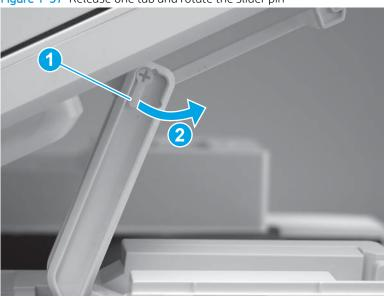
3. Remove the slider pin.
