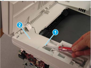
6. Release the flat cable (callout 1) from the guides (callout 2), and then release the flat cable (callout 3) through the opening in the cover.
