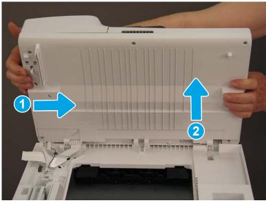
Step 5: Remove the document feeder top cover (M180nw and M181fw)
