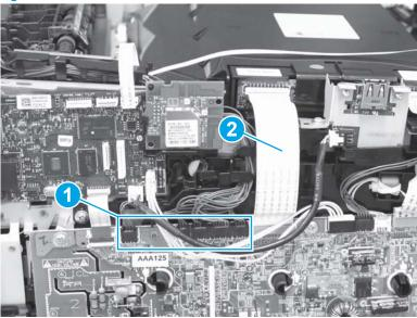
Release the engine controller unit cables (callout 1) from the cable guides (callout 2). 3.
