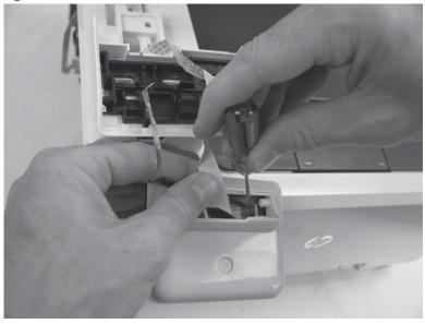
Step 10: Remove the document feeder and scanner assembly (M278-M281)
