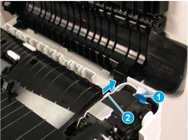
Use a small, flat-blade screwdriver to release the hinge (callout 1), and then lift the edge of the core 2. assembly up (callout 2).
