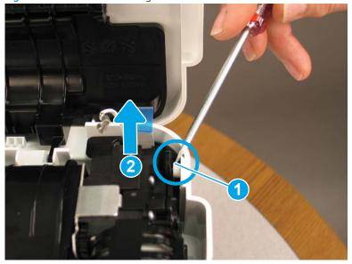
Rotate the core assembly toward the top cover.
