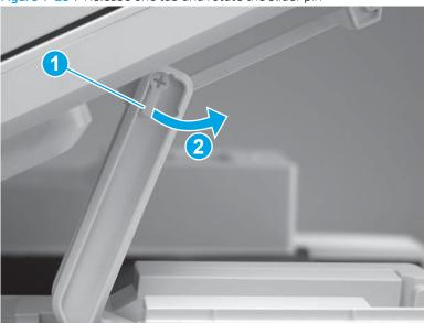
3. Remove the slider pin.
