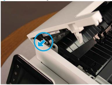
At the front of the printer, use a small, flat-blade screwdriver to flex the inner cover away from the outer cover (callout 1), and then lift up to release the arm from the hinge pin (callout 2).
