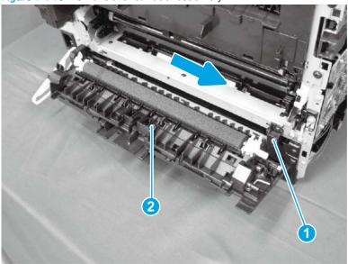
Step 11: Remove the rear door assembly (simplex models)
