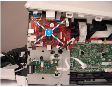
Step 7: Remove the engine controller unit (M178-M181 and M278-M281)
