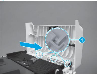
Step 6: Remove the document feeder core assembly (M180nw, M181fw)
