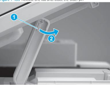
3. Remove the slider pin.
