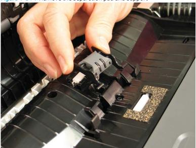
5. To remove the separation pad, release the pad (callout 1) from the tabs on each side.
