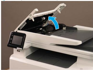
2. Release the hinge on the top cover by flexing the hinge retainer outward, and then fully open the cover.
