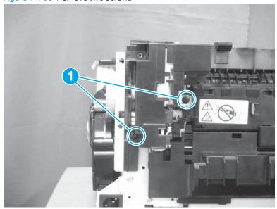
Disconnect two connectors (callout 1). Pulling the connectors away from the drive assembly first might make disconnecting them easier.
