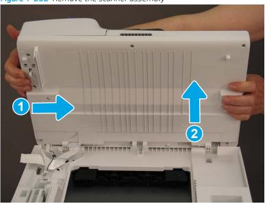
Step 6: Remove the document feeder and scanner (M180nw and M181fw)
