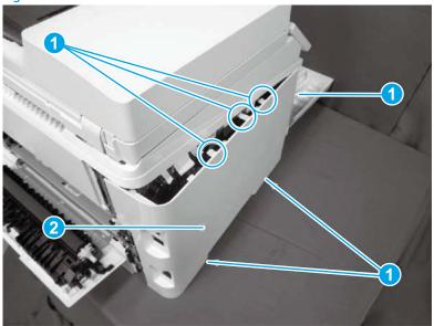
Step 4: Remove the document feeder and image scanner (M278-M281)
