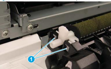
Figure 1-19 Release the left side of the secondary transfer roller
