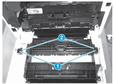
Rotate the shaft (callout 1) toward the printer to release it. 2.
