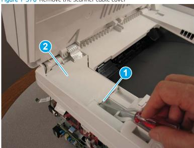
Release the flat cable (callout 1) from the guides (callout 2), and then feed the two flat cables (callout 3) 6. through the openings in the scanner.
