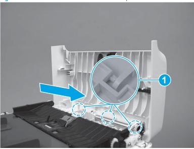
Step 2: Remove the pre-pick arm assembly (M180nw and M181fw)
