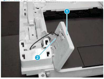
Step 11: Remove the top cover (M178-M181)
