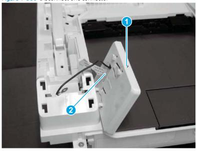
Step 9: Remove the control panel (M278-M281)
