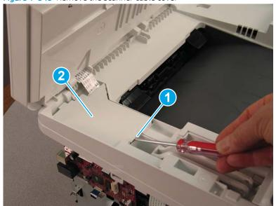
Release the flat cable (callout 1) from the guides (callout 2), and then release the flat cable (callout 3) through the opening in the cover.
