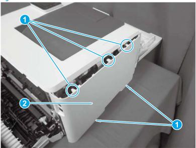
Step 4: Remove the engine controller unit (M153-M154 and M253-M254)
