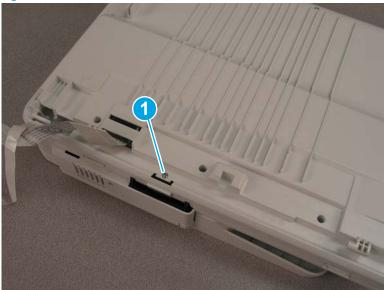
Turn the document feeder base and scanner over so the that the top is facing up, and then remove one Torx T10 screw (callout 1).
