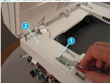
6. Release the flat cable (callout 1) from the guides (callout 2), and then feed the two flat cables (callout 3) through the openings in the scanner.
