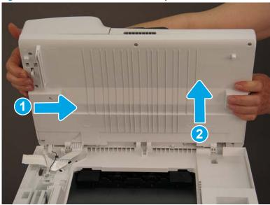
Step 5: Remove the document feeder top cover (M180nw and M181fw)
