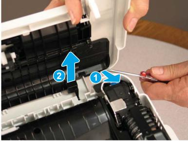
Step 2: Remove the document feeder pick extension shaft (M278-M281)
