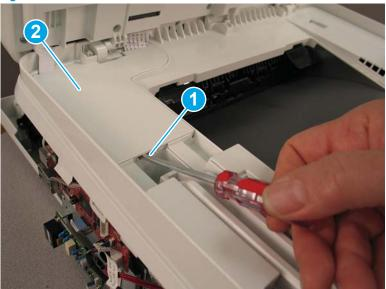
Release the flat cable (callout 1) from the guides (callout 2), and then feed the cables (callout 3) through the opening in the scanner.
