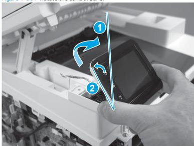
5. Firmly move the assembly to the right 7-8 mm (0.26-0.31 in) (callout 1) to release two tabs from the posts at the base of the control panel.
