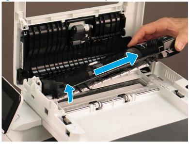
Step 8: Remove the document feeder base (M278-M281)
