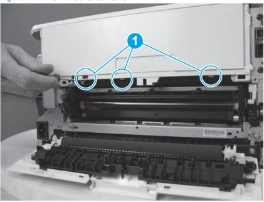
Step 6: Remove the flatbed scanner assembly (M180n)
