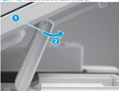
3. Remove the slider pin.
