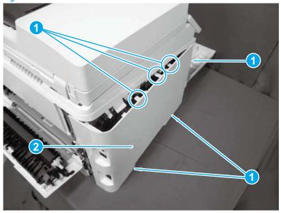
Step 7: Remove the control panel (M278-M281)
