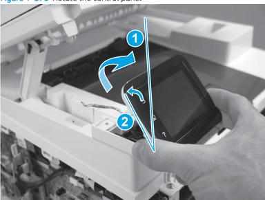
Firmly move the assembly to the right 7-8 mm (0.26-0.31 in) (callout 1) to release two tabs from the posts 5. at the base of the control panel.
