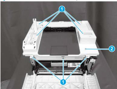
Step 12: Remove the low-voltage power supply
