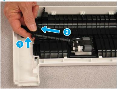
Step 3: Remove the document feeder pick assembly (M278-M281)
