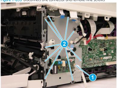
Figure 1-659 Disconnect one connector and remove nine screws
