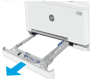
Step 3: Remove the priority feed slot tray (M253-M254 and M278-M281)
