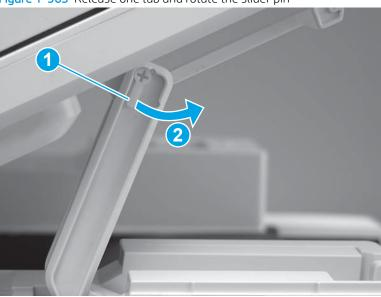
3. Remove the slider pin.
