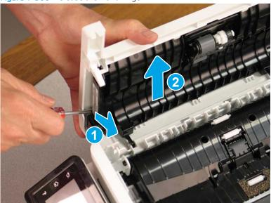
At the back of the printer, use a small, flat-blade screwdriver to flex the inner cover away from the outer 4. cover (callout 1), and then lift up to release the arm from the hinge pin (callout 2). Remove the top cover.
