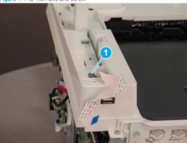
3. At the back of the printer, remove one screw (callout 1).
