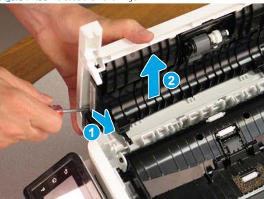
At the back of the printer, use a small, flat-blade screwdriver to flex the inner cover away from the outer cover (callout 1), and then lift up to release the arm from the hinge pin (callout 2). Remove the top cover.
