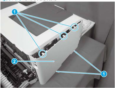
Step 7: Remove the right cover (M178-M181 and M278-M281)
