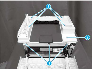
Step 9: Remove the output sensor assembly (M178-M181)
