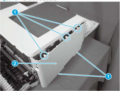
Step 5: Remove the right cover (M178-M181 and M278-M281)
