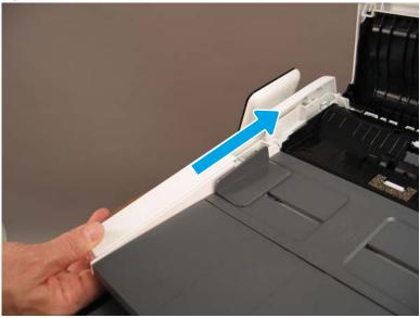
Step 6: Remove the document feeder input tray (M278-M281)
