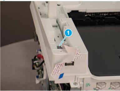
At the back of the printer, remove one screw (callout 1).
