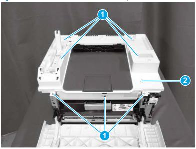
Step 16: Remove the top cover (M153-M154 and M253-M254)
