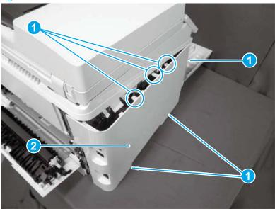
Step 9: Remove the duplexer door (duplex models)
