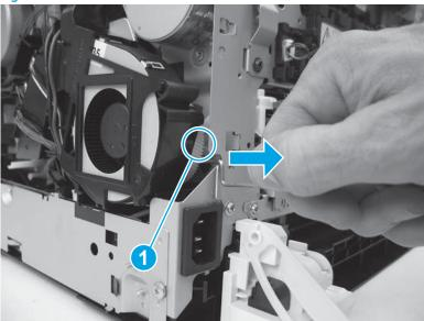
On the rear side of the printer, remove two screws (callout 1).
