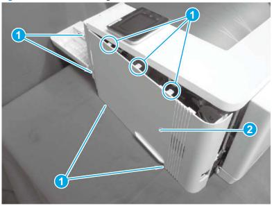
Step 4: Remove the right cover (M178-M181 and M278-M281)
