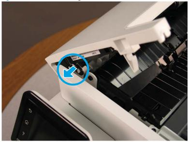
At the front of the printer, use a small, flat-blade screwdriver to flex the inner cover away from the outer cover (callout 1), and then lift up to release the arm from the hinge pin (callout 2).
