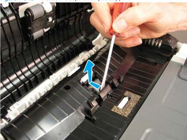
Remove the separation pad and support.
