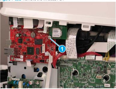
Step 5: Remove the wireless PCA (M278-M281 wireless models)
