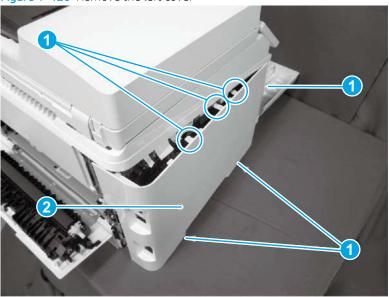
Step 4: Remove the document feeder and image scanner (M278-M281)
