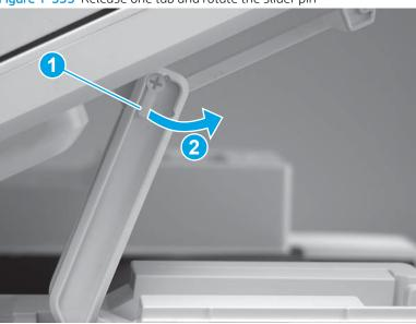
3. Remove the slider pin.
