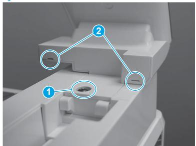
Remove the flat cable (callout 1) from the guides, and then remove three screws (callout 2).
