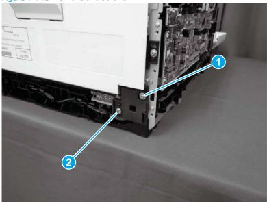
Open the rear door. Release the shaft holder (callout 1) to remove it from the rear door. 2.
