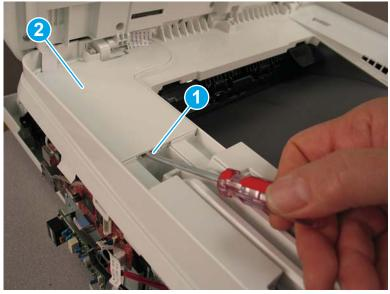
Release the flat cable (callout 1) from the guides (callout 2), and then feed the cables (callout 3) through 6. the opening in the scanner.
