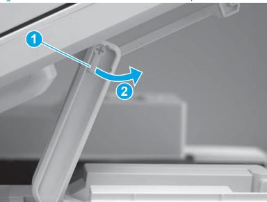
2. Remove the slider pin.
