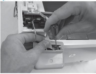
Step 7: Remove the document feeder and scanner assembly (M278-M281)
