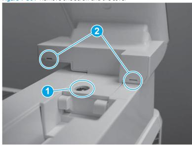
3. Remove the flat cable (callout 1) from the guides, and then remove three screws (callout 2).
