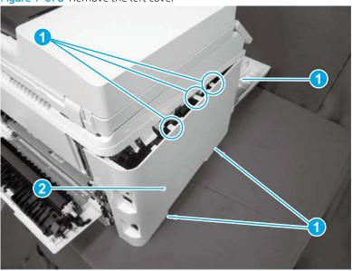
Step 9: Remove the duplexer door (duplex models)
