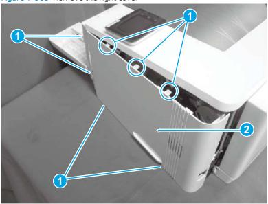
Step 4: Remove the right cover (M178-M181 and M278-M281)
