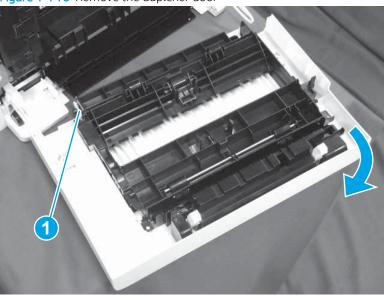
Step 10: Remove the rear door assembly (duplex models)
