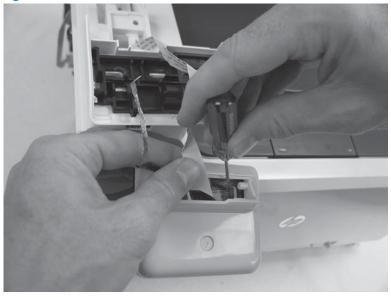
Step 8: Remove the document feeder and scanner assembly (M278-M281)
