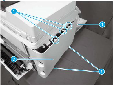
Step 5: Remove the rear lower cover (simplex models)
