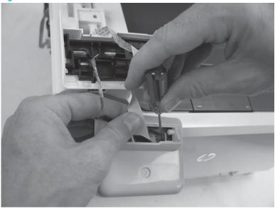
Step 14: Remove the document feeder and scanner assembly (M278-M281)
