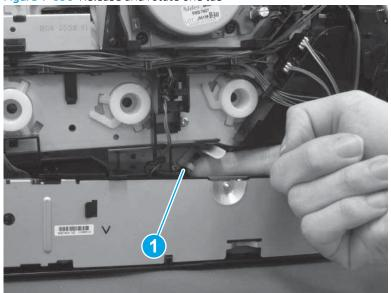
Pull the white plastic shaft (callout 1) away from the chassis to loosen it. 4.
