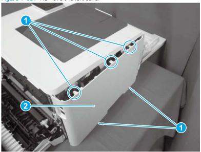
Step 5: Remove the right cover (M178-M181 and M278-M281)
