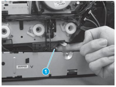
Pull the white plastic shaft (callout 1) away from the chassis to loosen it.
