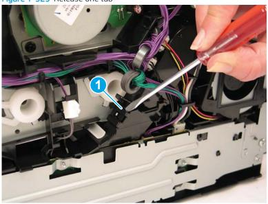
2. Release one tab (callout 1) on the rear of the fan duct cover, and then remove the fan duct cover (callout 2).
