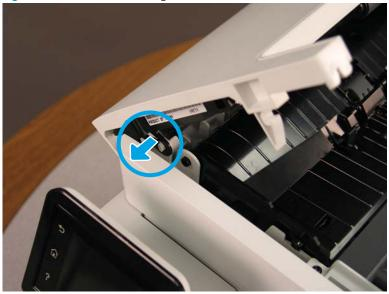
Carefully insert a small, flat-blade screwdriver between the separation pad support and the document feeder case. Rotate the end of the screwdriver towards the separation pad to release the support.
