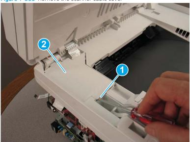
Release the flat cable (callout 1) from the guides (callout 2), and then feed the two flat cables (callout 3) 6. through the openings in the scanner.
