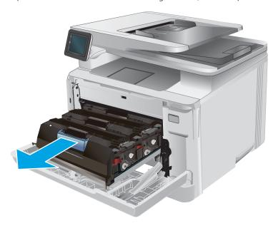
Grasp the handle on the toner cartridge, and then pull the toner cartridge straight up to remove it.
