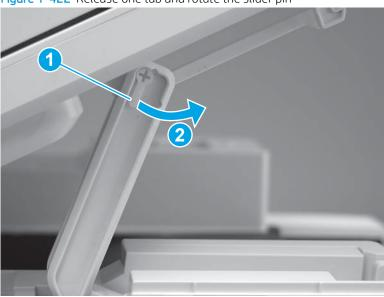
3. Remove the slider pin.
