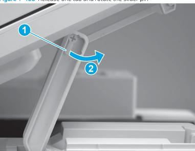
3. Remove the slider pin.
