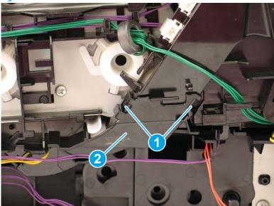
Disconnect three connectors (callout 1), and then release the cables from the cable guides (callout 2).
