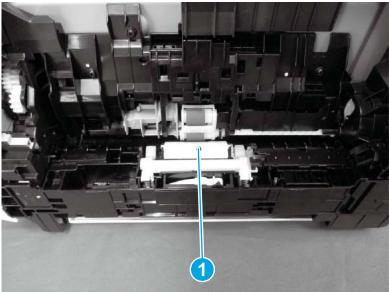
2. Release one tab (callout 1), and then remove the separation roller (callout 2).
