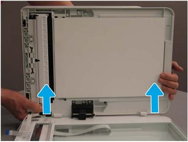
Step 6: Remove the document feeder hinge (M278-M281)
