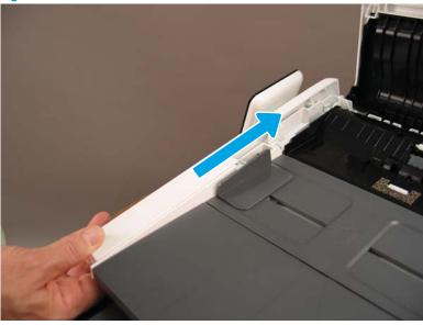
Step 2: Remove the document feeder input tray (M278-M281)
