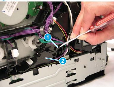
Remove one screw (callout 1), and then remove an M4 tapping screw (callout 2).
