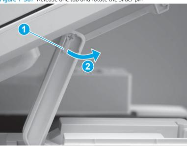
3. Remove the slider pin.
