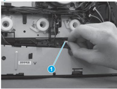
Find the ITB service tool and use the graphic below to see how to hold it correctly. 5.
