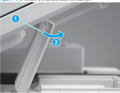
3. Remove the slider pin.
