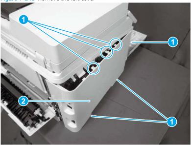
Step 5: Remove the flatbed scanner (M180n)
