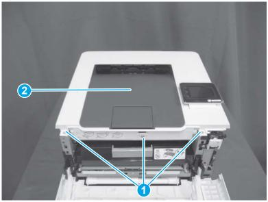
Step 7: Remove the control panel (M254dw touchscreen)
