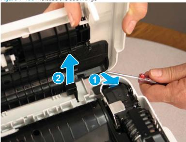
Step 2: Remove the document feeder pick extension shaft (M278-M281)
