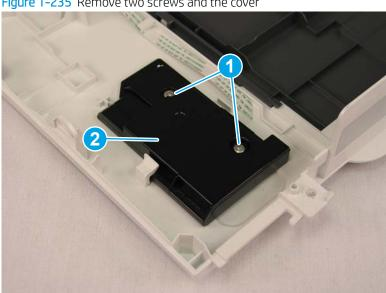
Figure 1-235 Remove two screws and the cover
