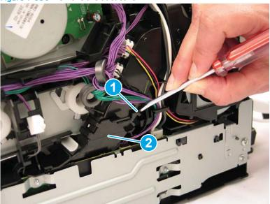
Remove one screw (callout 1), and then remove an M4 tapping screw (callout 2).
