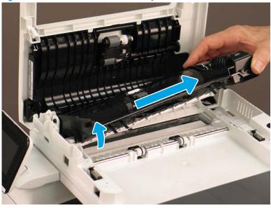
Step 9: Remove the document feeder flat cable (M278-M281)
