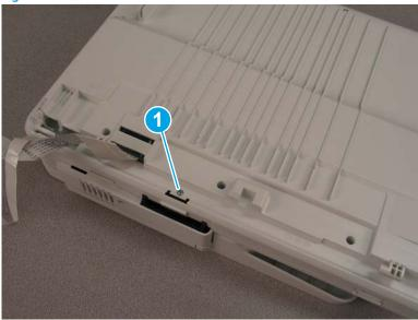
Turn the document feeder base and scanner over so the that the top is facing up, and then remove one Torx T10 screw (callout 1).
