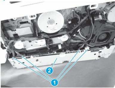
Step 6: Remove the pickup motor
