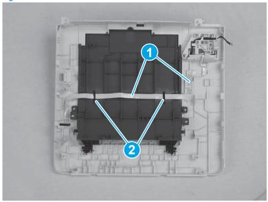
Remove the cable (callout 1) from the guides (callout 2), and then remove three screws (callout 3). 2.
