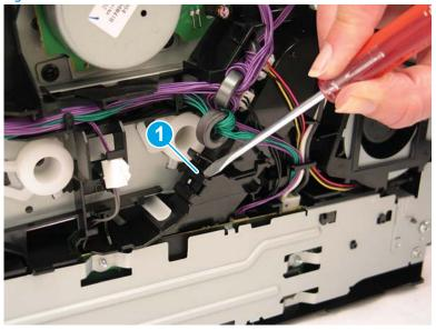
Release one tab (callout 1) on the rear of the fan duct cover, and then remove the fan duct cover (callout 2). 2.
