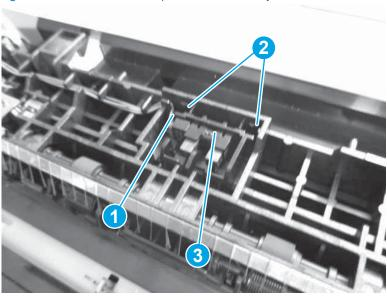
Step 13: Remove the control panel (M278-M281)
