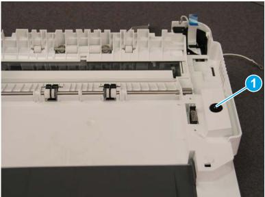
Open the document feeder base, and then lift up to remove it. 5.
