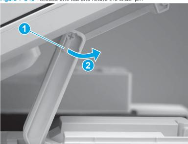
3. Remove the slider pin.
