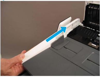
Step 6: Remove the document feeder input tray (M278-M281)
