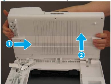
Step 7: Remove the document feeder and scanner assembly (M180nw and M181fw)
