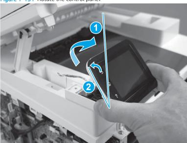
Firmly move the assembly to the right 7-8 mm (0.26-0.31 in) (callout 1) to release two tabs from the posts 5. at the base of the control panel.
