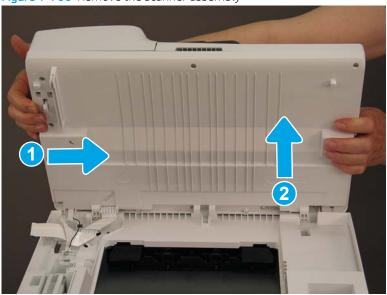
Step 6: Remove the document feeder and scanner assembly (M180nw and M181fw)
