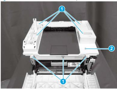
Step 12: Remove the output sensor assembly (M178-M181)
