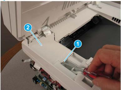
Release the flat cable (callout 1) from the guides (callout 2), and then feed the two flat cables (callout 3) through the openings in the scanner.
