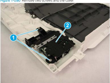
Figure 1-280 Remove two screws and the cover
