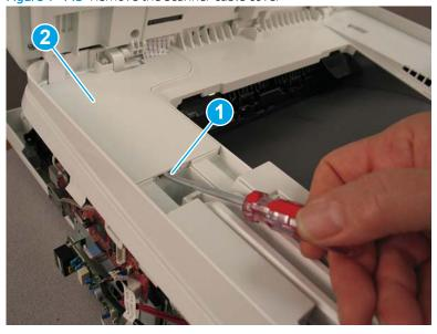
Release the flat cable (callout 1) from the guides (callout 2), and then feed the cables (callout 3) through the opening in the scanner.
