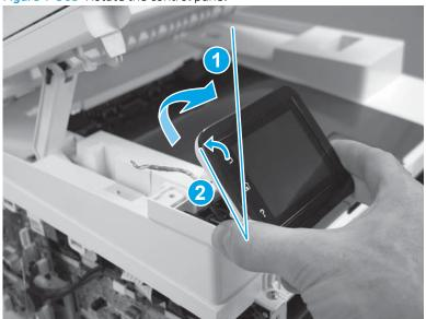
Firmly move the assembly to the right 7-8 mm (0.26-0.31 in) (callout 1) to release two tabs from the posts at the base of the control panel.
