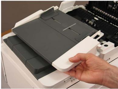
Step 7: Remove the document feeder core (M278-M281)
