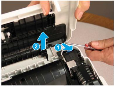
Step 2: Remove the document feeder inner cover or outer cover (M278-M281)
