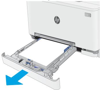
Step 3: Remove the priority feed slot tray (M253-M254 and M278-M281)
