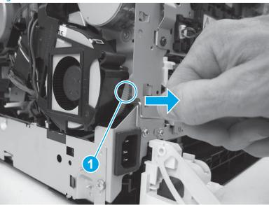
On the rear side of the printer, remove two screws (callout 1).
