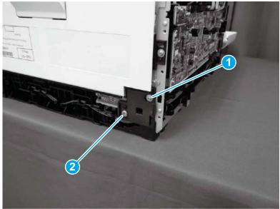
2. Open the rear door. Release the shaft holder (callout 1) to remove it from the rear door.
