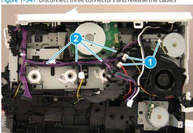
Figure 1-947 Disconnect three connectors and release the cables
