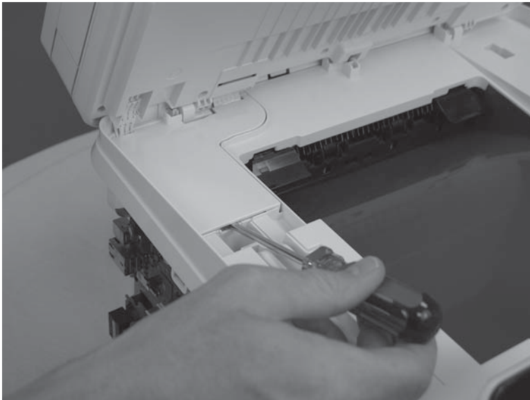
Figure 1-651 Remove the M274, M277 scanner (2 of 4)
