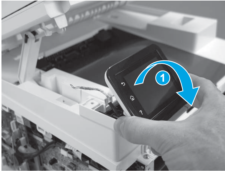
Figure 1-211 Remove the M274, M277 control panel (5 of 6)
