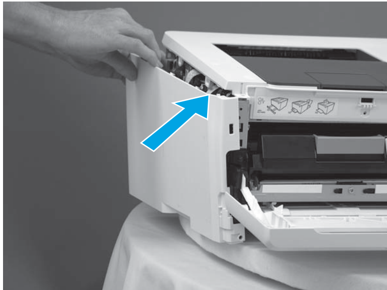
Figure 1-344 Install the left cover (1 of 3)
