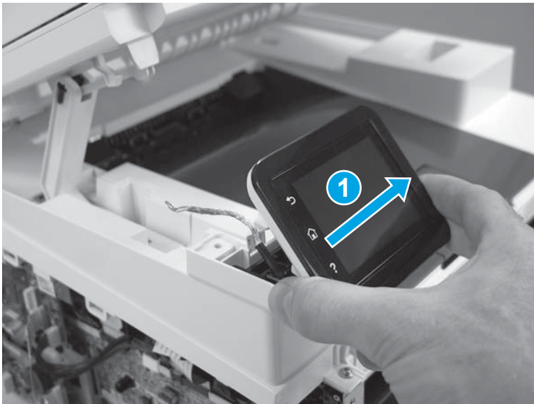
Figure 1-210 Remove the M274, M277 control panel (4 of 6)
