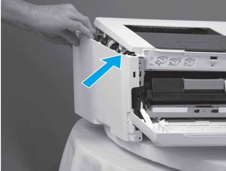
Figure 1-547 Install the left cover (1 of 3)
