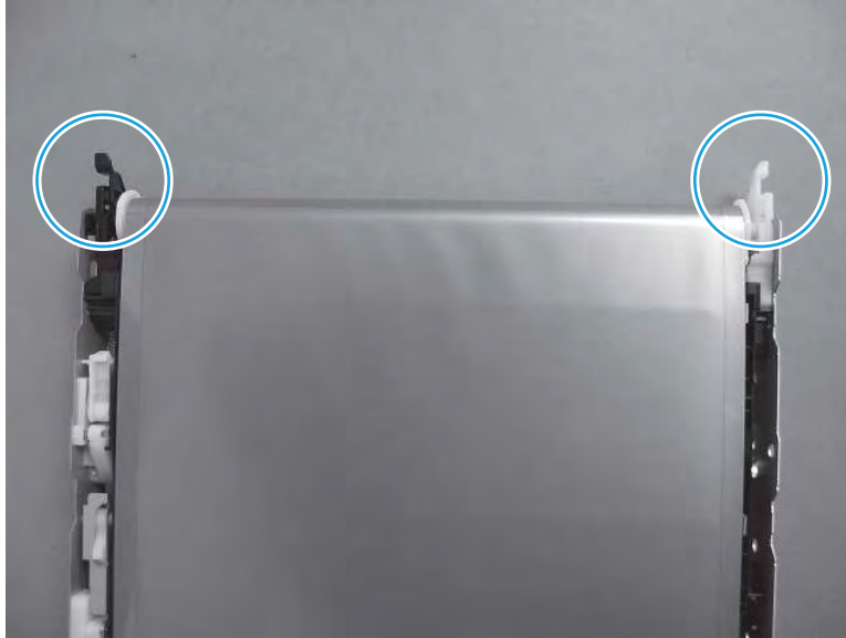
Figure 5-774 Check tabs on the end of the ITB
