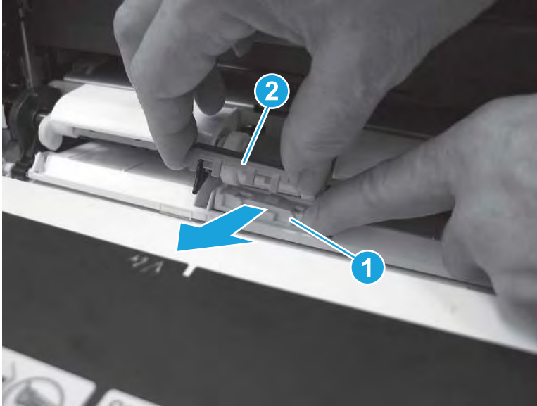
Figure 2-4 Remove the separation pad
