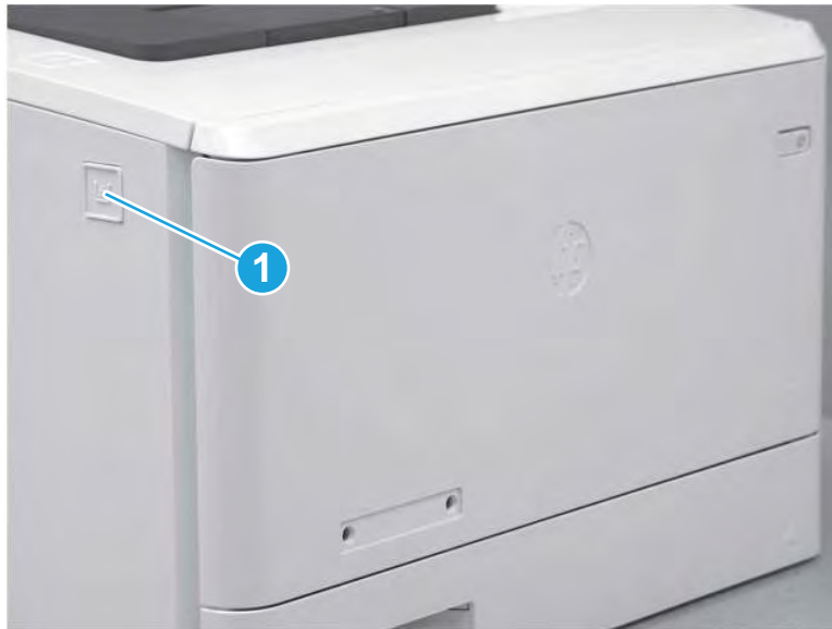
Figure 5-87 Release the front door
