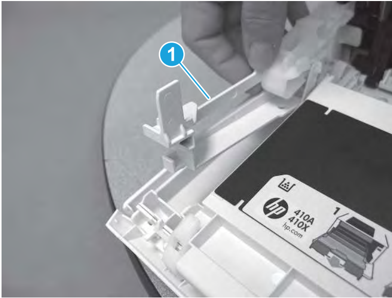
Figure 5-129 Release the left hinge cover
