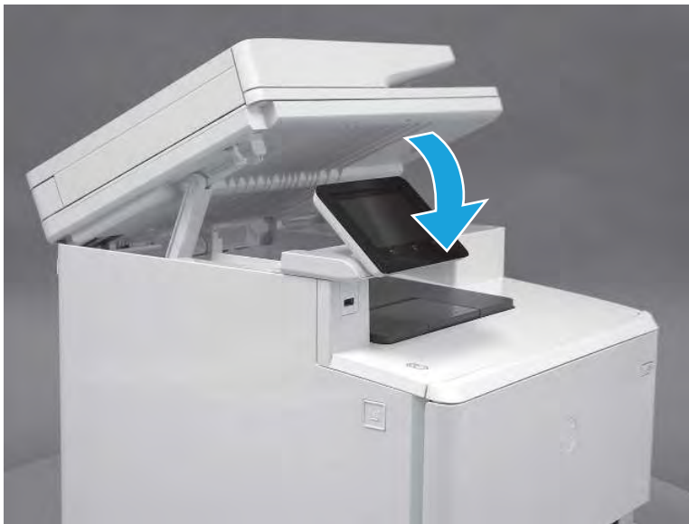
Figure 5-1216 Lower the scanner
