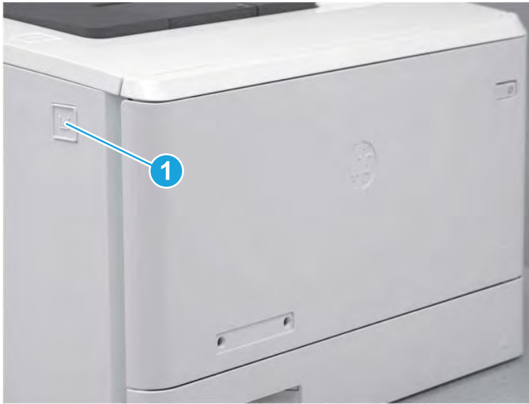
Figure 5-1920 Release the front door
