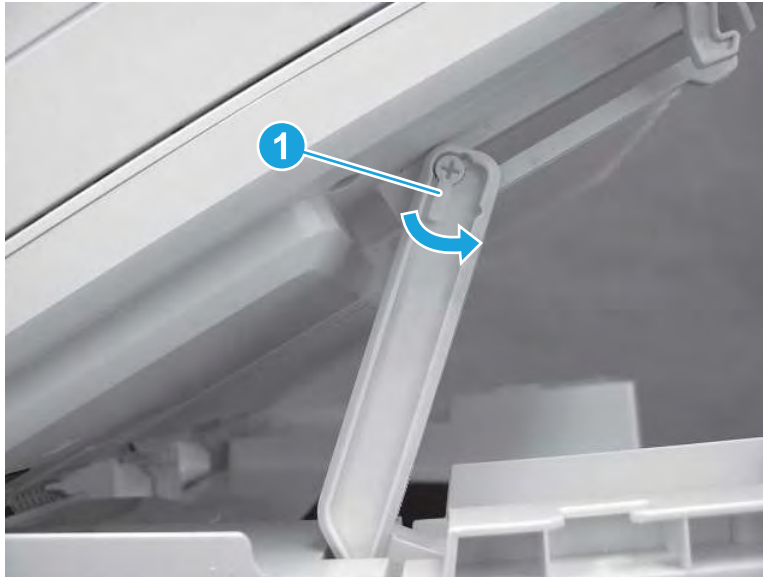
Figure 5-1759 Release scanner support arm pin
