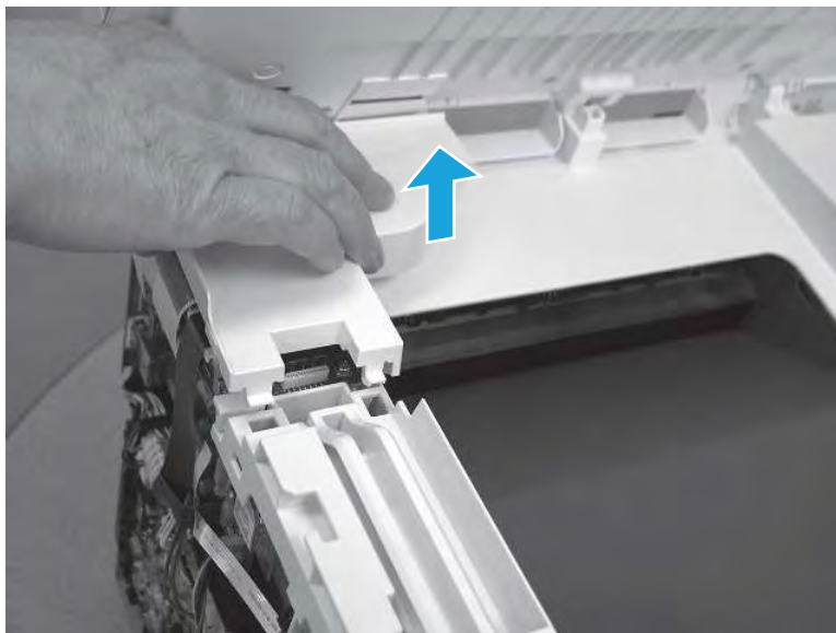
Figure 5-1912 Remove the scanner cable cover
