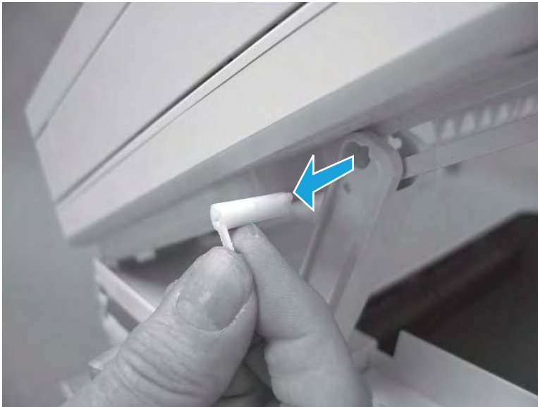
Figure 5-318 Remove the pin
