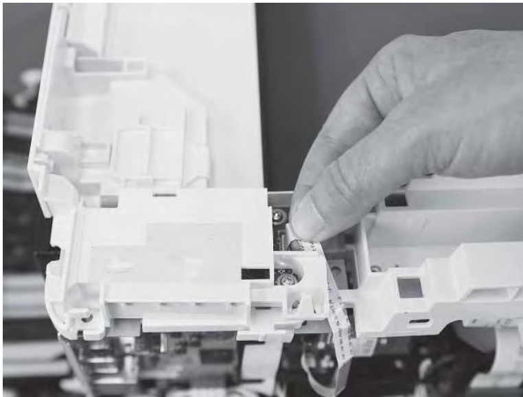
Figure 5-1953 Disconnect one connector
