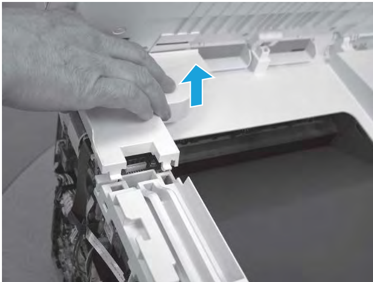
Figure 5-1762 Remove the scanner cable cover
