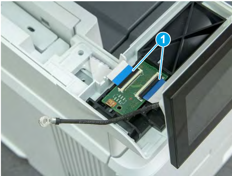
Figure 5-237 Disconnect two FFC
