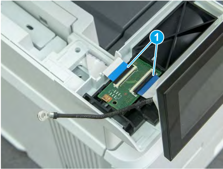
Figure 5-1753 Disconnect two FFC
