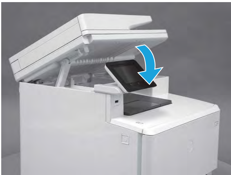
Figure 5-452 Lower the scanner
