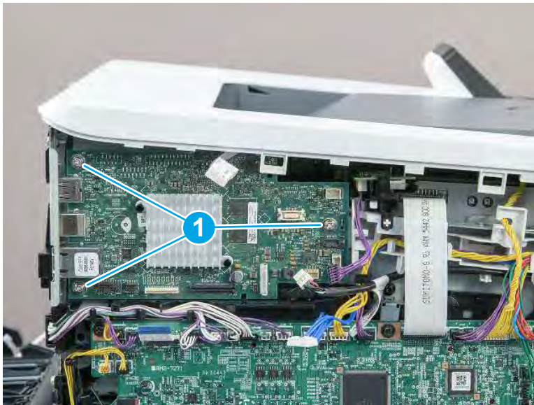
Figure 5-1858 Remove three screws (SFP)
