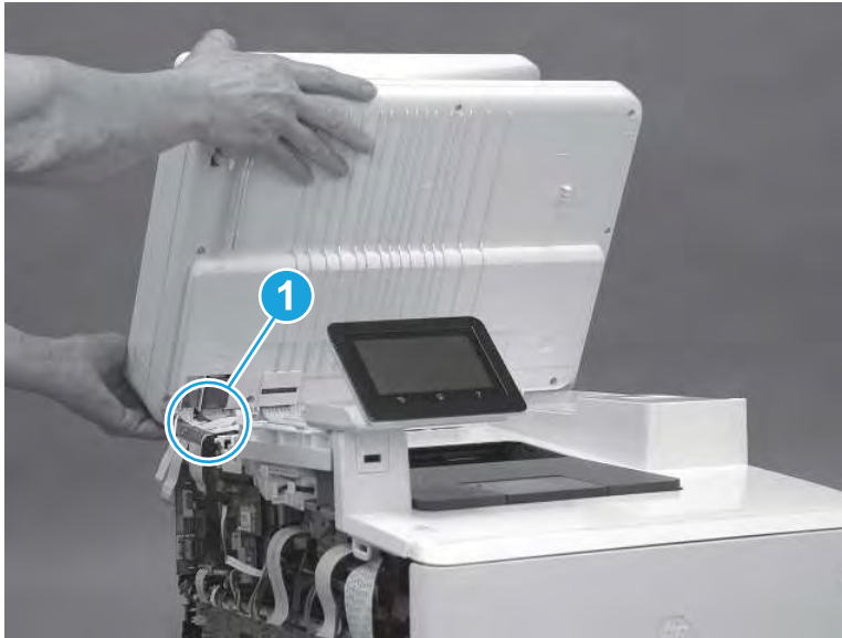
Figure 5-1556 Release the cables
