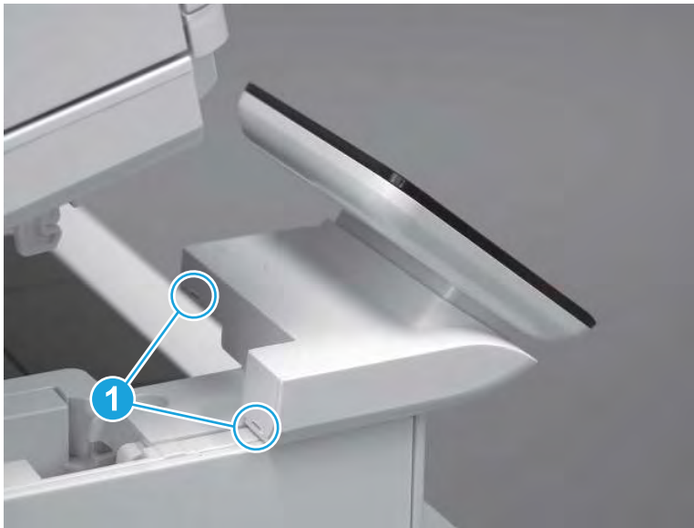
Figure 5-2007 Release two tabs
