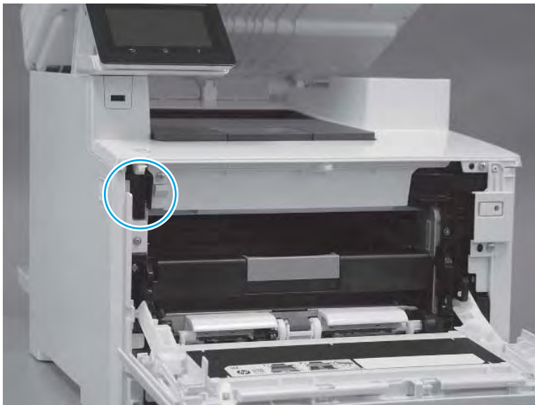
Figure 4-22 Defeat the front (cartridge) door interlock
