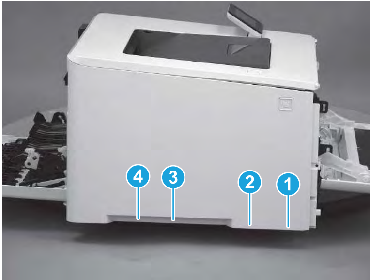
Figure 5-1804 Release bottom tabs
