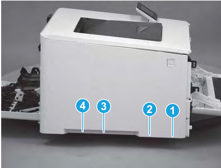
Figure 5-383 Release bottom tabs
