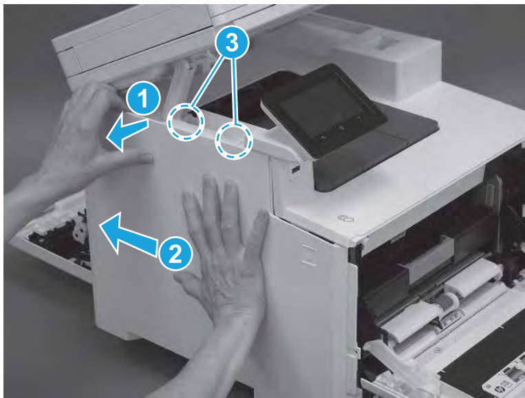
Figure 5-2052 Release one tab and two hooks
