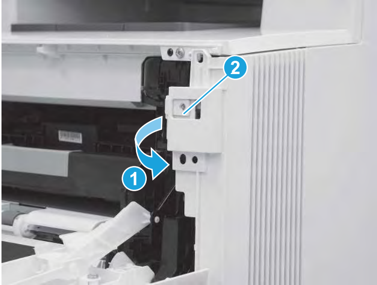
Figure 5-1416 Rotate the front of the cover
