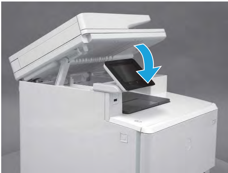
Figure 5-1904 Lower the scanner
