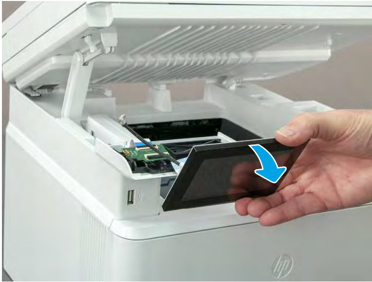
Figure 5-282 Remove the control-panel assembly
