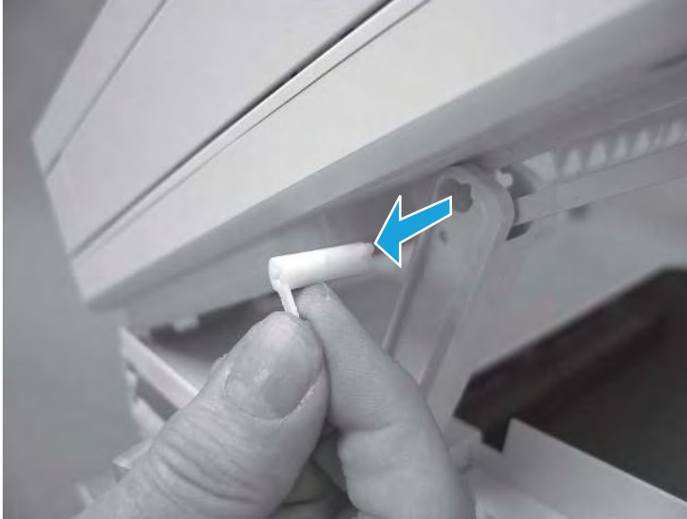
Figure 5-1647 Remove the pin
