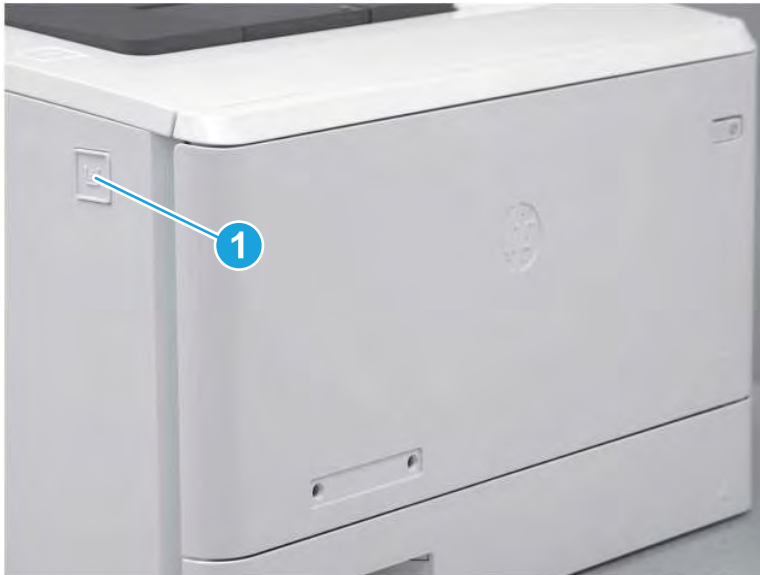
Figure 5-860 Release the front door
