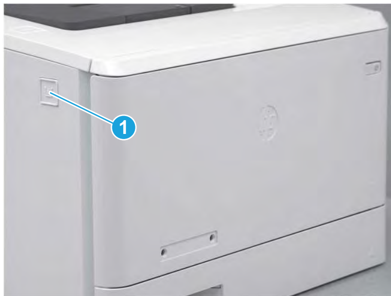
Figure 5-199 Release the front door
