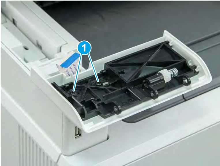
Figure 5-284 Remove two screws
