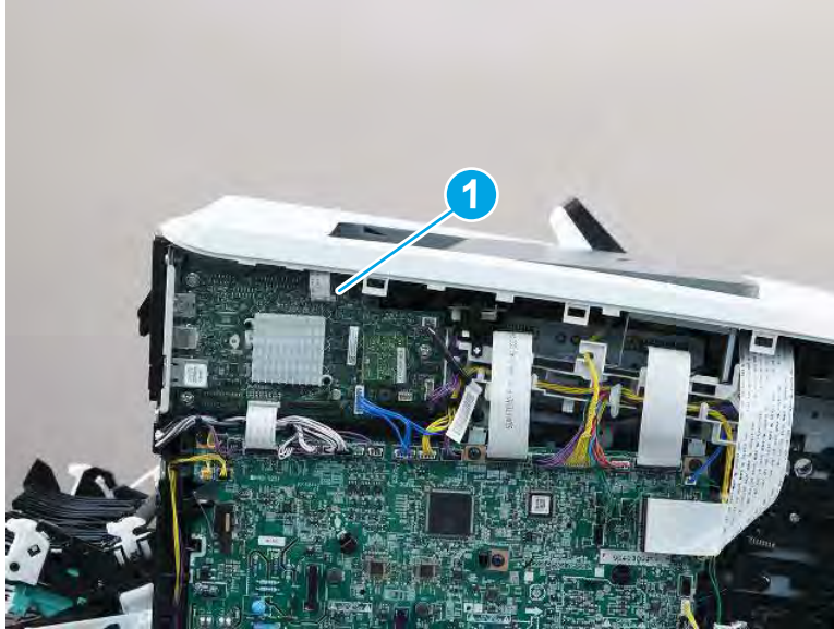
Figure 5-193 Disconnect one connector
