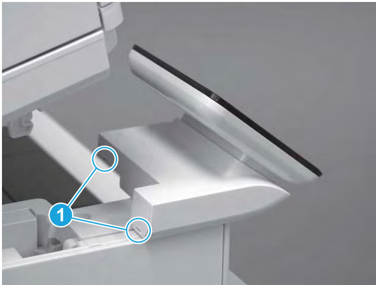
Figure 5-257 Release two tabs
