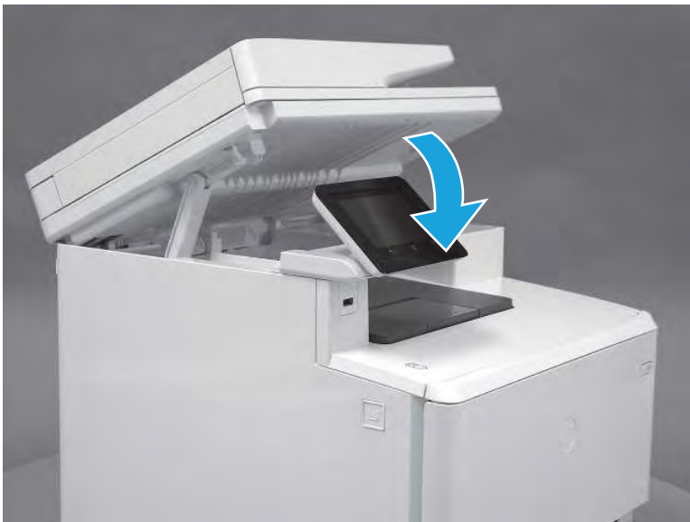
Figure 5-1746 Lower the scanner
