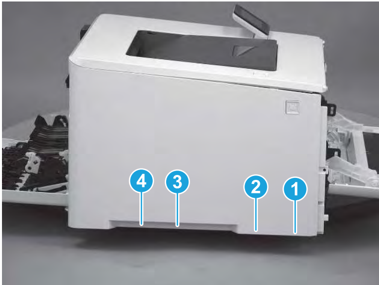
Figure 5-2044 Release bottom tabs
