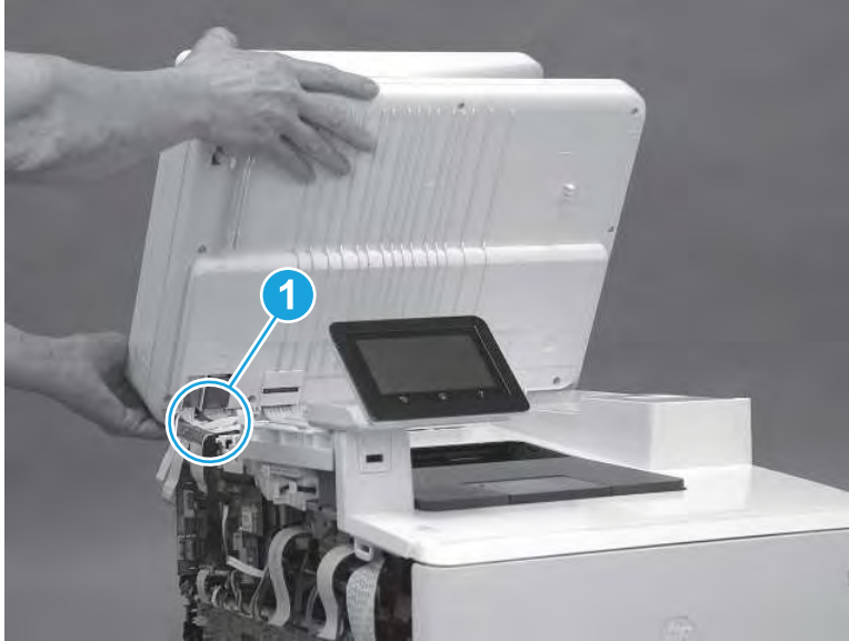
Figure 5-1450 Release the cables
