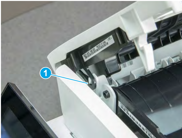
Figure 5-14 Release one hinge pin
