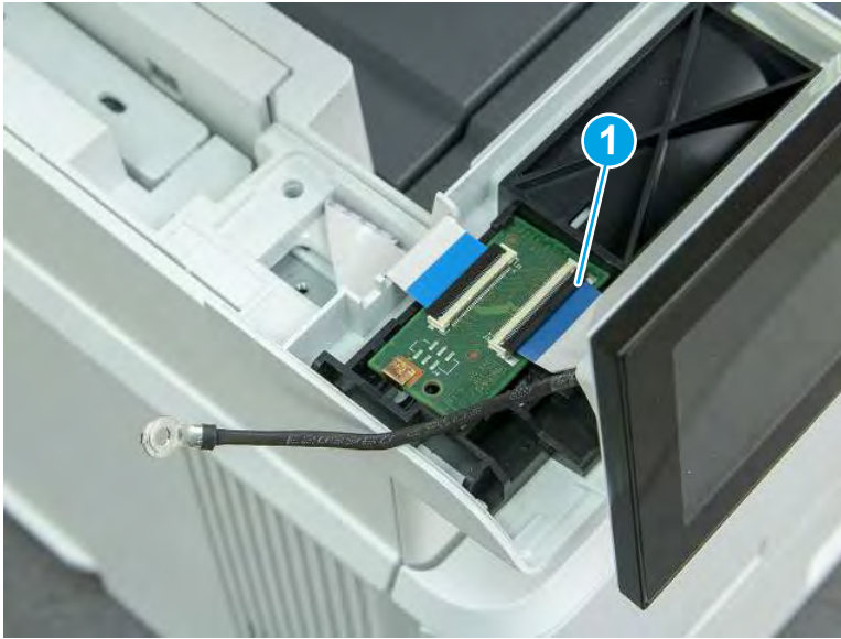
Figure 5-280 Disconnect one flat cable
