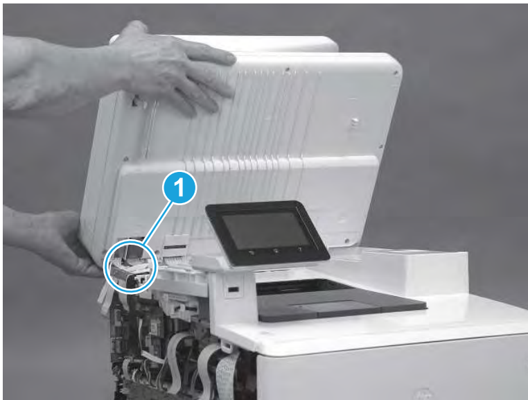
Figure 5-1650 Release the cables
