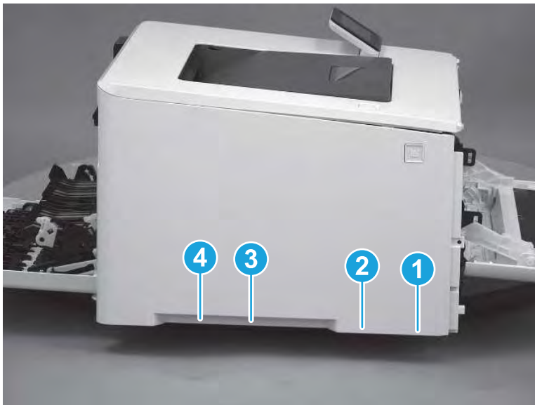
Figure 5-1867 Release bottom tabs
