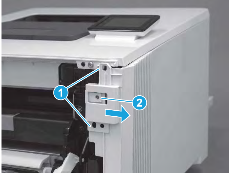
Figure 5-943 Release two front tabs
