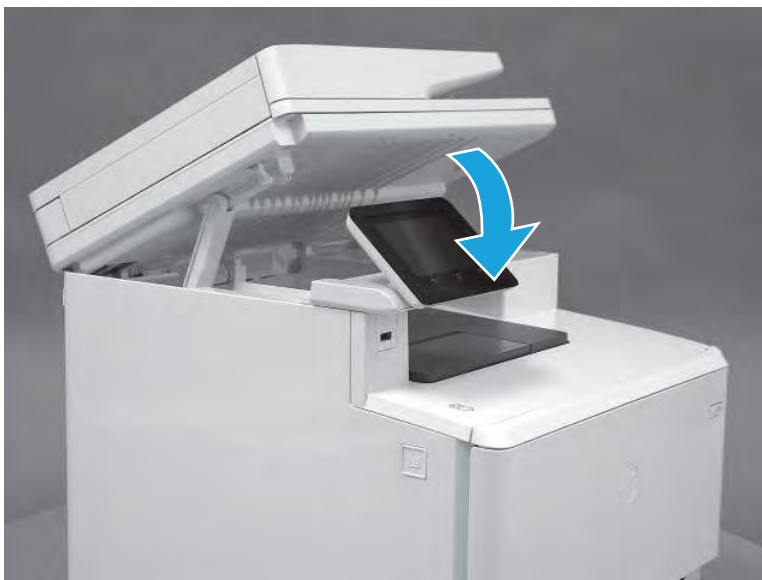
Figure 5-1834 Lower the scanner
