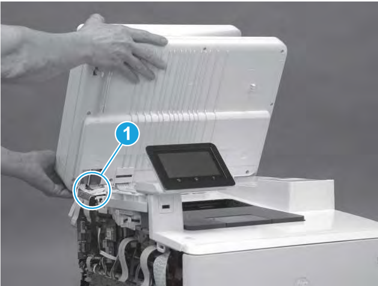
Figure 5-1951 Release the cables
