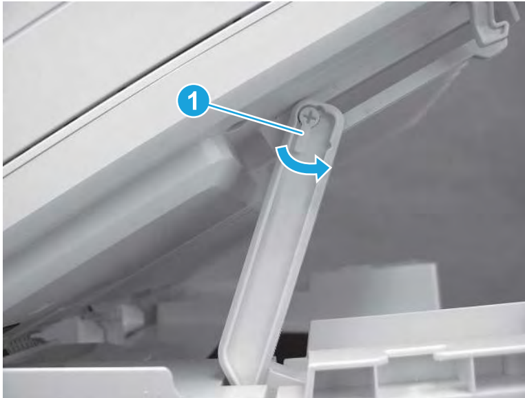
Figure 5-1552 Release scanner support arm pin
