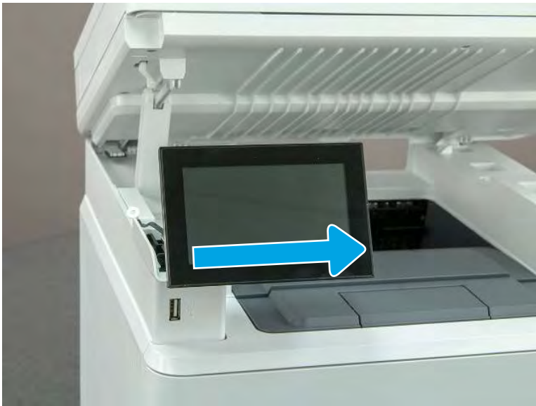
Figure 5-281 Slide the control panel display
