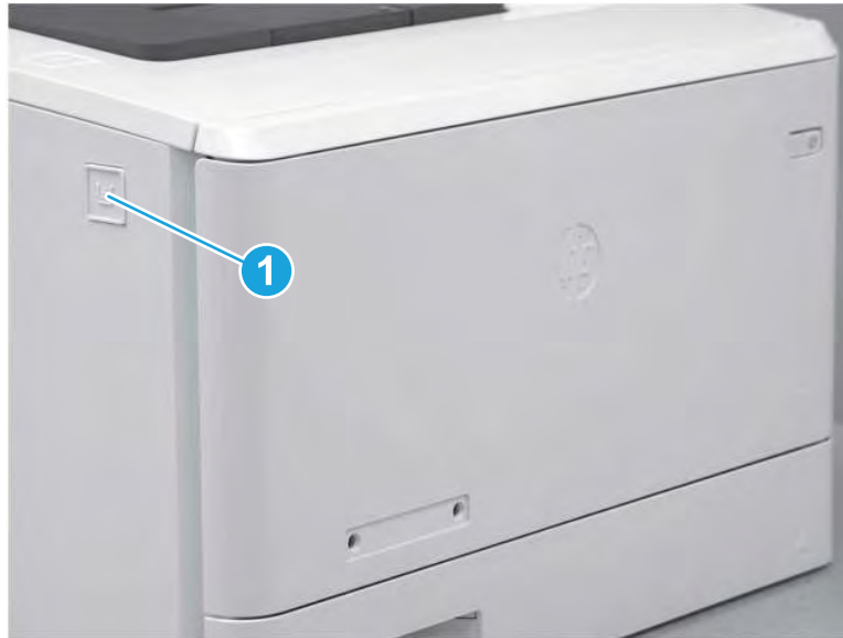
Figure 2-8 Release the front door
