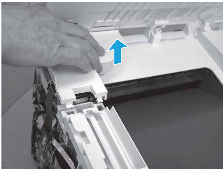
Figure 5-2019 Remove the scanner cable cover
