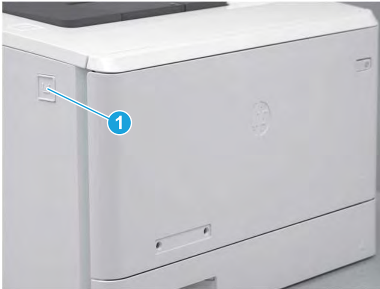
Figure 5-568 Release the front door
