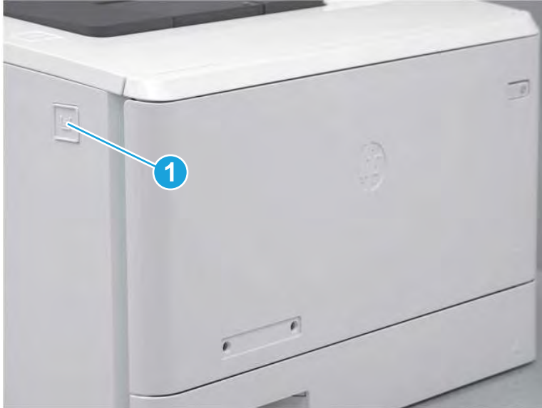
Figure 5-935 Release the front door
