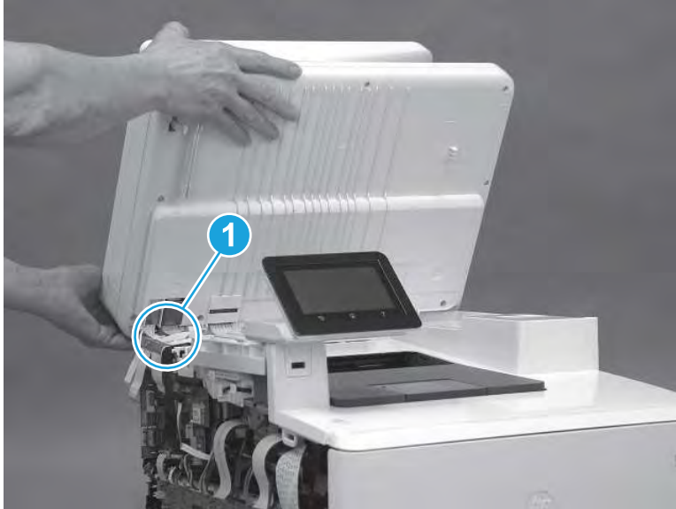
Figure 5-1763 Release the cables
