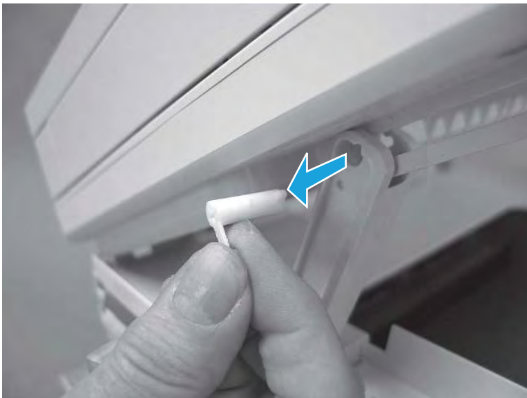
Figure 5-41 Remove the pin
