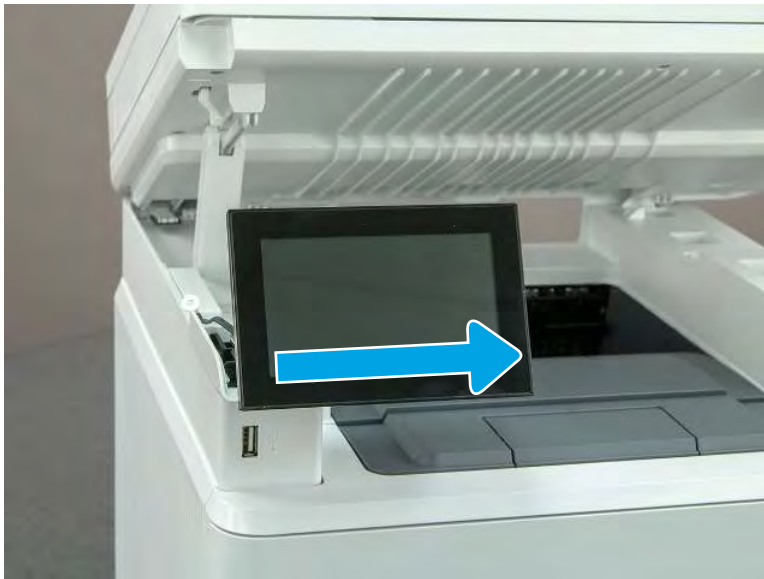
Figure 5-265 Slide the control panel display
