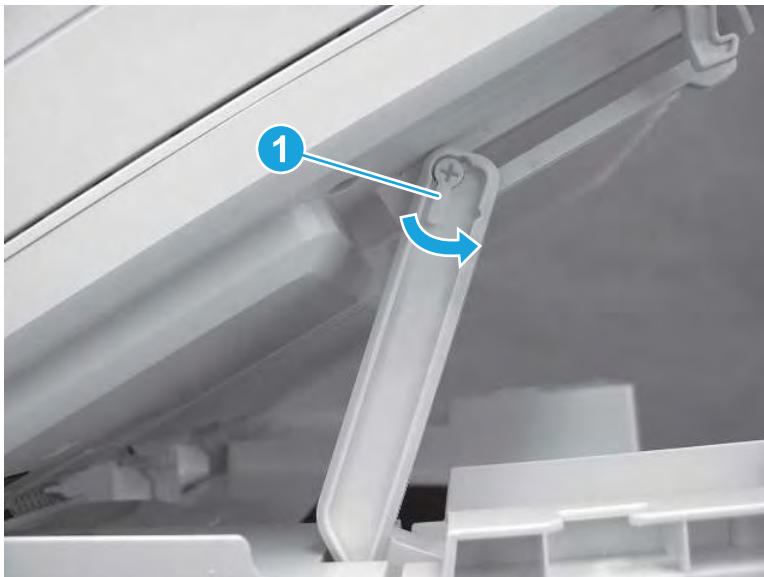
Figure 5-1646 Release scanner support arm pin
