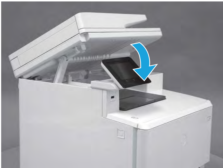
Figure 5-1732 Lower the scanner
