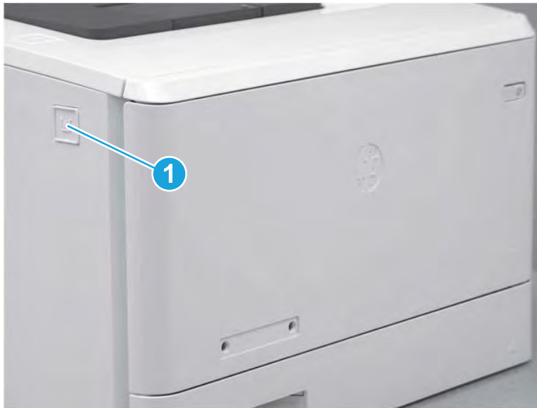
Figure 2-1 Release the front door
