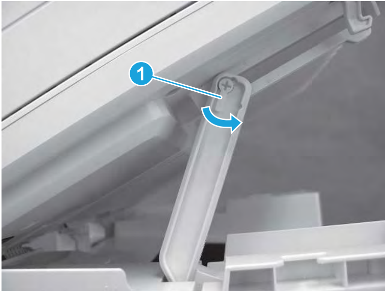
Figure 5-40 Release scanner support arm pin
