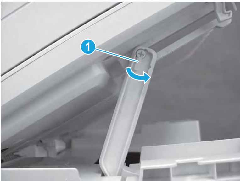
Figure 5-1947 Release scanner support arm pin
