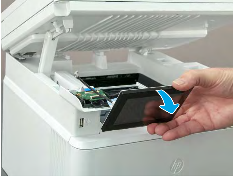
Figure 5-266 Remove the control-panel assembly
