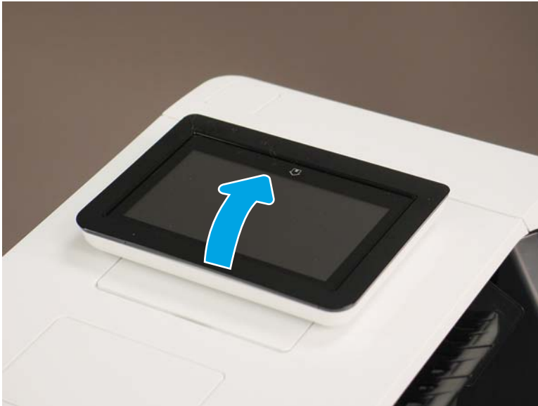
Figure 1-150 Tilt the control panel up
