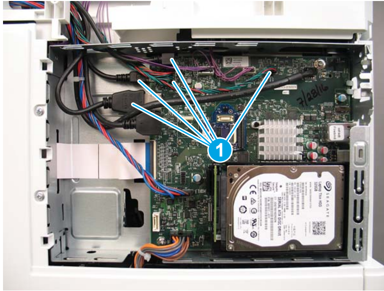
Figure 1-668 Disconnect six connectors
