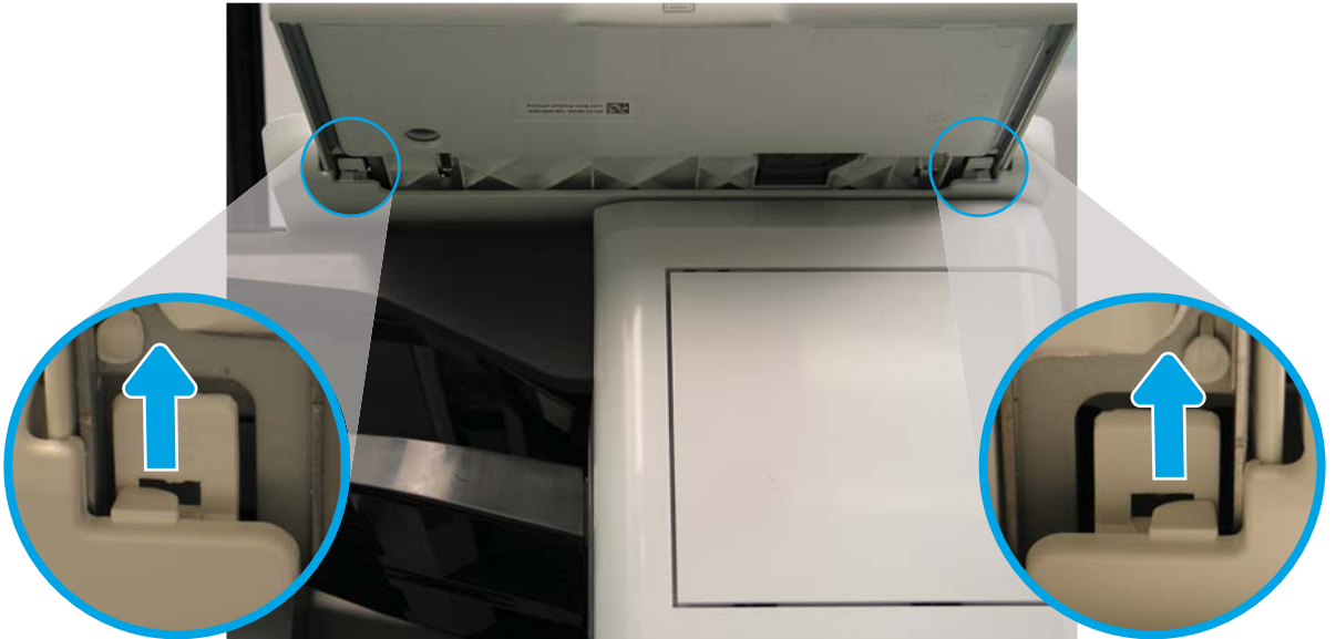
Figure 1-1185 Release two tabs
