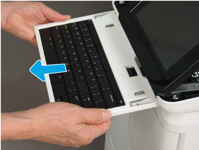
Figure 1-425 Remove the keyboard
