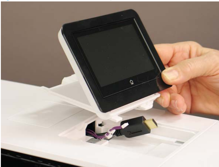
Figure 1-1382 Remove the control panel
