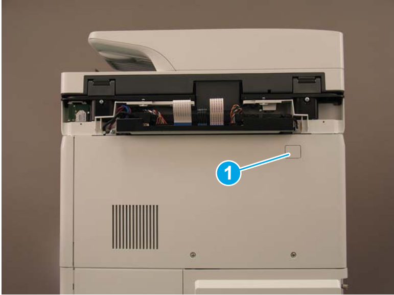
Figure 1-762 Remove one screw cover
