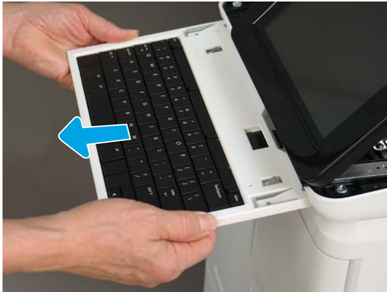
Figure 1-1029 Remove the keyboard
