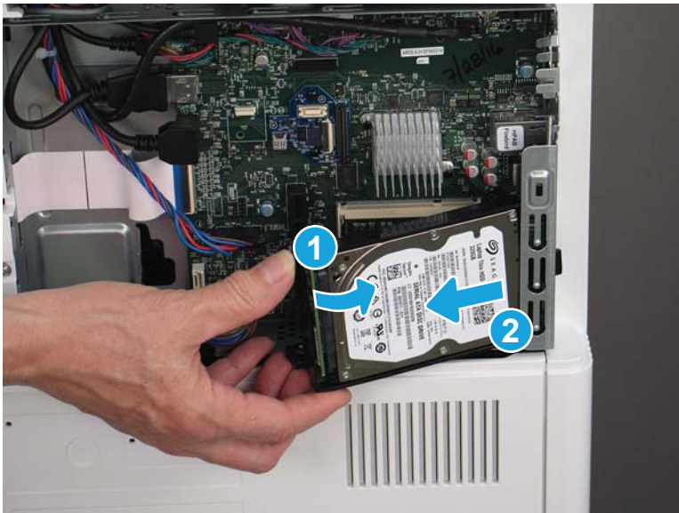
Figure 1-1714 Remove the HDD
