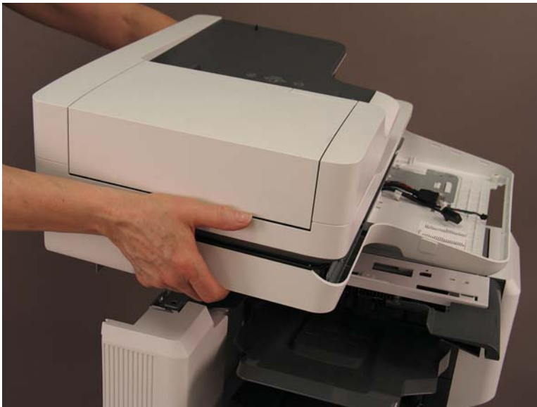
Figure 1-445 Remove the document feeder and image scanner
