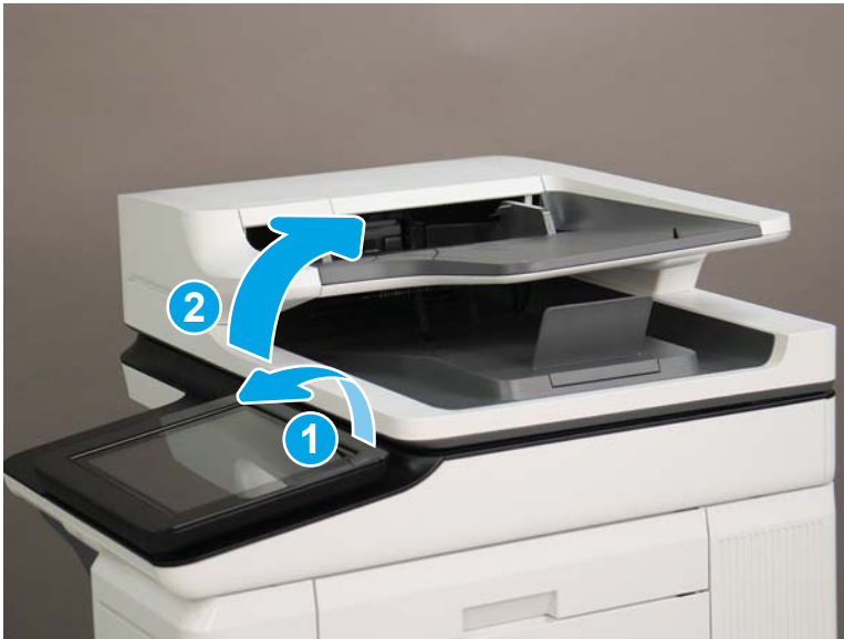
Figure 1-1023 Tilt the control panel and open the document feeder
