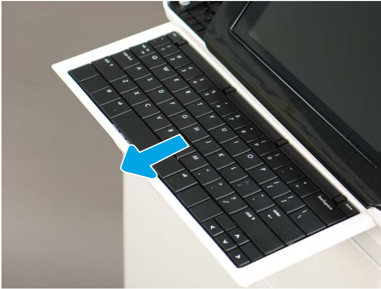
Figure 1-287 Slide the keyboard tray out
