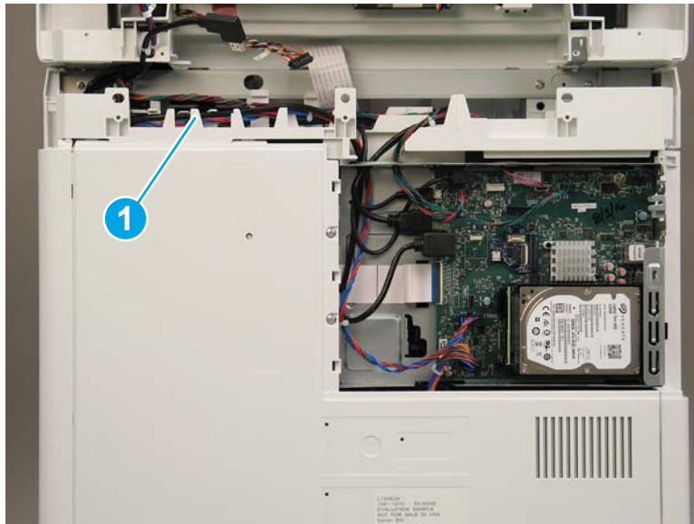
Figure 1-1342 Cable routing for M681 dh, M681f, and Flow M681f
