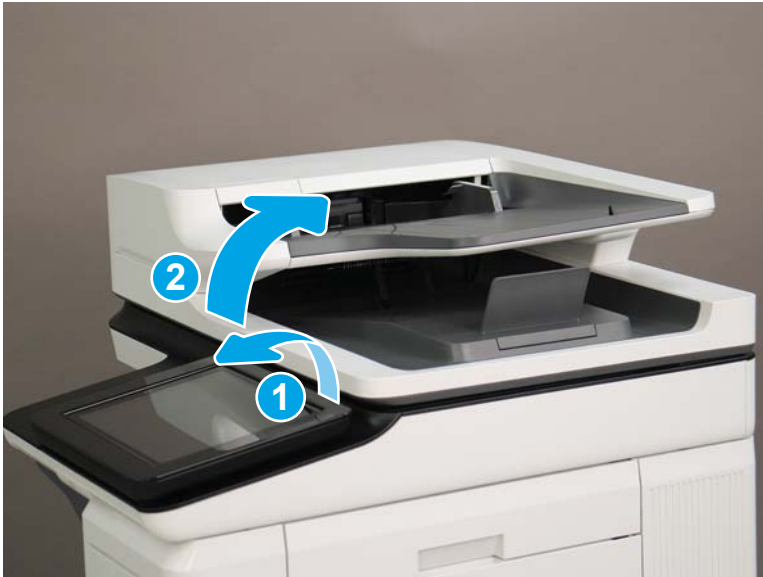
Figure 1-1764 Tilt the control panel and open the document feeder
