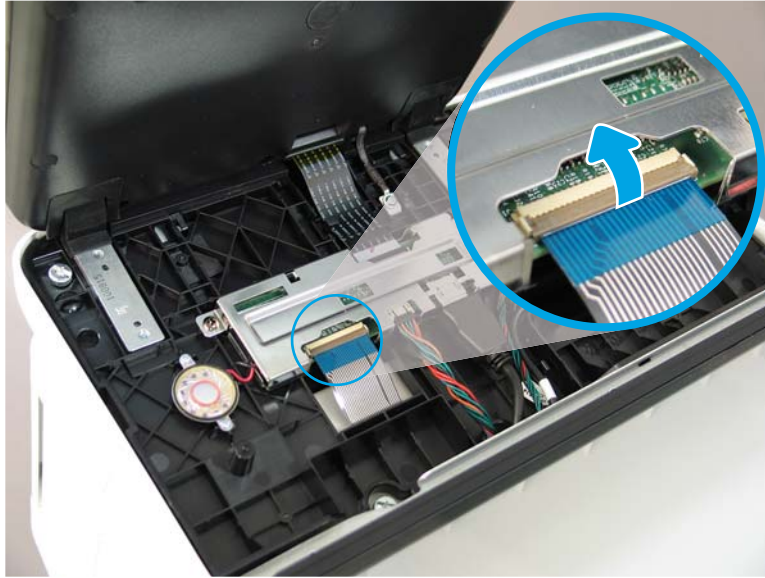
Figure 1-293 Disconnect the keyboard flat cable (keyboard models only)
