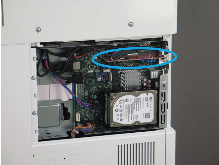
Figure 1-1392 Locate the fax PCA
