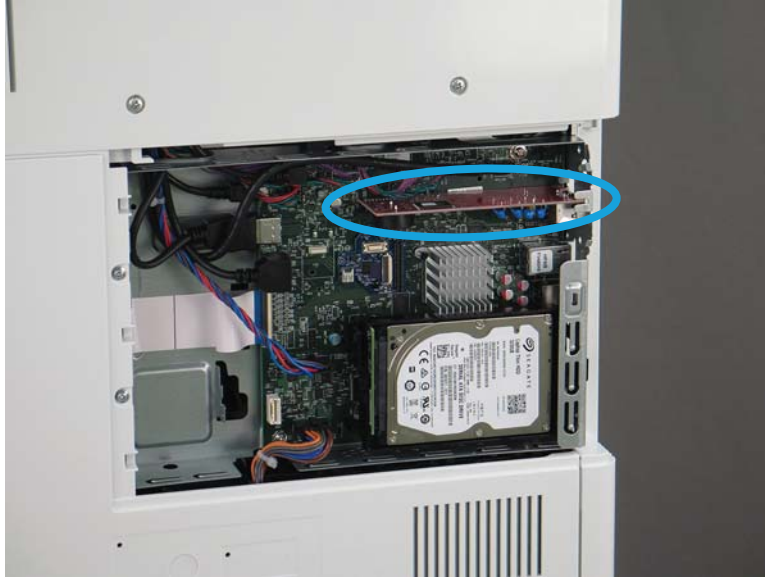
Figure 1-1833 Locate the fax PCA
