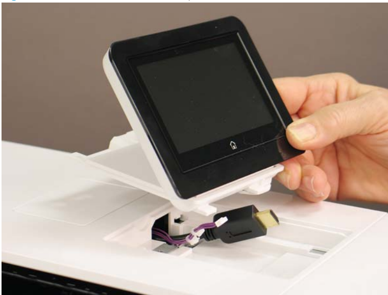
Figure 1-155 Remove the control panel
