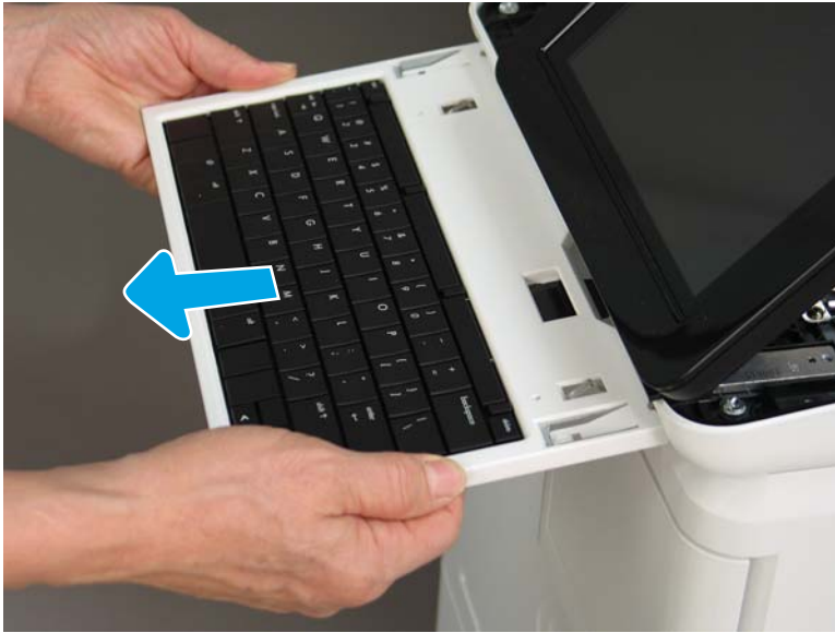
Figure 1-654 Remove the keyboard
