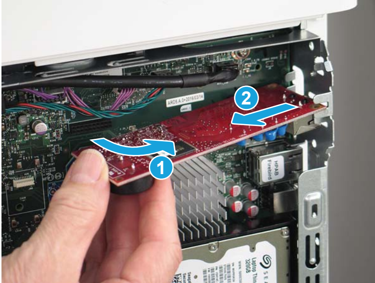
Figure 1-1622 Remove the fax PCA
