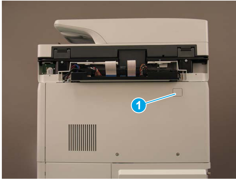
Figure 1-783 Remove one screw cover
