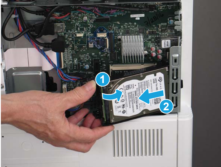
Figure 1-1745 Remove the HDD
