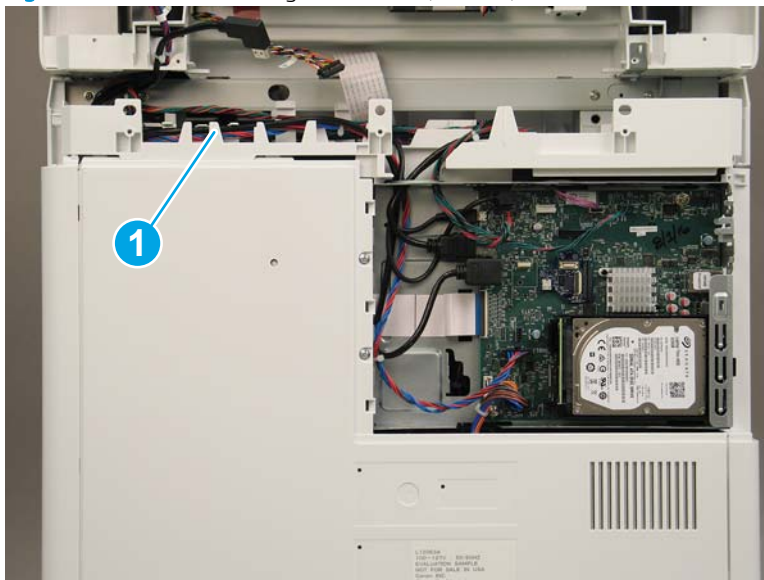
Figure 1-551 Cable routing for M681dh, M681f, and Flow M681f
