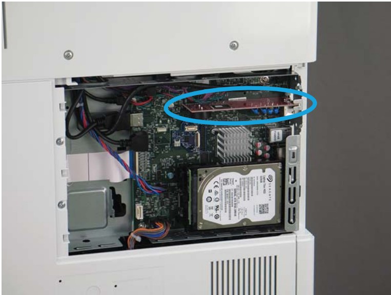
Figure 1-1742 Locate the fax PCA
