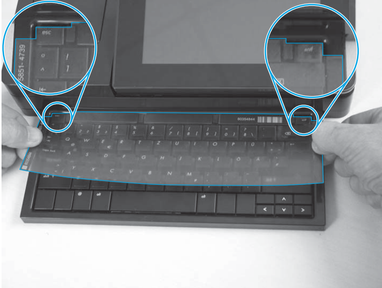
Figure 1-204 Position the keyboard overlay
