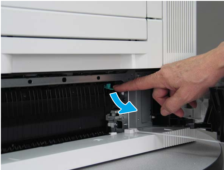
Figure 1-232 Lower the assembly cover
