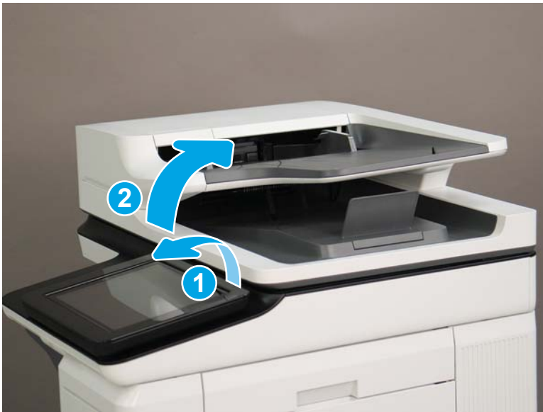
Figure 1-655 Tilt the control panel forward and open the document feeder
