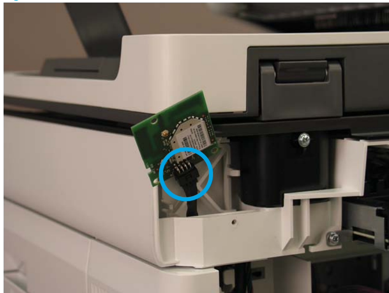
Figure 1-1051 Connect the wireless card connector
