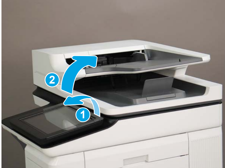
Figure 1-426 Tilt the control panel forward and open the document feeder
