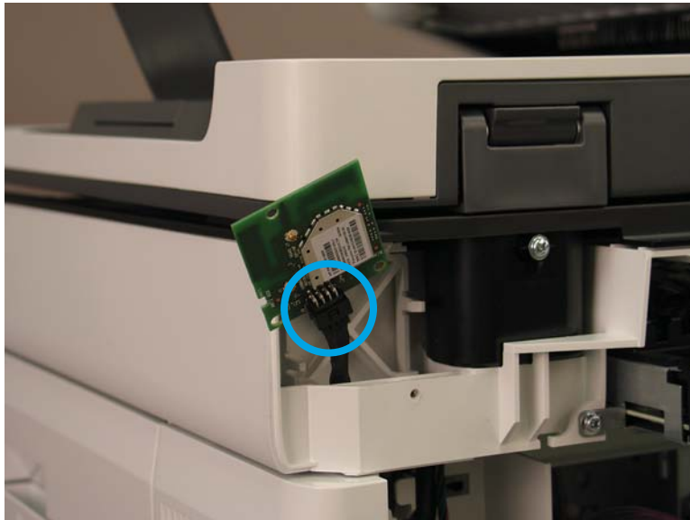
Figure 1-1670 Connect the wireless card connector
