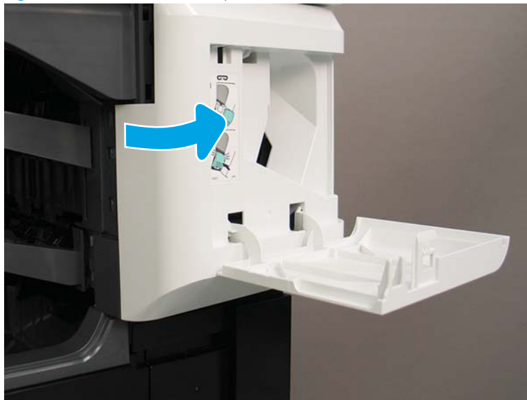
Figure 1-742 Remove the stapler cover.
