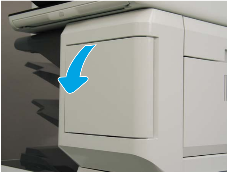
Figure 1-1355 Open the stapler door
