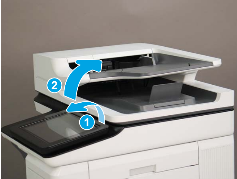
Figure 1-316 Tilt the control panel and open the document feeder
