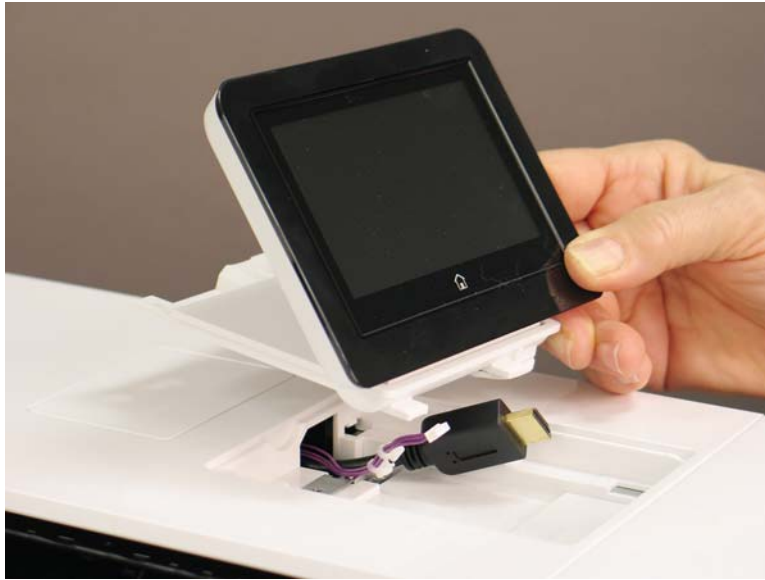
Figure 1-1162 Remove the control panel
