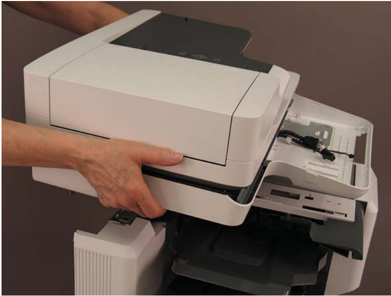
Figure 1-376 Remove the document feeder and image scanner
