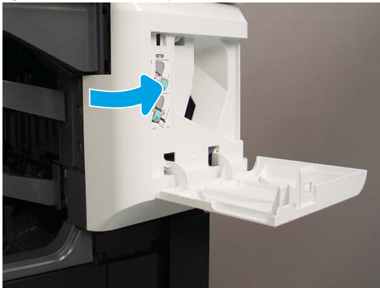
Figure 1-1358 Remove the stapler cover
