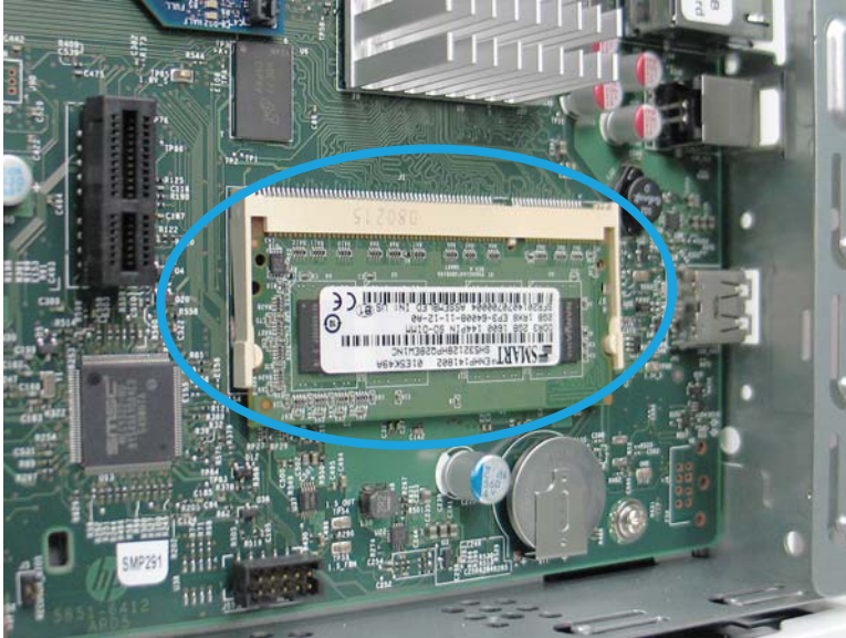
Figure 1-99 Locate the DIMM
