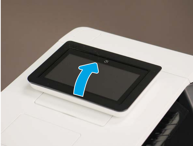
Figure 1-1461 Tilt the control panel up
