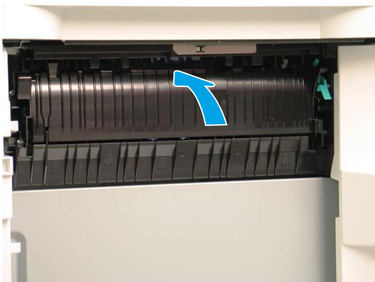
Figure 1-278 Close the feed assembly cover
