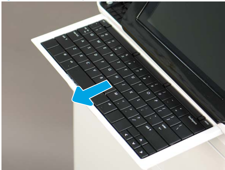
Figure 1-423 Slide the keyboard tray out
