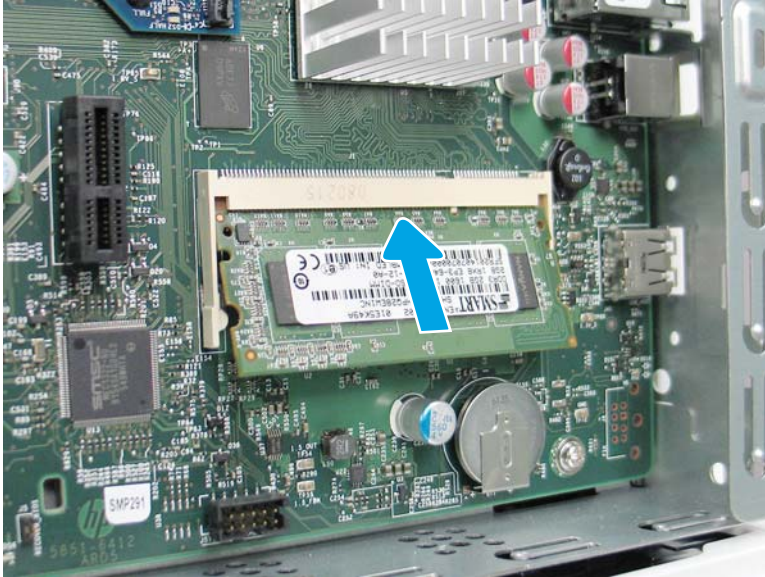
Figure 1-102 Insert the DIMM
