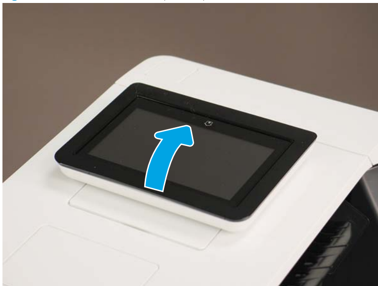
Figure 1-1234 Tilt the control panel up
