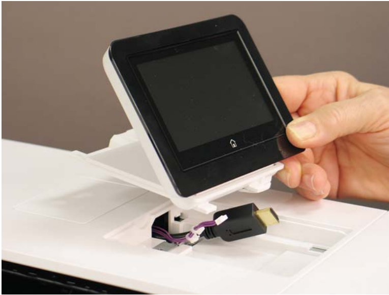
Figure 1-1239 Remove the control panel
