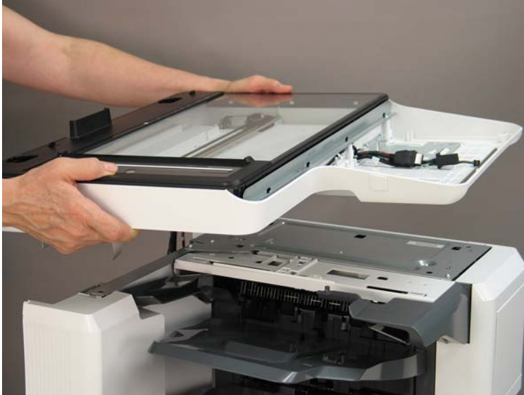
Figure 1-678 Remove the image scanner assembly
