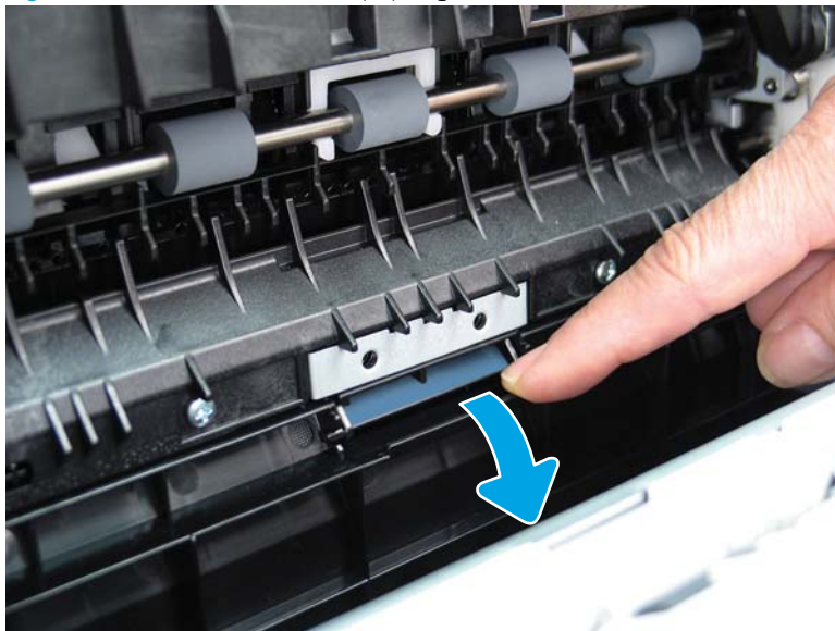
Figure 1-226 Lower the outer paper guide
