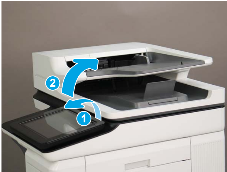
Figure 1-1904 Tilt the control panel forward and open the document feeder
