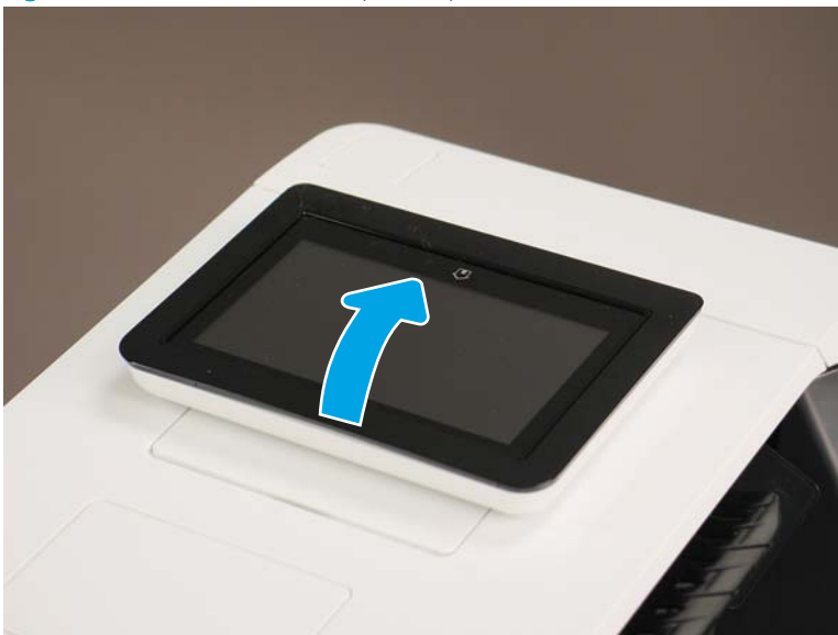
Figure 1-1818 Tilt the control panel up
