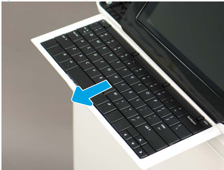
Figure 1-1184 Slide the keyboard tray out
