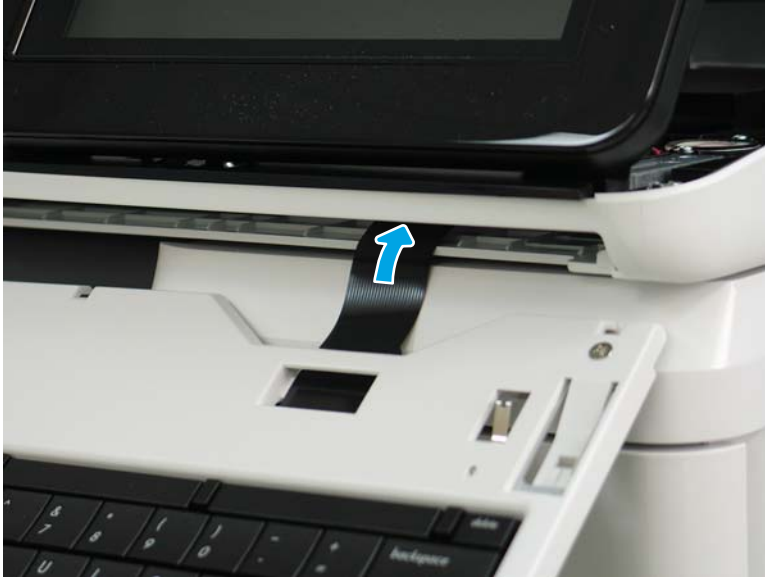
Figure 1-195 Position the flat cable in the slot
