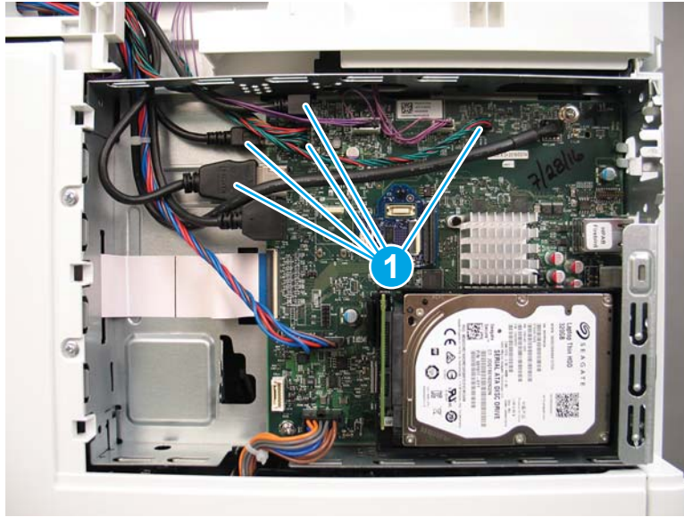
Figure 1-1044 Disconnect five connectors
