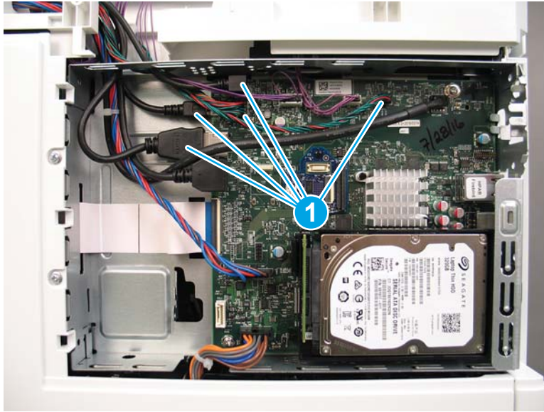
Figure 1-1124 Disconnect five connectors
