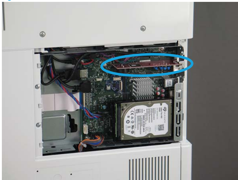
Figure 1-1621 Locate the fax PCA
