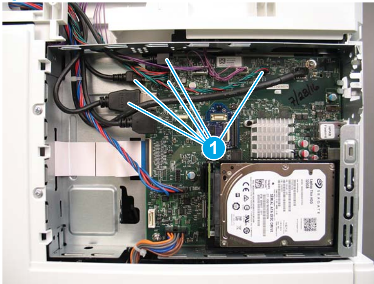
Figure 1-371 Disconnect five connectors
