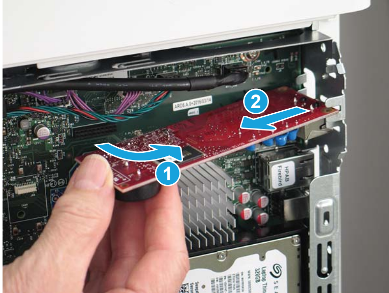
Figure 1-1604 Remove the fax PCA
