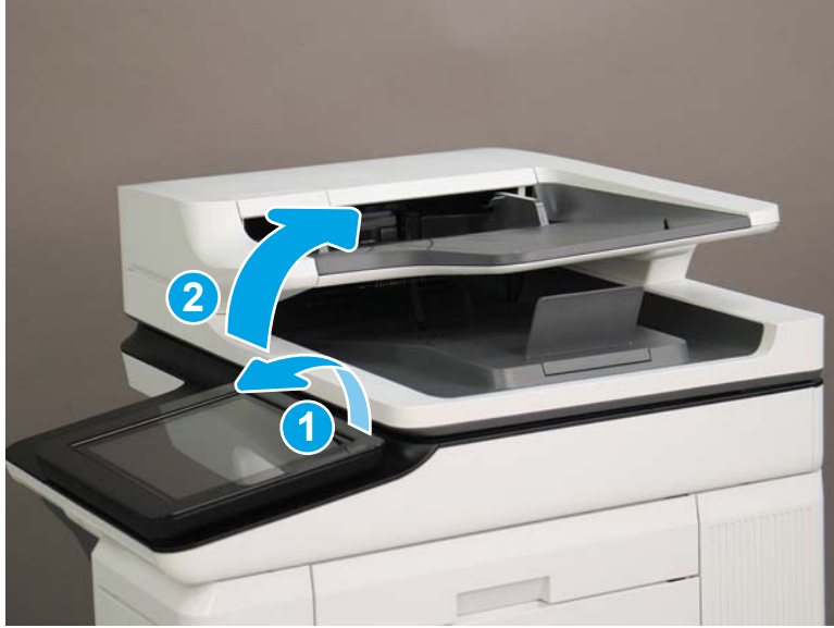
Figure 1-911 Tilt the control panel and open the document feeder
