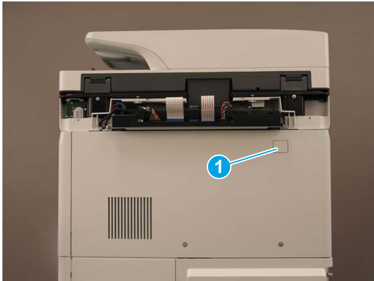
Figure 1-758 Remove one screw cover
