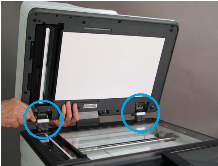
Figure 1-627 Release two tabs
