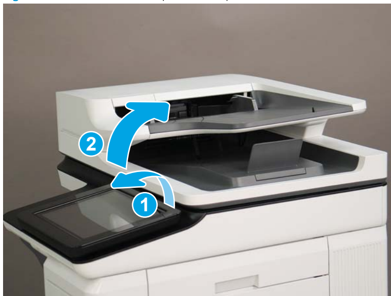
Figure 1-350 Tilt the control panel and open the document feeder
