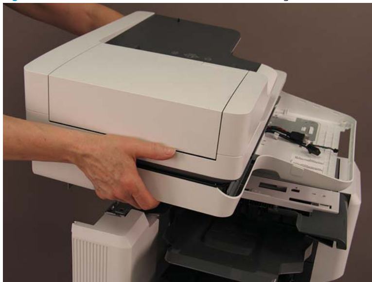
Figure 1-1049 Remove the document feeder and image scanner
