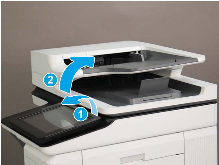
Figure 1-1642 Tilt the control panel and open the document feeder
