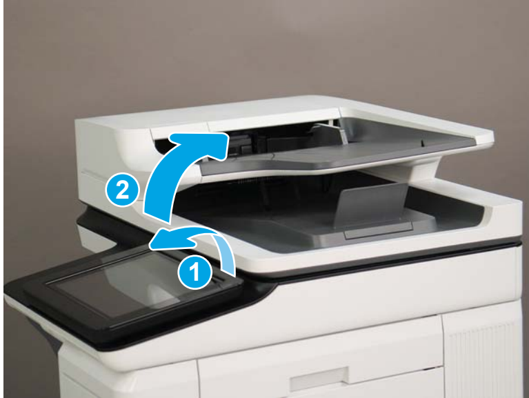
Figure 1-836 Tilt the control panel and open the document feeder
