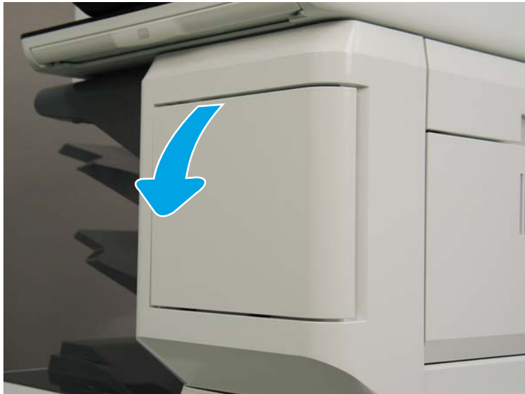
Figure 1-789 Open the stapler door
