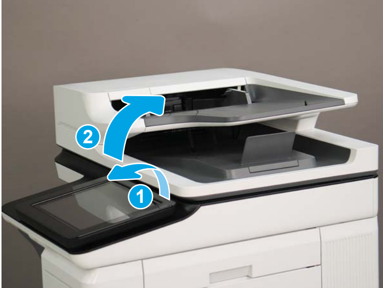
Figure 1-1771 Tilt the control panel forward and open the document feeder
