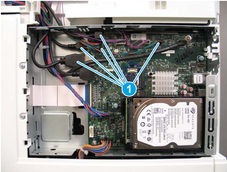
Figure 1-1344 Disconnect five connectors
