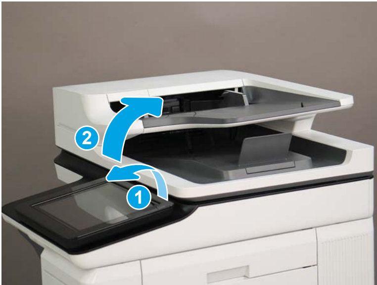
Figure 1-817 Tilt the control panel and open the document feeder
