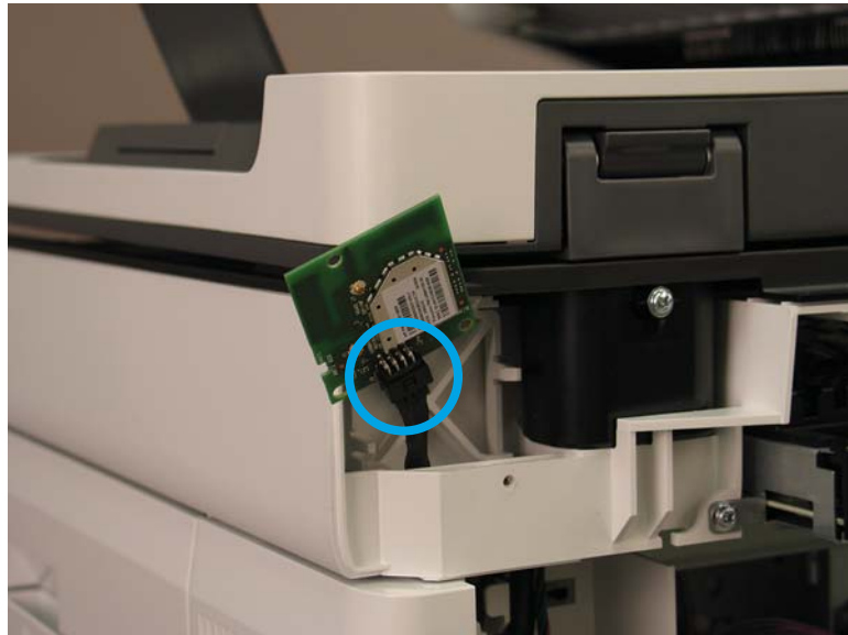
Figure 1-712 Connect the wireless card connector
