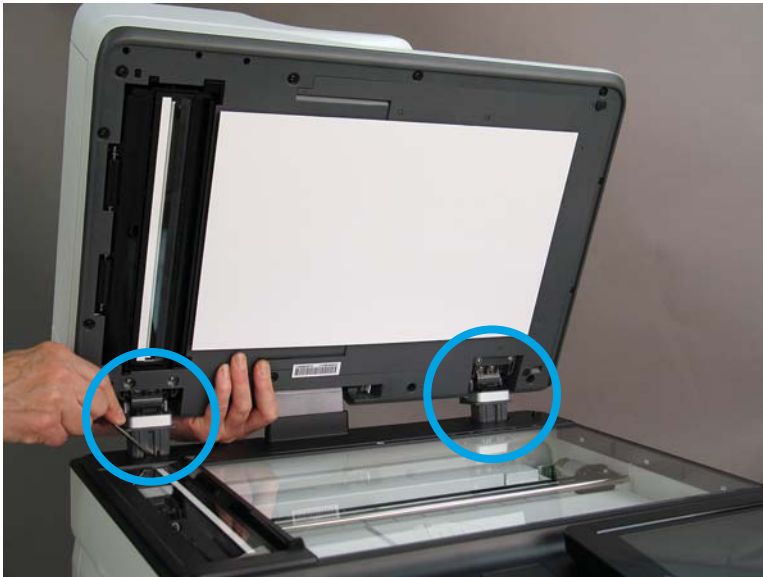
Figure 1-635 Release two tabs
