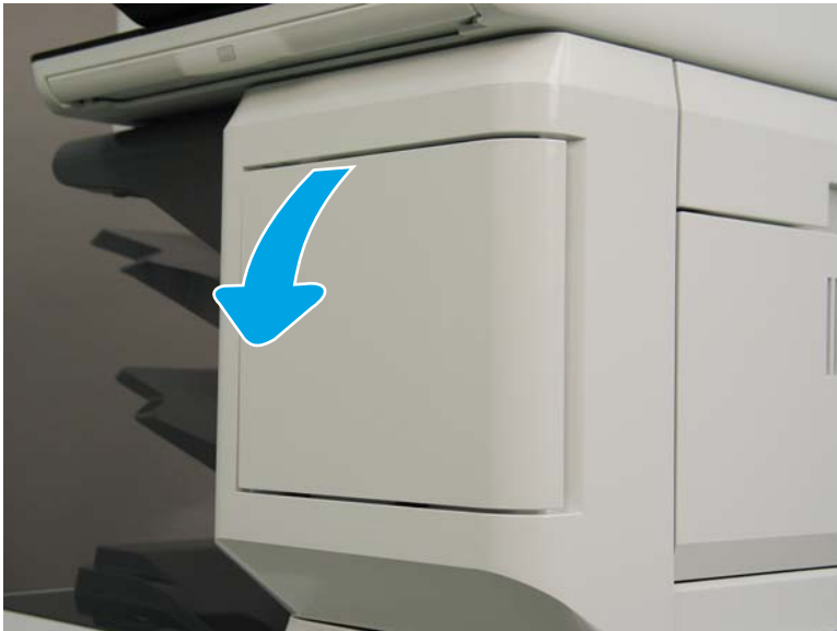
Figure 1-813 Open the stapler door
