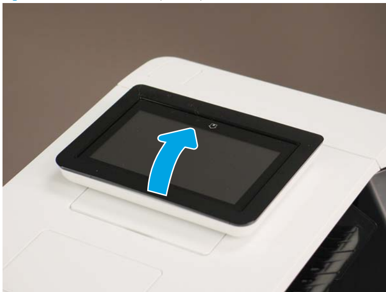
Figure 1-518 Tilt the control panel up
