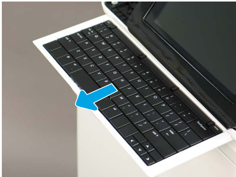
Figure 1-202 Slide the keyboard tray out
