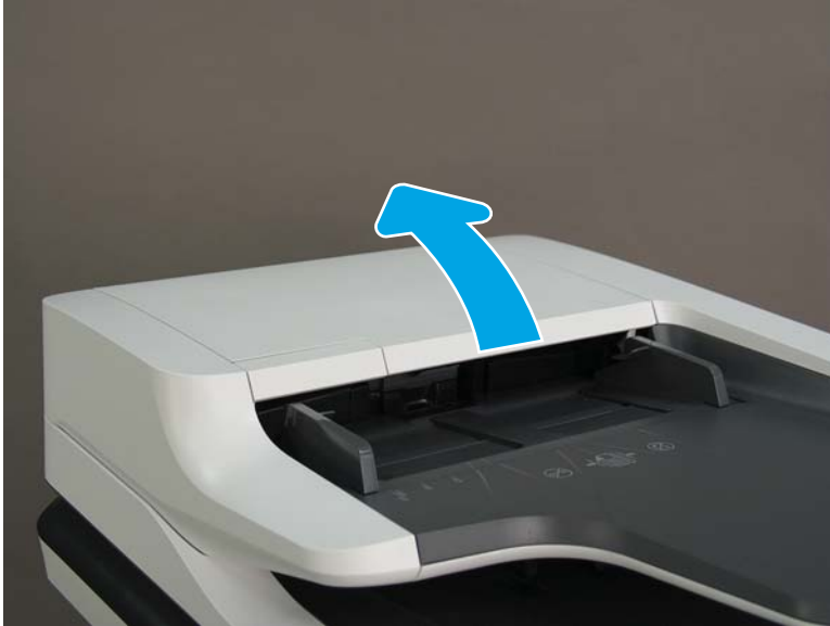
Figure 1-116 Open the document feeder cover
