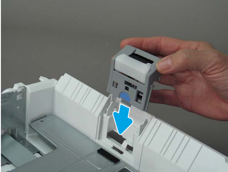
Figure 1-238 Install the roller assembly
