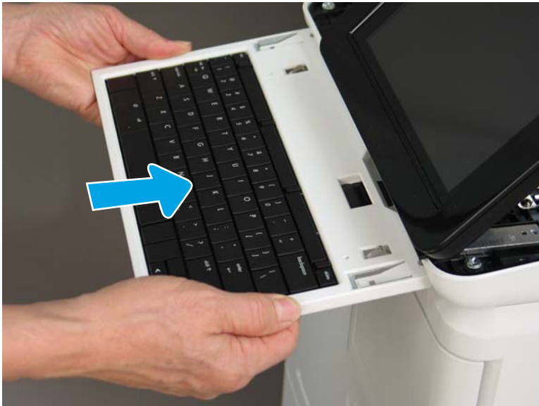
Figure 1-196 Slide the keyboard tray into the slot
