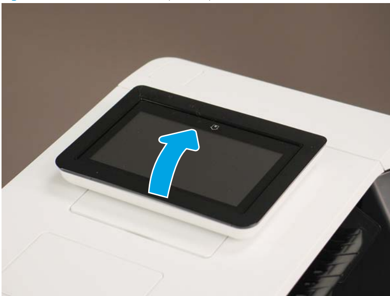
Figure 1-1157 Tilt the control panel up
