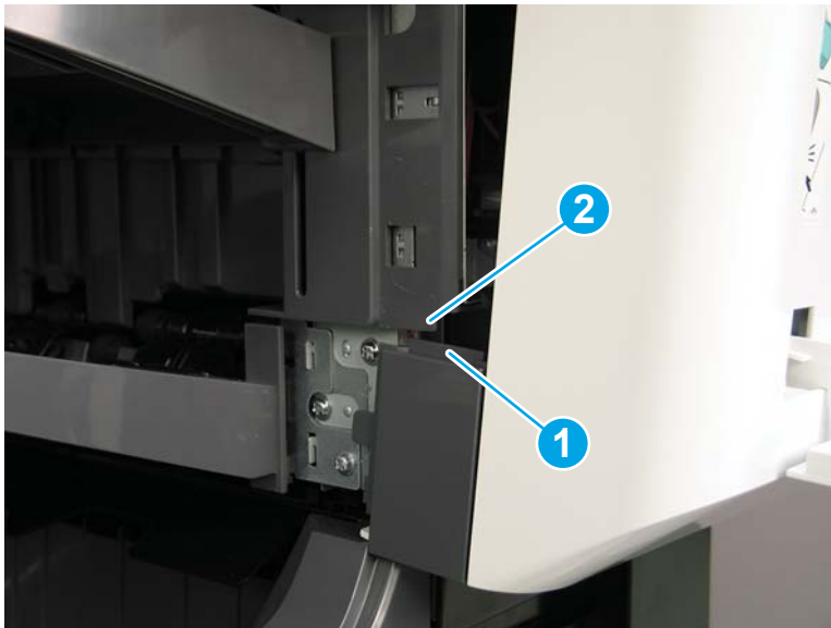
Figure 1-835 Position the tab
