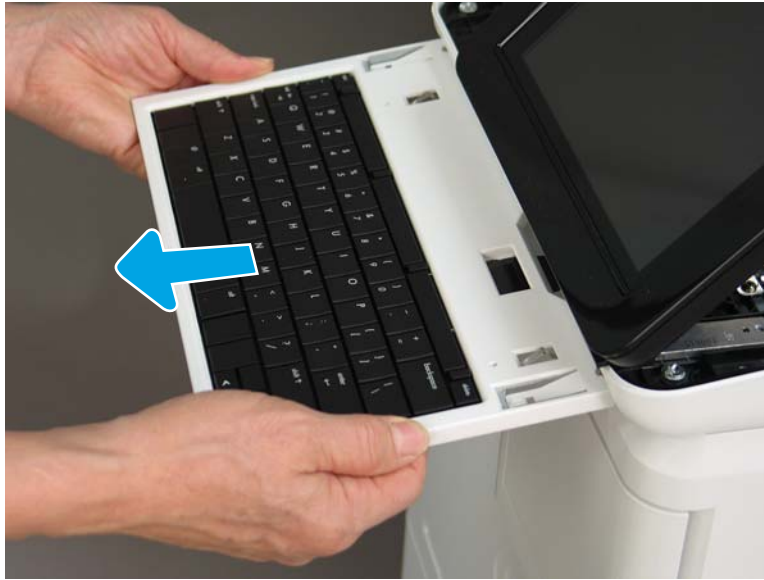
Figure 1-194 Remove the keyboard
