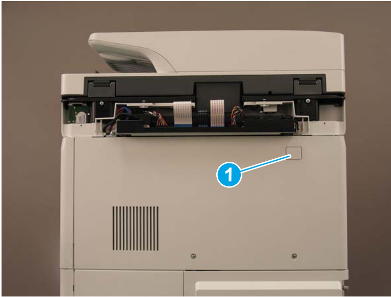
Figure 1-824 Remove one screw cover
