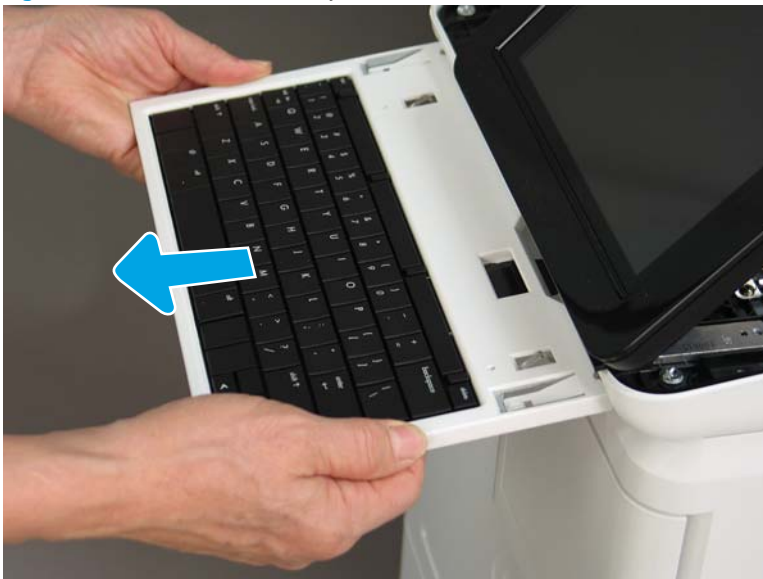
Figure 1-1186 Remove the keyboard
