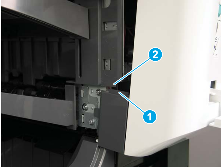
Figure 1-781 Position the tab
