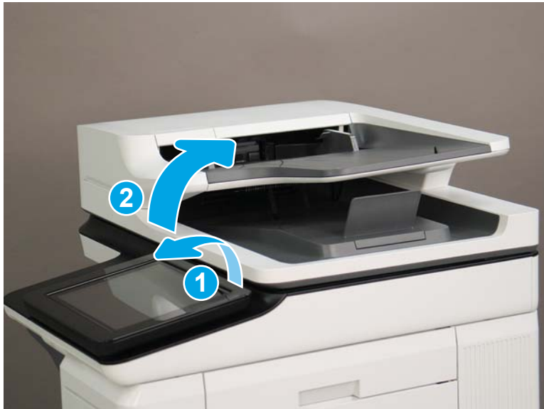
Figure 1-1414 Tilt the control panel forward and open the document feeder
