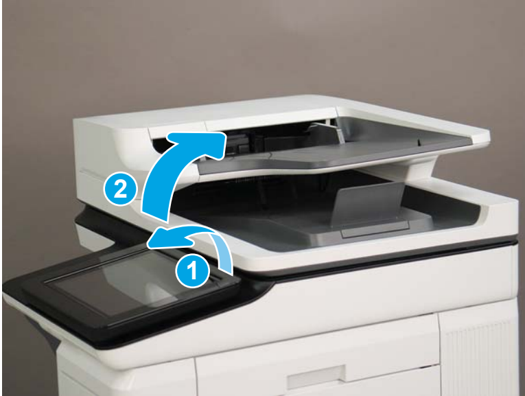
Figure 1-1030 Tilt the control panel forward and open the document feeder
