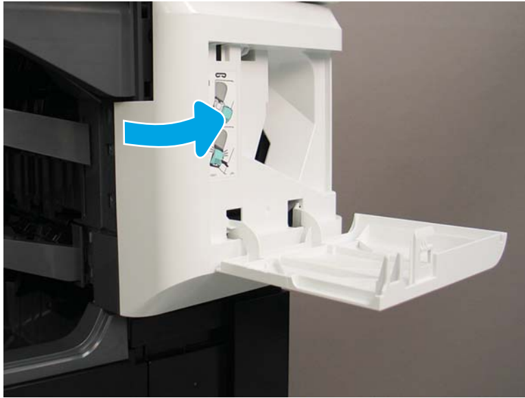
Figure 1-748 Remove the stapler cover.
