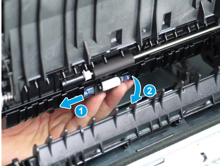
Figure 1-229 Remove the pickup roller assembly
