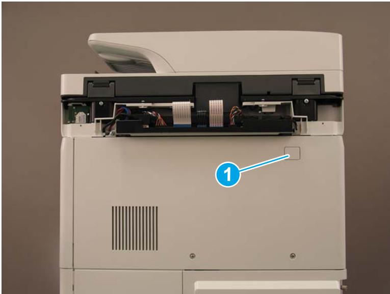
Figure 1-843 Remove one screw cover
