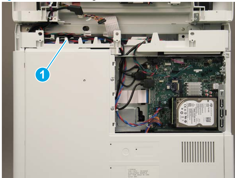
Figure 1-1916 Cable routing for M681 dh, M681f, and Flow M681f
