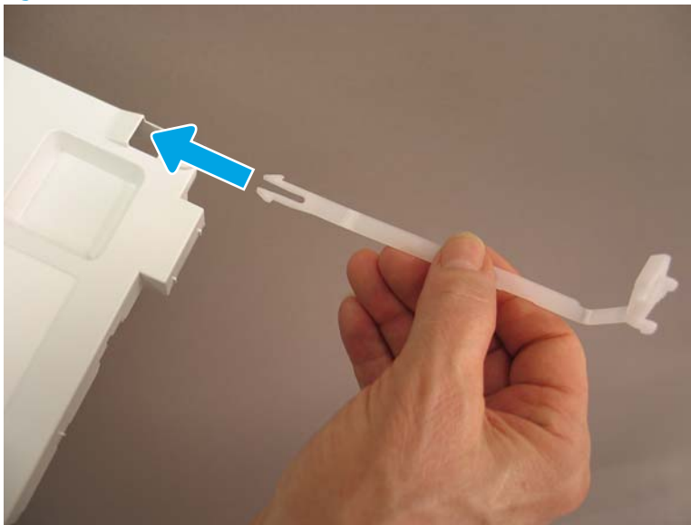
Figure 1-503 Reinstall the link arm
