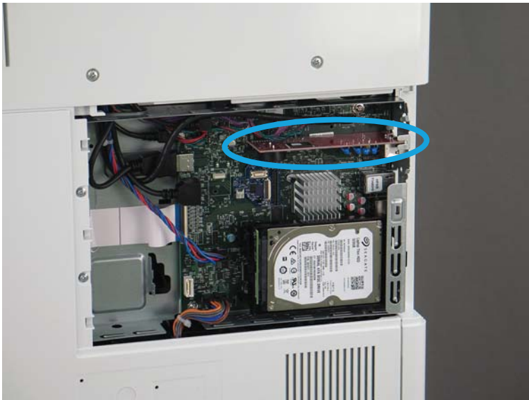
Figure 1-1603 Locate the fax PCA
