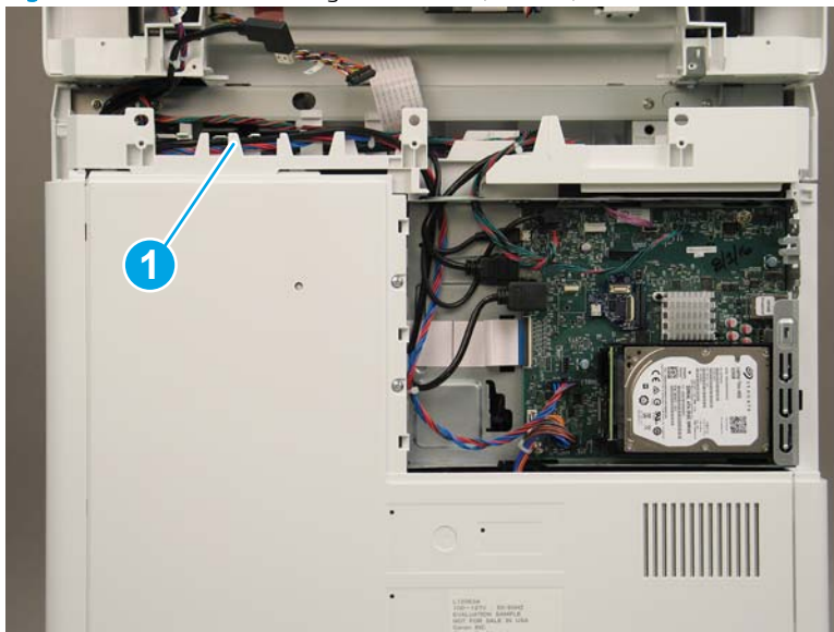
Figure 1-1426 Cable routing for M681 dh, M681f, and Flow M681f
