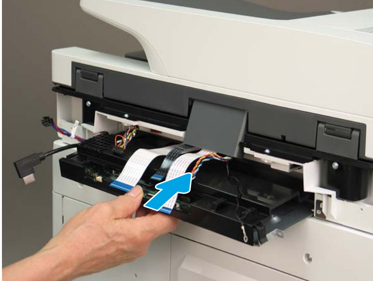
Figure 1-690 Check the cables when installing the SCB
