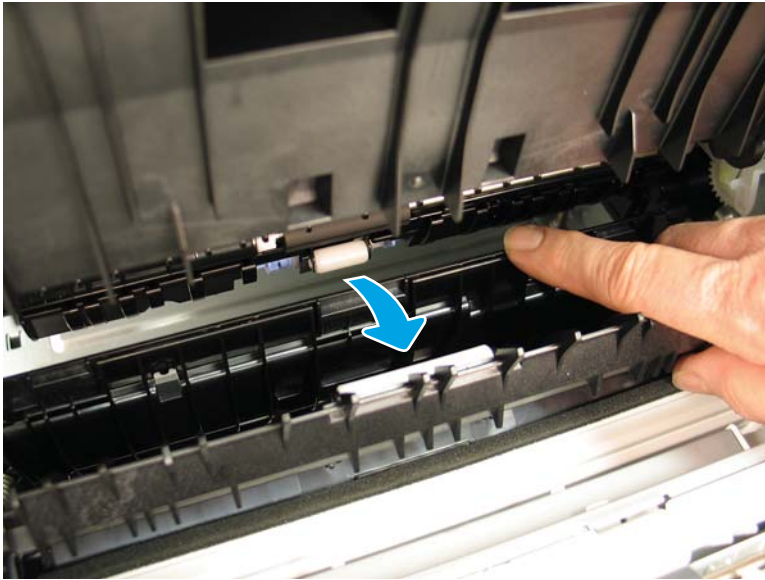
Figure 1-227 Lower the outer paper guide
