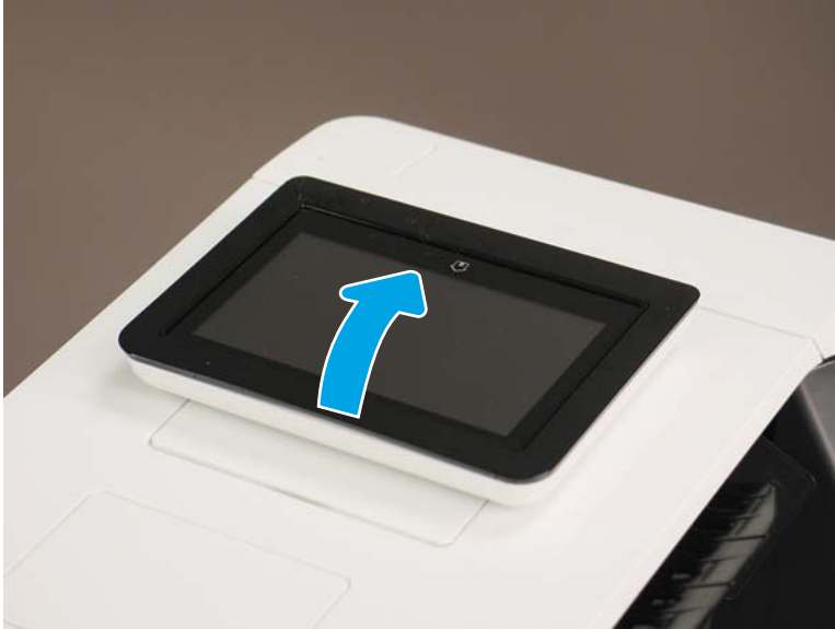
Figure 1-586 Tilt the control panel up
