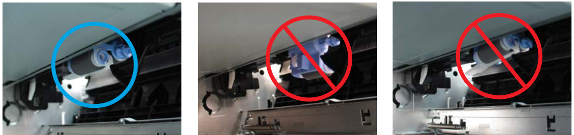
Figure 1-249 Roller correct and incorrect installation
