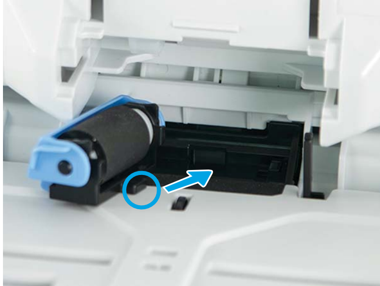
Figure 1-66 Note the tab on the roller
