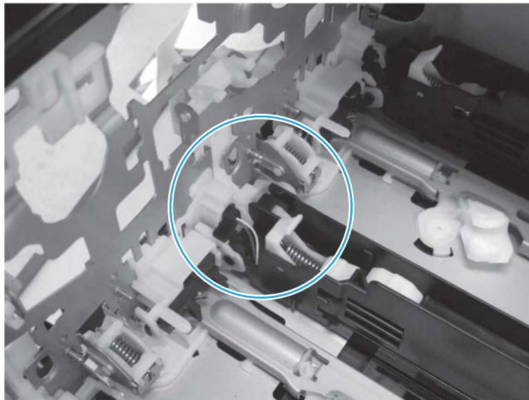
Figure 1-1016 Link arm correct installation (M751/E75245/M856/E85055/M776dn/M776z/M776zs)
