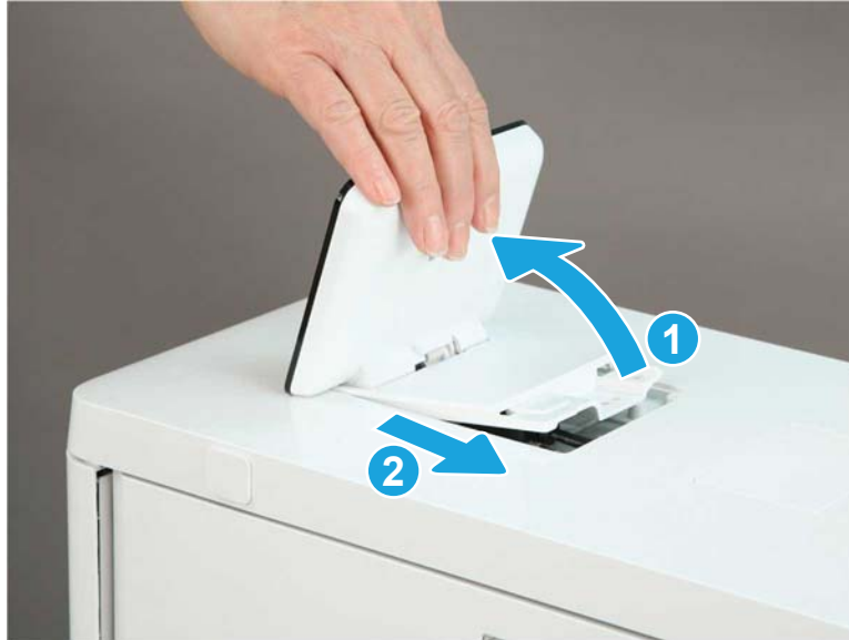
Figure 1-499 Slide the control panel back
