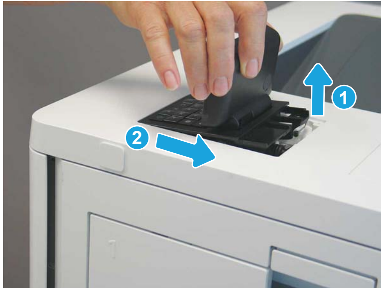
Figure 1-1416 Slide the control panel back
