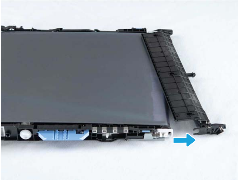
Figure 1-1208 Pivot the cleaner away from the ITB
