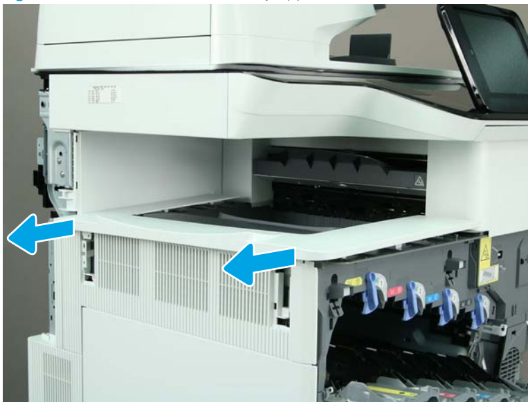
Figure 1-261 Remove the accessory upper cover
