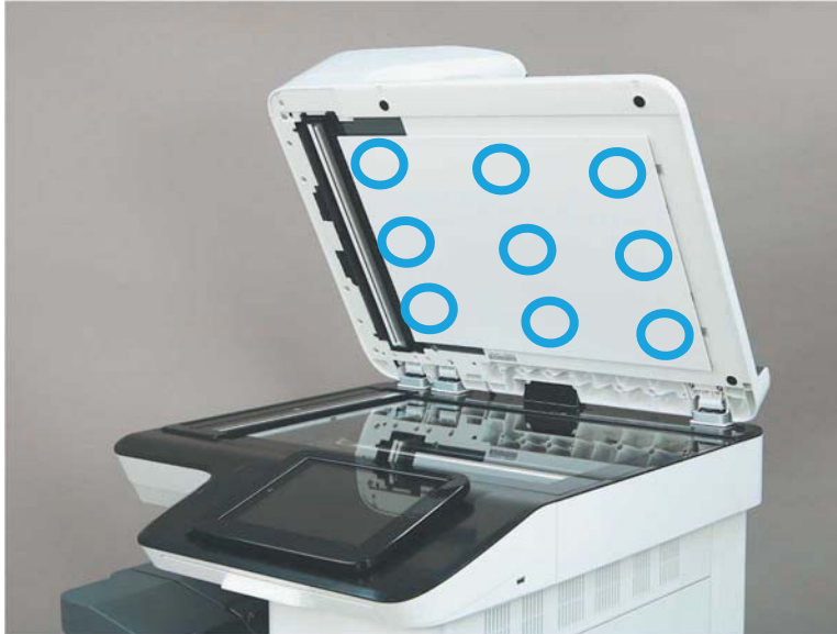
Figure 1-141 Reflector tabs location
