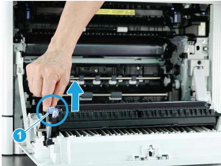
Figure 1-1596 Release the transfer roller
