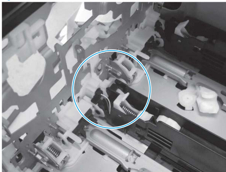
Figure 1-1040 Link arm correct installation (M751/E75245/M856/E85055/M776dn/M776z/M776zs)
