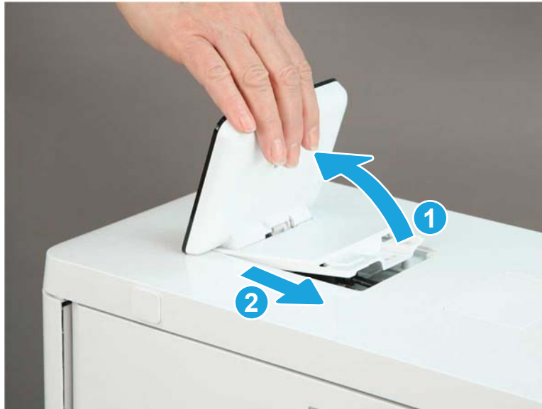
Figure 1-2460 Slide the control panel back
