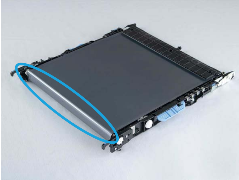
Figure 1-1196 Examine the front edge of the ITB
