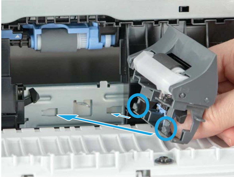
Figure 1-3211 Position the separation roller assembly
