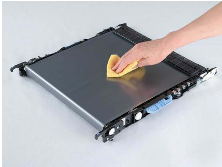
Figure 1-1203 Clean the ITB
