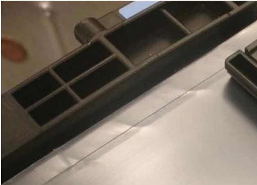
Figure 1-1200 Check for bent or creased edges
