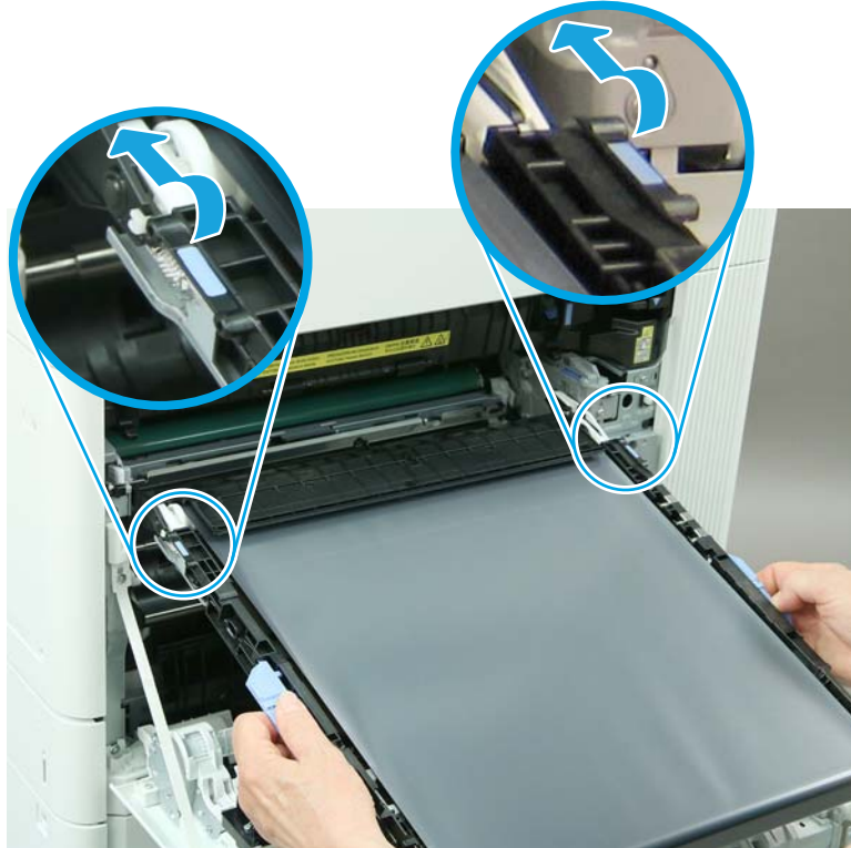
Figure 1-90 Align the ITB
