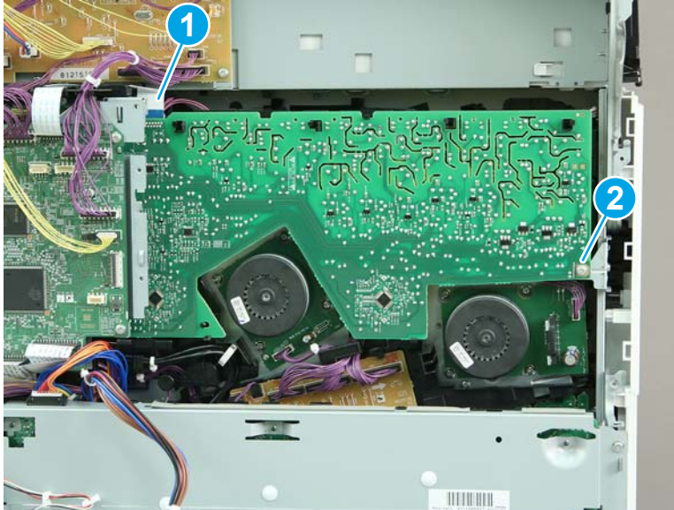
Figure 1-885 Disconnect one connector and remove one screw
