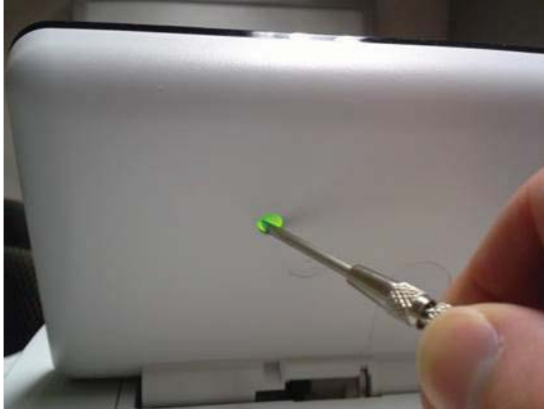
Figure 2-28 Press the diagnostics-access button (M856/E85055)
