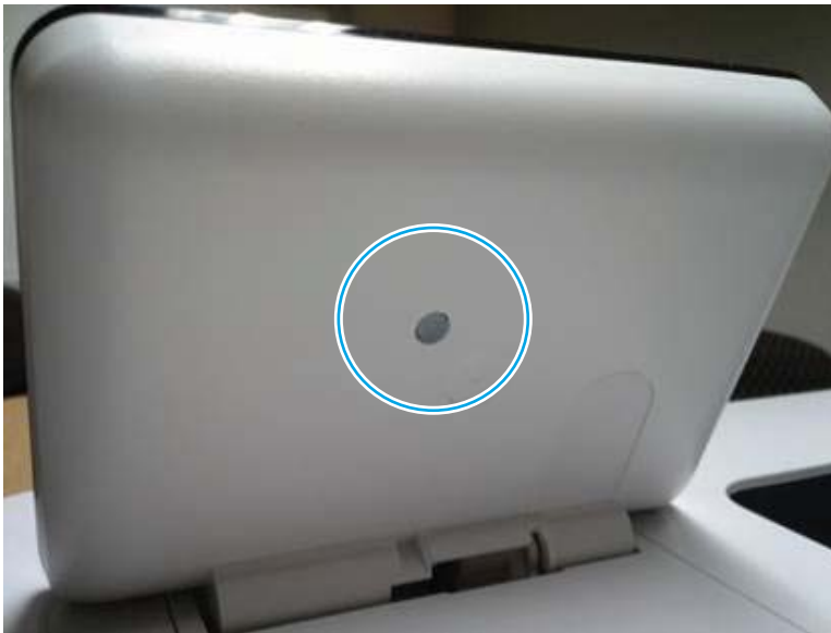
Figure 2-27 Diagnostic-tests access button (M856/E85055)
