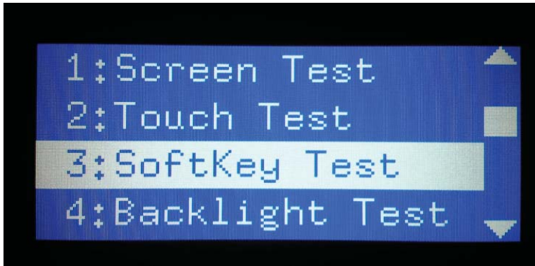
Figure 2-41 Open the softkey test
