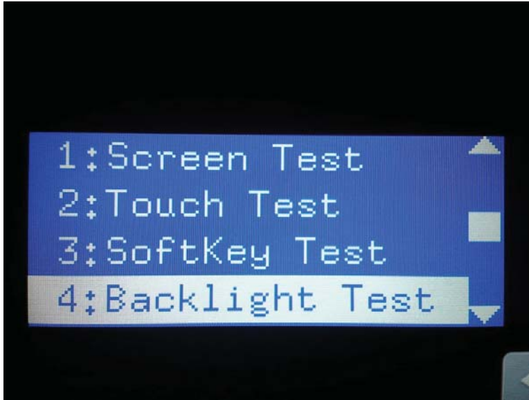
Figure 2-44 Open the backlight test
