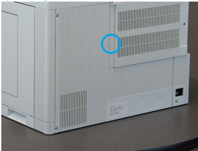
Figure 2-54 Engine test button
