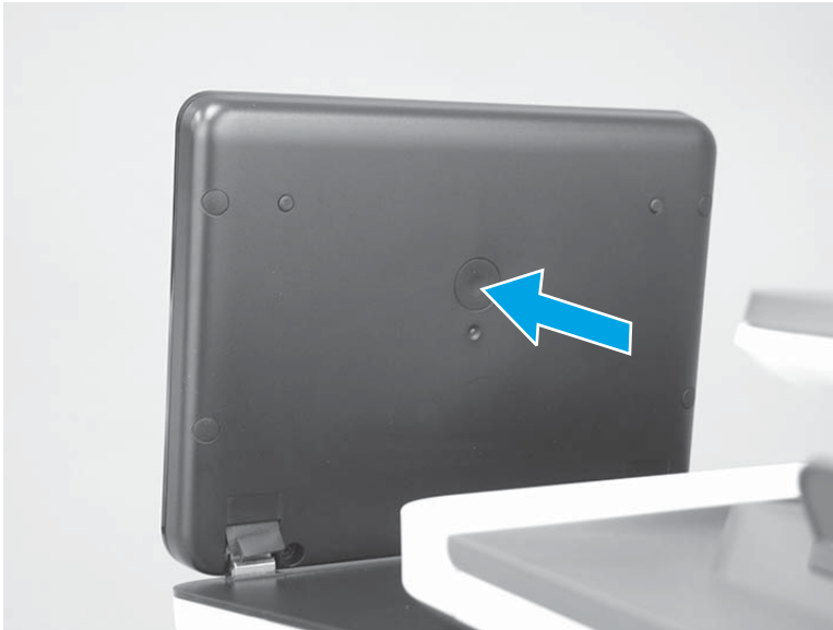
Figure 2-30 Press the diagnostics-access button (M776)
