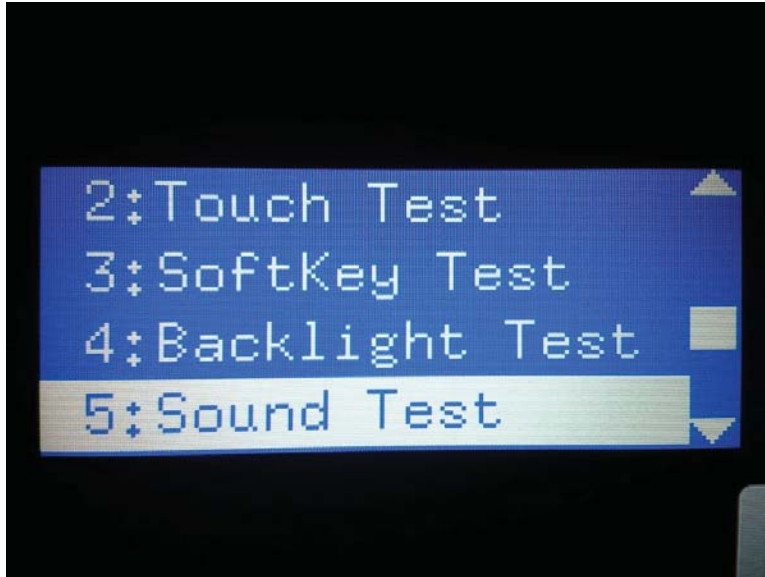
Figure 2-45 Open the sound test
