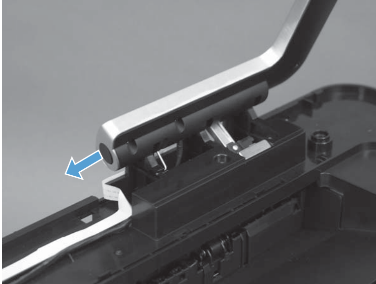
Figure 1-18 Remove the camera arm assembly (2 of 6)
