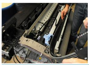
NOTE: After installing the carriage, when closing the latch, make sure the carriage is placed in the printhead replacement position so the carriage doesn't interfere with the rear guide.
