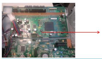
MARNING! If the engine PCA is not removed before the formatter, the bridge connections may be damaged.
