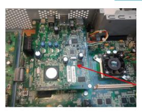
4. Remove the two screws shown.
