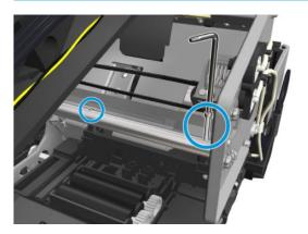
Remove the 2 T-15 screws and the left bracket. 6.
