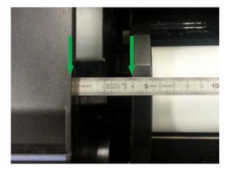
If customer is using 36 inch paper roll width, measure distance on the blue hub on the right (as shown in picture below). This distance should be greater than 4.5 cm otherwise, the blue hub is probably not completely inserted into the roll core.
