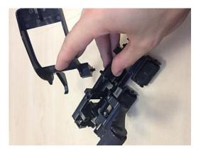
Assemble multi-function printer stacker wheel lifters
