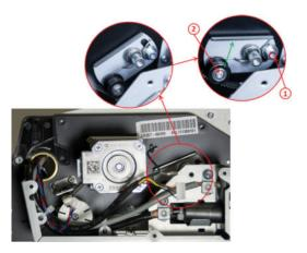
Remove the motor screws.
