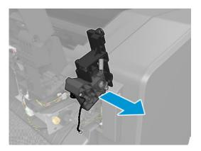
**6.** Remove the screw and microswitch (sensor).
