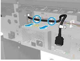
6. Remove the screw, pull the cable through the hole, and unclip it.
