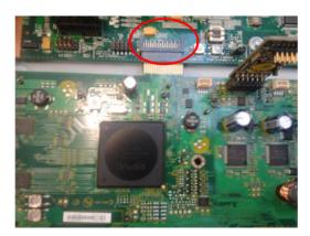
NOTE: The red PCA, Cryptoasic sim, must be installed in the new engine PCA.
