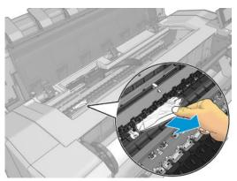
**IMPORTANT:** Remove remaining paper by carefully pulling it out in the direction of the paper axis.
