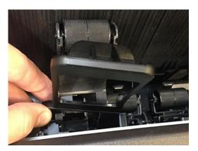
2. Push the stacker wheel lifter's left leg to align the left pin with the left groove.
