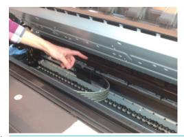
NOTE: An angle screwdriver is needed, if not, you will have to remove scanner covers (FP and SVS side).
