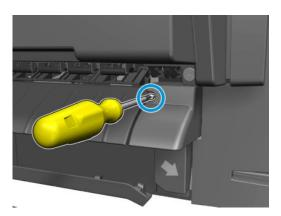
Remove the arch sidewall cover from the service station side.
