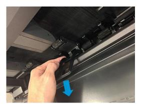
2. Push the stacker wheel lifter's left leg to unclip it. Be sure not unclip the second wheel holder.
