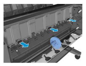
Remove the 3 T-15 screws underneath.
