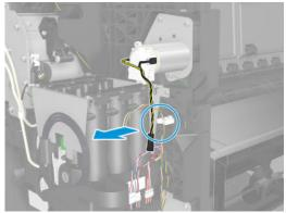
Remove 3 T-15 screws and the rewinder.
