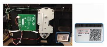
5. Disconnect and take out from route location the encoder cable and motor cable.
