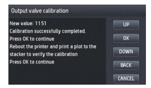
5. By pressing **OK** in the next screen, the printer will shut down automatically.
