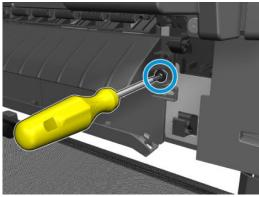
Remove the output platen.
