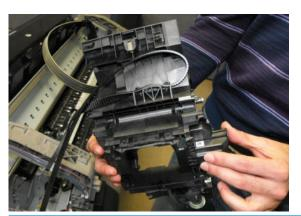
NOTE: When assembling the belt, make sure that it is correctly attached to the tensioner and scan axis motor pin. If not, the belt can rapidly become worn out, and/or make noise.
