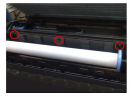
Unhook the 2 hooks, and remove the bumper.
