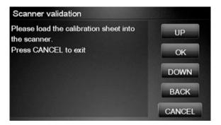
Hold the calibration sheet from both sides and place it facing the arrow in the centre of the sheet in front of the Page icon present on the input tray of the scanner. Push the sheet with both hands on both sides at the same time to load the sheet with no skew. Press OK to continue with the test.
