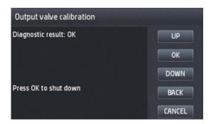
6. Power – on the printer, and print (for example a Drawing Demo print) to the stacker, to verify the success of the calibration.
