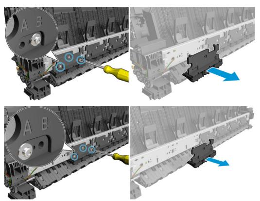
NOTE: For installation make sure that you install the 1st pinch using hole B.
