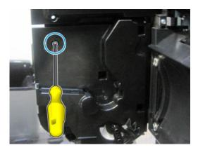
6. Remove 3 T-15 screws and the rewinder.
