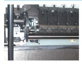
Remove the circlip.
