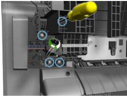
Remove the stacker, pulling the handles on the back.
