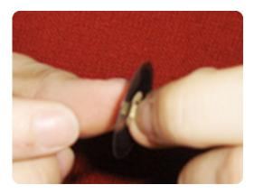
2. Pre-assemble the encoder on the roller without using pressure.
