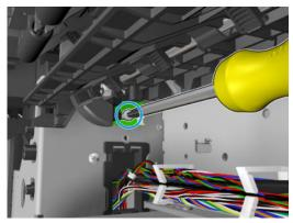
Remove the sensor valves.
