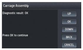
If an error has been found in any of the steps of this diagnostic (parameter values are out of the allowed range; printhead improperly detected or not detected, sensor errors, etc.) the diagnostic test will automatically detect it and stop the test (checks will stop), and the error description will be shown in the front panel. The error description will contain the System Error code (for determining the recovery action) and the specific error cause, if known.
