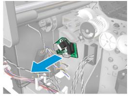
6. Disconnect the cable, and remove the 3 screws.
