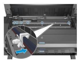
4. Remove 2 T-20 screws, and the second starwheel rail.
