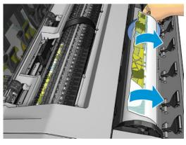
7. If the leading edge of the paper is ragged, trim it carefully with scissors.
