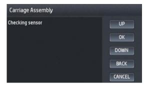
After the line sensor has been checked, you're asked to insert the printheads again. To do so, open the printer window, open the carriage cover, and insert the printheads into the carriage. Then, close the carriage cover, printer window, and then press **OK**.
