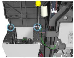
Remove the bracket and side plate.
