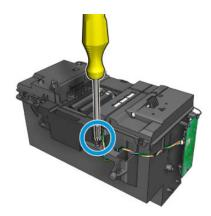
Remove the Drop Detector from the service station.
