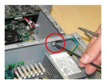
Remove the power supply unit.
