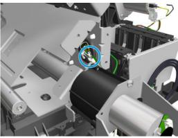
11. Rotate, unlock, and remove the auto pinch lifter.
