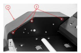
3. Remove the screws (1), and then the motor cover (2).
