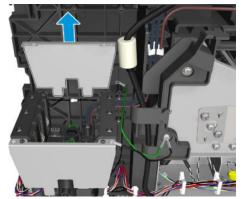
Remove 2 screws and the side plate.
