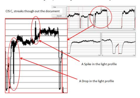
A light profile with an about 20 pixel drop can be a contaminated lens in the CIS module.
