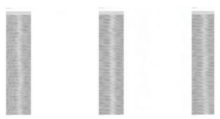
The most uniformly centered will be the white/lightest band; better the media advance the printer has.
