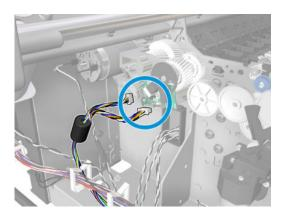
Remove the 2 screws and remove the connectors.
