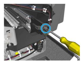
Remove the bump cutter actuator.
