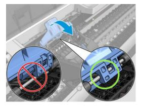
**b.** The latch is completely down.
