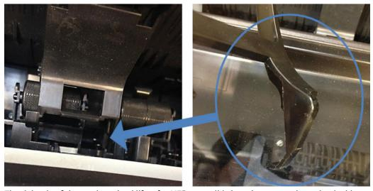
The right pin of the stacker wheel lifter for MFP must slide into the groove shown by the blue arrow.
