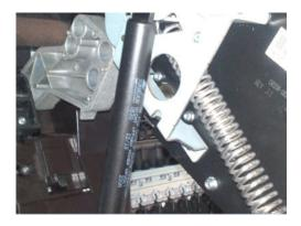
Remove the lift assembly. See <u>Lift assembly on page 422</u>.
