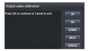
The screen will show the 'calibrating status' during some minutes, while the output valve is performing some movements.
