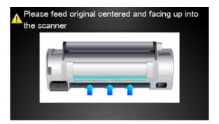
The Control Panel prompts you to feed the original. Load the Scanner IQ plot that you printed previously 8. in the Scanner input tray. Wait then for the product to scan and print the image.
