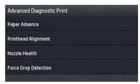
All the diagnostic Prints (except **Force Drop Detection**) require that the printer be ready to print (paper loaded, printhead and supplies installed). At the beginning of each diagnostic, you will see the following screen:
