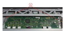
Unclip the USB Cable and pull it gently out of the CIS bridge (1). Remove the screws and unclip the cable (2).
