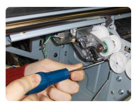
Loosen the encoder sensor adjustment screw.
