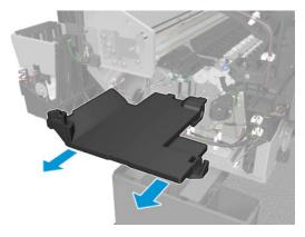
Remove the first starwheel rail. See <u>Customer Self Repair Flyers on page 442</u>.
