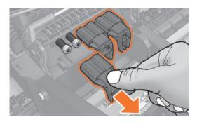
3. After inserting the printhead, the printer will check electronic connections. If the check fails, the printer will ask to reseat the printhead.
