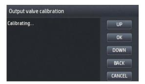
At the end of the process, you will have the result of the calibration. The screen will show also a recommendation to verify the calibration (print a plot to stacker). Typical values for the calibration range from 1015 to 1225.
