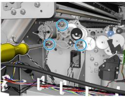
**7.** Remove the paper axis motor.
