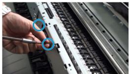
Remove the ISSWALL (removing 2 T-10 screws).
