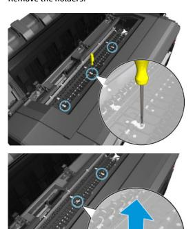
5. Lift up the flap at both sides and remove the overdrive.
