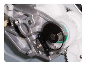
Press the encoder using the Media Advance Drive Adjustment Tool (reversed) so that it sticks to the roller.
