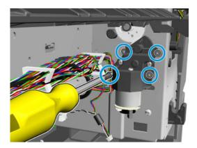
4. Remove the valves motor.
