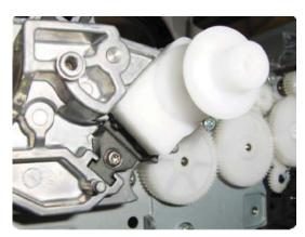
Position the Media Advance Drive Adjustment Tool on the end Media Advance Roller shaft, push it firmly onto the shaft and maintain a constant pressure to ensure it is flush to the Media Advance Drive.
