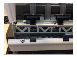
Replace the broken batch scanning piece.
