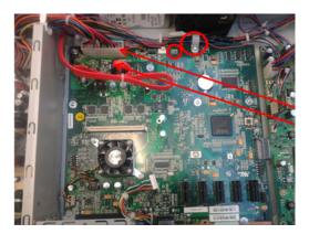
Remove four T-8 screws and the L-shaped metal sheet.
