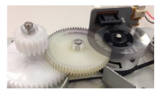
12. Reassemble the Transmission Plate in the Service Station. First screw the Grounding Cable.
