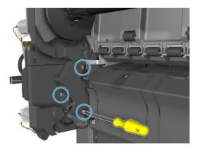
7. Remove the bottom rewinder support.
