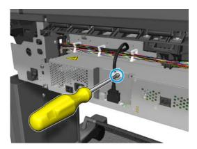
Disconnect and unclip the front panel cable.
