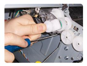
**7.** While maintaining pressure on the Media Advance Drive Adjustment Tool, fully tighten the encoder sensor adjustment screw.
