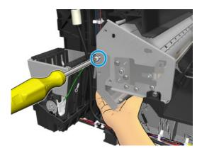
8. Remove the Scan Axis Motor.
