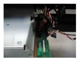
6. Remove the E-Box from the printer.
