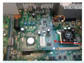
NOTE: When replacing the Jester PCA, also replace the small inter-connector provided with the kit.
