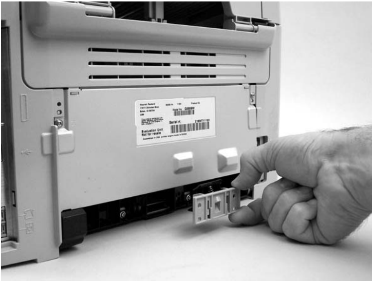
Figure 5-87 Removing the printer separation pad (2 of 2)
