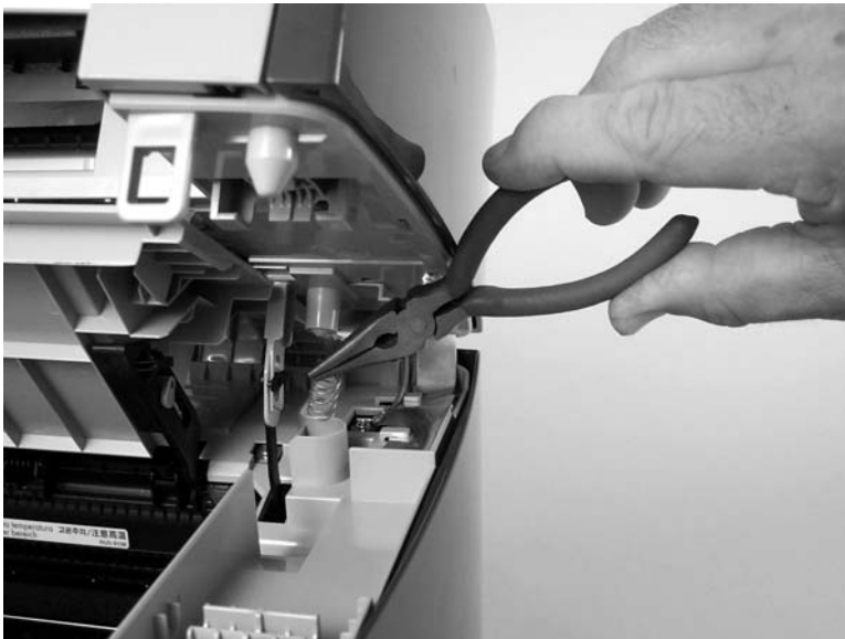
Figure 5-9 Removing the link assemblies and scanner support-frame springs (4 of 4)
