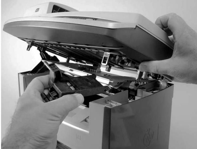
Figure 5-56 Removing the link assemblies and scanner support-frame springs (3 of 4)
