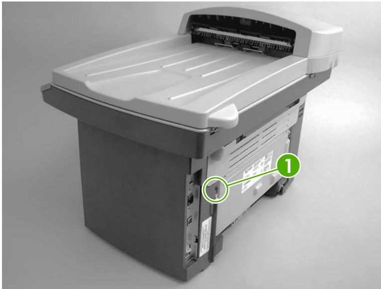
Figure 5-72 Removing the scanner assembly (1 of 13)
