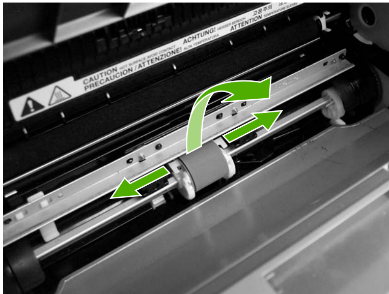
Figure 5-91 Removing the printer pickup roller (2 of 5)
