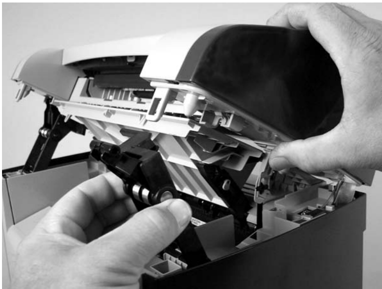
Figure 5-7 Removing the link assemblies and scanner support-frame springs (2 of 4)
