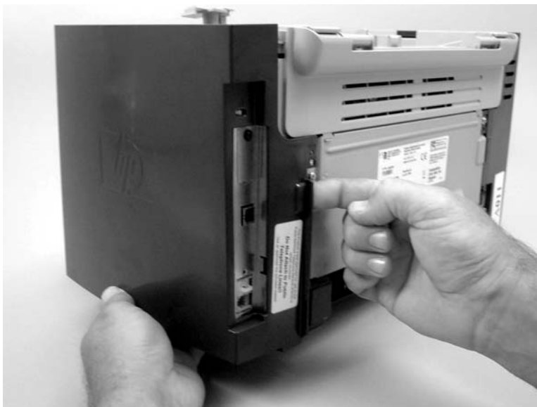
Figure 5-103 Removing the side covers (2 of 4)
