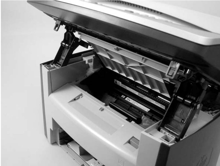
Figure 5-88 Removing the print cartridge (1 of 2)
