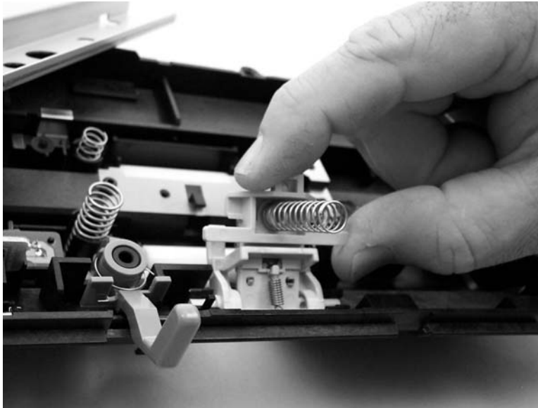
Figure 5-20 Removing the separation-pad assembly (2 of 3)
