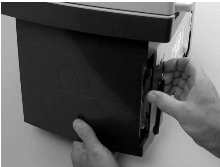
Figure 5-73 Removing the scanner assembly (2 of 13)
