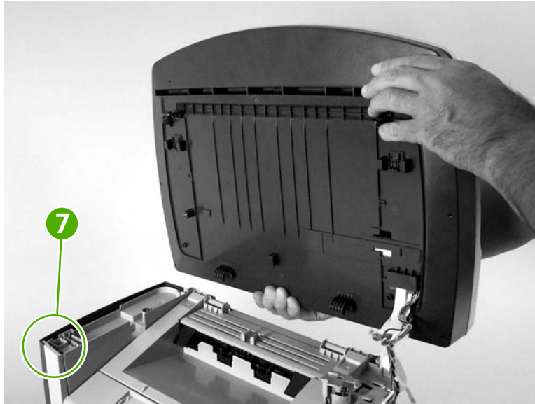
Figure 5-84 Removing the scanner assembly (13 of 13)
