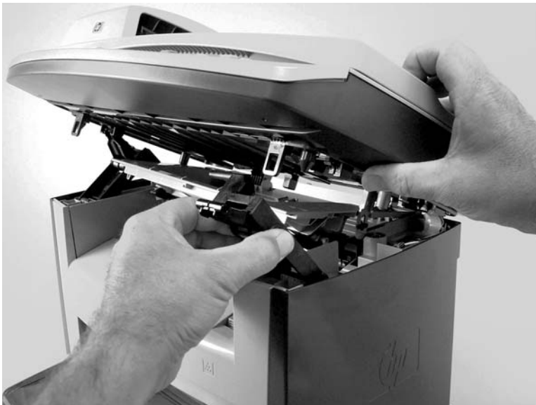
Figure 5-55 Removing the link assemblies and scanner support-frame springs (2 of 4)
