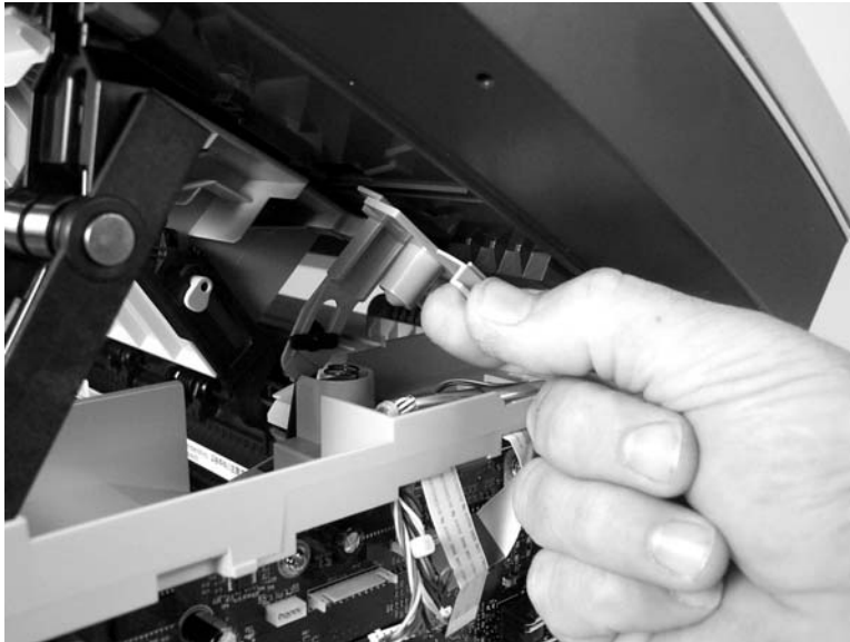
Figure 5-79 Removing the scanner assembly (8 of 13)
