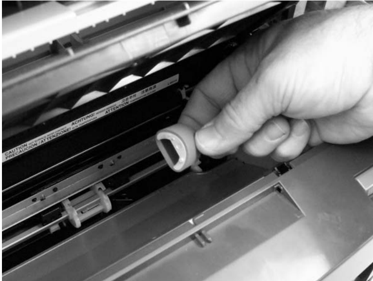
Figure 5-92 Removing the printer pickup roller (3 of 5)
