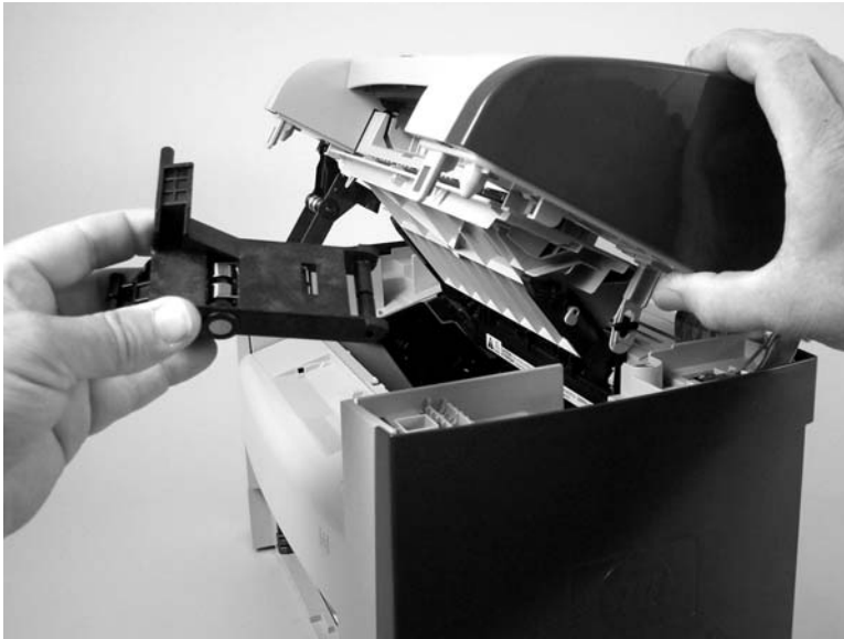
Figure 5-8 Removing the link assemblies and scanner support-frame springs (3 of 4)
