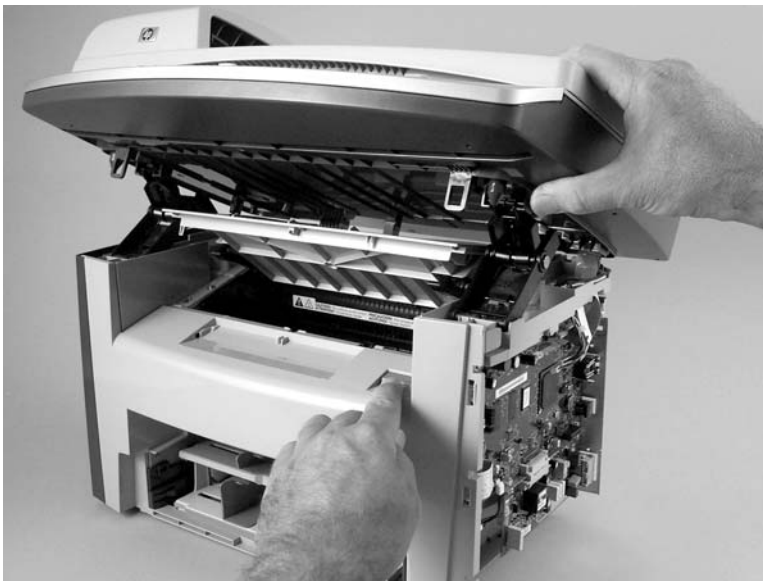
Figure 5-77 Removing the scanner assembly (6 of 13)
