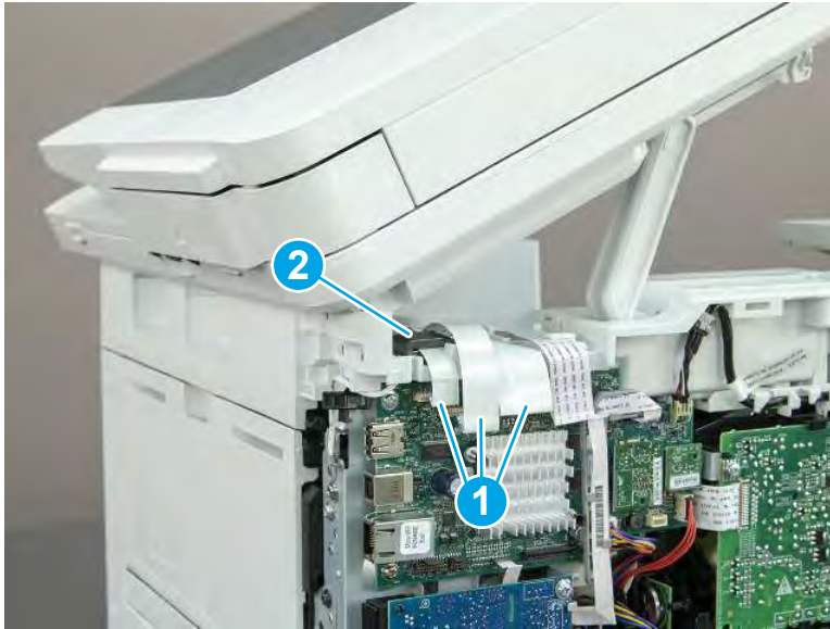
Figure 5-264 Disconnect three FFCs
