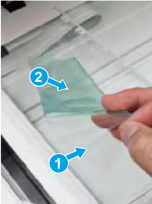
Figure 5-63 Remove the protective film (bottom)
