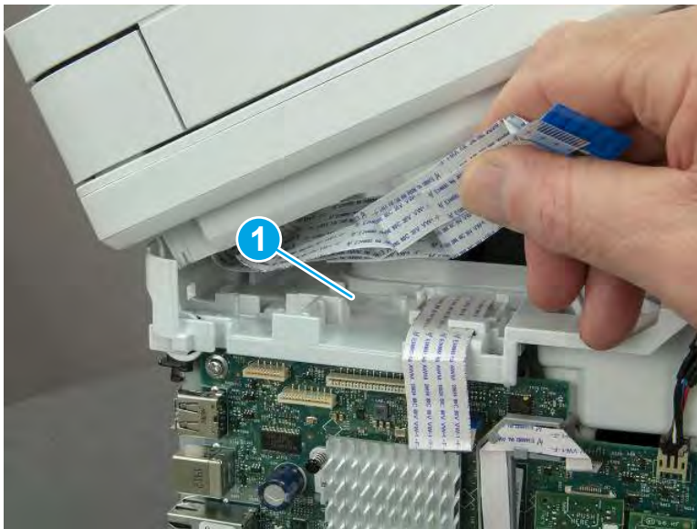
Figure 5-865 Release the tape
