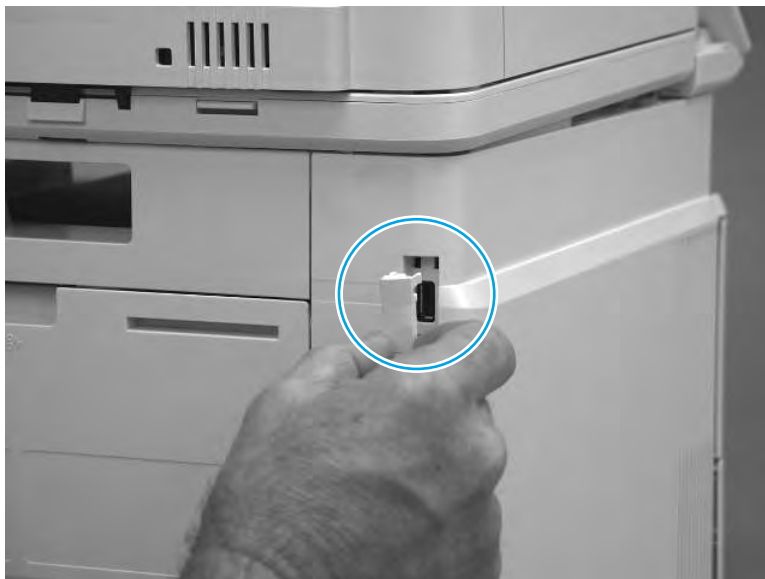
Figure 5-104 Remove the rear USB cover
