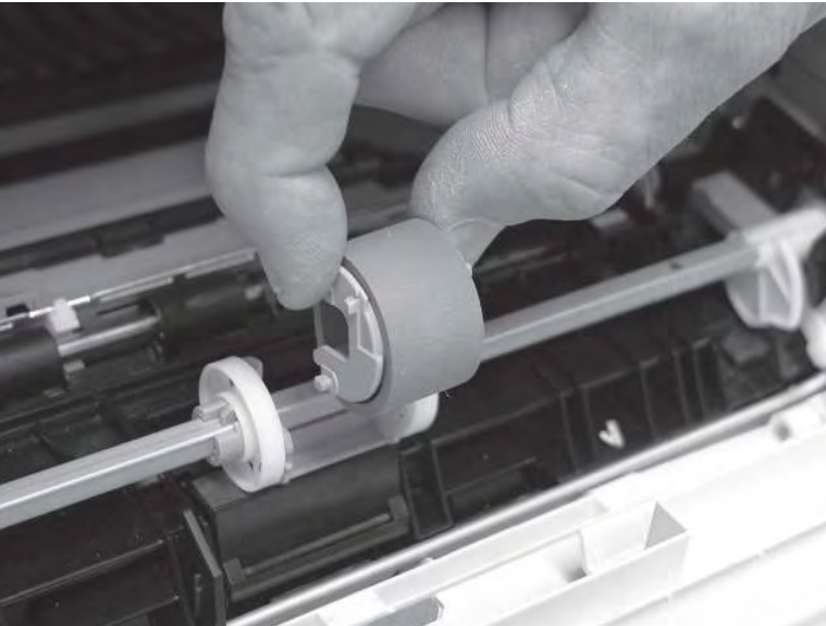
Figure 5-9 Remove the roller
