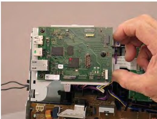
Figure 5-954 Remove the bracket
