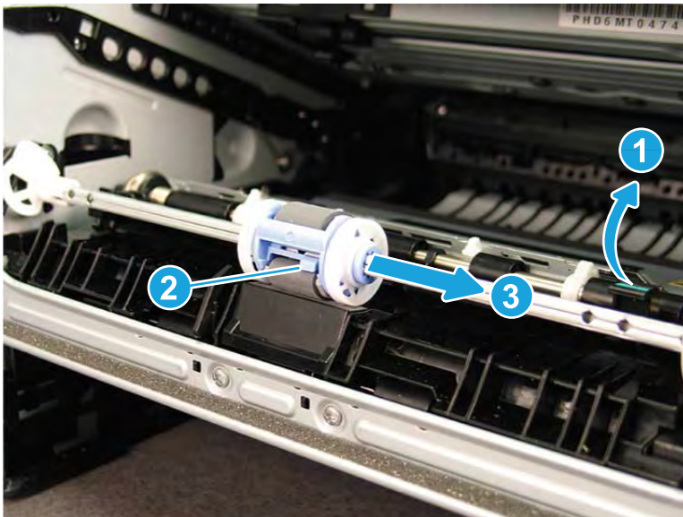
Figure 5-1028 Slide the roller and holder out of the way
