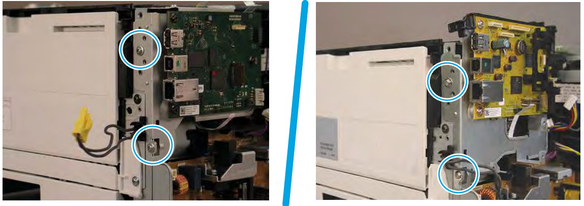
Figure 5-837 Remove two screws
