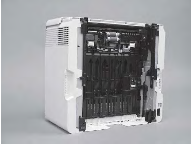
Figure 4-35 Place the printer bottom-side face forward
