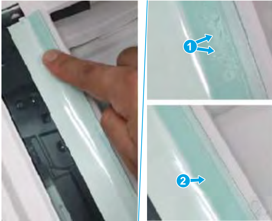
Figure 5-65 Install the Mylar
