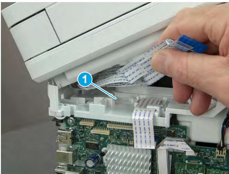
Figure 5-600 Release the tape
