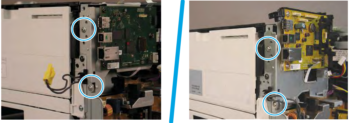
Figure 5-732 Remove two screws
