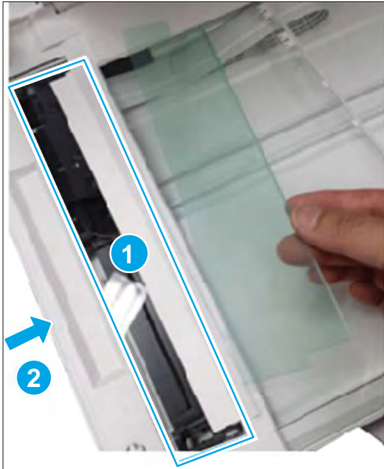
Figure 5-62 Remove adhesive residue
