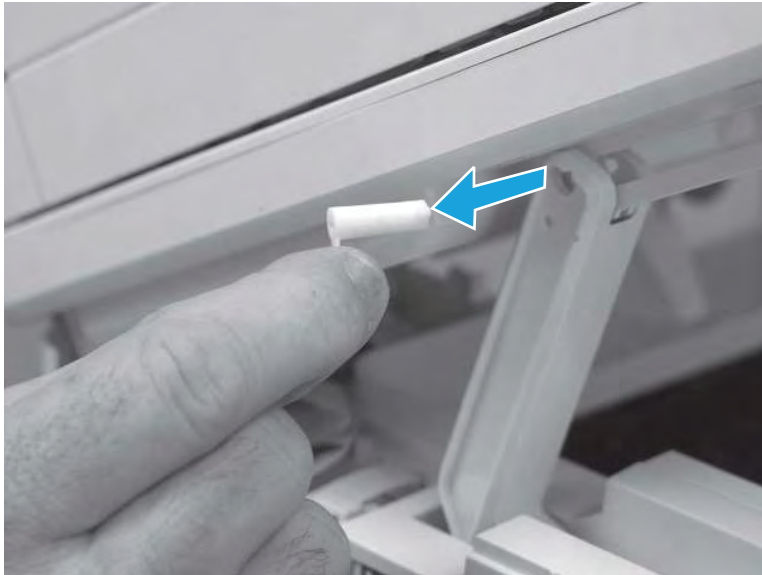
Figure 5-198 Remove the slider pin
