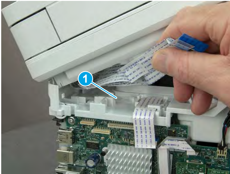
Figure 5-919 Release the tape
