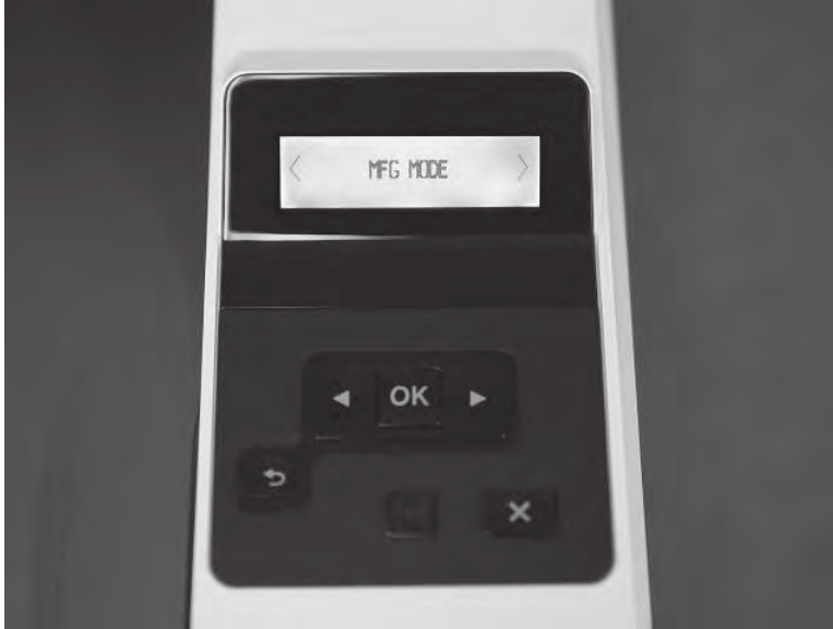
Figure 4-21 2-line control panel
