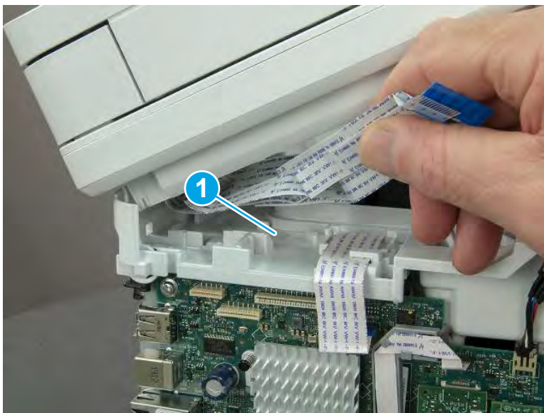
Figure 5-650 Release the tape
