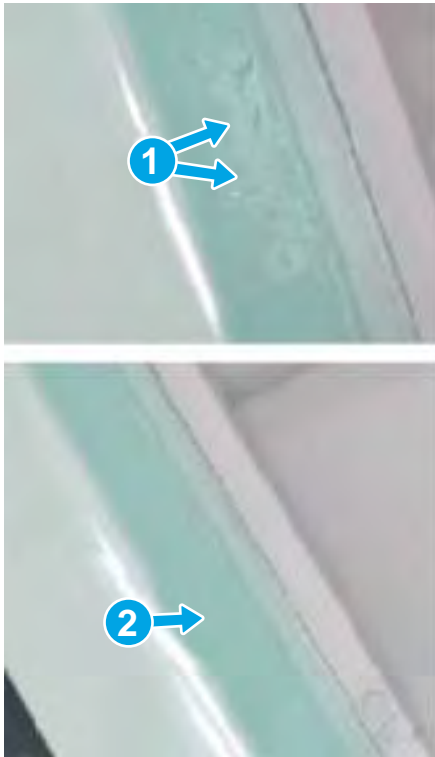
Figure 5-75 Incorrect/correct Mylar installation
