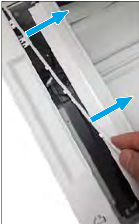
Figure 5-61 Remove the Mylar holder
