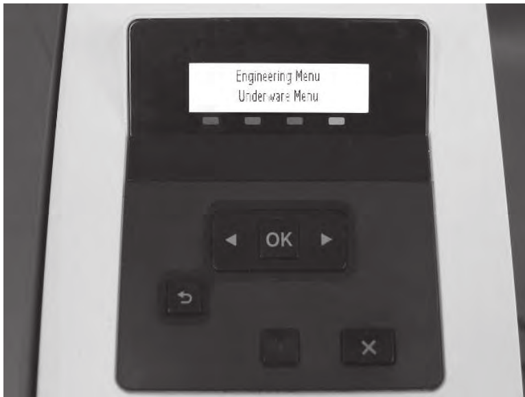
Figure 4-19 2-line control panel
