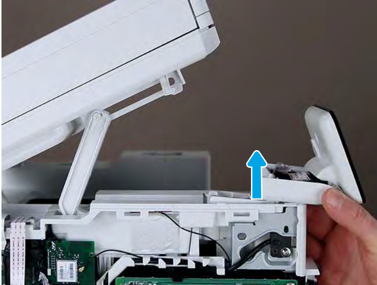
Figure 5-718 Lift up the control-panel assembly
