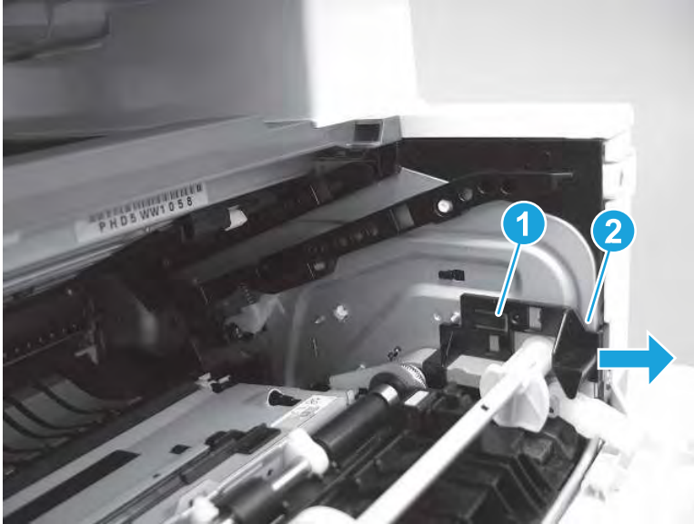
Figure 5-377 Remove the guide
