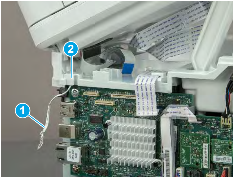
Figure 5-921 Release the ground wire
