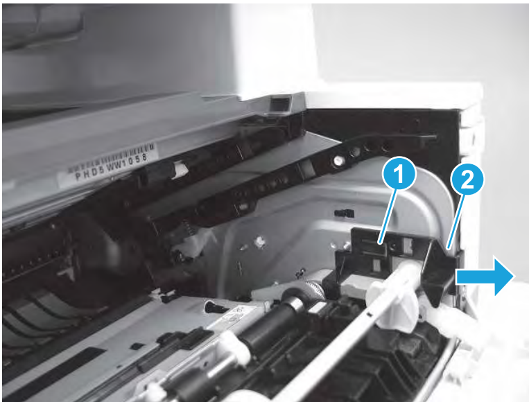
Figure 5-391 Remove the guide
