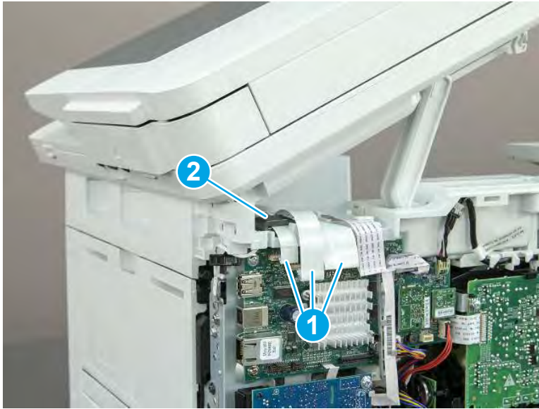
Figure 5-864 Disconnect three FFCs
