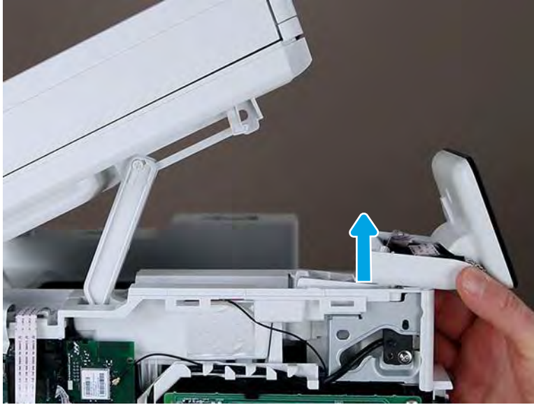
Figure 5-341 Lift up the control-panel assembly
