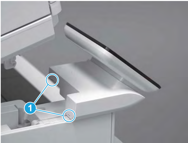
Figure 5-875 Release two tabs
