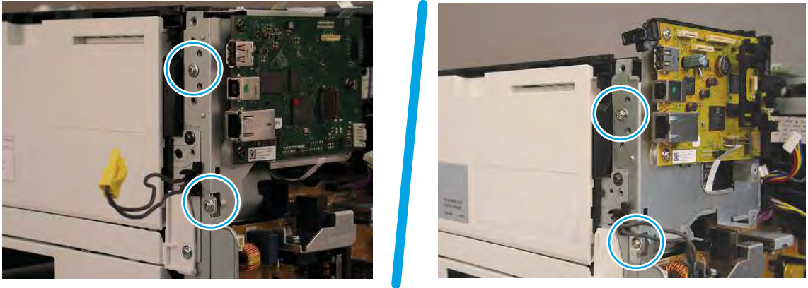
Figure 5-894 Remove two screws
