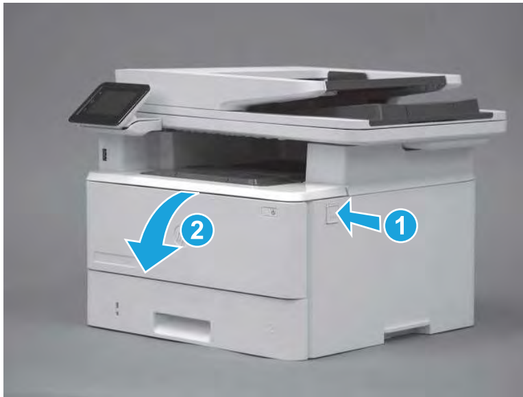
Figure 5-7 Open the toner-cartridge door
