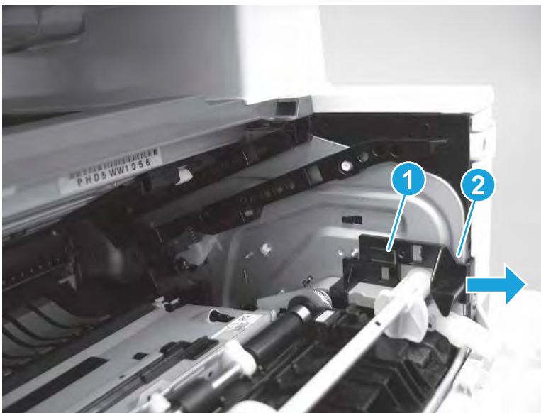
Figure 5-148 Remove the guide
