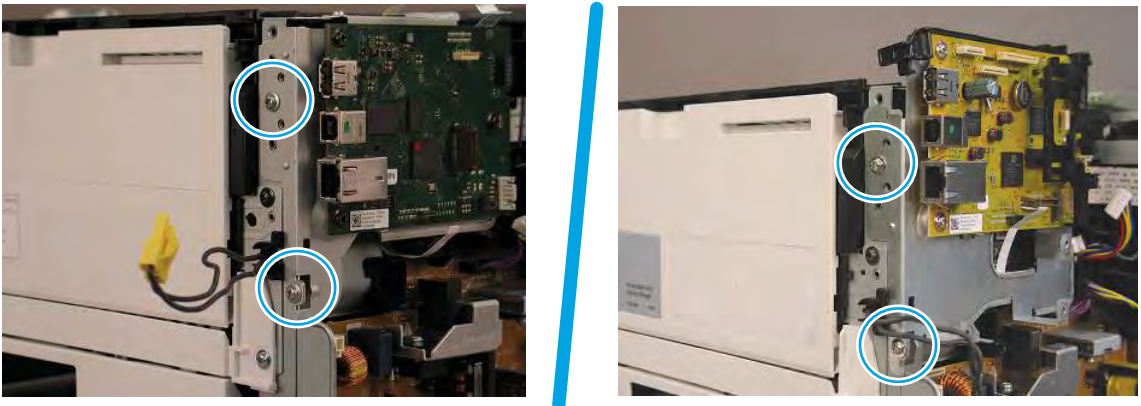
Figure 5-951 Remove two screws
