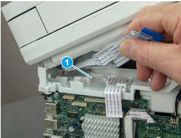
Figure 5-808 Release the tape
