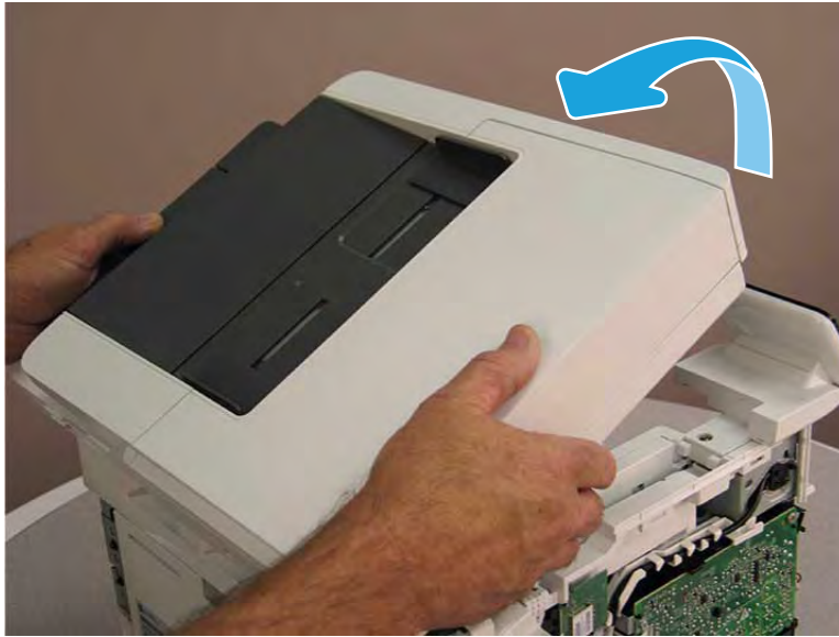
Figure 5-605 Rotate the ISA towards the rear of the printer
