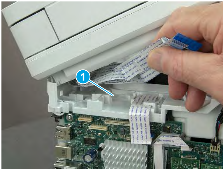
Figure 5-94 Release the tape
