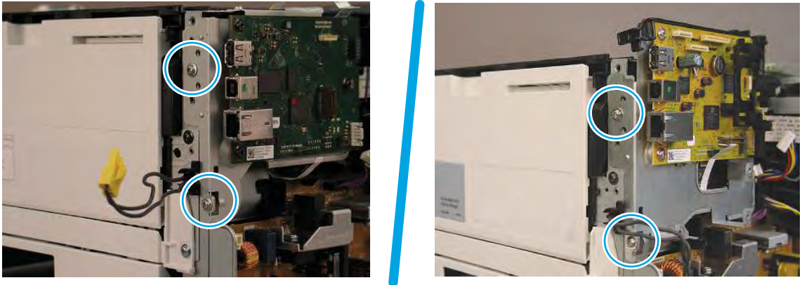
Figure 5-784 Remove two screws
