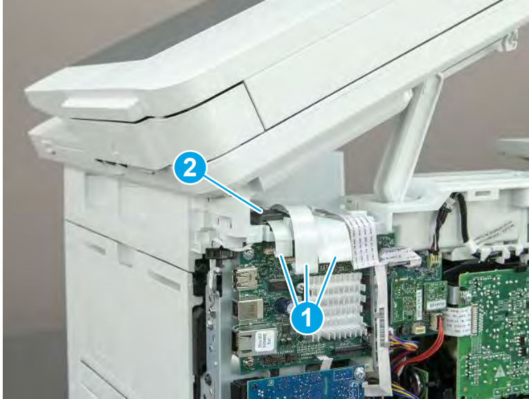
Figure 5-918 Disconnect three FFCs
