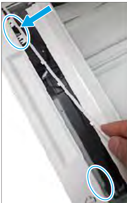
Figure 5-70 Reinstall the Mylar holder
