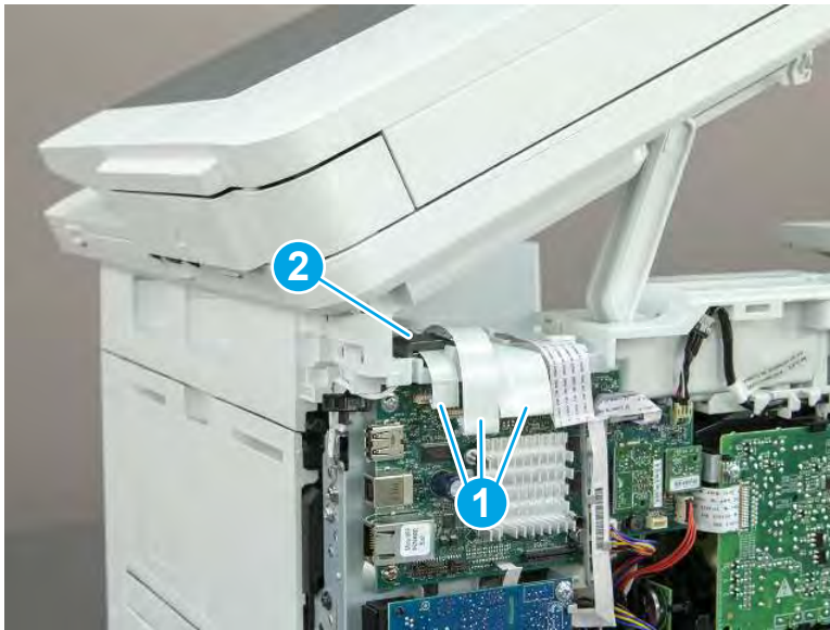
Figure 5-649 Disconnect three FFCs
