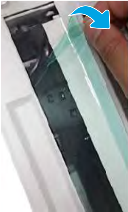
Figure 5-69 Remove the protective film (top)
