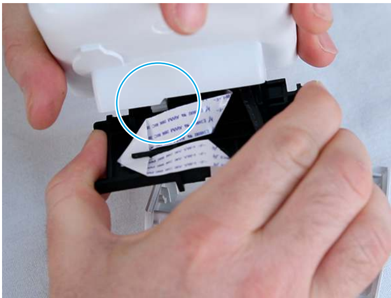
Figure 5-1009 Disengage the ratchet wheel
