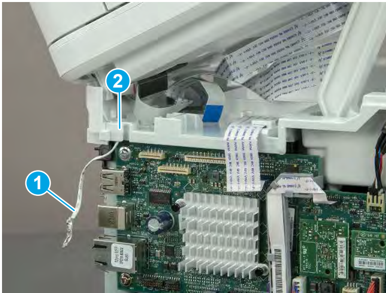
Figure 5-602 Release the ground wire
