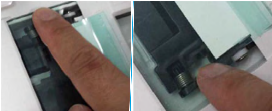
Figure 5-66 Check the install of the Mylar
