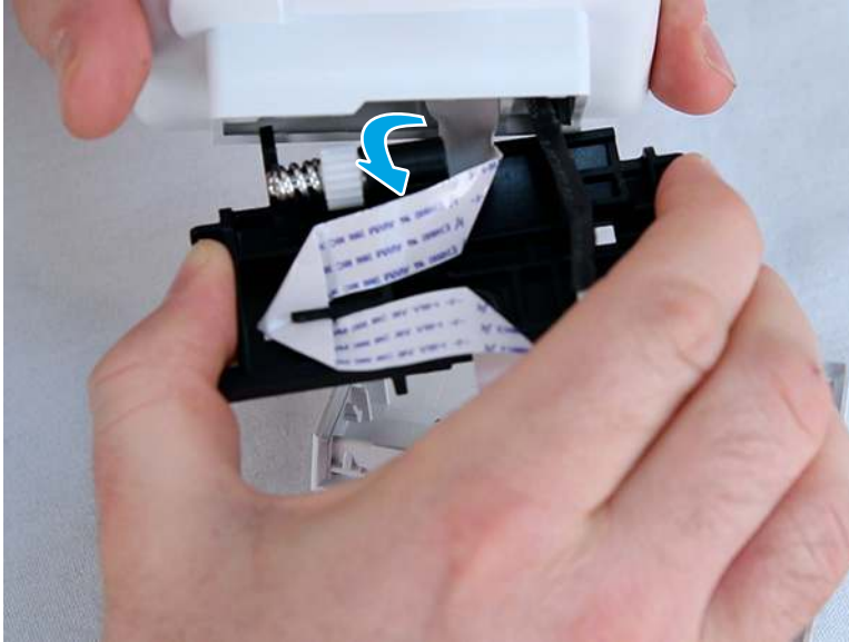
Figure 5-1010 Separate the control panel and mount chassis
