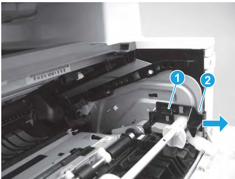
Figure 5-431 Remove the guide
