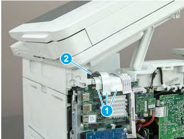
Figure 5-489 Disconnect three FFCs
