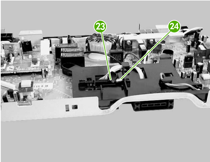
Figure 5-147 Removing the high-voltage power supply (16 of 17)
