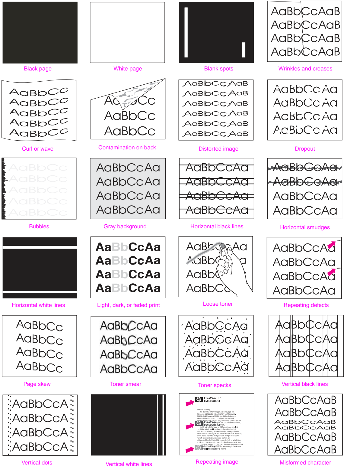
Figure 129. Image defect examples
