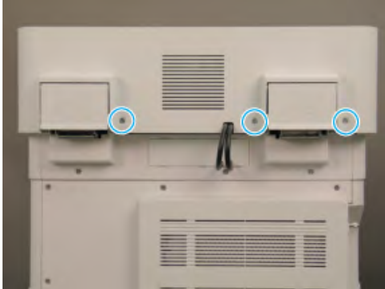
Figure 2-344 Remove the document feeder back cover bottom screws
