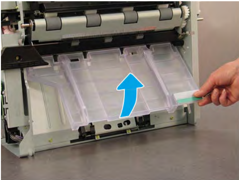
Figure 5-1502 Raise the jam access cover
