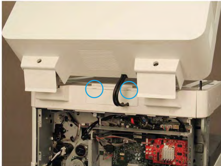
Figure 3-57 Remove ADF connector cover
