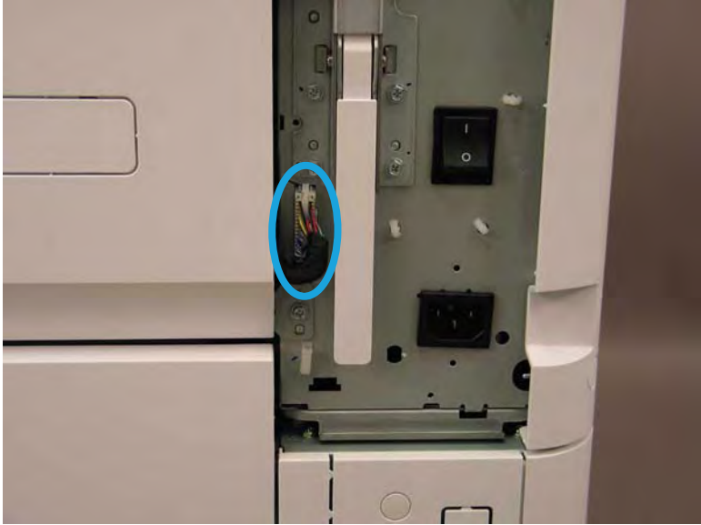
Figure 2-186 Disconnect right door connector
