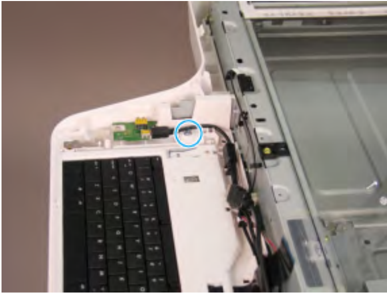
Figure 2-47 Remove USB interconnect cable
