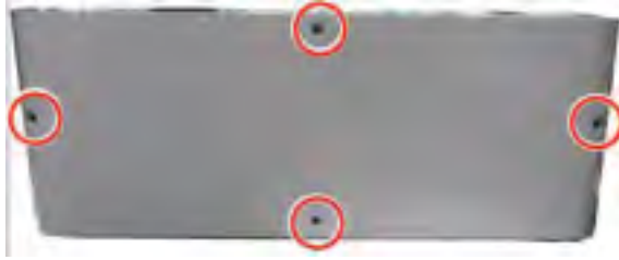
Figure 2-460 Remove the DCF rear cover
