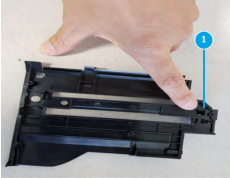
Figure 5-757 Remove rear tamper home sensor
