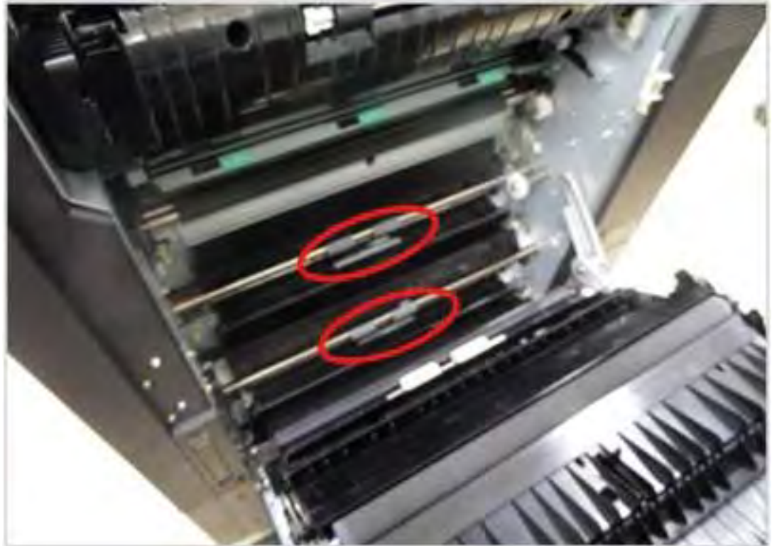
Figure 3-72 Check feed rollers
