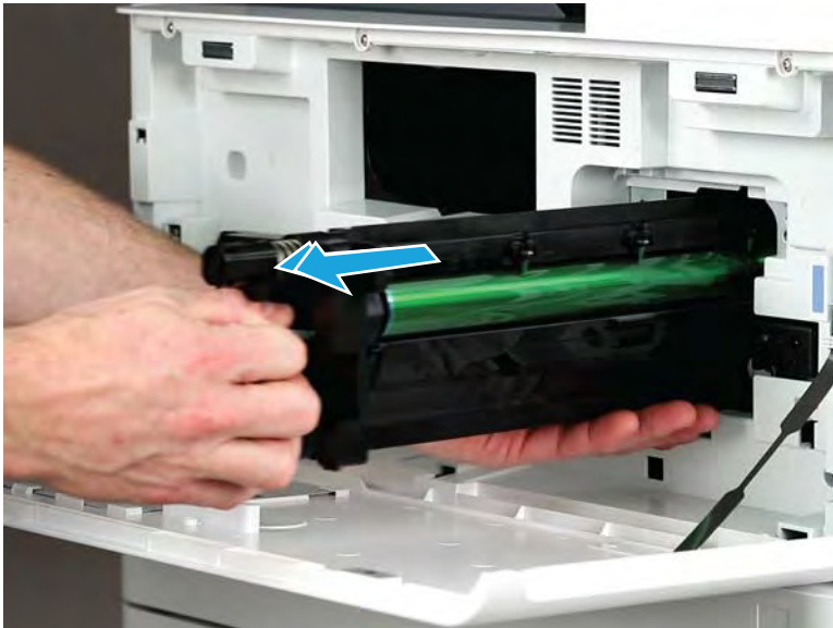
Figure 2-192 Remove drum unit
