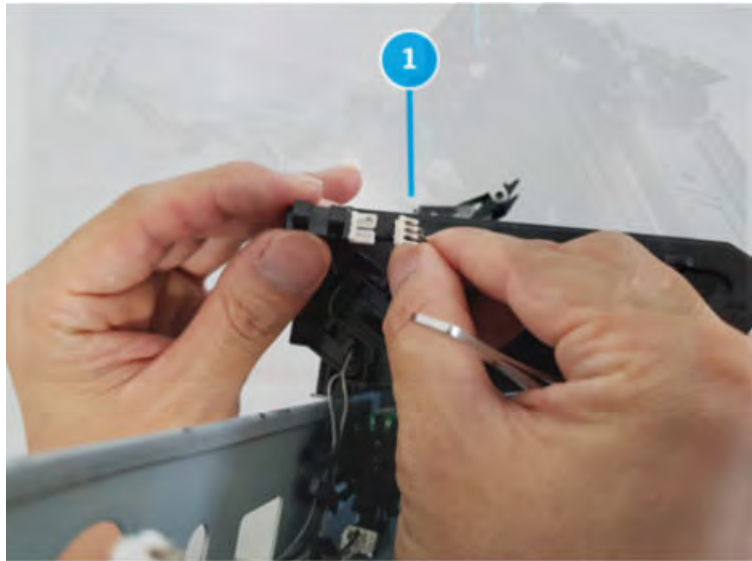
Figure 5-1119 Disconnect the connector from ejector2 home sensor
