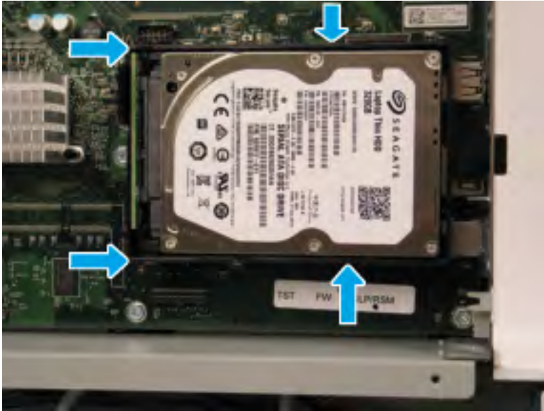
Figure 2-138 Remove the hard-disk drive (HDD)
