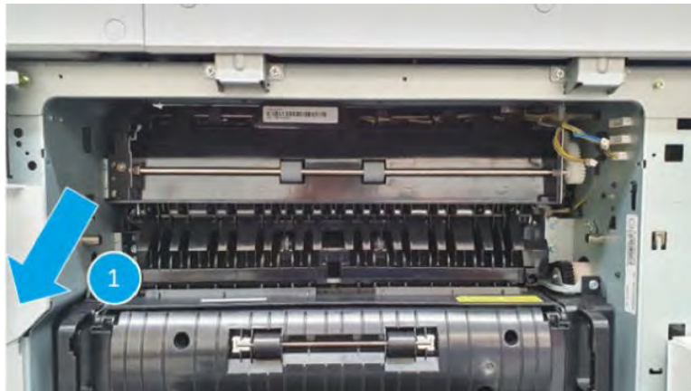
Figure 2-446 Remove the second exit unit
