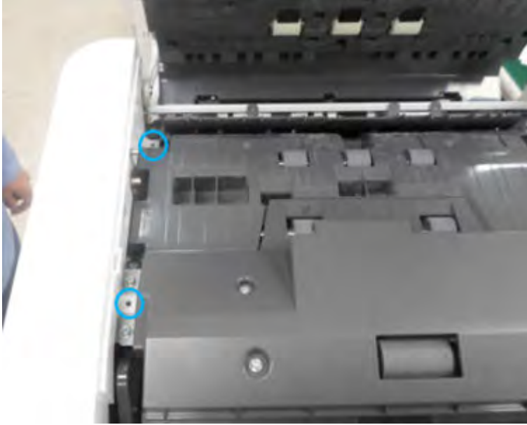
Figure 2-349 Remove the document feeder front cover top screws
