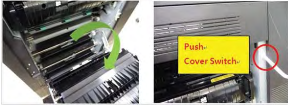
Figure 3-71 Open right door and push cover switch
