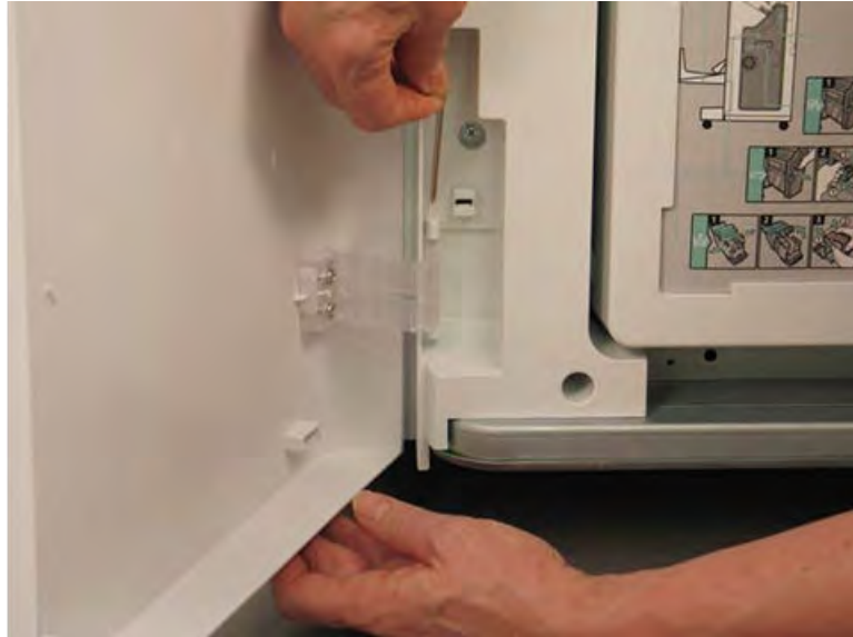
Figure 5-830 Remove the lower hinge pin
