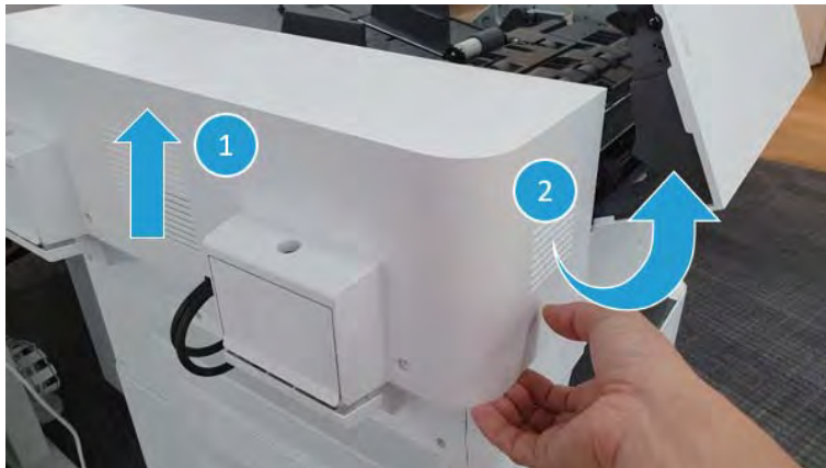
Figure 2-294 Release the top back cover.
