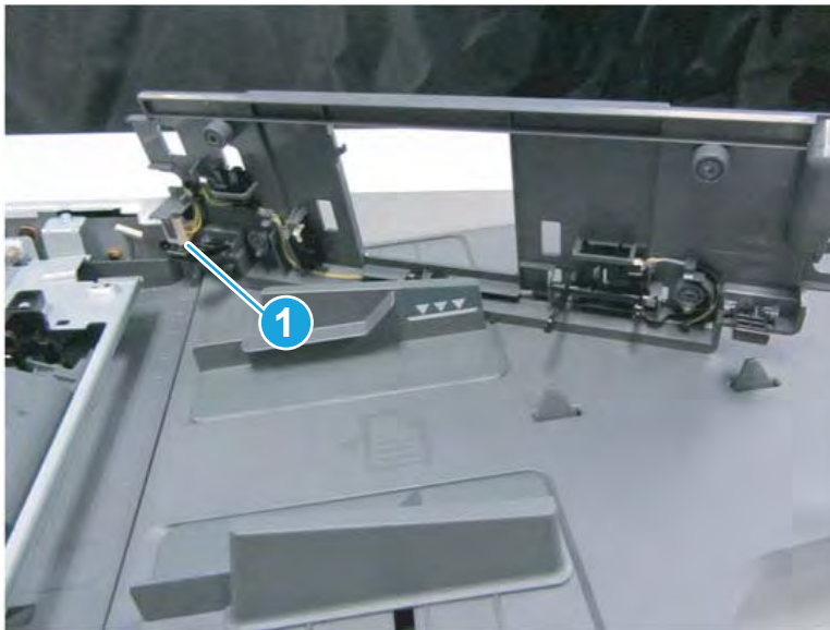
Figure 2-326 Turn the cover over and disconnect connector
