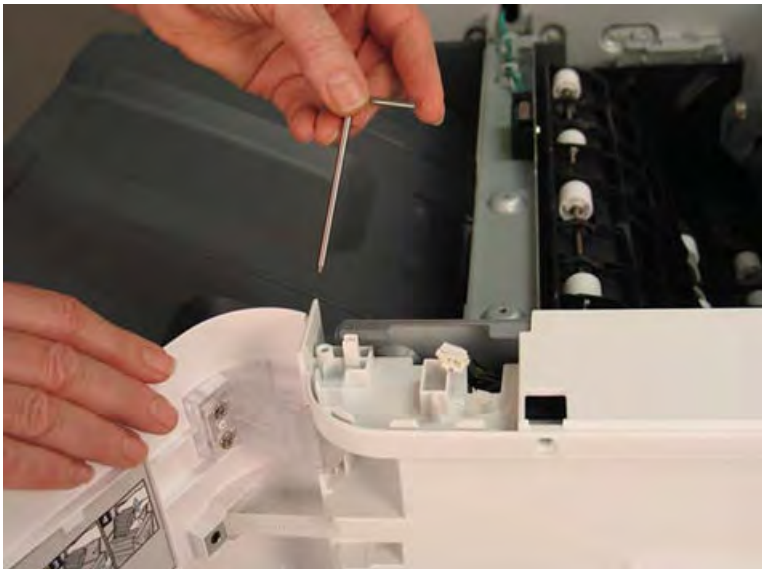
Figure 5-1080 Remove the top hinge pin
