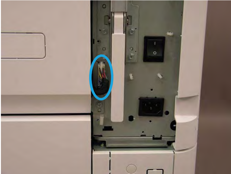
Figure 2-63 Disconnect right door connector
