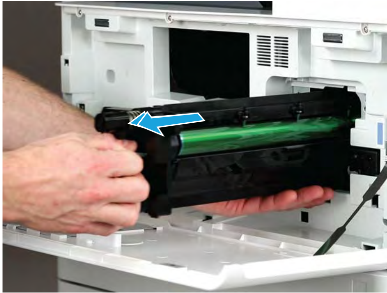
Figure 2-110 Remove drum unit
