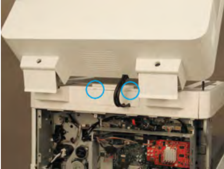
Figure 2-39 Remove document feeder connector cover
