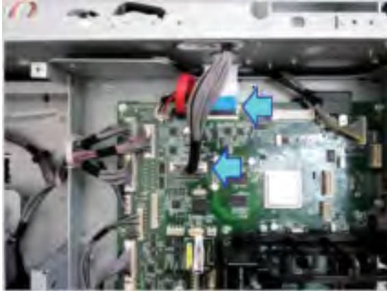
Figure 2-53 Disconnect scan cables
