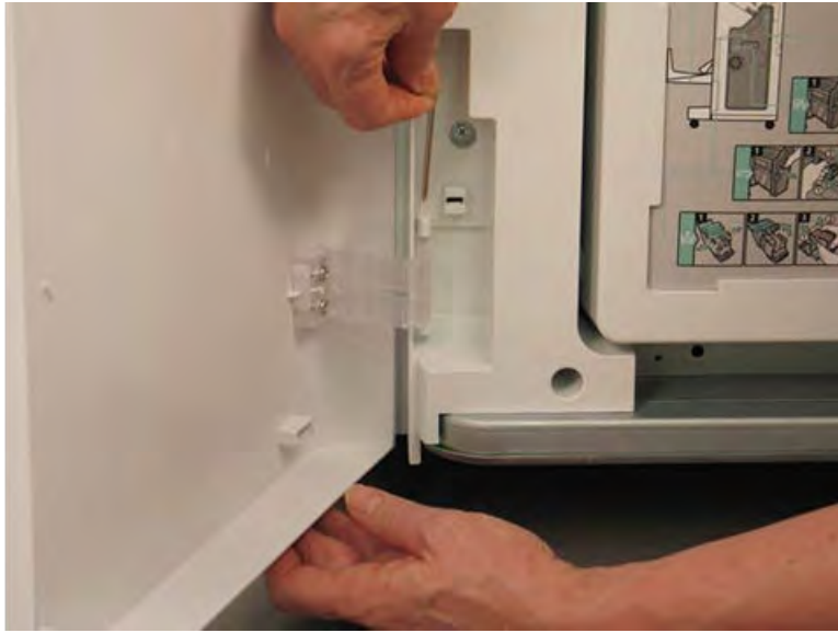
Figure 5-211 Remove the lower hinge pin
