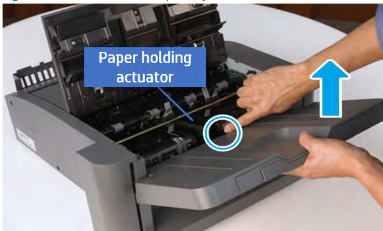
Figure 7-352 Remove the output tray.
