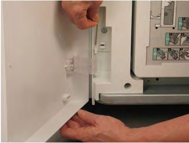
Figure 5-1247 Remove the lower hinge pin
