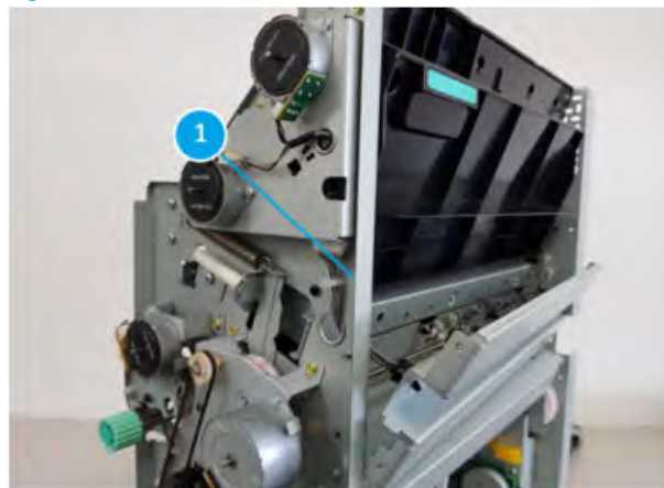
Figure 5-1653 Disconnect one connector
