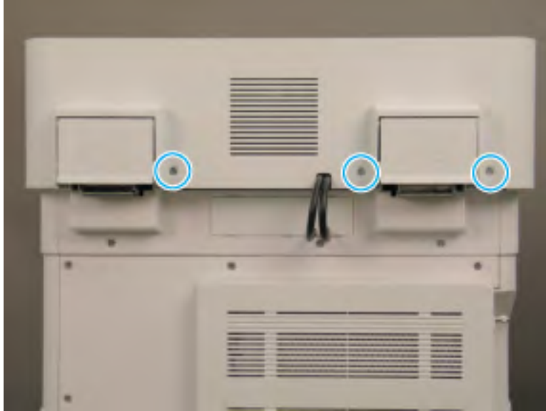
Figure 2-409 Remove the document feeder back cover bottom screws
