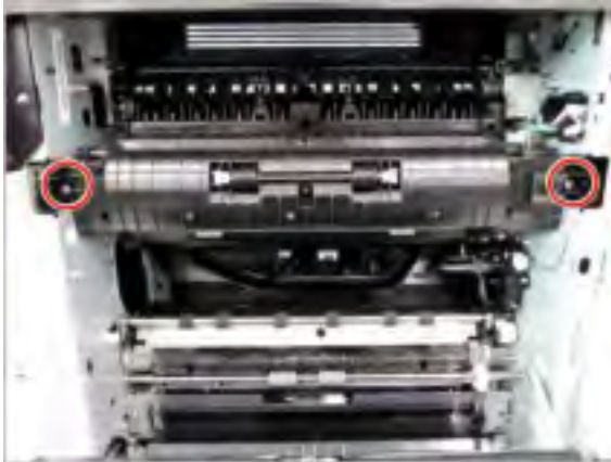
Figure 2-107 Remove two fuser unit screws
