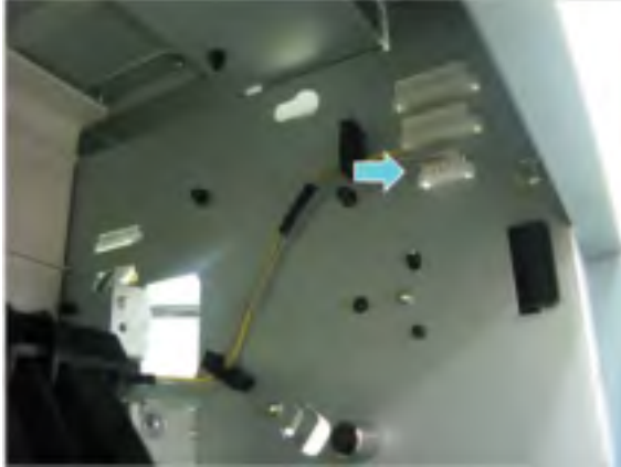
Figure 2-70 Disconnect exit unit connector and cable restraints
