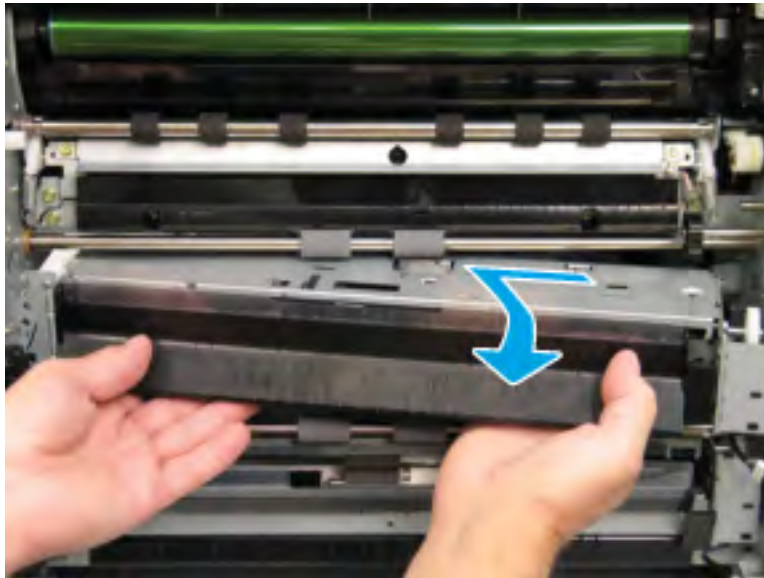
Figure 2-203 Remove the pickup assembly
