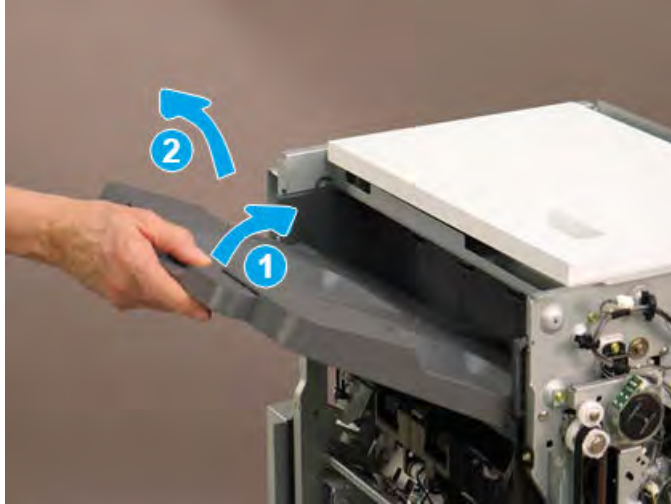
Figure 5-358 Remove the top output tray
