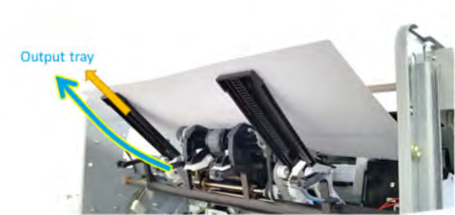
Figure 7-25 Inner finisher system - paper support unit operation
