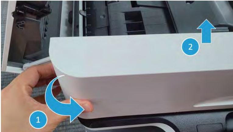
Figure 2-407 Remove the document feeder front cover
