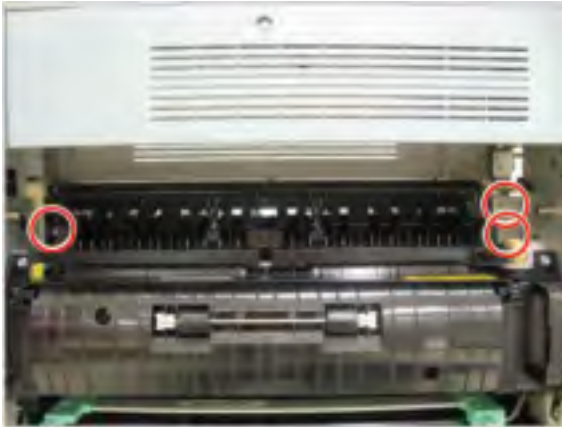
Figure 2-71 Remove screws and exit unit
