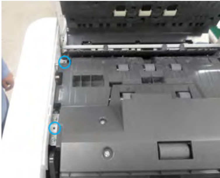
Figure 2-289 Remove the document feeder front cover top screws
