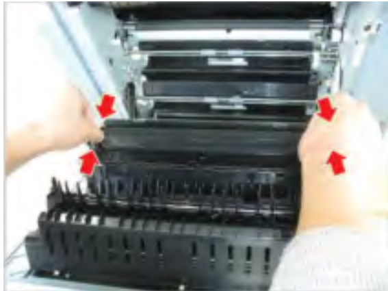
Figure 2-225 Remove transfer roller
