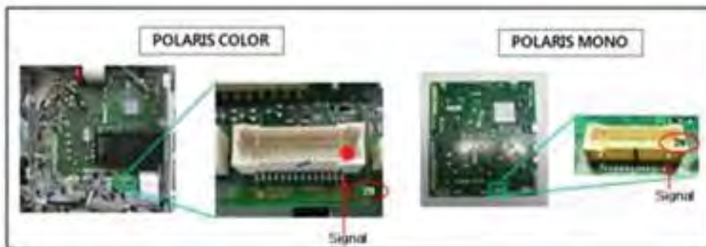
Figure 3-76 Check 24V on/off signal pin
