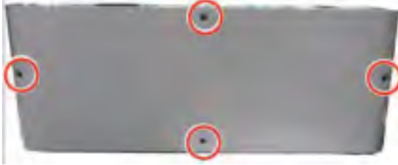
Figure 2-454 Remove the DCF rear cover
