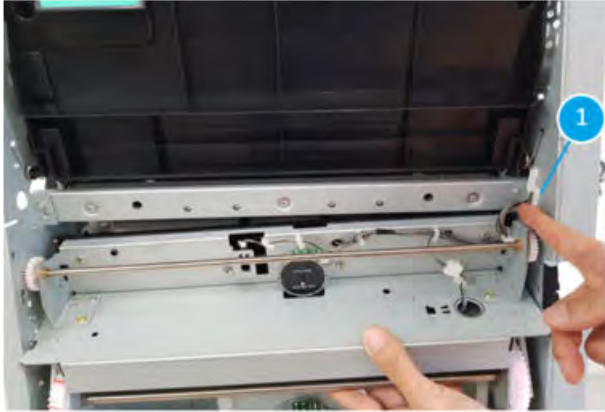
Figure 5-1766 Disconnect one connector
