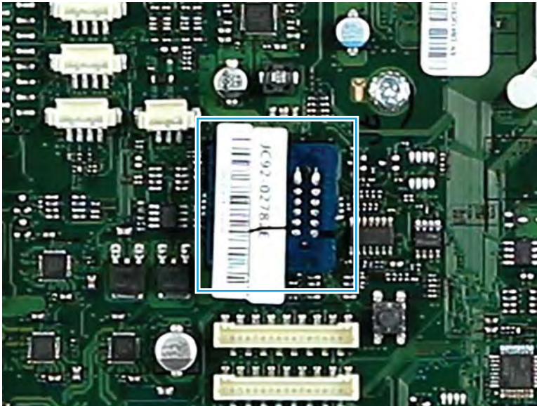
Figure 2-220 MSOK installation orientation
