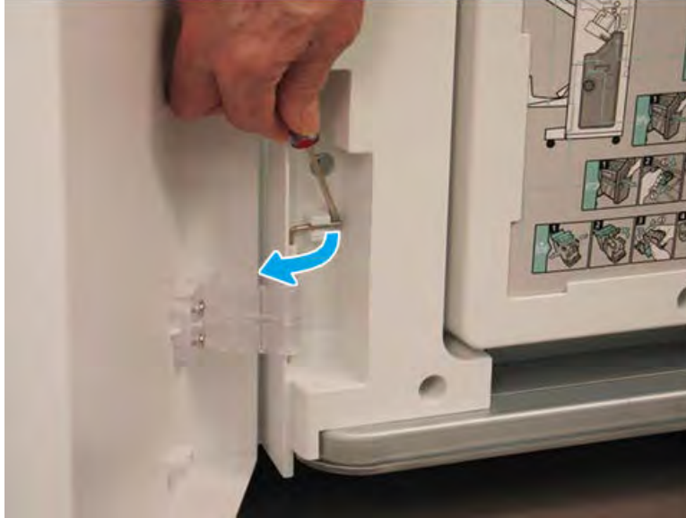
Figure 5-522 Release the lower hinge pin
