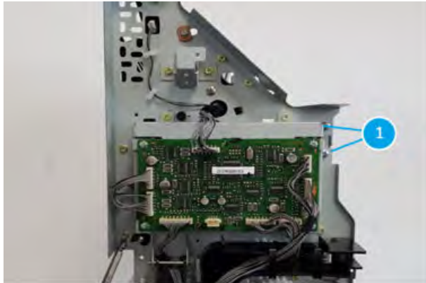
Figure 5-1688 Remove two screws
