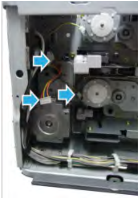
Figure 2-457 Disconnect two connectors and open one retainer
