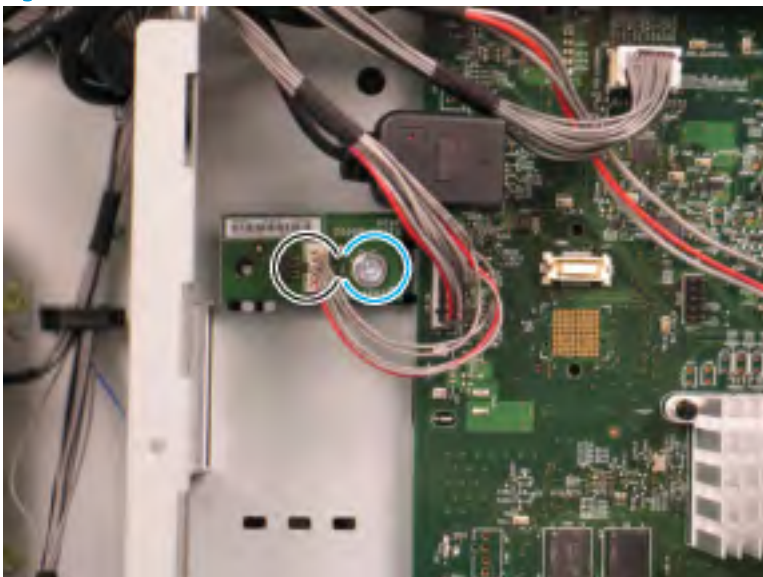
Figure 2-139 Remove the IOD
