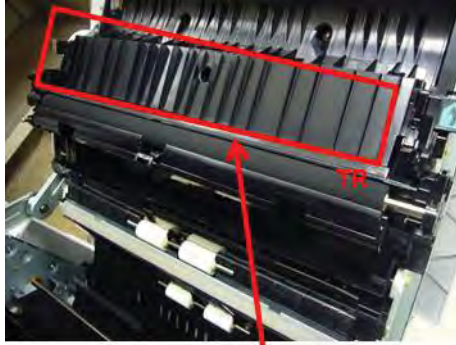
Figure 3-54 Paper guide rib contamination
