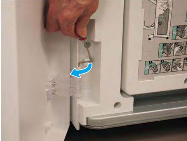
Figure 5-1035 Release the lower hinge pin
