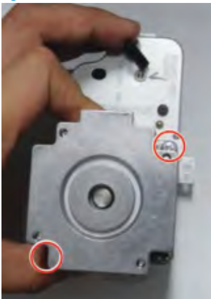
Figure 2-459 Remove the feed motor
