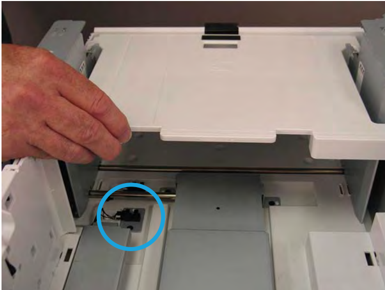
Figure 2-567 Remove the HCI photo interrupter and sensor bracket
