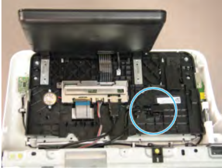
Figure 2-151 Remove the USB interconnect cable
