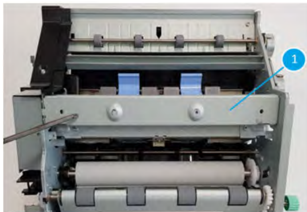
Figure 5-1689 Remove the metal frame
