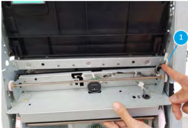
Figure 5-1587 Disconnect one connector
