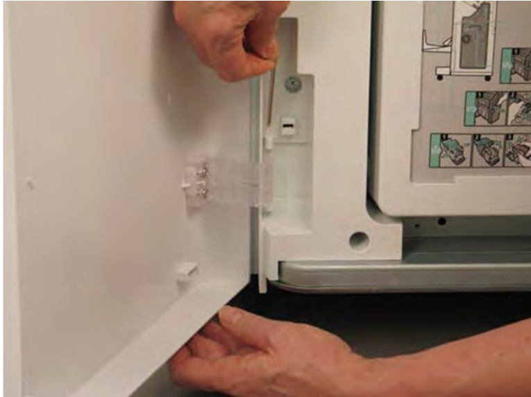
Figure 5-811 Remove the lower hinge pin
