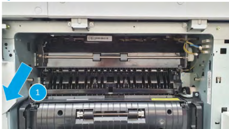
Figure 2-441 Remove the second exit unit
