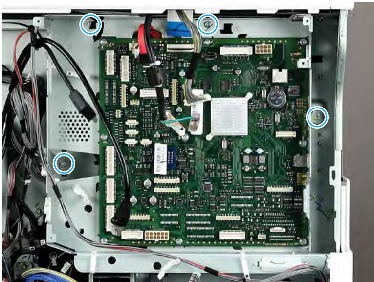
Figure 2-222 Remove the main board cage screws
