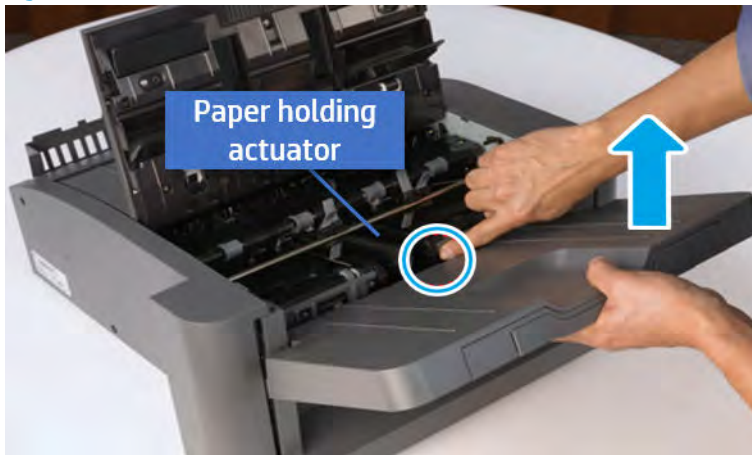
Figure 7-707 Remove the output tray.
