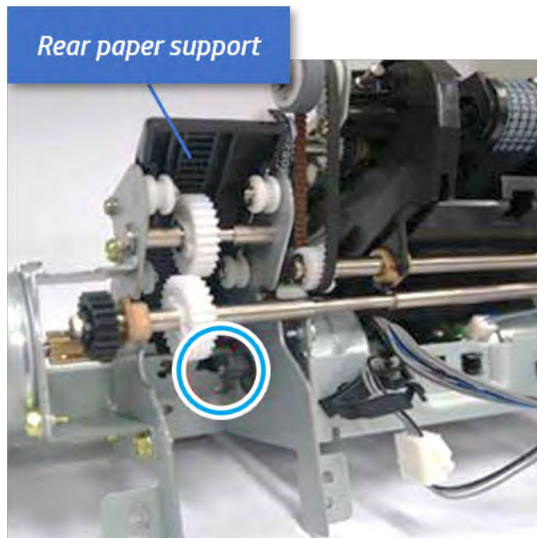
Figure 7-235 Remove the rear paper support
