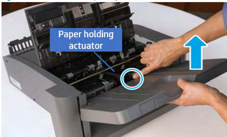
Figure 7-73 Remove the output tray.
