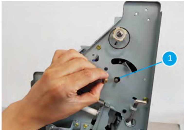
Figure 5-1547 Remove one e-clip on top of the bush then remove the bush
