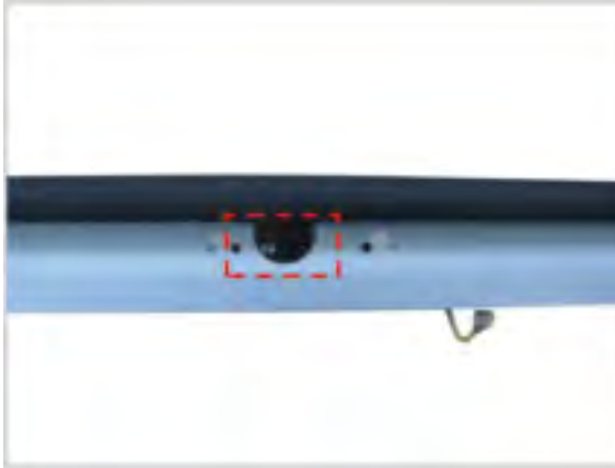
Figure 2-195 Remove registration sensor
