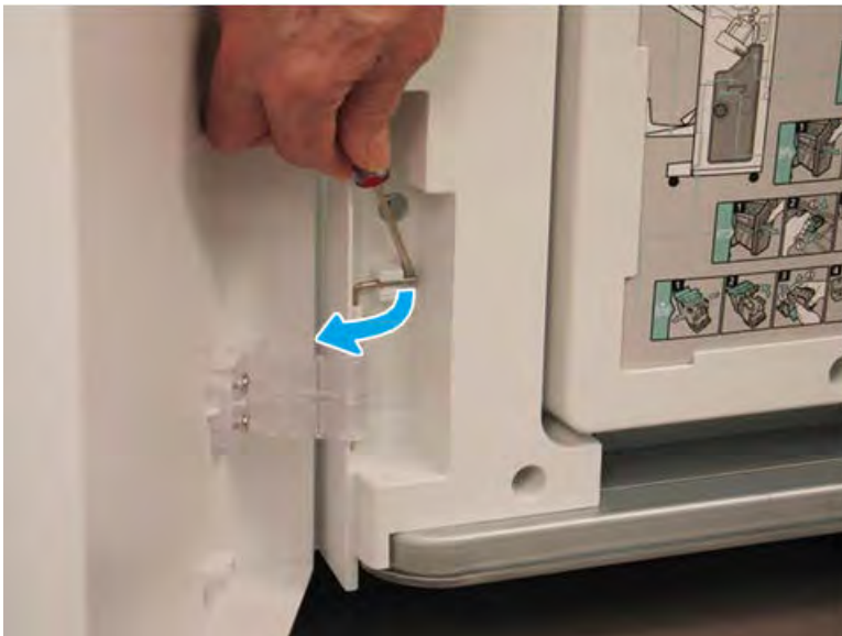
Figure 5-1271 Release the lower hinge pin
