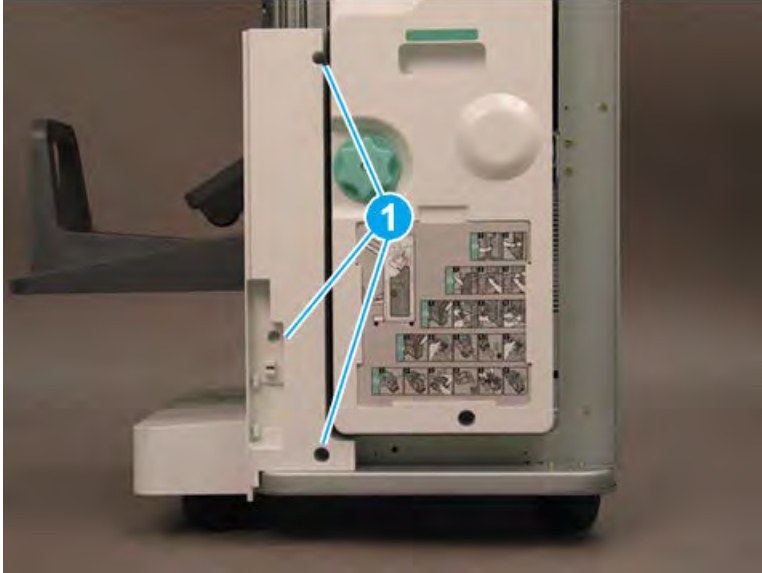
Figure 5-199 Remove the front lower cover
