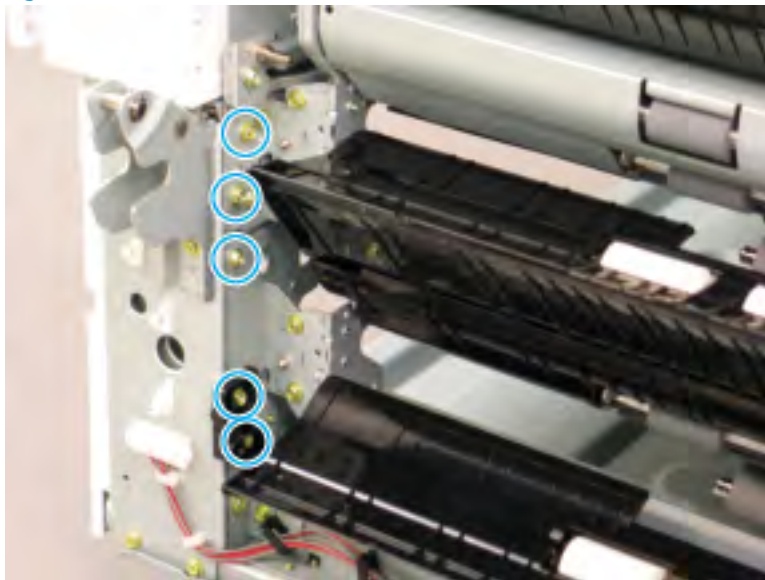
Figure 2-465 Remove five screws and two brackets
