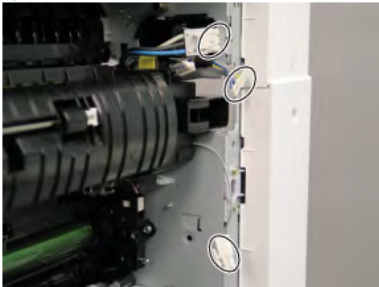
Figure 2-106 Disconnect the connectors
