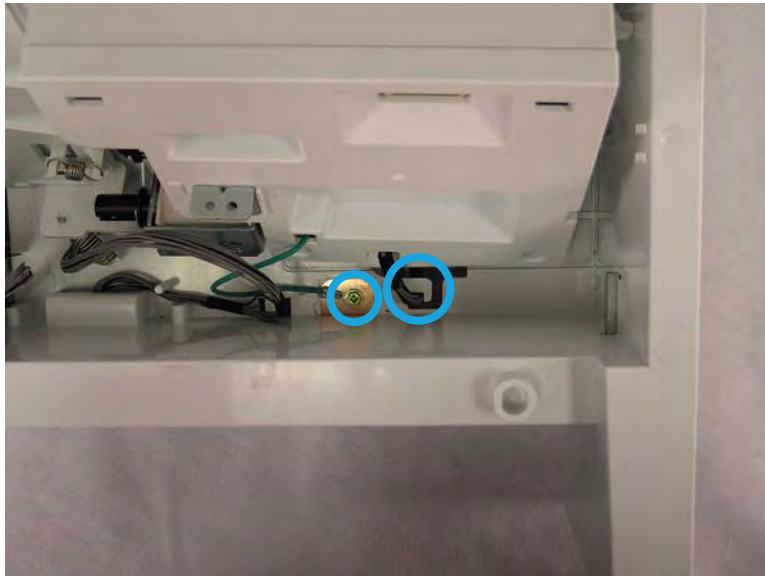
Figure 2-559 Remove one screw and release the wire harness
