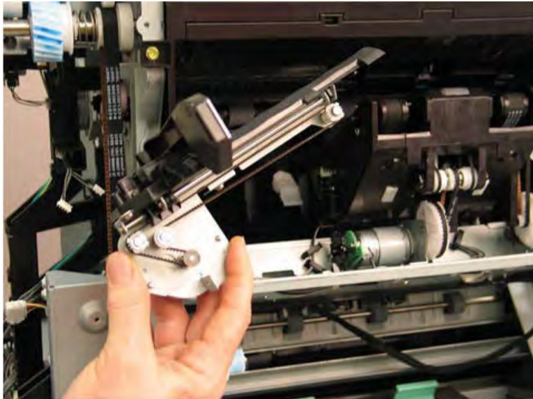
Figure 5-801 Remove the rear tamper
