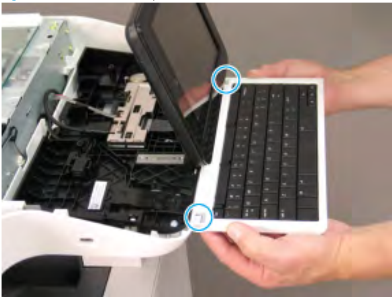
Figure 2-48 Remove the keyboard
