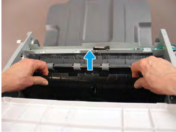
Figure 5-354 Remove the top lower feed assembly
