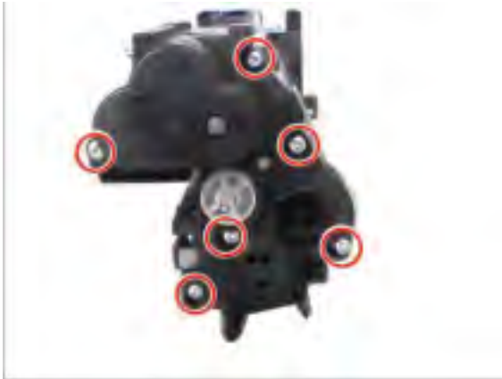
Figure 2-126 Remove rear cover screws
