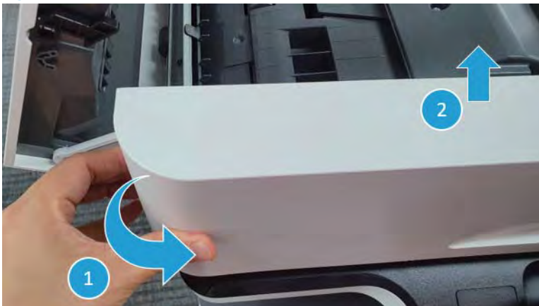
Figure 2-291 Remove the document feeder front cover
