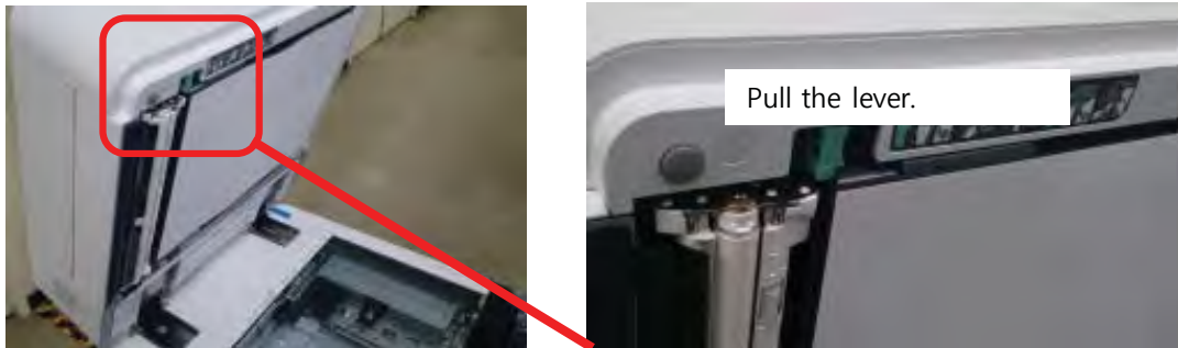
Figure 1-64 Flow document feeder dual sensor cleaning method (2 of 2)
