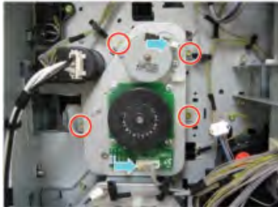
Figure 2-182 Remove screws and fuser/exit drive unit
