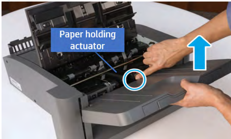
Figure 7-324 Remove the output tray.
