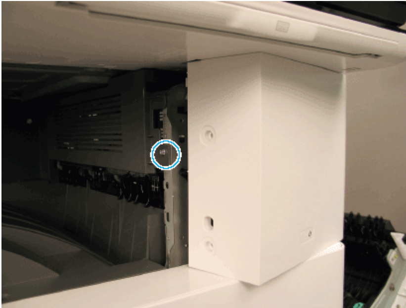
Figure 2-146 Remove the cover exit right
