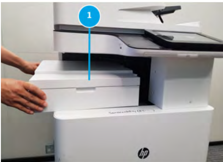
Figure 5-144 Pull out the bridge unit
