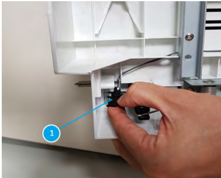
Figure 5-154 Remove the bridge door sensor
