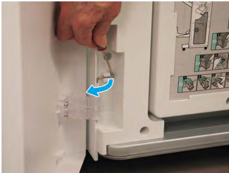
Figure 5-210 Release the lower hinge pin
