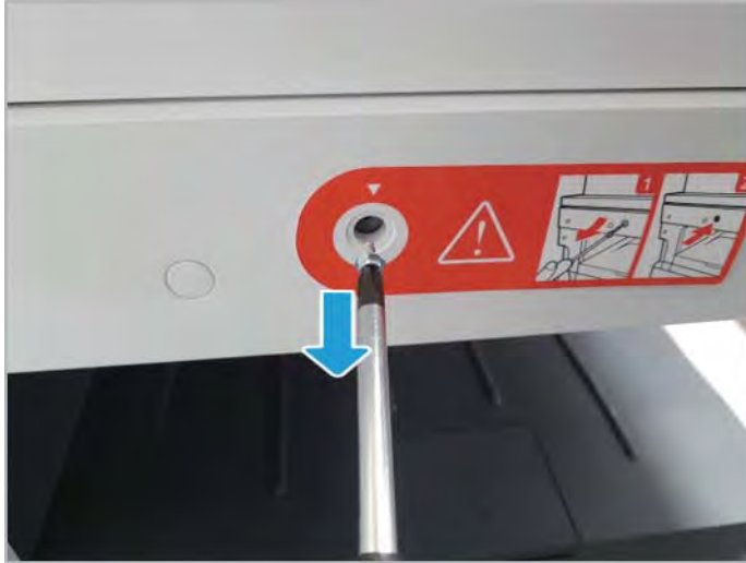
Figure 1-44 Remove scan locking screw
