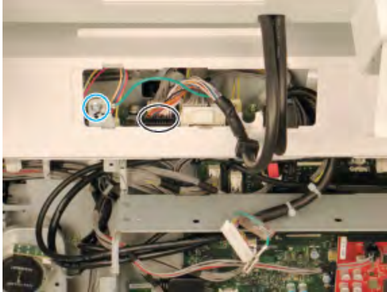
Figure 2-41 Disconnect document feeder harness
