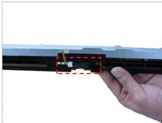
Figure 2-69 Remove feed sensor 2
