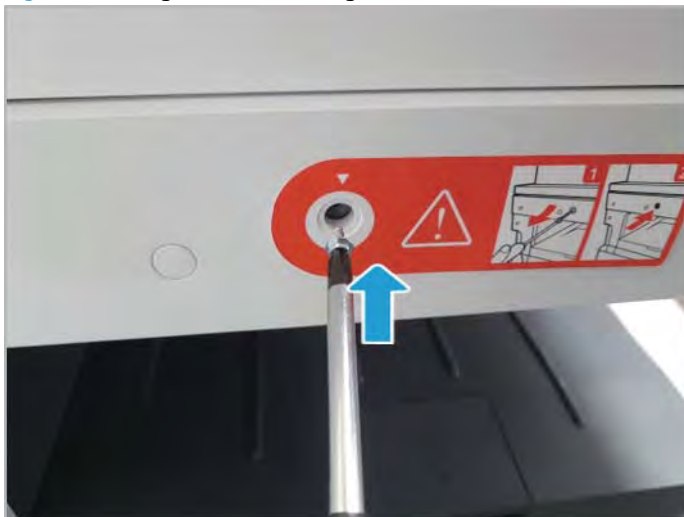
Figure 1-45 Tighten scan locking screw
