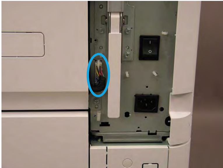
Figure 2-56 Disconnect right door connector
