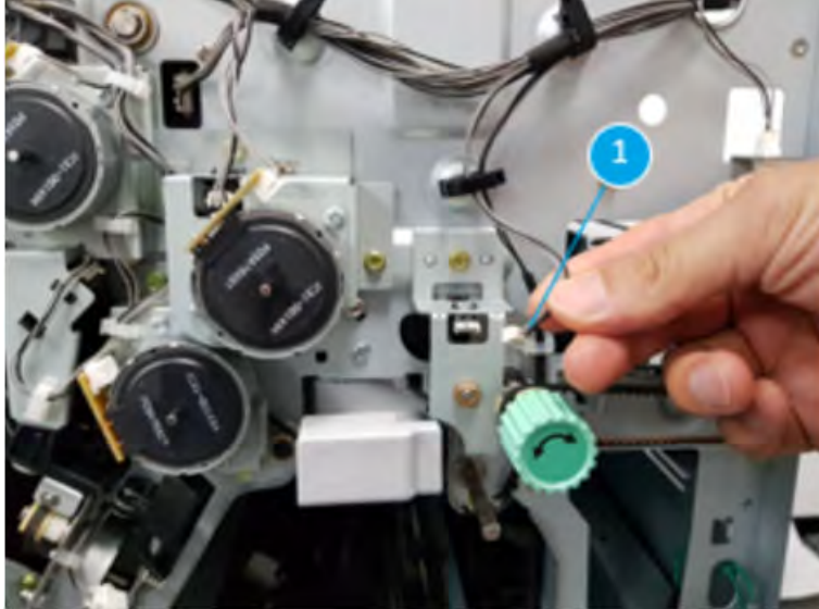
Figure 5-307 Disconnect one connector
