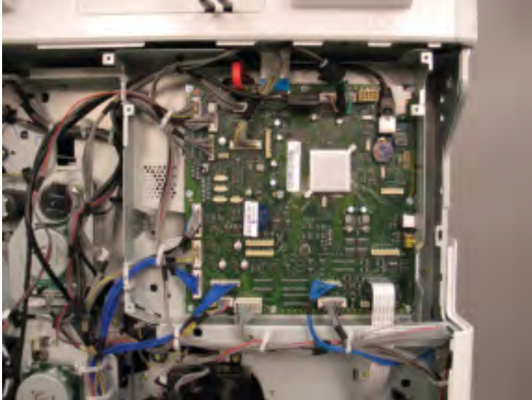
Figure 2-90 Remove the main board connectors and screws
