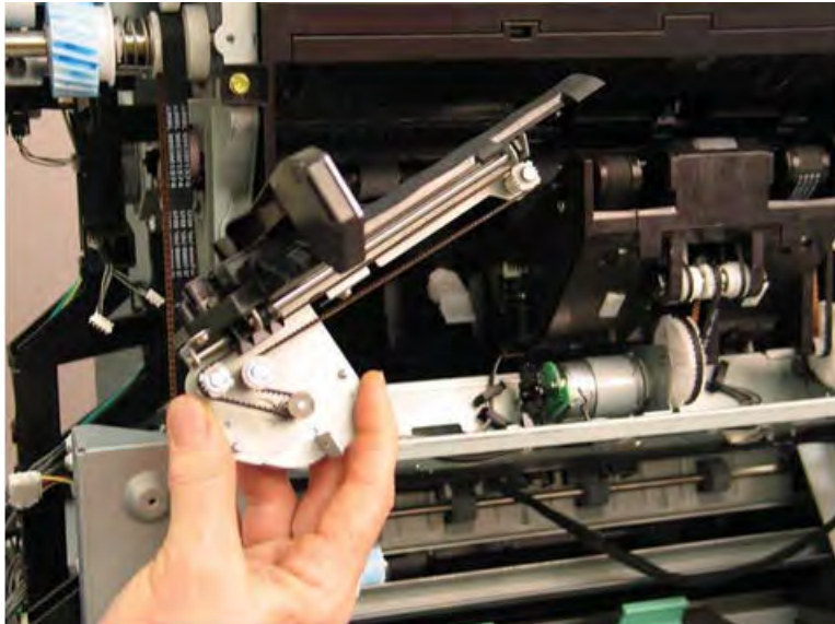
Figure 5-710 Remove the rear tamper
