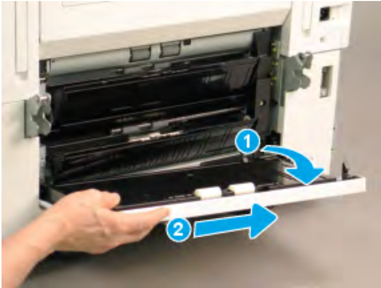
Figure 2-453 Remove the DCF right door
