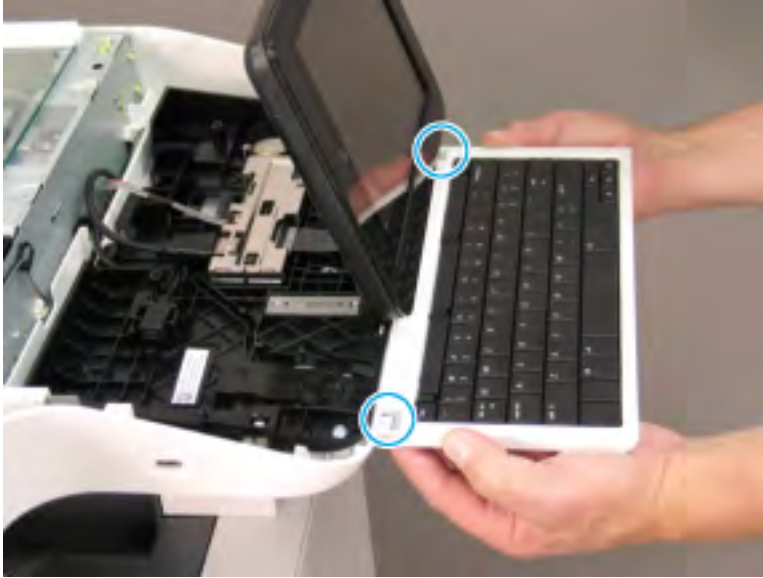
Figure 2-154 Remove the control-panel keyboard
