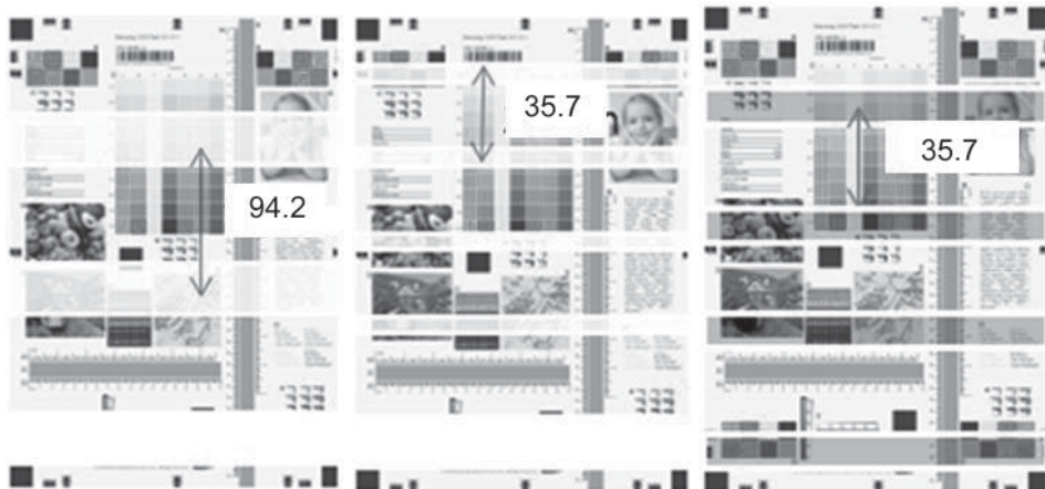
Figure 3-45 Typical faulty images
