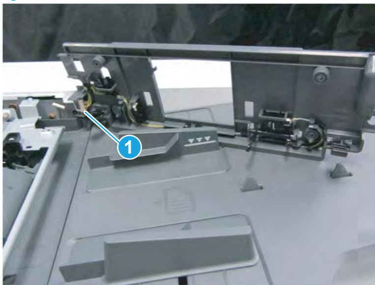
Figure 2-319 Turn the cover over and disconnect connector
