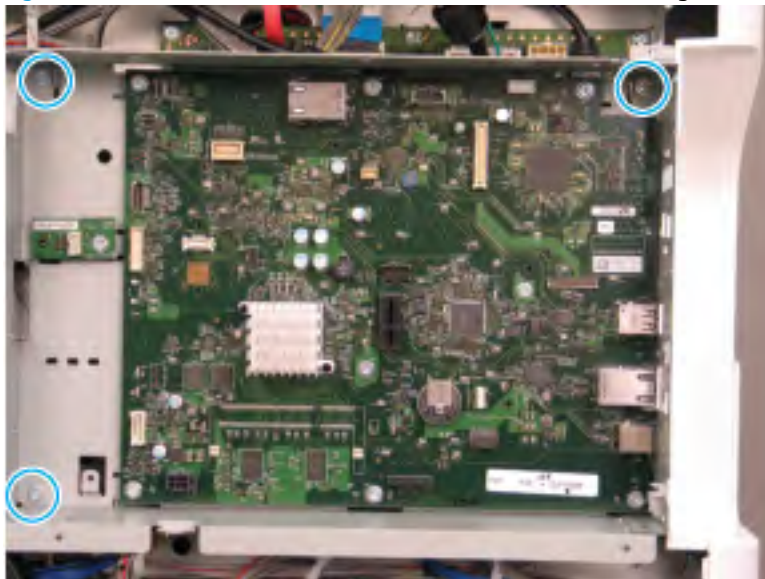
Figure 2-143 Remove three screws to remove the formatter cage
