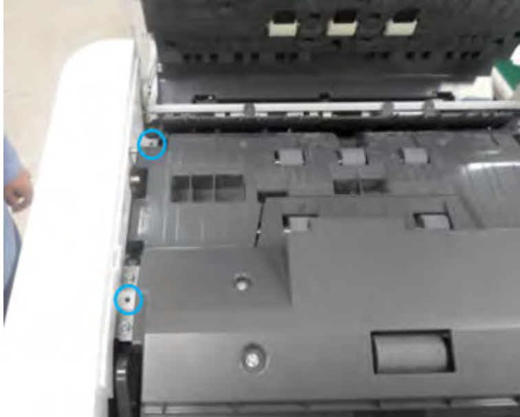
Figure 2-405 Remove the document feeder front cover top screws
