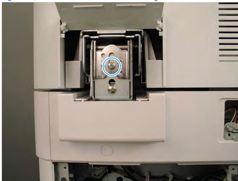
Figure 2-21 Release the document feeder hinge screws
