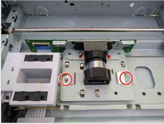
Figure 2-429 Remove screws and release scanner imaging unit
