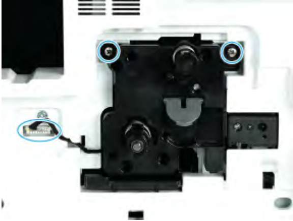
Figure 2-191 Disconnect drum unit connector
