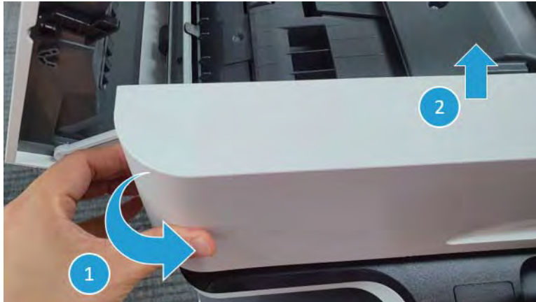
Figure 2-351 Remove the document feeder front cover
