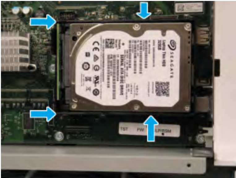
Figure 2-133 Remove the hard-disk drive (HDD)
