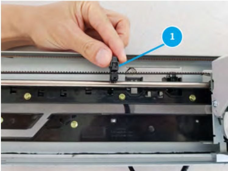
Figure 5-884 Remove stapler mid-rear sensor
