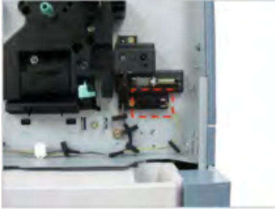
Figure 2-210 Disconnect connector and remove sensor
