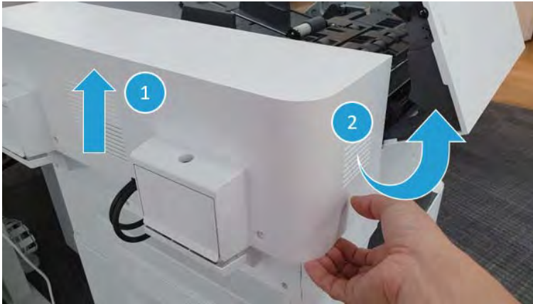
Figure 2-315 Release the top back cover.
