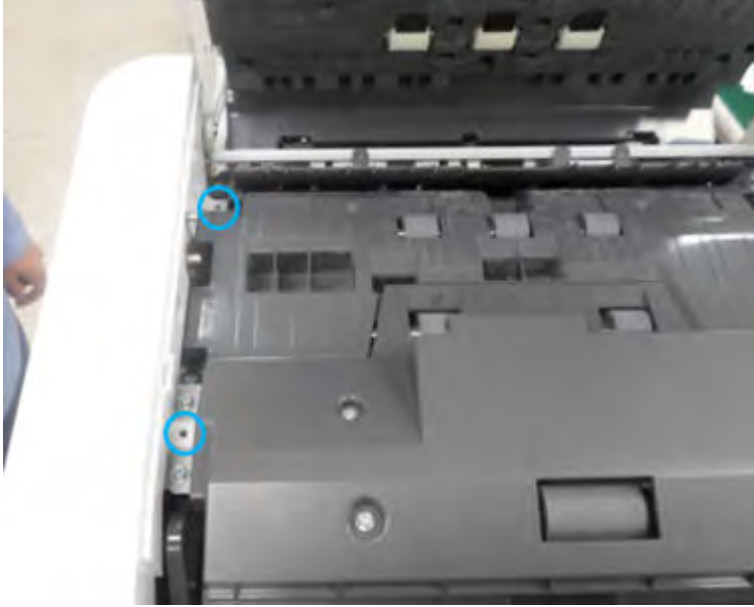
Figure 2-340 Remove the document feeder front cover top screws
