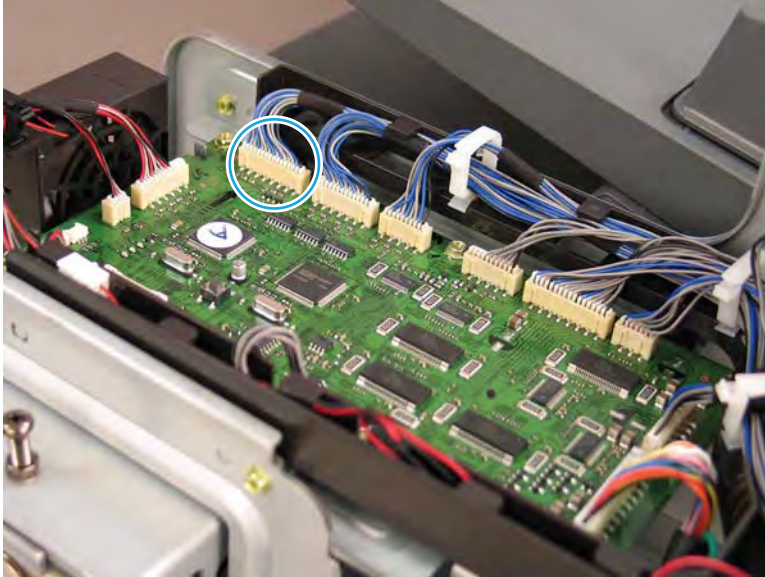
Figure 2-348 Disconnect the document feeder PCA connector
