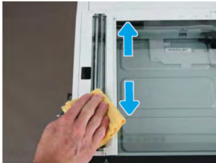
Figure 2-10 Clean the scanner glass (2 of 2)
