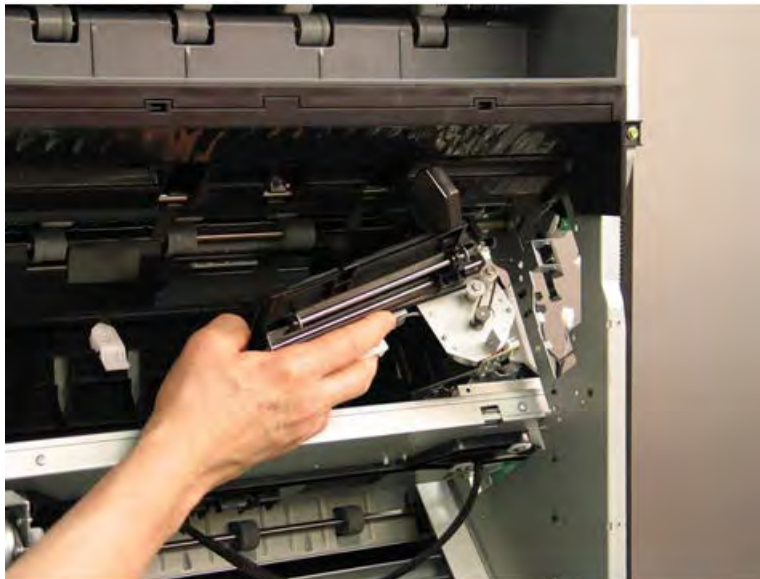
Figure 5-514 Remove the front tamper
