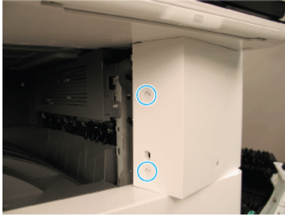
Figure 2-144 Remove the power-switch cover
