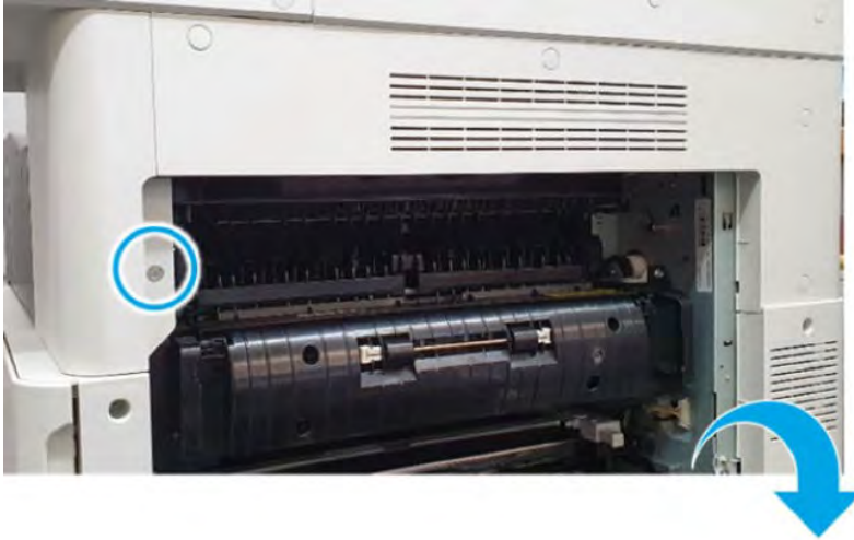
Figure 2-442 Remove the screw
