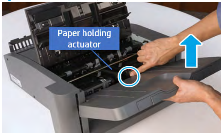
Figure 7-241 Remove the output tray.
