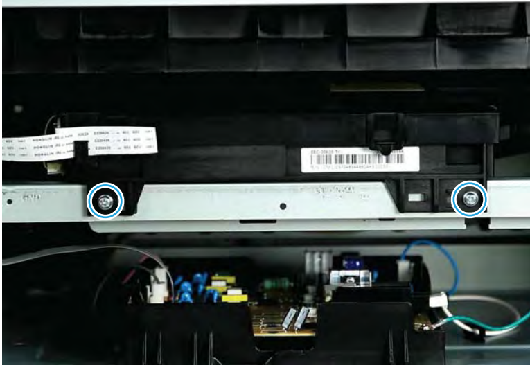
Figure 2-94 Remove the laser scanner assembly
