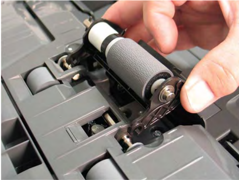
Figure 2-381 Release the separation roller
