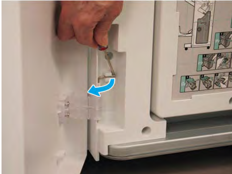
Figure 5-580 Release the lower hinge pin
