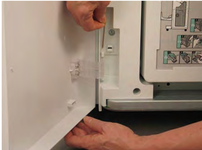
Figure 5-425 Remove the lower hinge pin
