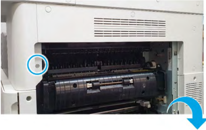
Figure 2-437 Remove the screw
