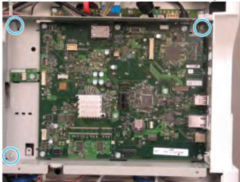
Figure 2-218 Remove three screws to remove the formatter cage
