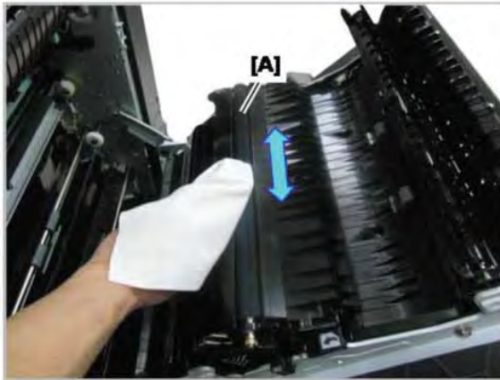
Figure 2-12 Transfer roller cleaning
