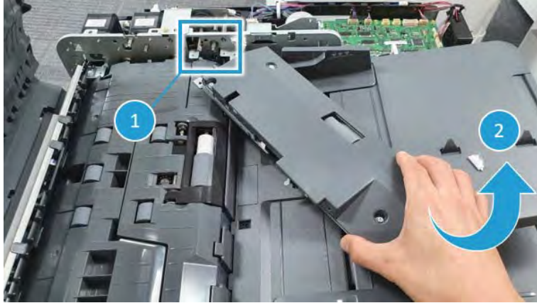
Figure 2-355 Remove the pickup roller assembly
