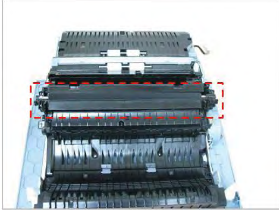
Figure 2-273 Remove transfer roller assembly
