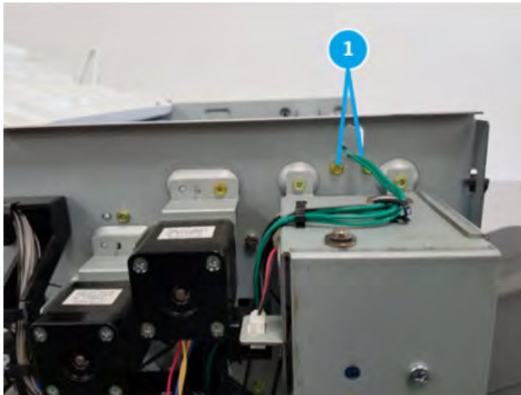
Figure 5-433 Remove two screws
