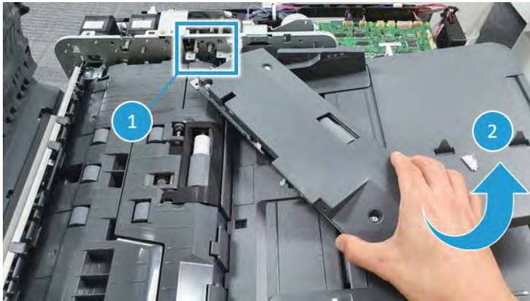
Figure 2-375 Remove the pickup roller assembly
