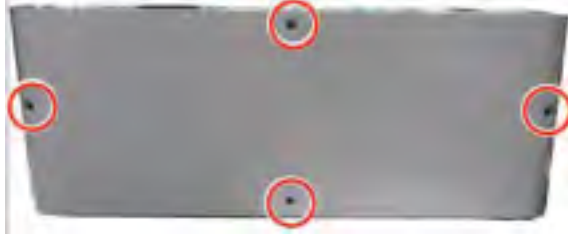
Figure 2-456 Remove the DCF rear cover
