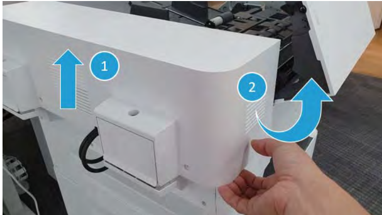
Figure 2-336 Release the top back cover.
