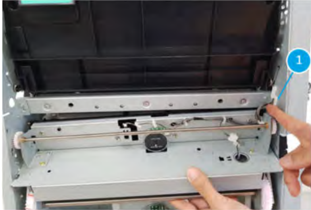
Figure 5-1731 Disconnect one connector
