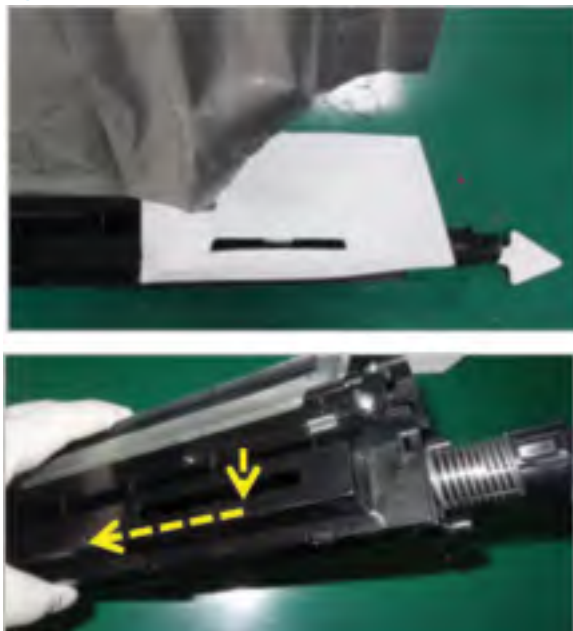
Figure 2-119 Fill developer unit with developer powder
