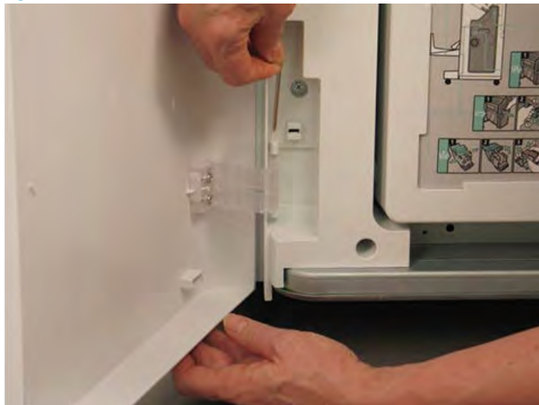
Figure 5-1219 Remove the lower hinge pin
