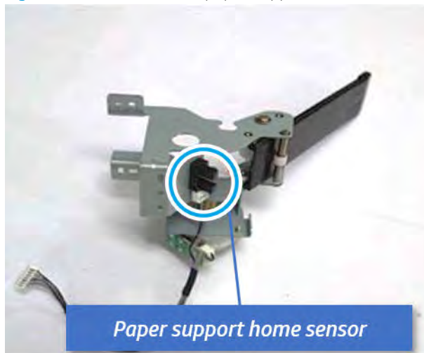
Figure 7-236 Remove the paper support home sensor
