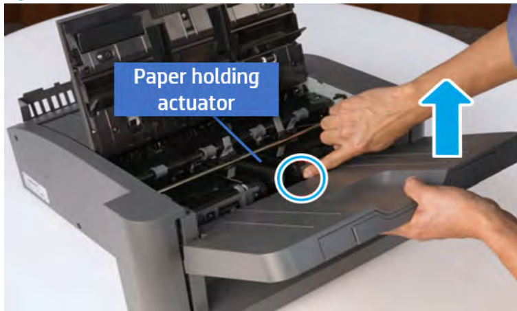
Figure 7-205 Remove the output tray.
