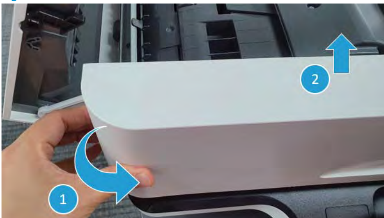
Figure 2-284 Remove the document feeder front cover
