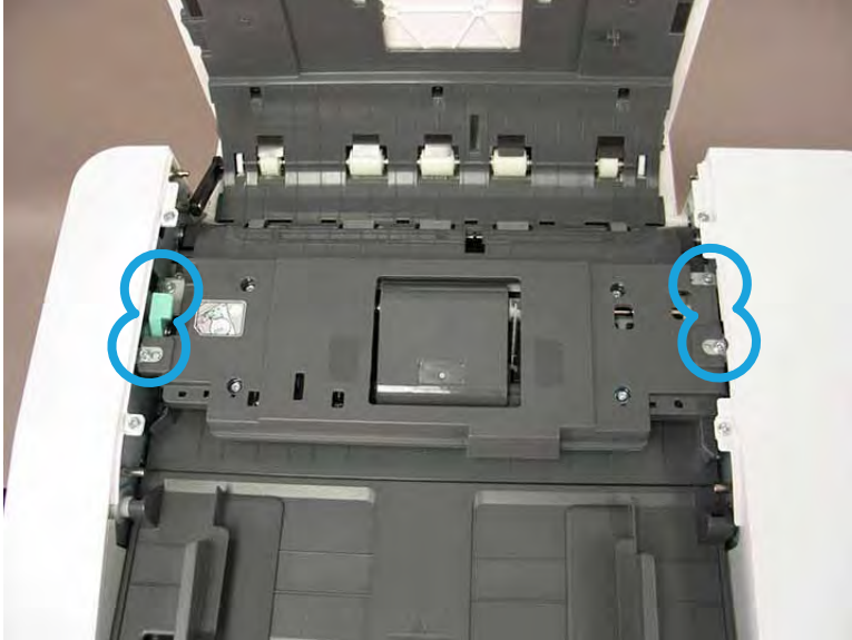
Figure 2-295 Remove four screws
