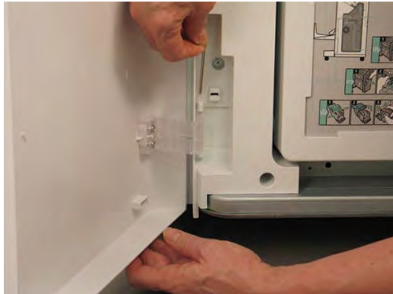
Figure 5-194 Remove the lower hinge pin
