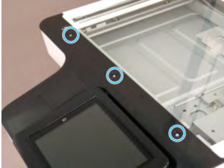
Figure 2-152 Remove the document feeder bezel
