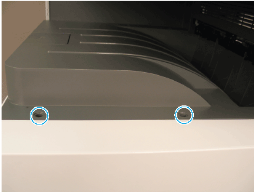
Figure 2-145 Remove screw-caps and screws
