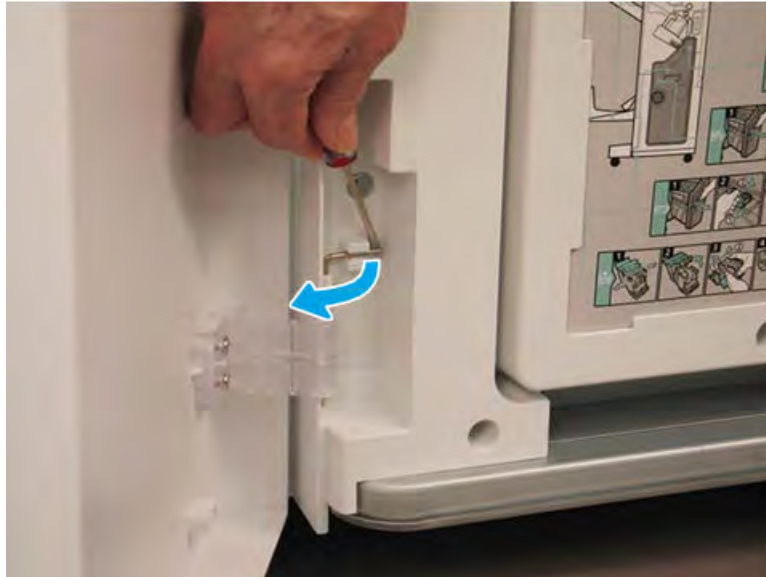
Figure 5-193 Release the lower hinge pin
