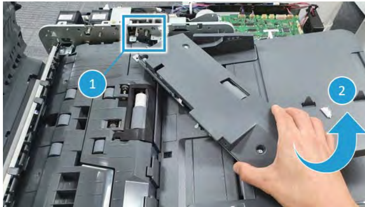
Figure 2-370 Remove the pickup roller assembly
