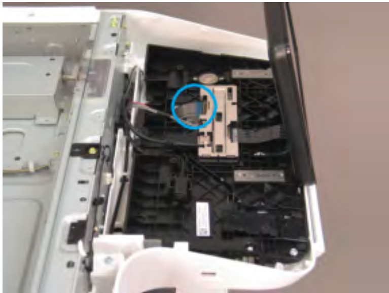
Figure 2-153 Disconnect one FFC
