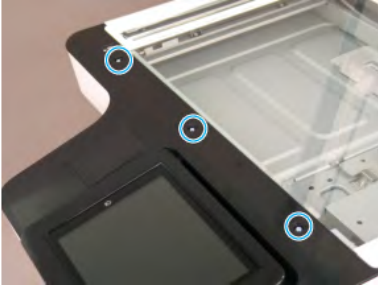
Figure 2-149 Remove the document feeder bezel
