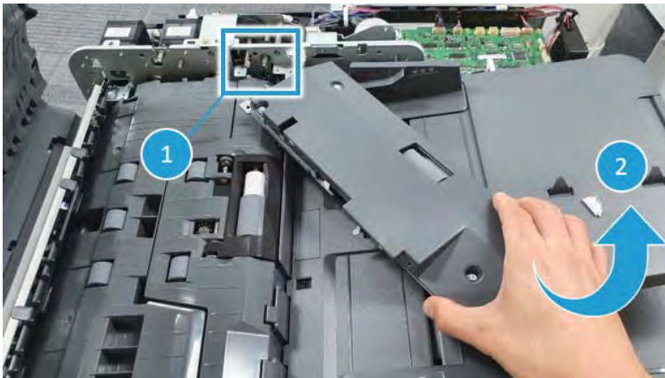
Figure 2-347 Remove the pickup roller assembly
