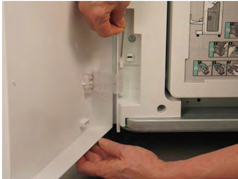
Figure 5-523 Remove the lower hinge pin
