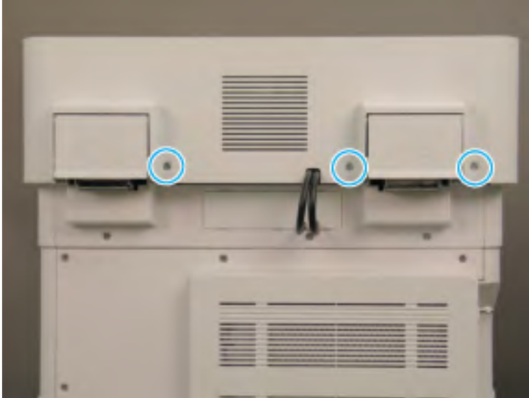
Figure 2-353 Remove the document feeder back cover bottom screws
