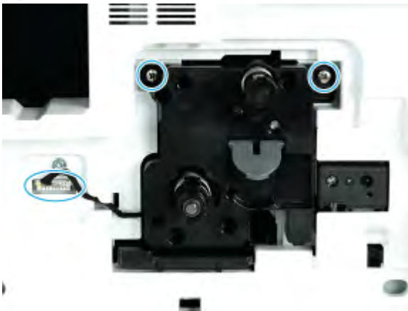
Figure 2-109 Disconnect drum unit and remove two screws
