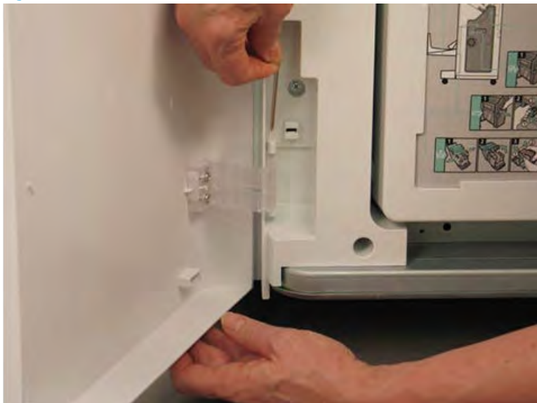
Figure 5-990 Remove the lower hinge pin
