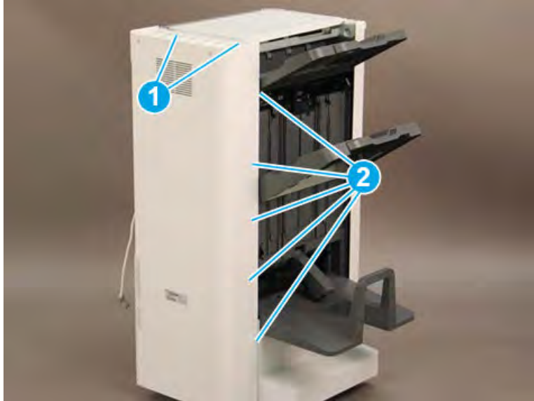
Figure 5-1420 Remove seven screws
