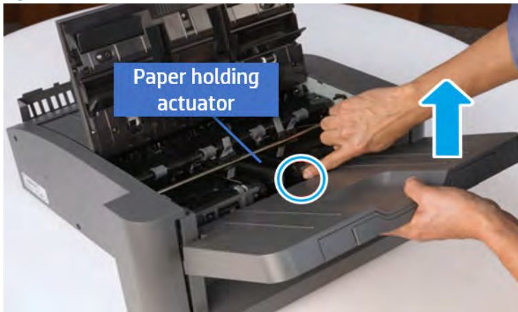
Figure 7-653 Remove the output tray.
