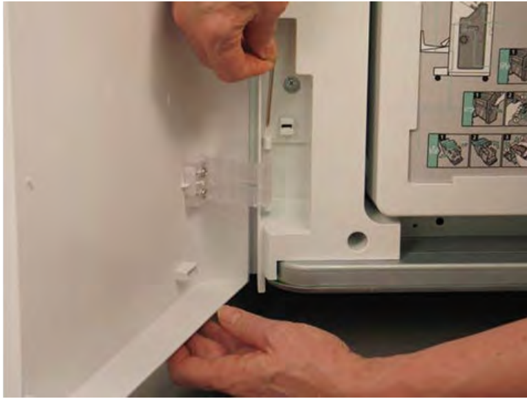
Figure 5-537 Remove the lower hinge pin
