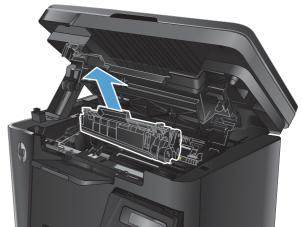
Remove any jammed paper visible in the input tray area. Use both hands to remove jammed paper to avoid tearing the paper.
