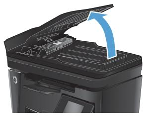
Use a moist, lint-free cloth to wipe both pickup rollers and the separation pad to remove dirt.
