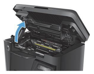
3. Remove any jammed paper from the output bin area. Use both hands to remove jammed paper to avoid tearing the paper.
