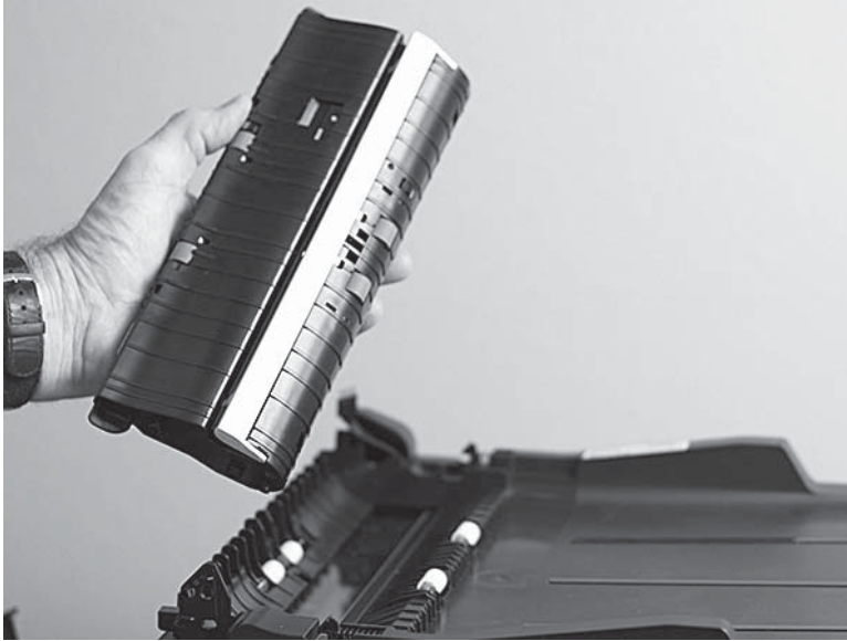
Figure 1-172 Remove the document feeder core assembly (5 of 5)
