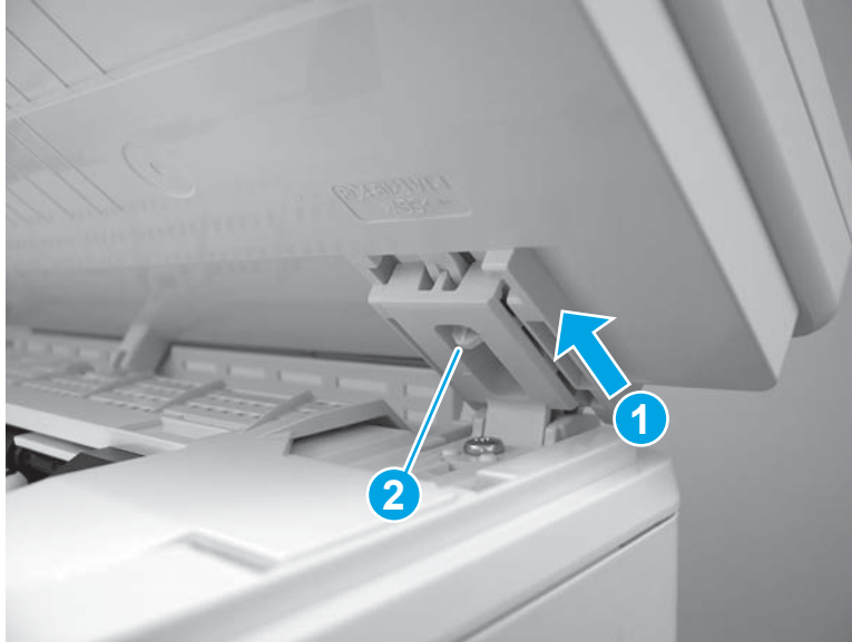
Figure 1-1847 Engage the right hinge (MFP)
