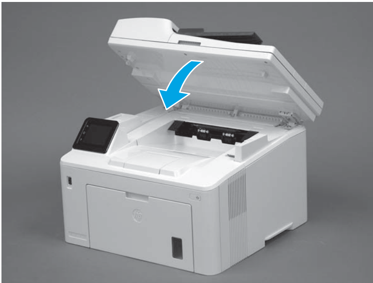
Figure 1-22 Close the scanner assembly
