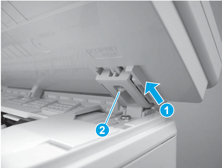
Figure 1-428 Engage the right hinge (MFP)
