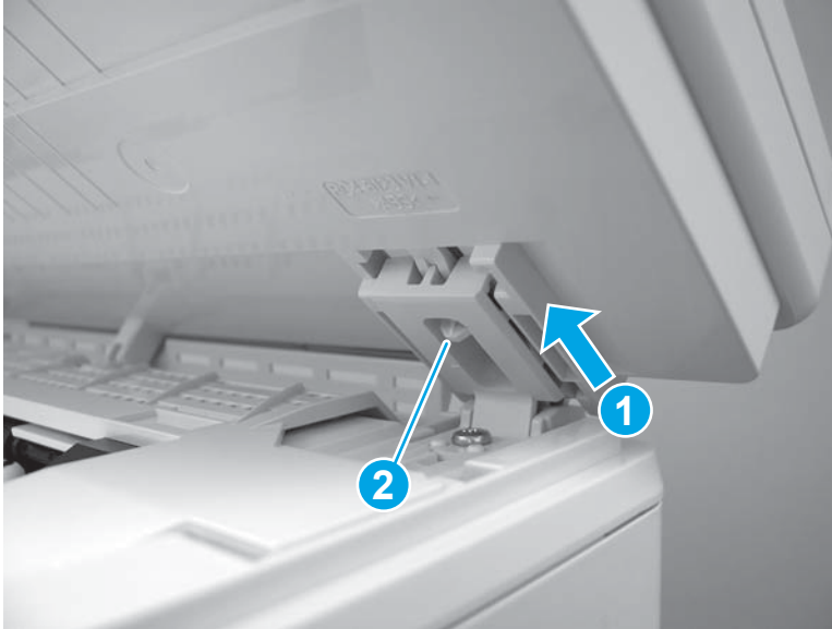
Figure 1-1125 Engage the right hinge (MFP)
