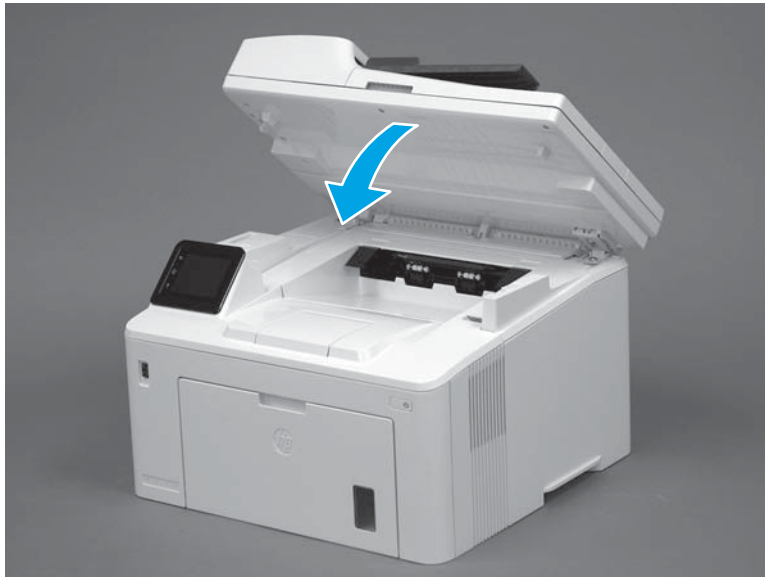
Figure 1-387 Close the scanner assembly
