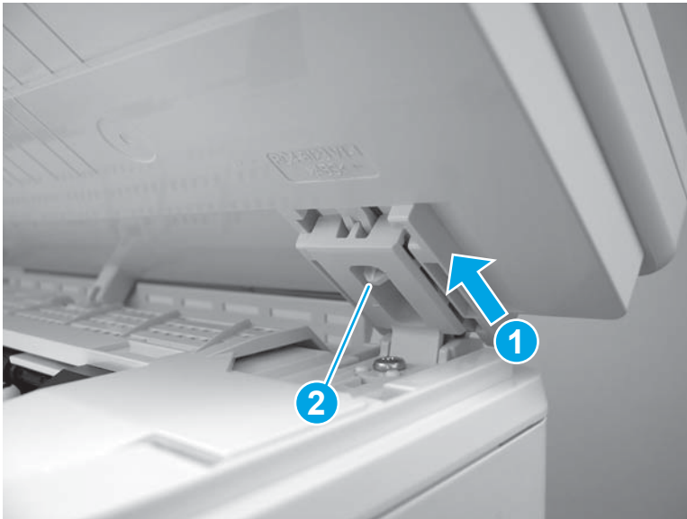
Figure 1-123 Engage the right hinge (MFP)
