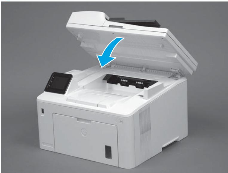
Figure 1-127 Close the scanner assembly
