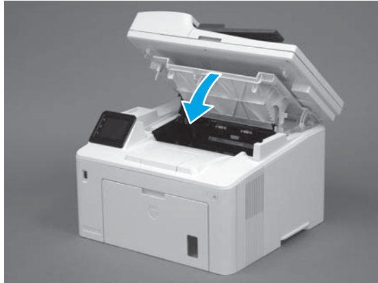
Figure 1-10 Close the cartridge door
