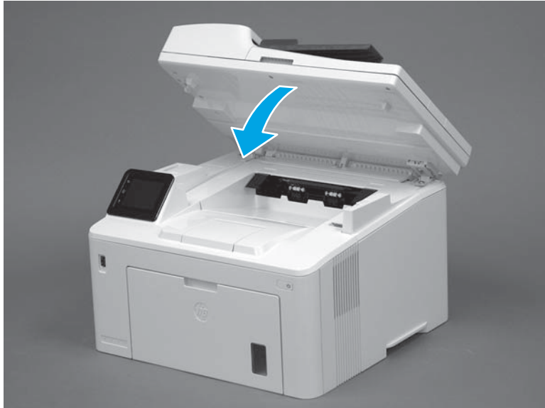
Figure 1-645 Close the scanner assembly
