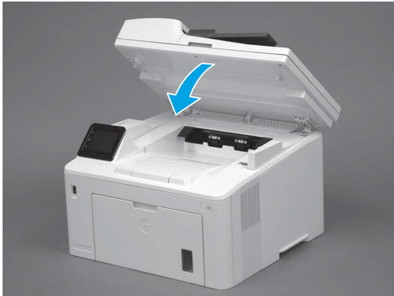
Figure 1-40 Close the scanner assembly
