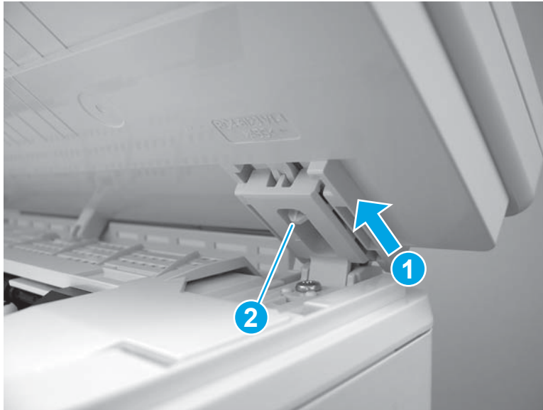
Figure 1-1929 Engage the right hinge (MFP)
