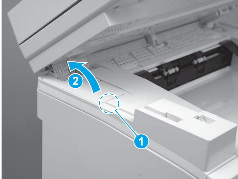
Figure 1-139 Remove the cable cover (MFP)
