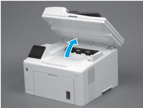
Figure 1-514 Open the cartridge door
