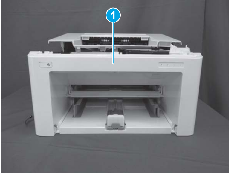
Figure 1-1207 Install the front cover (SFP)
