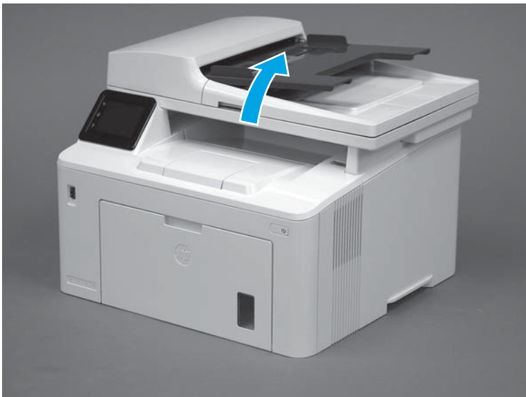
Figure 1-138 Open the scanner assembly
