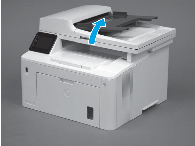
Figure 1-12 Open the scanner assembly
