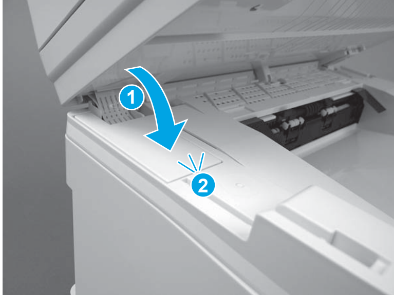
Figure 1-644 Install the cable cover (MFP)
