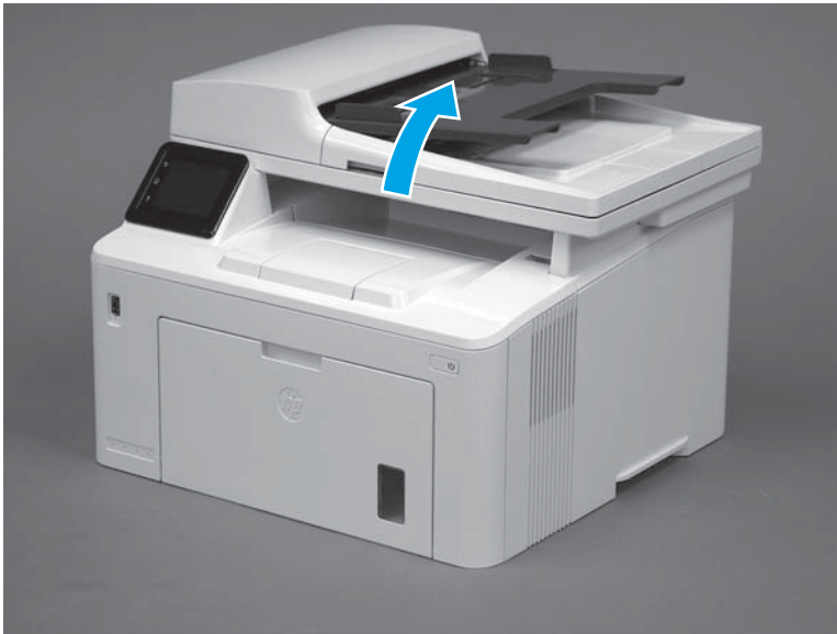
Figure 1-8 Open the scanner assembly
