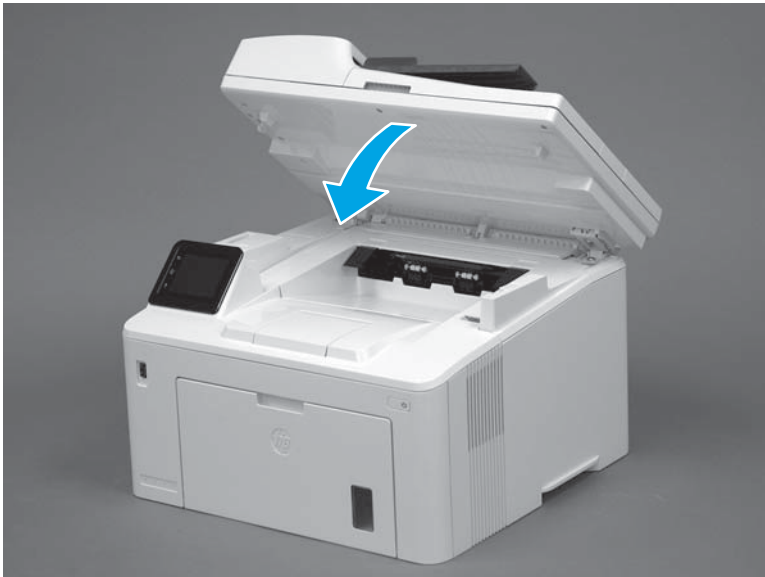
Figure 1-333 Close the scanner assembly
