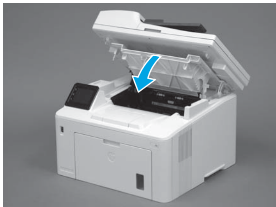
Figure 1-5 Close the cartridge door
