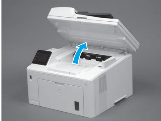
Figure 1-9 Open the cartridge door
