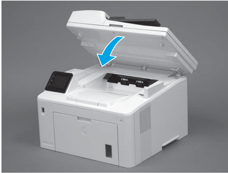
Figure 1-947 Close the scanner assembly
