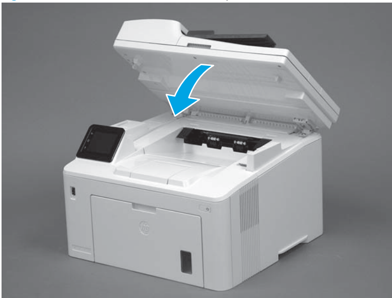
Figure 1-520 Close the scanner assembly
