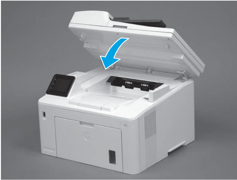
Figure 1-179 Close the scanner assembly
