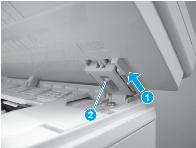
Figure 1-383 Engage the right hinge (MFP)
