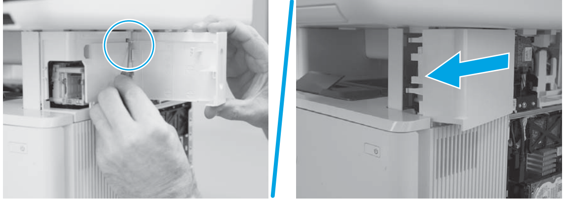
Figure 1-550 Release the upper hinge or remove the cover
