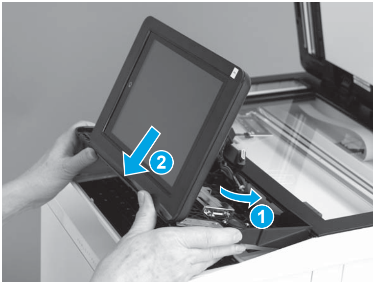
Figure 1-65 Install the control-panel
