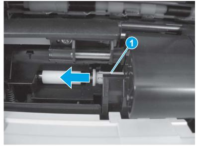
**4.** Remove the separation roller.
