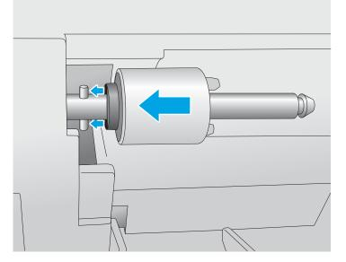
5. Slide the feed roller onto the shaft. You might have to rotate the roller while sliding it onto the shaft to make sure it clicks into place.
