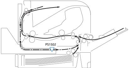
The duplexer determines a jam if the sensor detects media presence at a specified timing stored in the duplex driver.
