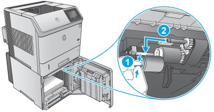
5. Inside the tray cavity, pinch the blue tab that is on the left side of the lower pick roller (callout 1), and then slide the roller off of the shaft (callout 2).
