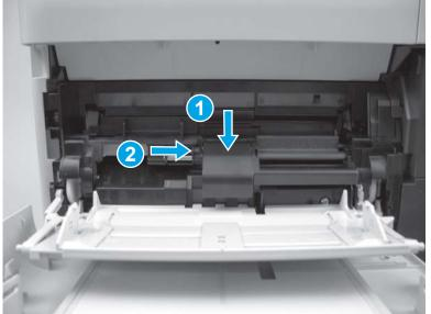
3. Slide the roller-shaft bushing (callout 1) to the right and onto the shaft to install it.
