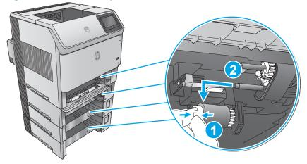
Figure 2-126 Remove the pick roller
