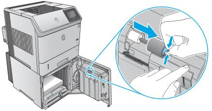
4. Inside the tray cavity, pinch the blue tab that is on the left side of the upper feed roller (callout 1), and then slide the roller off of the shaft (callout 2).
