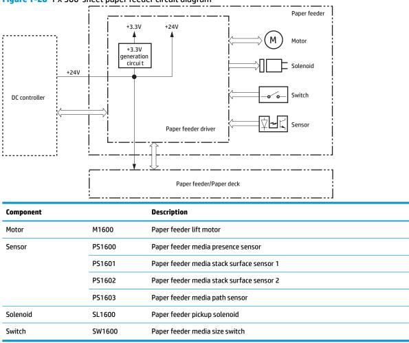
Figure 1-28 1 x 500-sheet paper feeder circuit diagram
