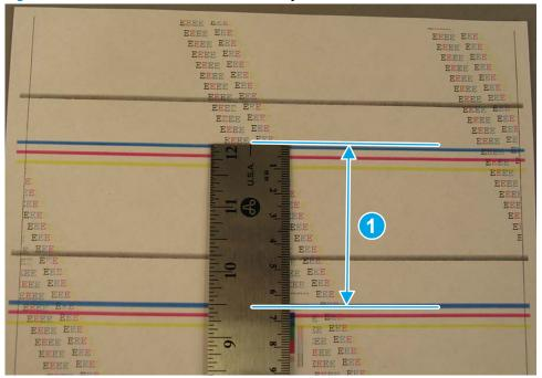
Figure 2-102 Determine the defective assembly
