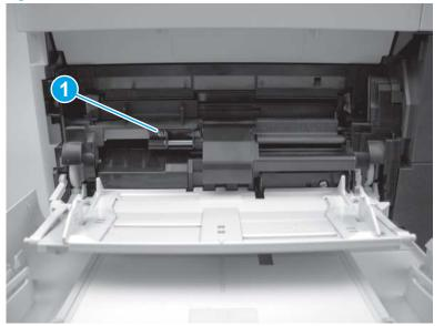
6. Push down on the roller-shaft bushing (callout 1) to release two alignment pins, and then slide the bushing to the left and off of the shaft to remove it.
