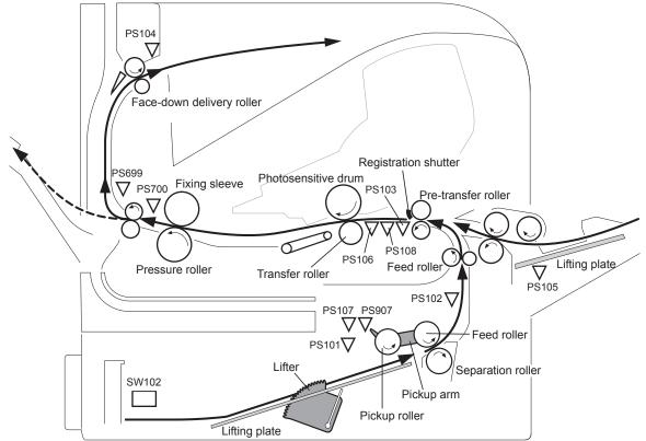
Table 2-13 Product base, sensors and switches block diagram
