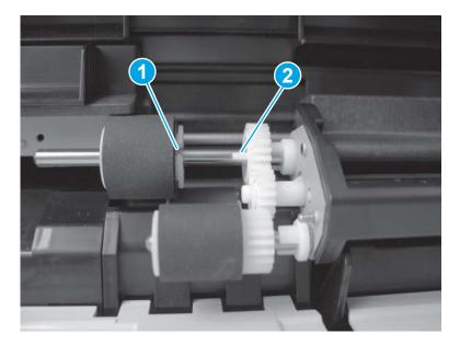
2. Position the Tray 1 rollers cover over the pickup and feed rollers (callout 1), and then slide the cover to the right (callout 2) to install it.
