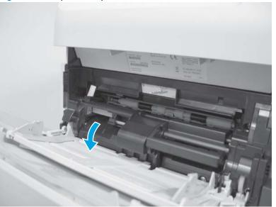
Figure 2-106 Open the separation roller cover
