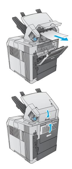
3. Close the door on the stacker or stapler/stacker, and close the rear output bin.
