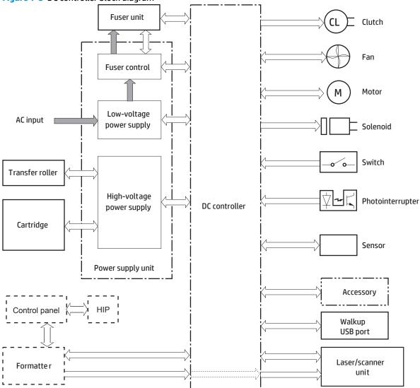
Figure 1-3 DC controller block diagram
