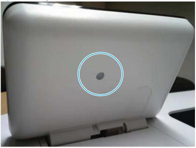
Figure 2-21 Diagnostic-tests access button
