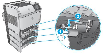
4. Inside the tray cavity, pinch the blue tab that is on the left side of the lower pick roller (callout 1), and then slide the roller off of the shaft (callout 2).
