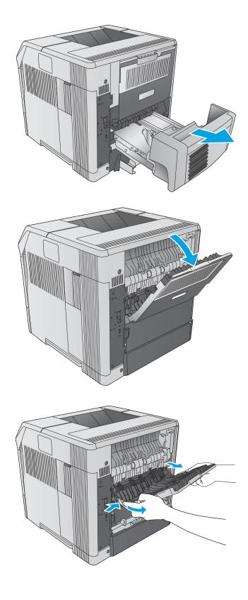
Push up on the two blue levers on the sides of the fuser to release it, and then pull the fuser straight out of the product to remove it..
