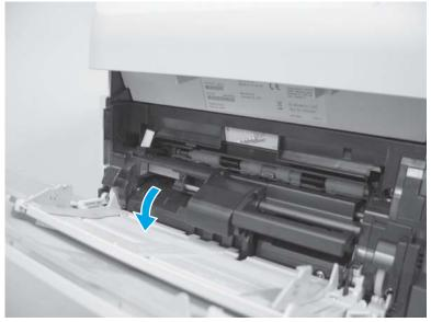
6. Position the separation roller onto the shaft.
