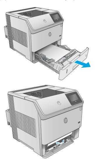
2. If the edge of the jammed paper is visible in the feed area, slowly pull the paper down and toward the back of the product. Then pull it out of the product. (Do not pull the paper straight out, or it will tear.) If the paper is not visible, look in the next tray or in the top-cover area.
