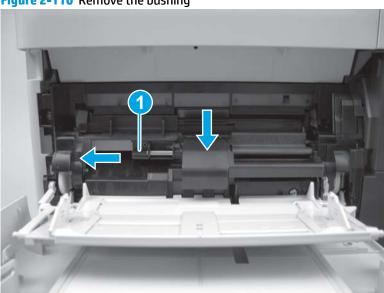
Figure 2-110 Remove the bushing
