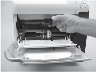
8. Slide the Tray 1 pickup roller (callout 1) and the feed roller (callout 2) to the left and off of the shafts to remove them.
