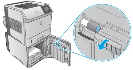
3. Pinch the blue tab that is on the left side of the separation roller, and then slide the roller off of the shaft.
