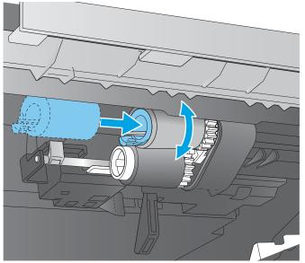
Figure 2-141 Install the feed roller
