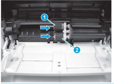
Figure 2-114 Install the Tray 1 pickup and feed rollers
