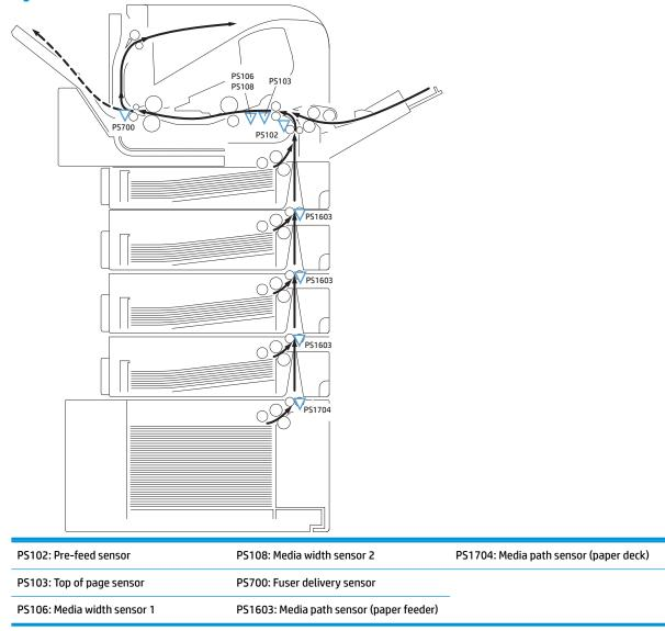
The printer determines a jam if the sensor detects paper presence at a specified timing stored in the DC controller.
