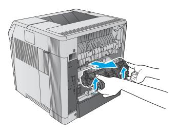
Remove the jammed paper. If necessary, lift the black plastic guide that is located on the top of the fuser to gain access to the jammed sheet.
