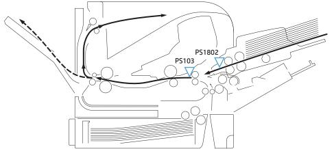
The envelope feeder driver determines a jam if the sensor detects envelope presence at a specified timing stored in the envelope feeder driver. The envelope feeder driver stops a print operation and notifies the DC controller when it determines a jam has occurred.
