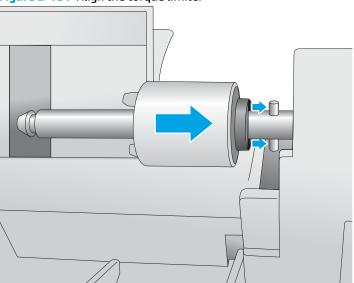
Figure 2-131 Align the torque limiter
