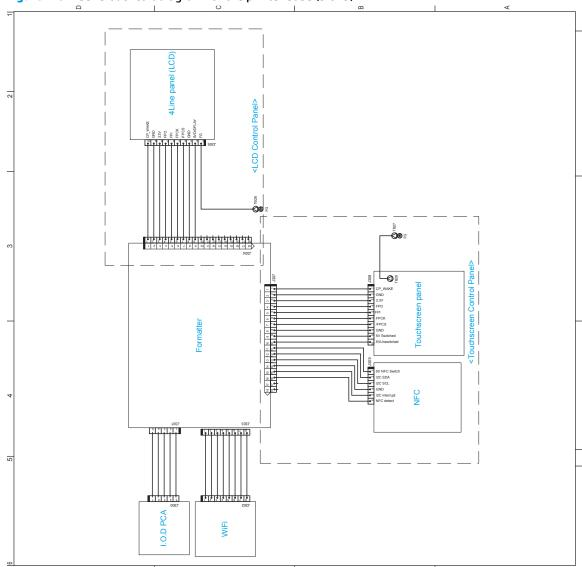
Figure 2-81 General circuit diagram for the printer base (3 of 3)
