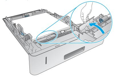
2. Pinch the blue tab that is on the left side of the roller, and then slide the roller off of the shaft.
