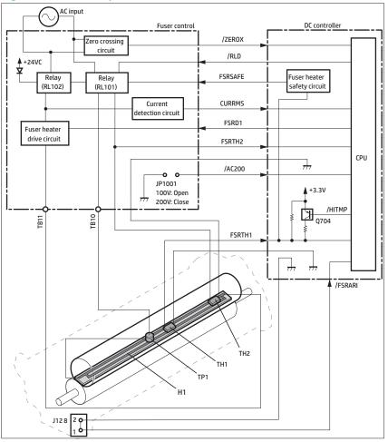
Figure 1-7 Fuser temperature-control circuit
