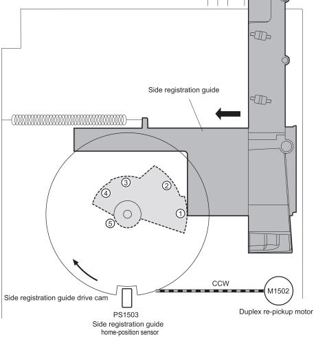
The sequence of the side registration adjustment operation is as follows:
