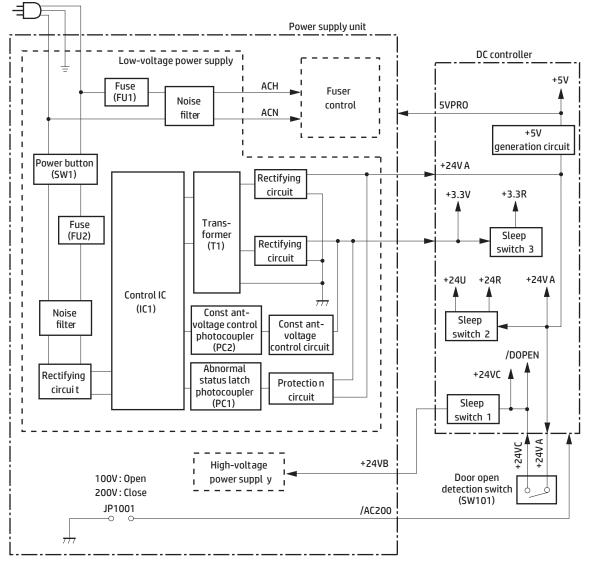
Figure 1-4 Low-voltage power-supply circuit
