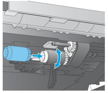
2. Inside the tray cavity, slide the upper feed roller onto the shaft. You might have to rotate the roller while sliding it onto the shaft to make sure it clicks into place.
