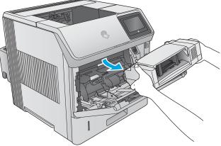
2. Grasp both sides of the envelope feeder and carefully pull it out of the product.
