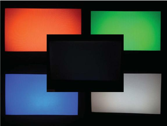
5. Pressing the diagnostic-tests button with the black screen displayed, exits the diagnostic mode.
