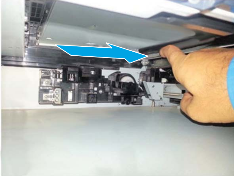
Figure 2-63 Removing paper Stuck in Duplex re-feed path.
