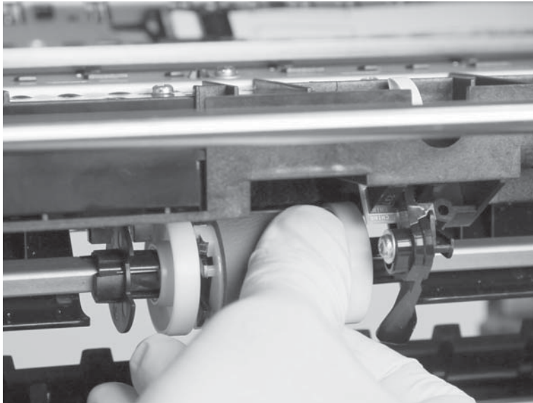
Figure 1-67 Reinstall the separator/pick assembly (4 of 5)
