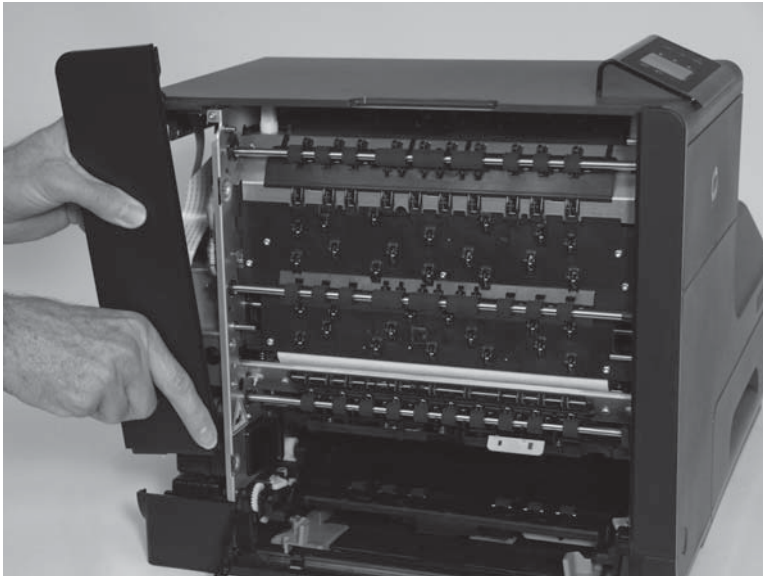
Figure 1-33 Remove the left rear cover (2 of 2)
