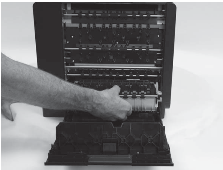
Figure 1-15 Remove the duplex module (2 of 2)
