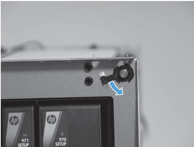
Figure 1-131 Remove the output drive shaft 6 (2 of 3)
