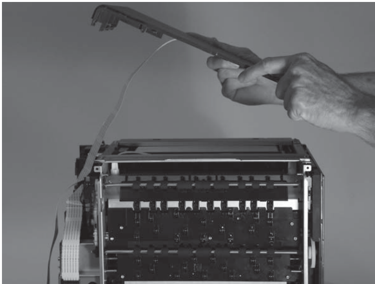
Figure 1-43 Remove the top cover (8 of 8)
