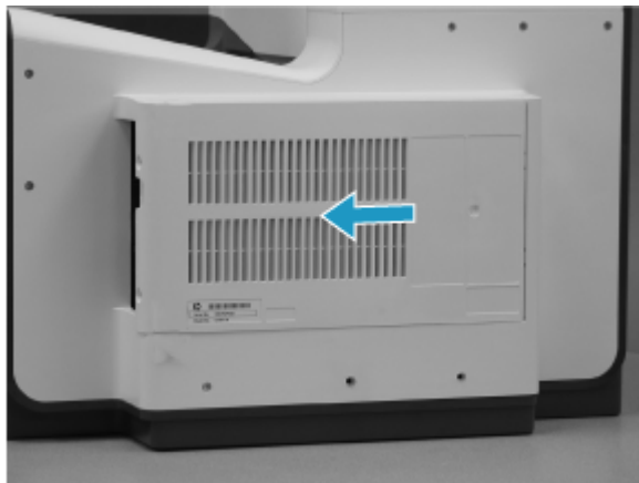
Figure 5-547 Remove the formatter cover (PM)
