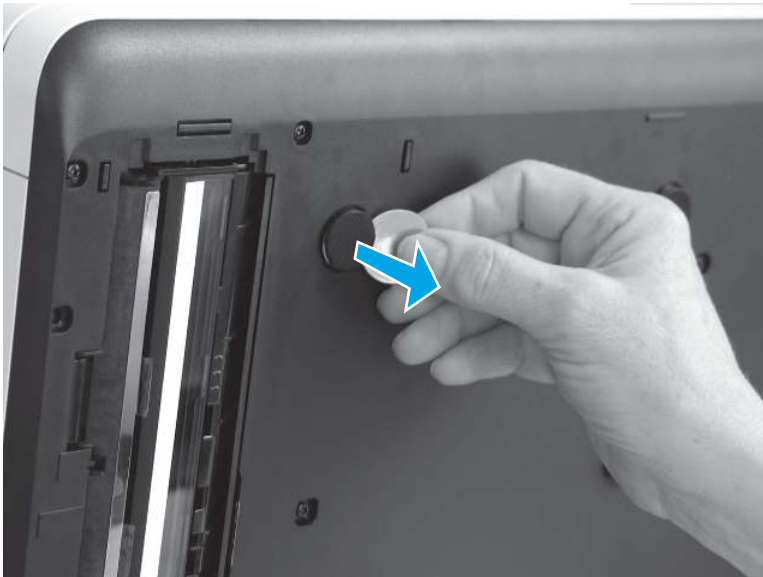
Figure 5-17 Loosen damaged clips
