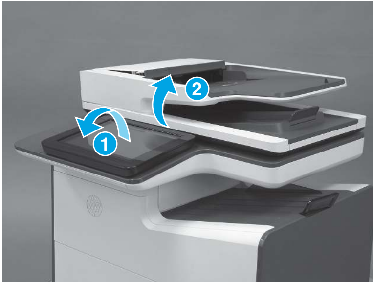
Figure 5-182 Tilt the control panel up
