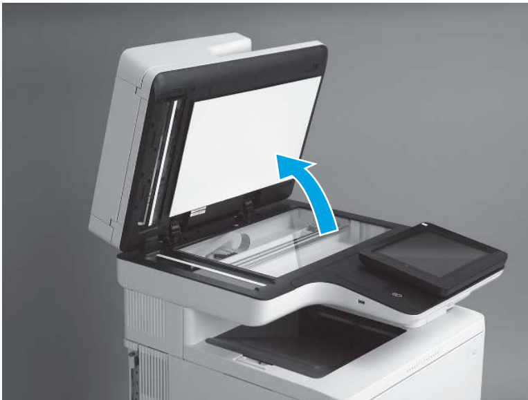
Figure 5-24 Check the white backing
