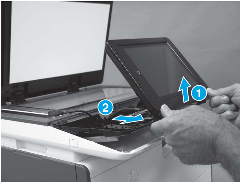
Figure 5-41 Remove the control panel
