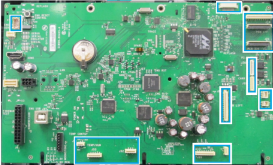
Figure 5-681 Disconnect the cables and FCCs from the ECB
