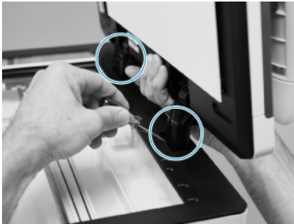
Figure 5-291 Release two tabs on the hinges
