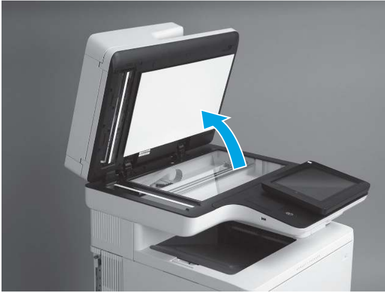
Figure 5-26 Open the document feeder
