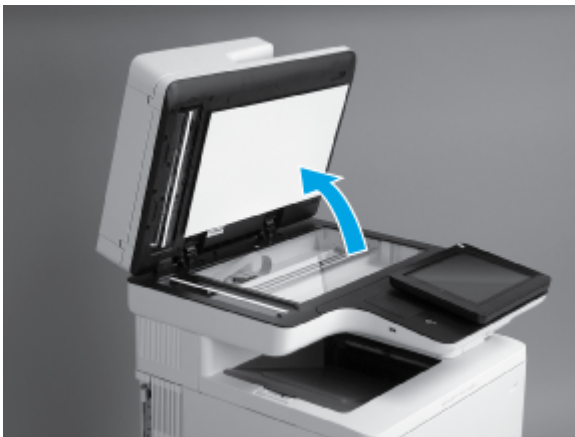
Figure 5-337 Open the document feeder
