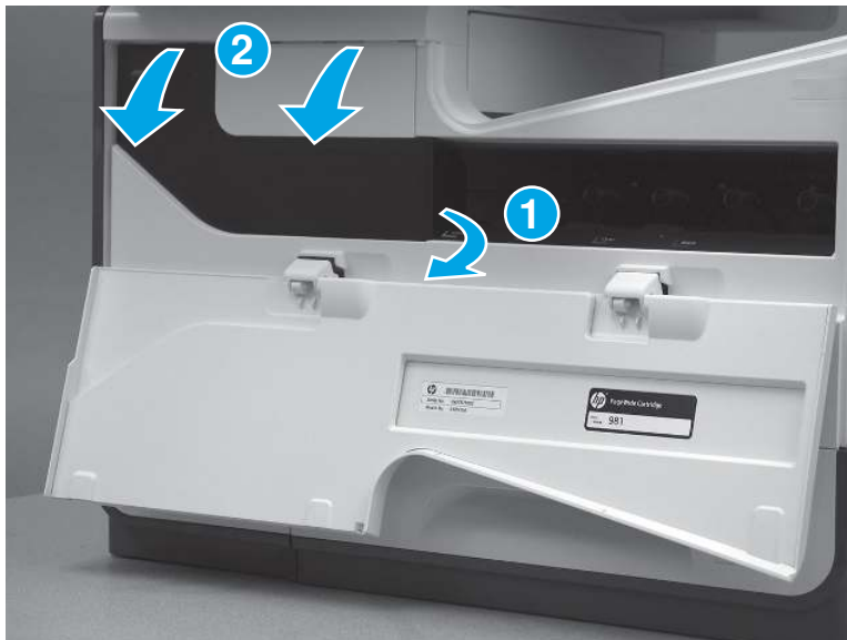
Figure 5-499 Open the blank cover
