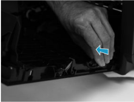
Figure 5-94 Reattach each restraining strap
