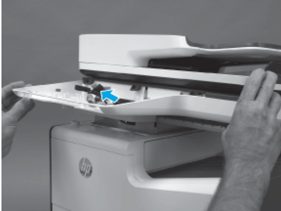
Figure 5-600 Pass the wire harnesses and cables through the opening
