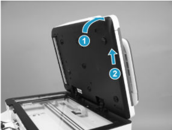
Figure 5-366 Tilt the document feeder back
