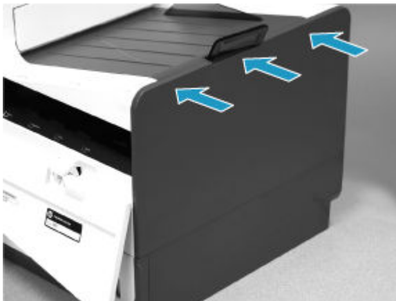
Figure 5-332 Install the right cover (outer)
