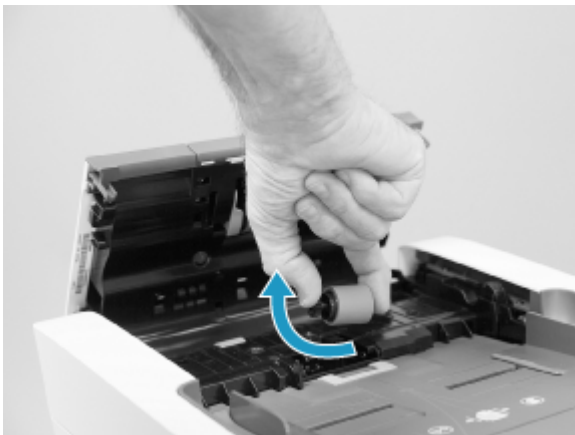
Figure 5-700 Remove the roller assembly
