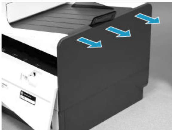
Figure 5-118 Release the right cover (outer)
