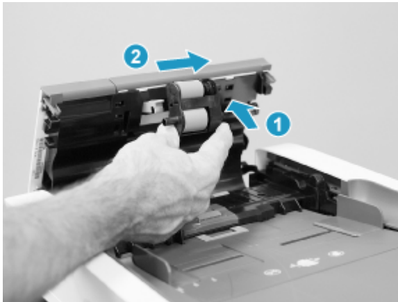
Figure 5-705 Install the roller assembly
