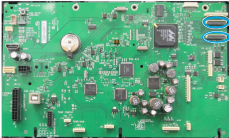
Figure 5-680 Zero Insertion Force (ZIF) and ECB sockets
