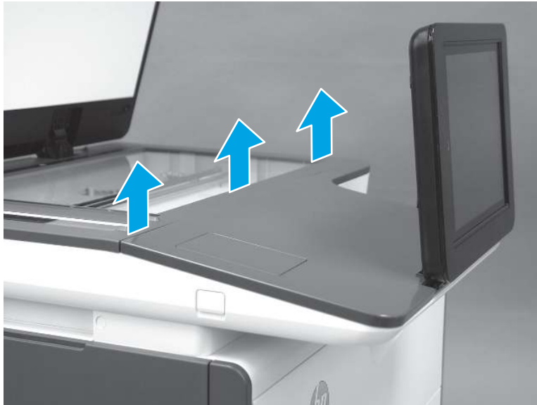
Figure 5-53 Release three bosses
