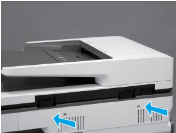
Figure 5-410 Install the SCB cover
