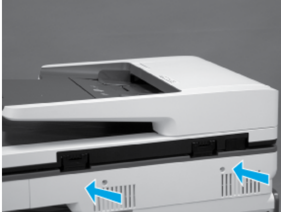
Figure 5-335 Install the SCB cover
