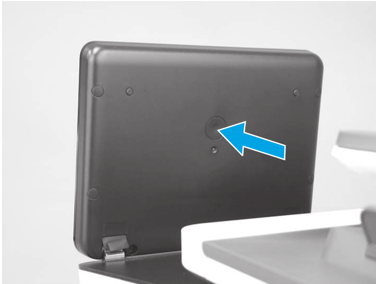
Figure 4-47 Press the diagnostics-access button (586)
