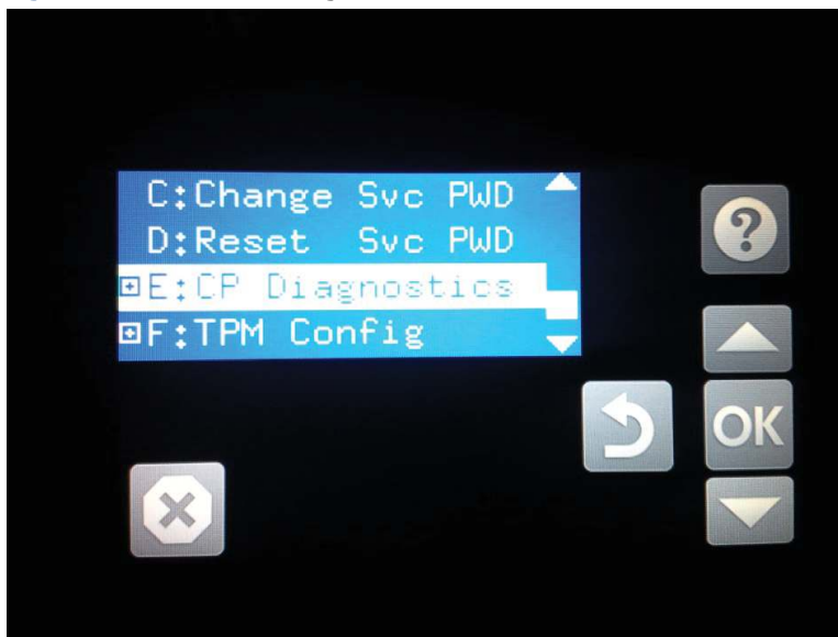
Figure 4-53 Access the diagnostics menu
