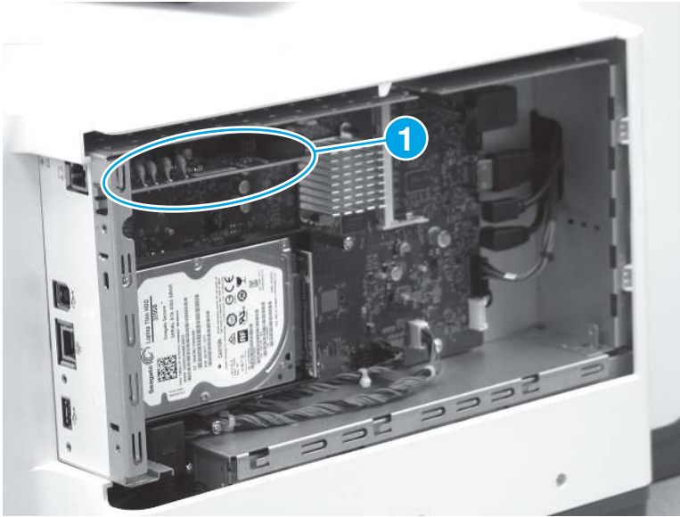
Figure 5-709 Locate the fax PCA
