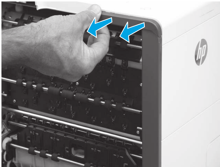
Figure 5-108 Remove left-rear top cover cap (556)
