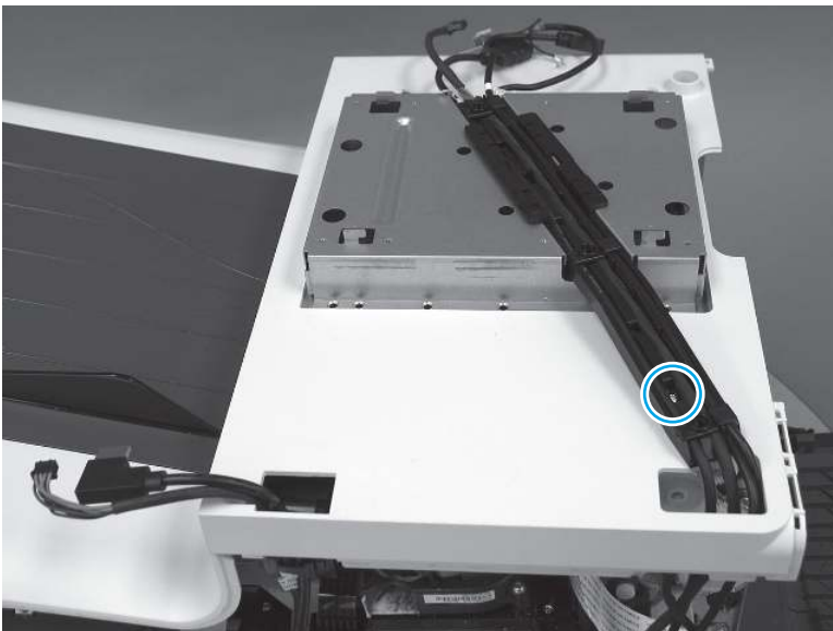
Figure 5-170 Remove one screw
