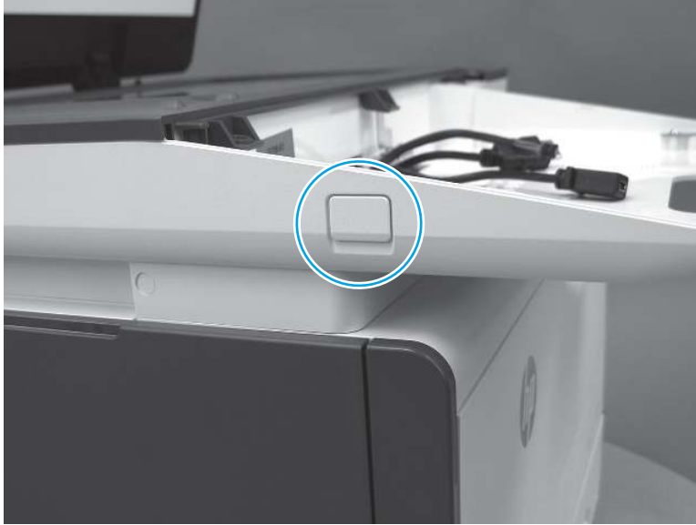
Figure 5-390 Install the USB port cover
