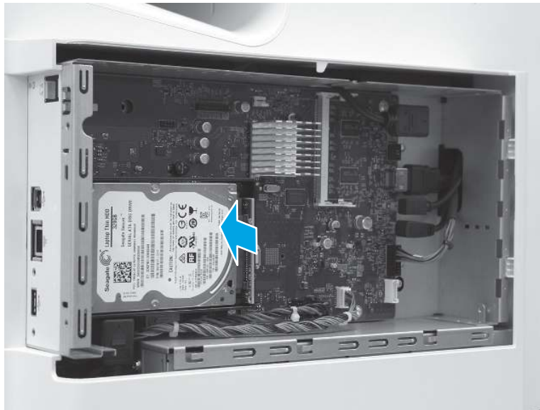
Figure 5-73 Install the HDD
