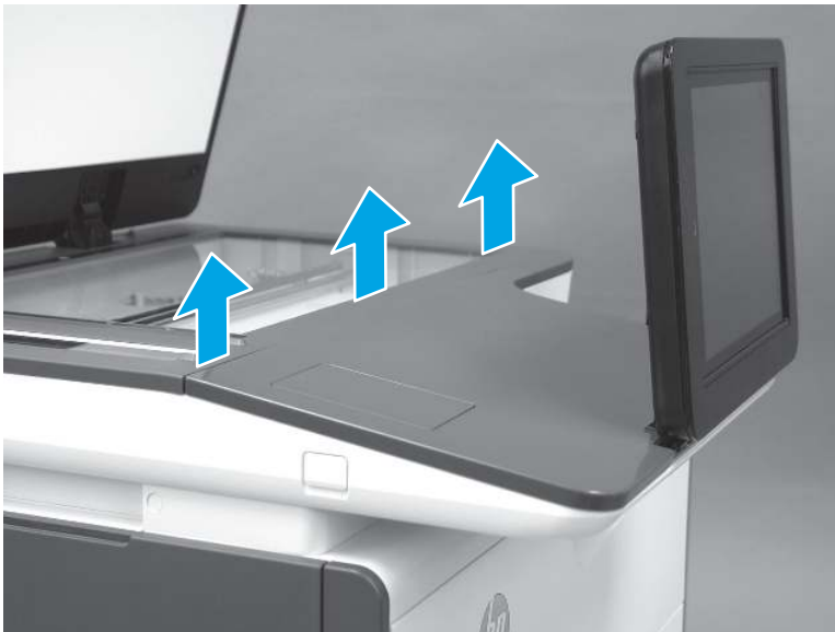
Figure 5-185 Release three bosses
