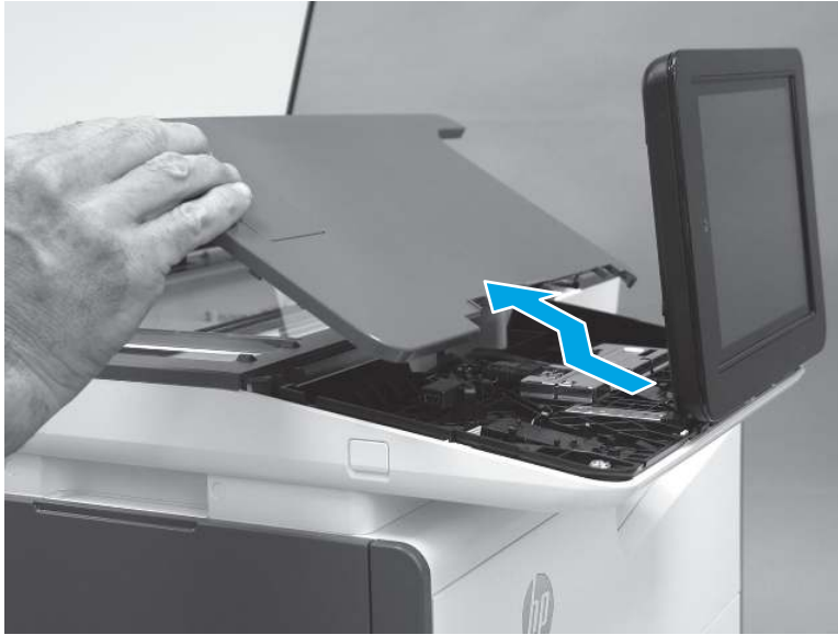
Figure 5-186 Remove the control-panel cover
