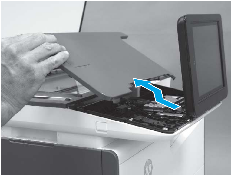
Figure 5-579 Remove the control-panel cover
