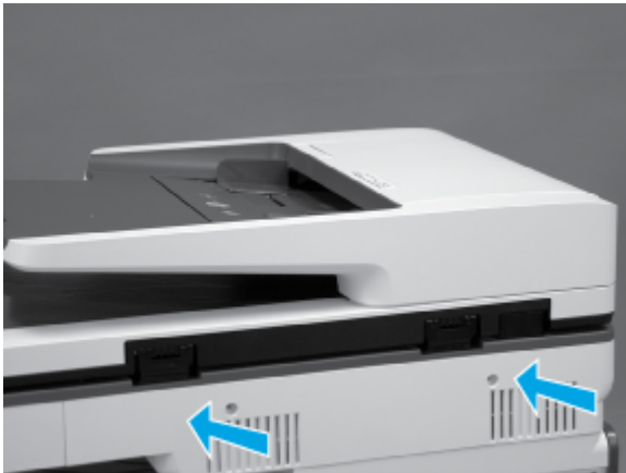
Figure 5-100 Install the SCB cover
