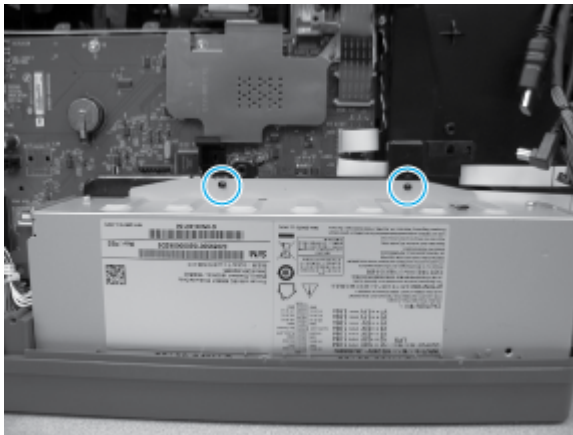
Figure 5-521 Check the locator pins
