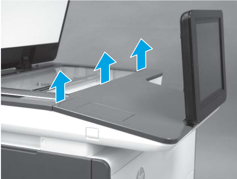
Figure 5-578 Release three bosses
