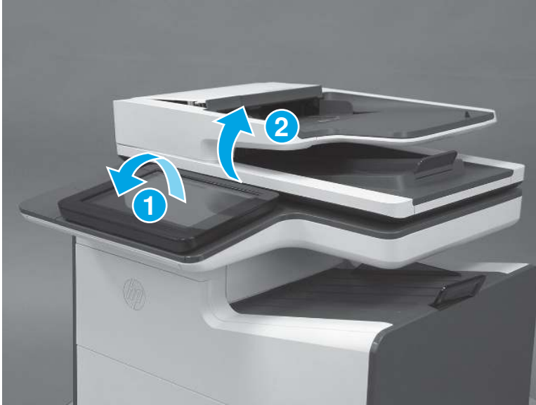
Figure 5-50 Tilt the control panel up
