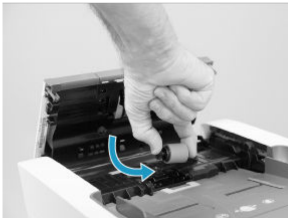
Figure 5-701 Install the roller assembly
