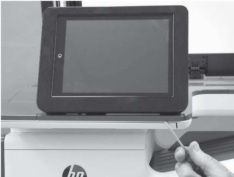
Figure 5-134 Release the small gray plastic cover
