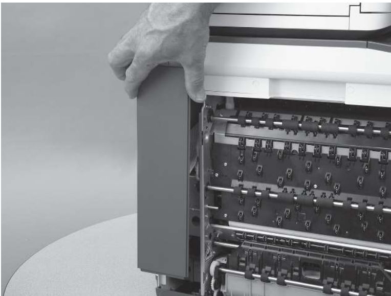
Figure 5-158 Remove the cover
