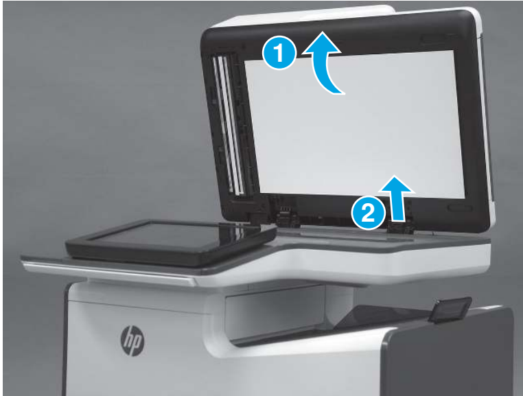
Figure 5-290 Tilt the document feeder back
