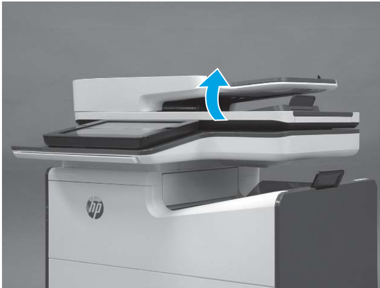
Figure 5-289 Open the document feeder
