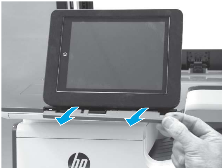
Figure 5-577 Remove the cover
