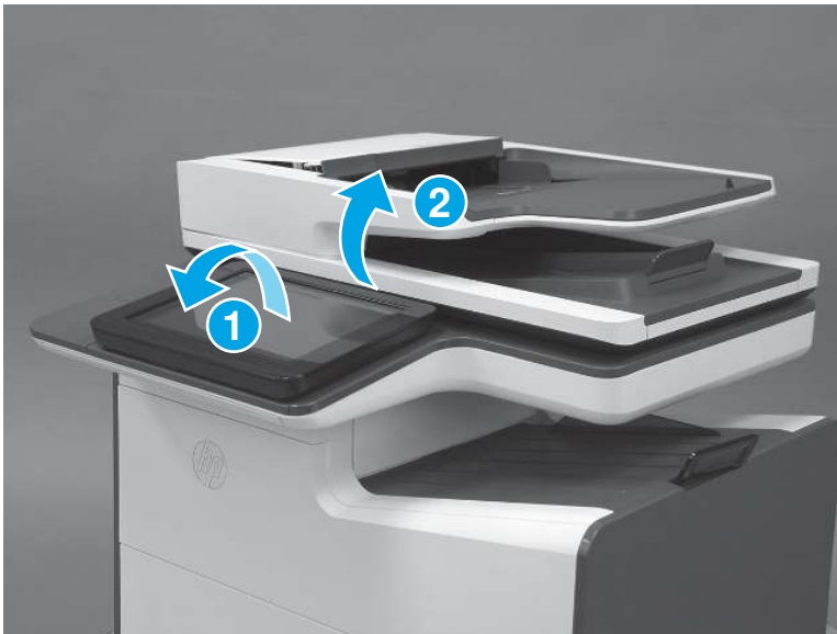
Figure 5-575 Tilt the control panel up
