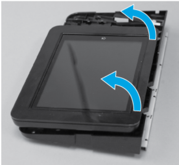
Figure 5-42 Open the replacement control panel
