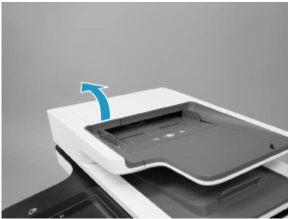
Figure 5-695 Open the door
