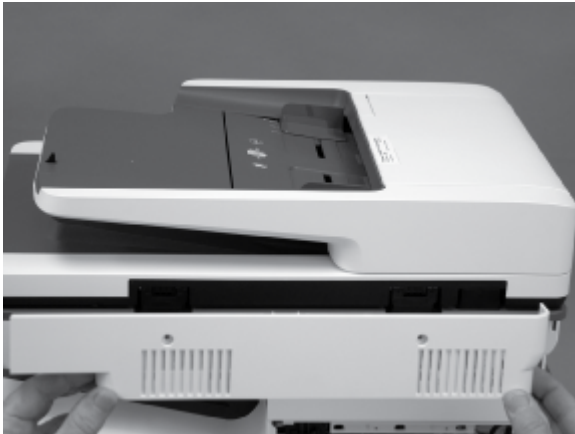
Figure 5-334 Align the SCB cover tabs and printer slots
