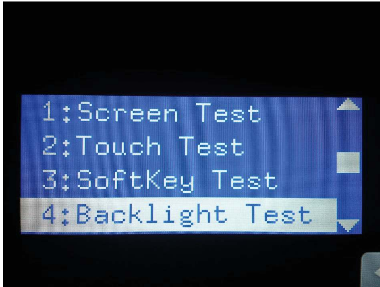
Figure 4-62 Open the backlight test
