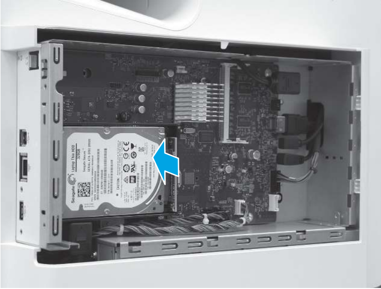
Figure 5-281 Install the HDD
