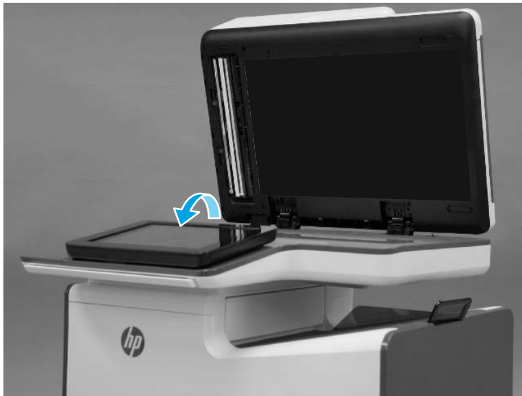
Figure 5-339 Tilt the control panel up
