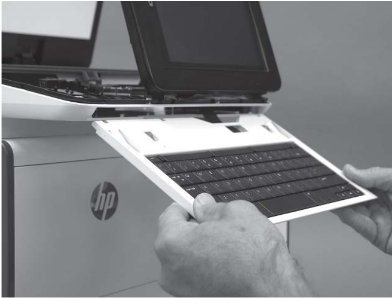
Figure 5-582 Remove the keyboard (586z)
