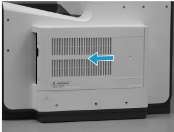
Figure 5-471 Remove the formatter cover (PM)
