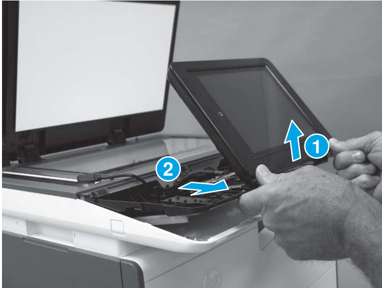
Figure 5-584 Remove the control panel
