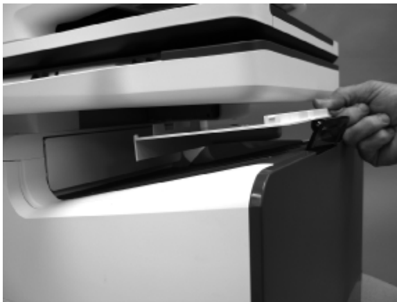
Figure 5-594 Remove the scanner base cover
