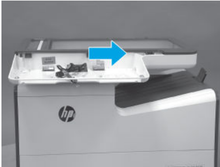
Figure 5-382 Slide the SSA right
