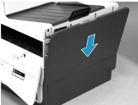
Figure 5-534 Position the right cover (outer) on the printer
