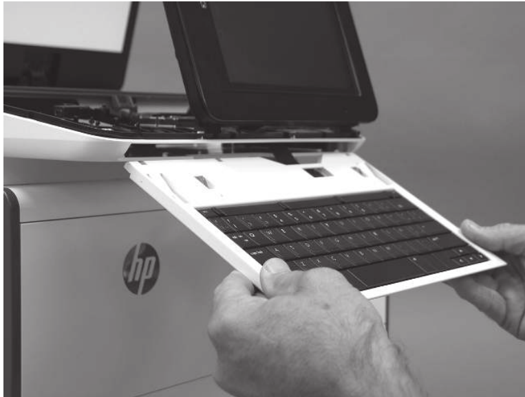
Figure 5-59 Install the keyboard
