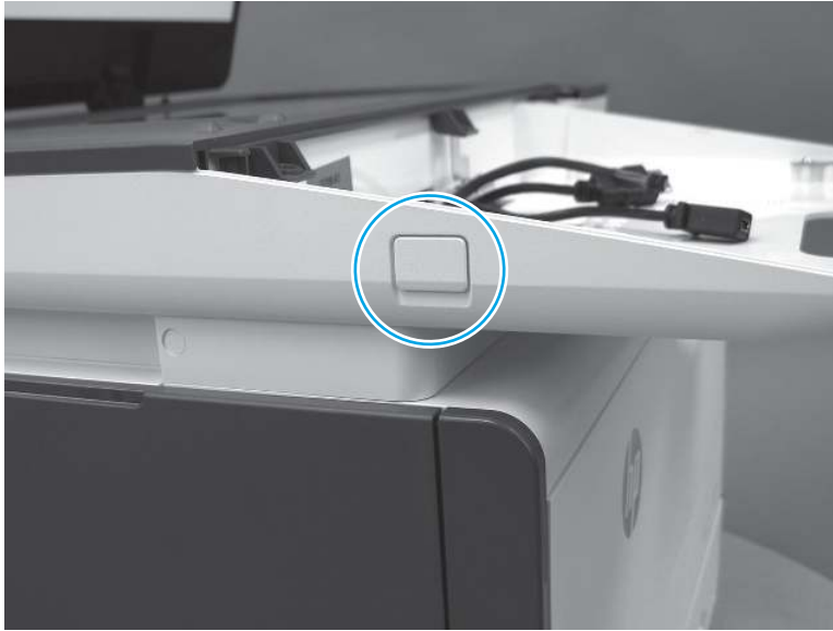
Figure 5-613 Install the USB port cover
