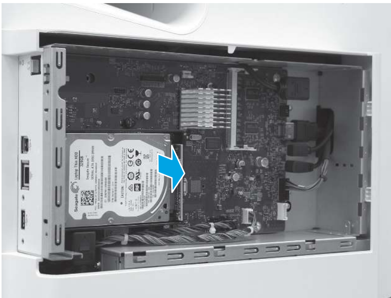
Figure 5-262 Remove the HDD
