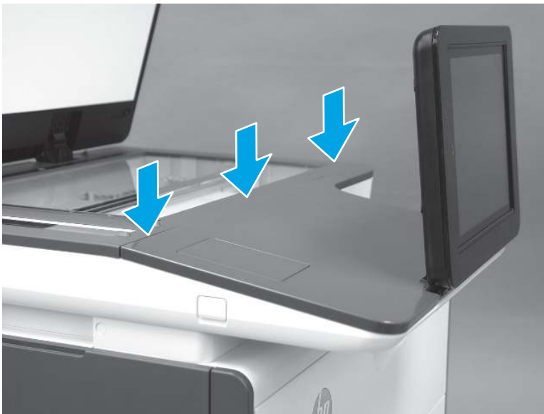
Figure 5-62 Engage three bosses
