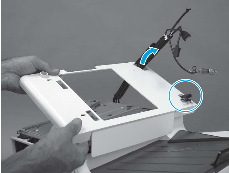
Figure 5-234 Remove the cover
