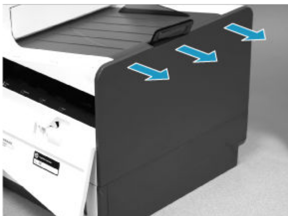
Figure 5-7 Release the right cover (outer)
