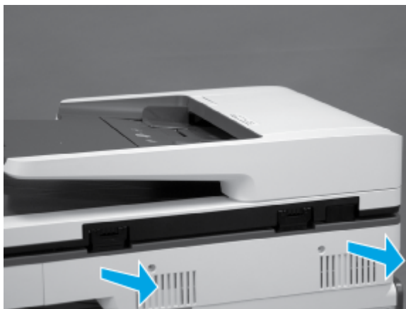
Figure 5-287 Remove the SCB cover
