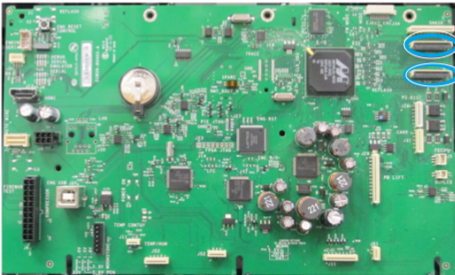
Figure 5-686 Zero Insertion Force (ZIF) and ECB sockets
