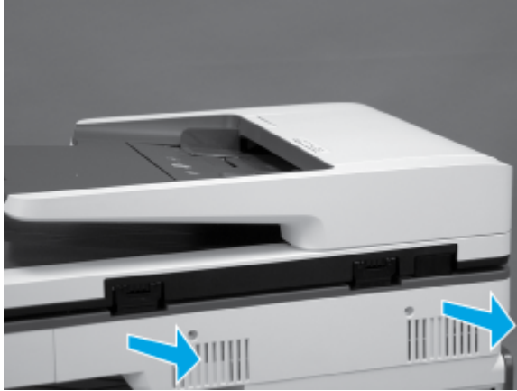
Figure 5-350 Remove the SCB cover
