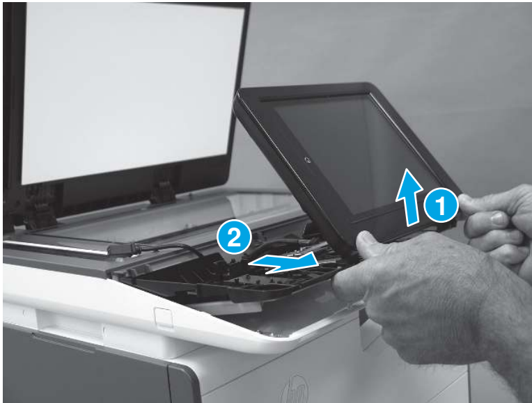
Figure 5-348 Remove the control panel
