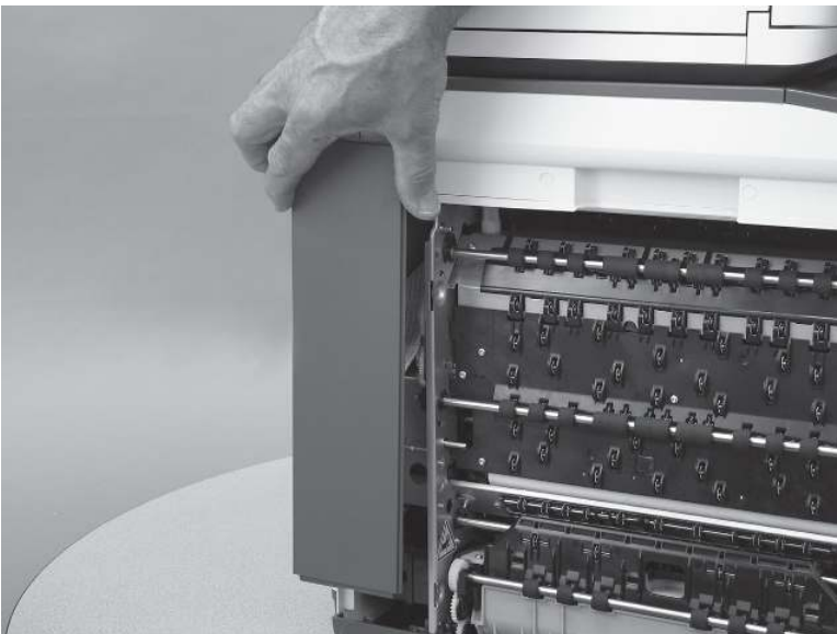
Figure 5-113 Remove the cover
