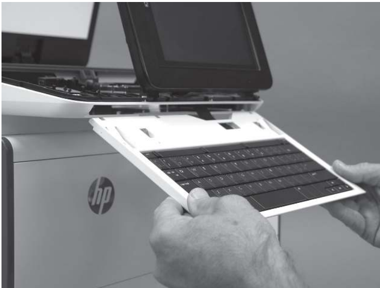
Figure 5-189 Remove the keyboard (586z)
