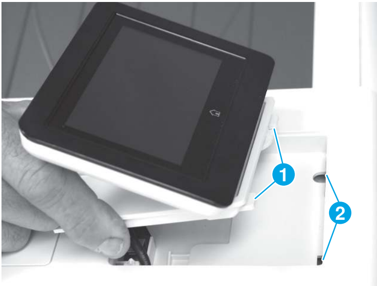
Figure 5-83 Install the control panel
