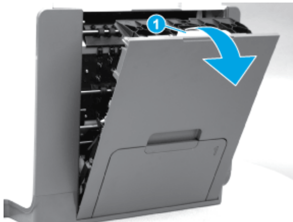
Figure 5-87 Open the left door
