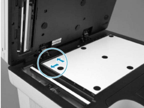
Figure 5-299 Place the white backing on the glass
