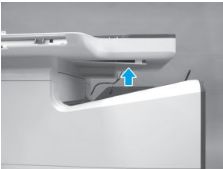
Figure 5-385 Install the cover
