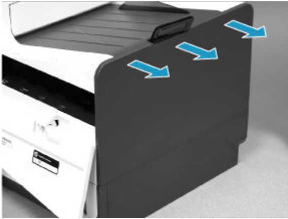
Figure 5-422 Release the right cover (outer)
