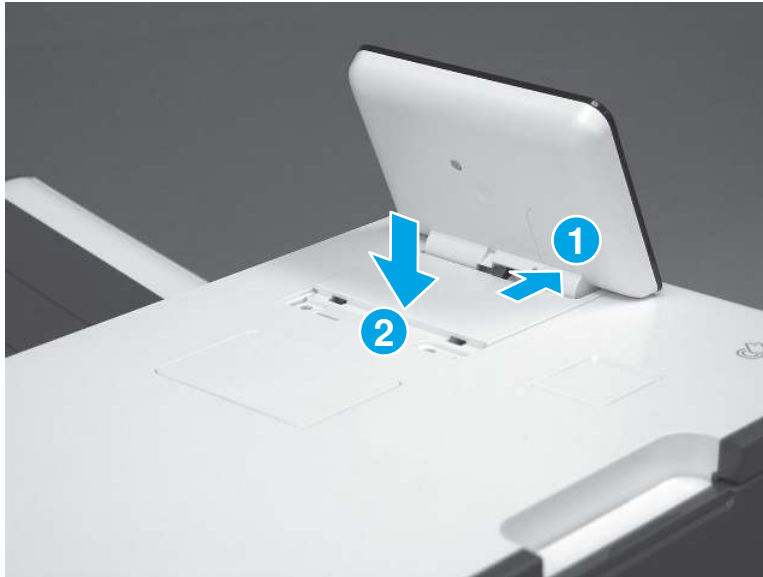
Figure 5-84 Rotate the control-panel base down
