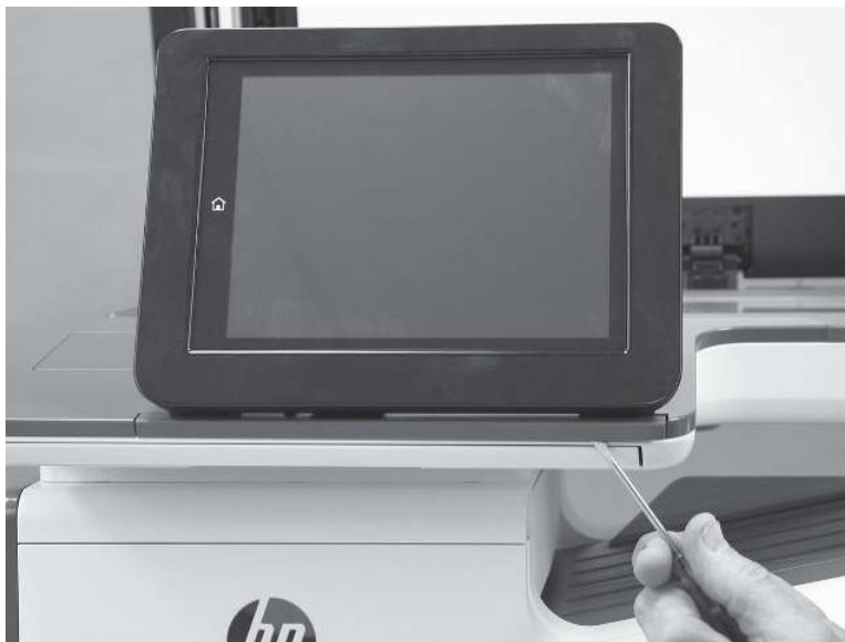
Figure 5-183 Release the small gray plastic cover
