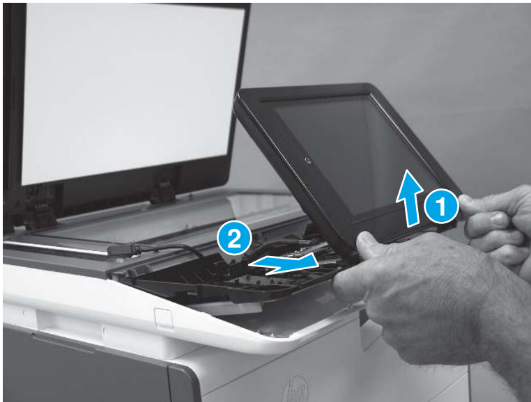
Figure 5-191 Remove the control panel
