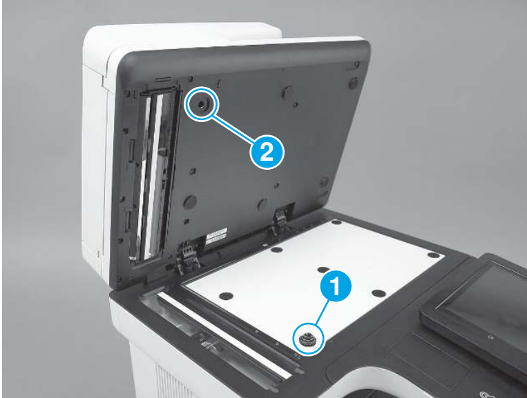
Figure 5-16 Check the retention clips
