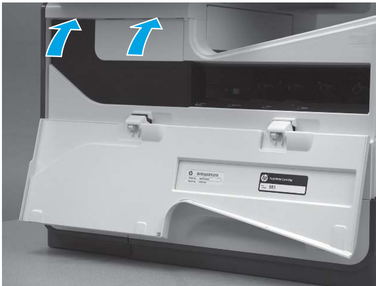
Figure 5-626 Close the blank cover
