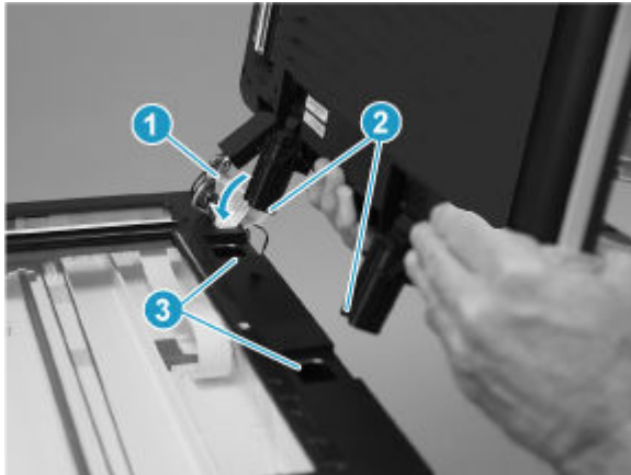
Figure 5-391 Align the hinges
