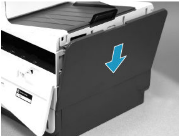
Figure 5-131 Position the right cover (outer) on the printer
