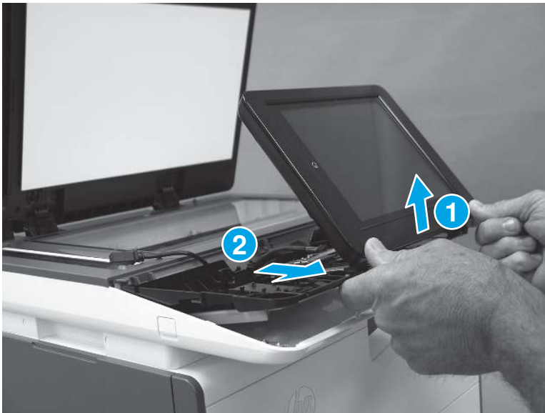
Figure 5-142 Remove the control panel
