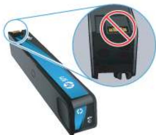
Figure 4-71 Examine the ink cartridge
