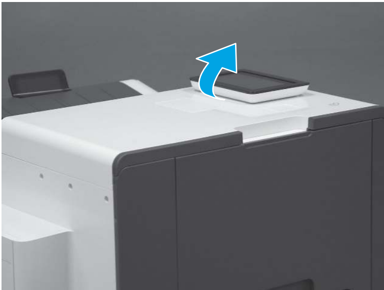
Figure 5-503 Tilt the control panel up
