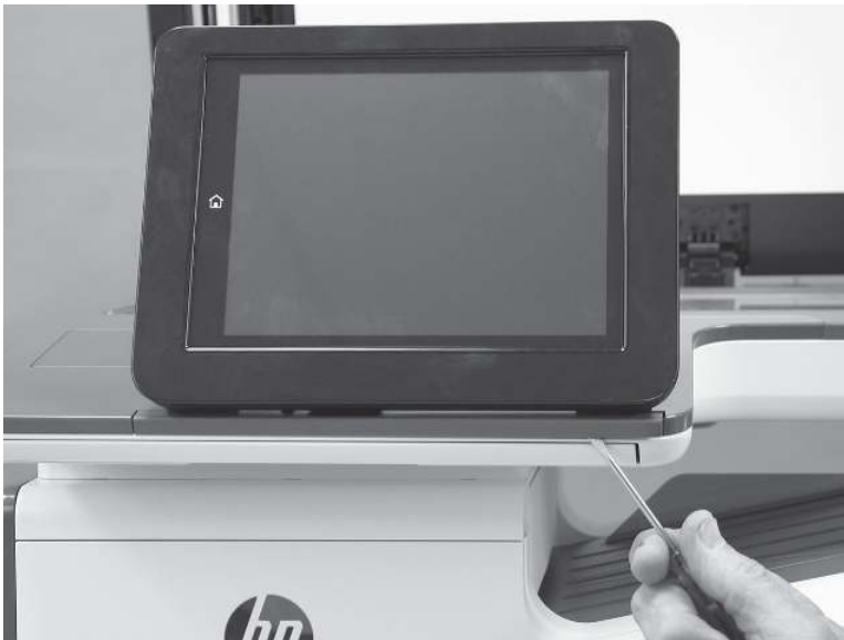
Figure 5-51 Release the small gray plastic cover
