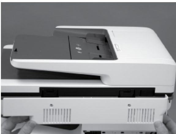
Figure 5-608 Align the tabs on the SCB cover
