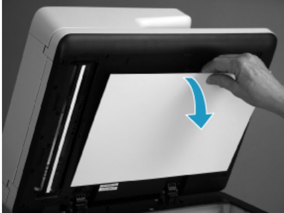
Figure 5-338 Remove the white backing
