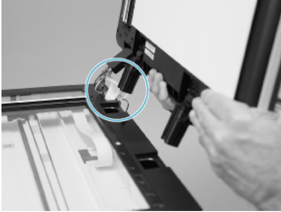
Figure 5-292 Remove the document feeder
