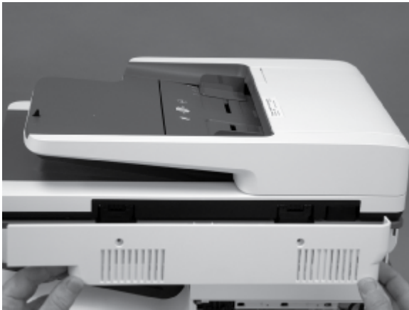
Figure 5-99 Align the SCB cover tabs and printer slots
