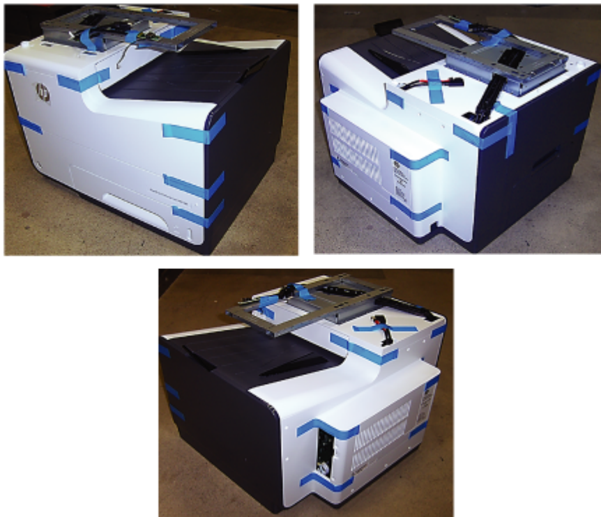
Figure 5-542 Remove the shipping tape
