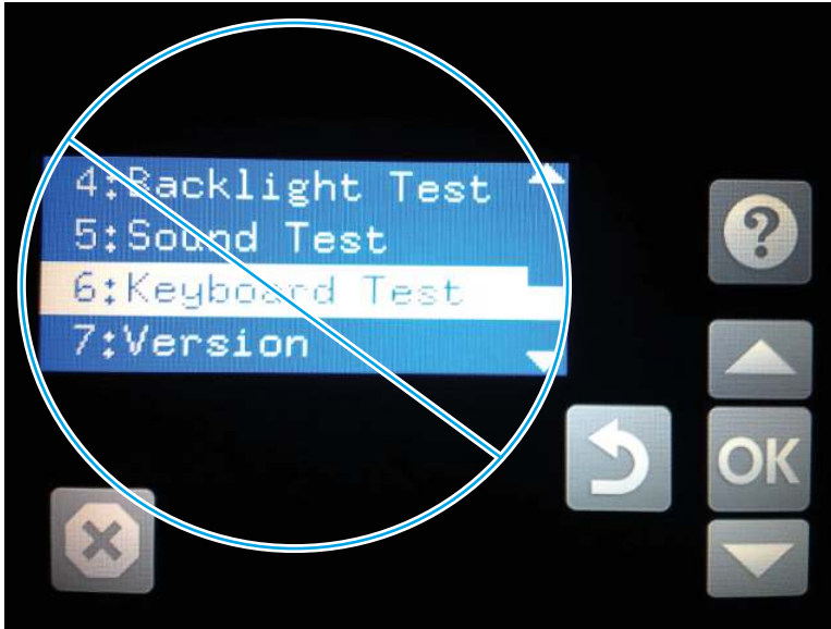
Figure 4-64 Open the keyboard test
