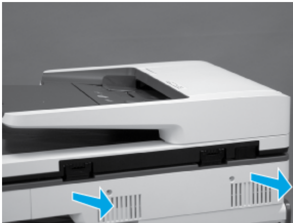
Figure 5-98 Remove the SCB cover
