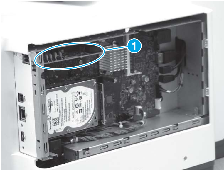
Figure 5-259 Locate the fax PCA
