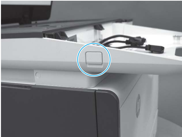
Figure 5-585 Remove the USB port cover
