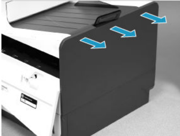
Figure 5-159 Release the right cover (outer)
