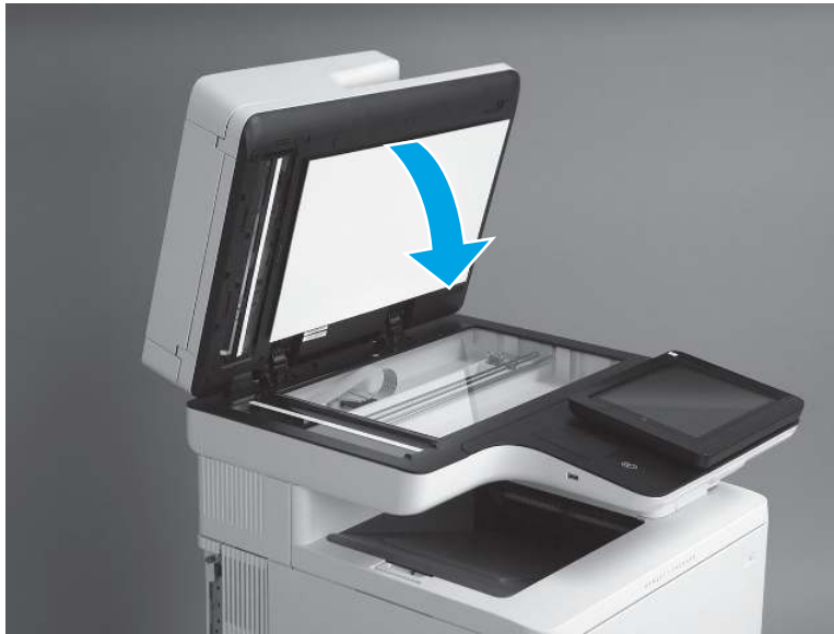
Figure 5-25 Close the document feeder
