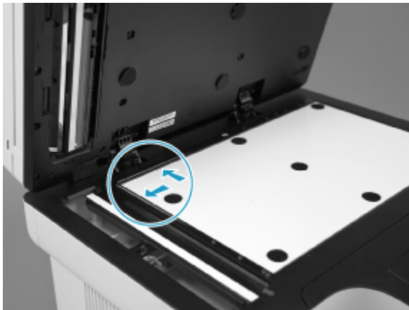
Figure 5-32 Place the white backing on the glass
