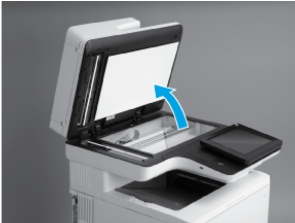
Figure 5-34 Check the white backing
