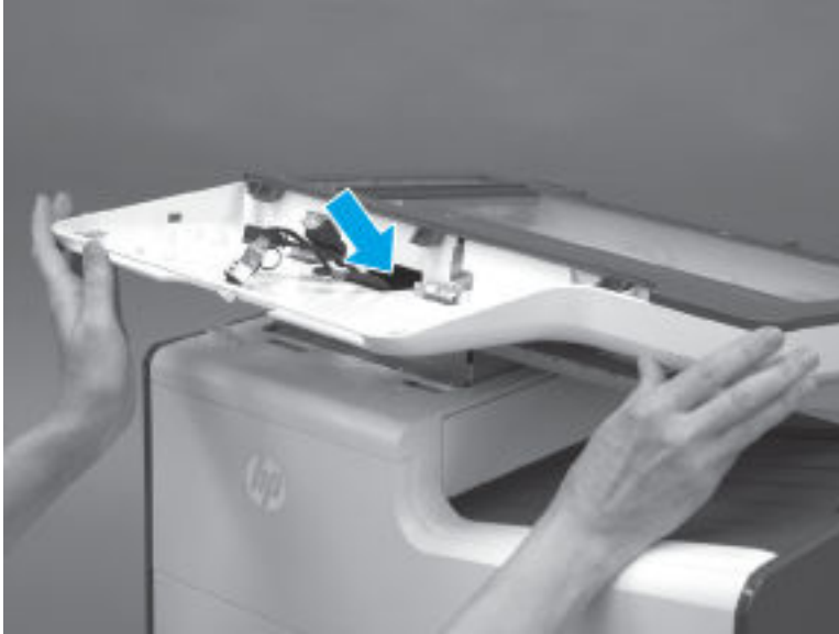
Figure 5-377 Pass the wire harnesses and cables through the opening
