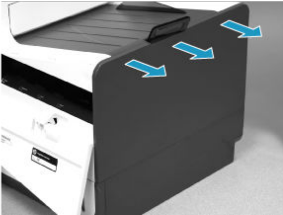
Figure 5-104 Release the right cover (outer)
