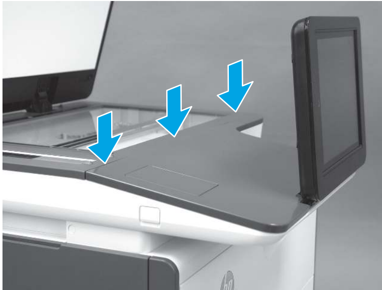
Figure 5-49 Engage three bosses
