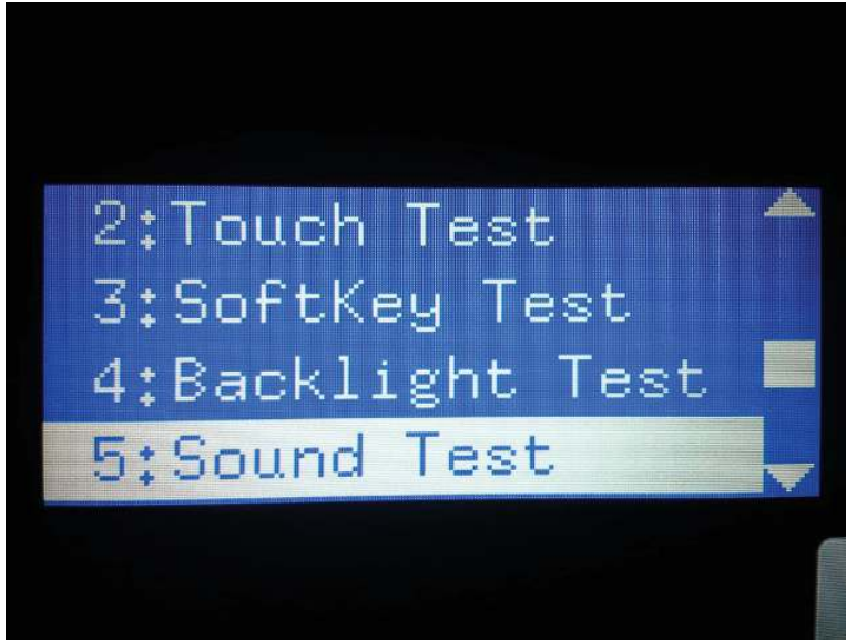
Figure 4-63 Open the sound test
