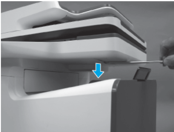
Figure 5-151 Release the cover
