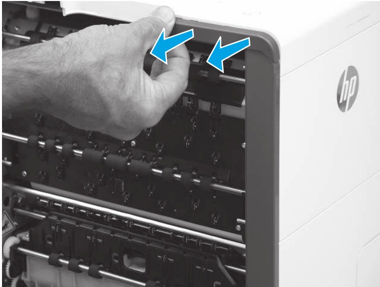
Figure 5-205 Remove left-rear top cover cap (556)
