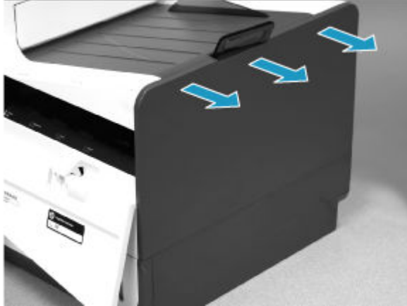
Figure 5-479 Release the right cover (outer)
