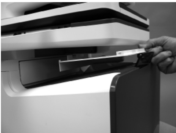
Figure 5-152 Remove the scanner base cover
