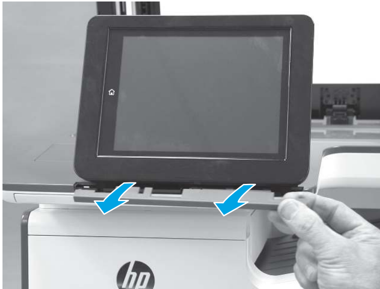
Figure 5-135 Remove the cover
