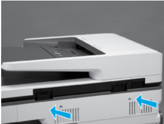
Figure 5-297 Install the SCB cover
