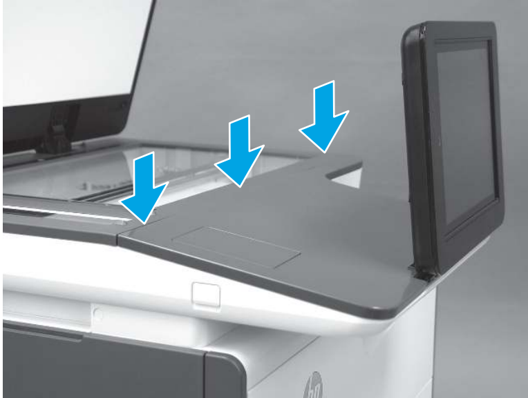
Figure 5-621 Install the control-panel cover
