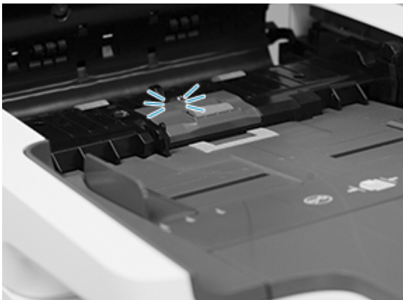
Figure 5-704 Push down on the roller cover
