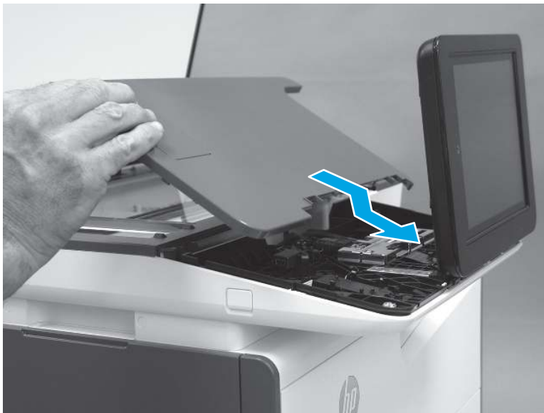
Figure 5-620 Install the cover
