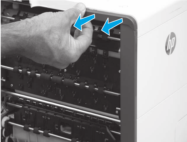
Figure 5-114 Remove left-front top cover cap (556)
