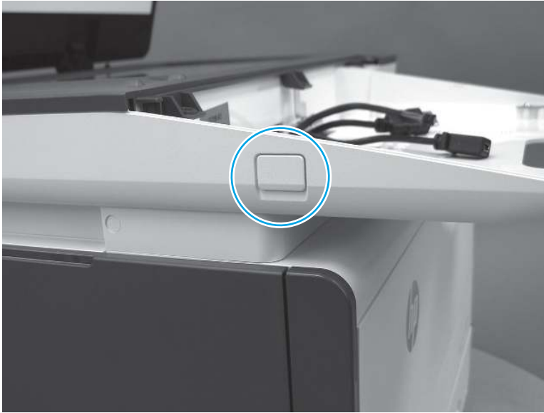
Figure 5-369 Remove the USB port cover
