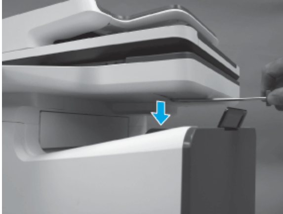
Figure 5-593 Release the cover
