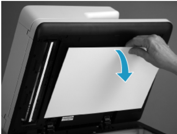
Figure 5-15 Remove the white backing
