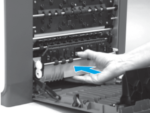
Figure 5-651 Install a new ink collection unit
