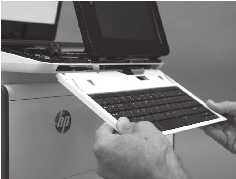
Figure 5-57 Remove the keyboard
