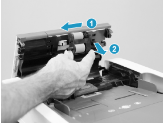
Figure 5-697 Remove the roller assembly
