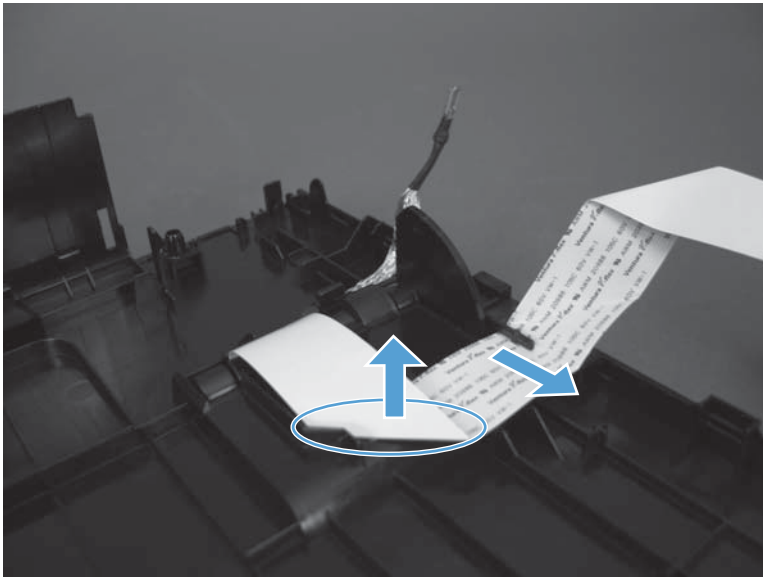
Figure 1-34 Remove the touchscreen control-panel (1 of 2)
