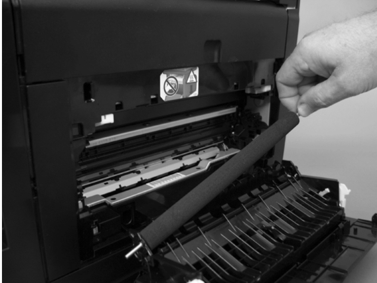
Figure 1-8 Remove the transfer roller (3 of 3)
