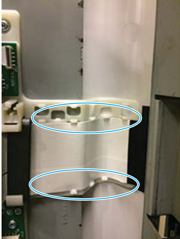
Figure 1-9 FFC pill bump retainers
