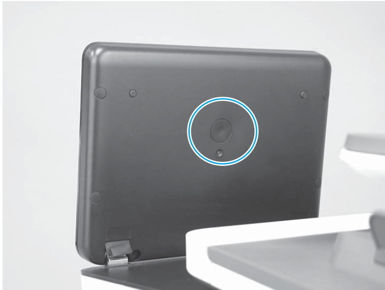
Figure 2-5 Press the diagnostics-access button (780/785 printers)
