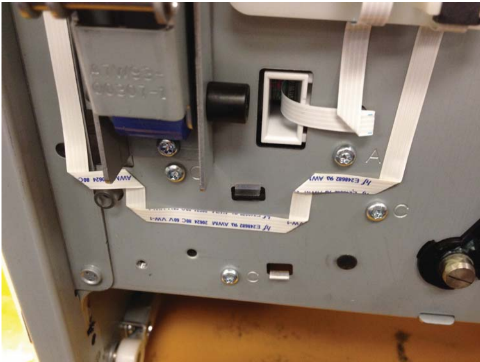
Figure 1-11 FFC double-sided tape retainer
