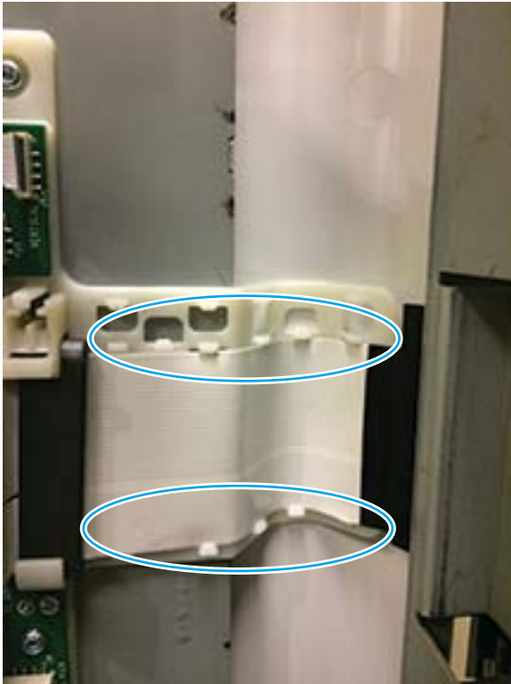
Figure 1-42 FFC pill bump retainers
