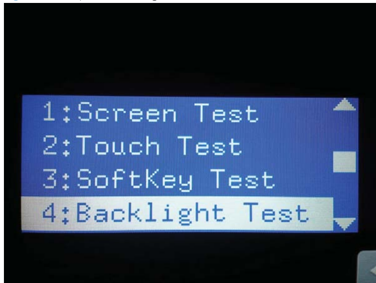
Figure 2-20 Open the backlight test
