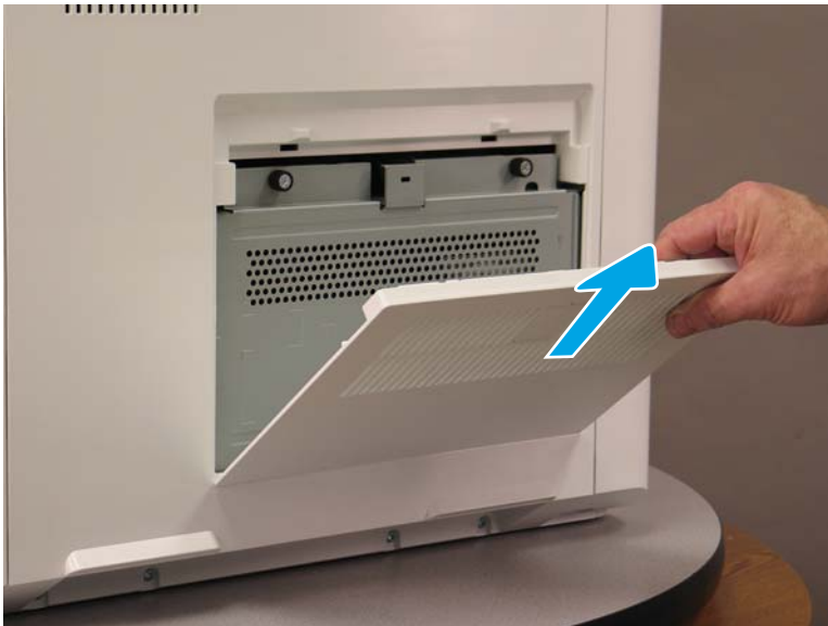
Figure 1-2424 Remove the formatter cover
