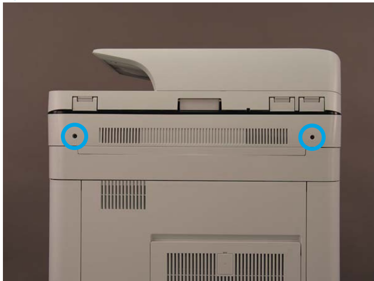
Figure 1-524 Remove two screws
