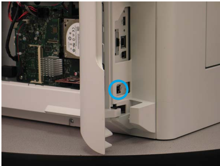
Figure 1-1325 Locate the slot in the sheet metal
