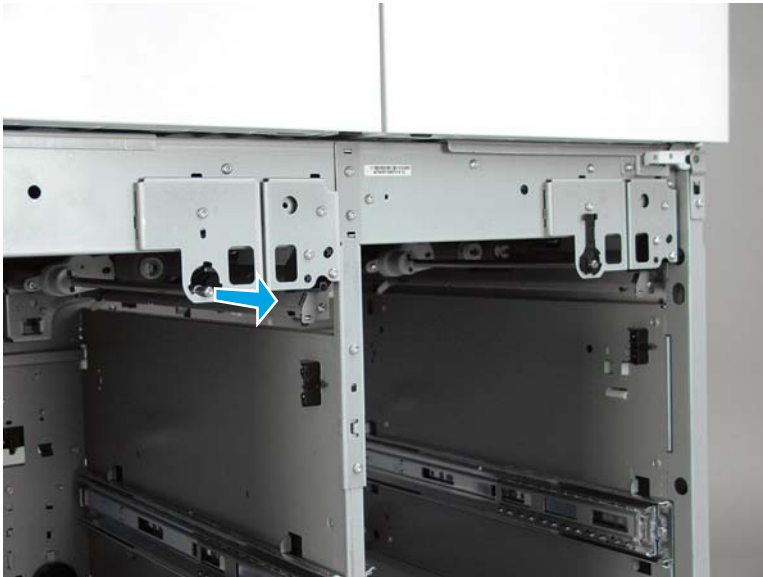
Figure 1-2605 Pull the shaft out
