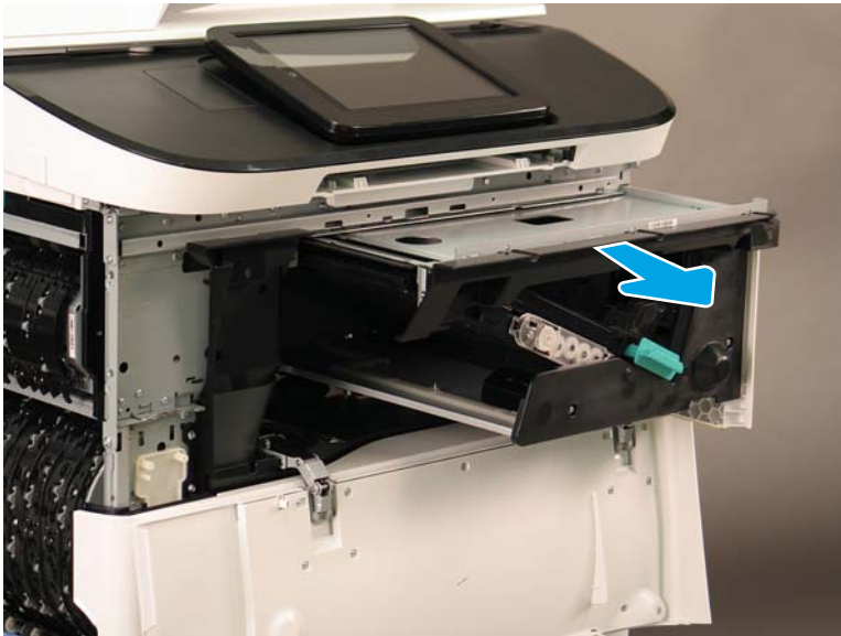
Figure 1-730 Remove the bridge assembly
