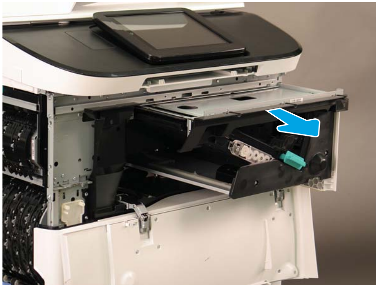
Figure 1-691 Remove the bridge assembly
