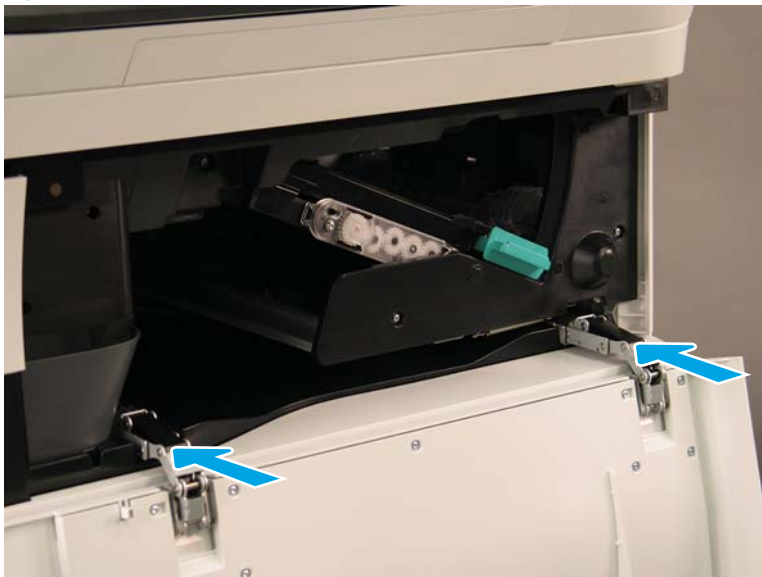
Figure 1-2031 Release the door hinges
