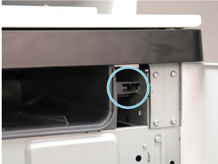
Figure 1-2055 Check the output bin installation
