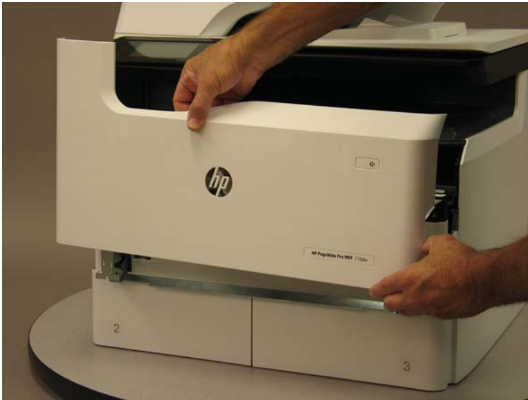
Figure 1-967 Remove the cartridge door
