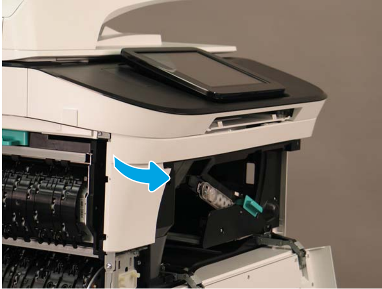
Figure 1-383 Rotate the left edge of the cover out
