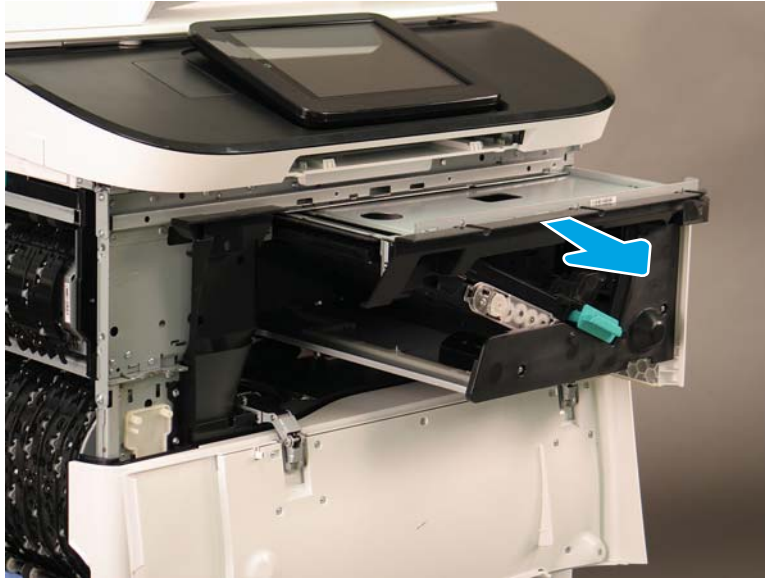
Figure 1-610 Remove the bridge assembly
