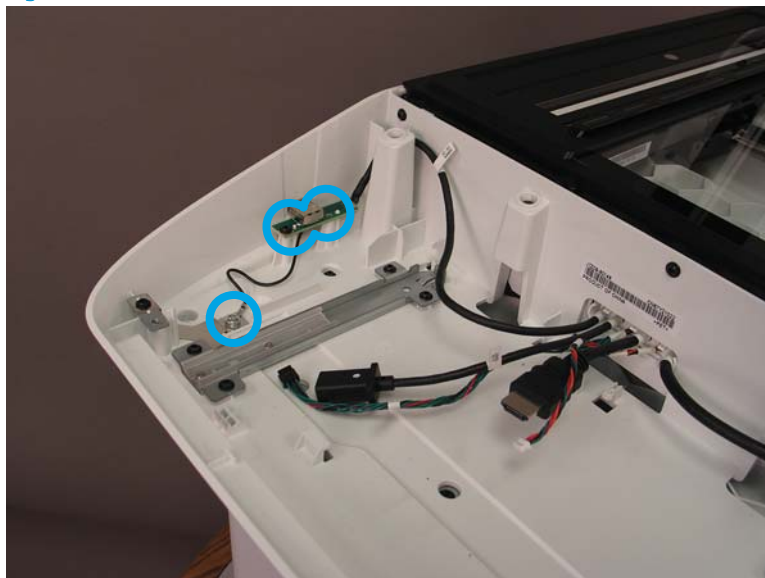
Figure 1-517 Release the USB PCA (1 of 2) (785/E776)
