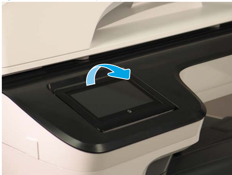
Figure 1-435 Tilt the control panel up
