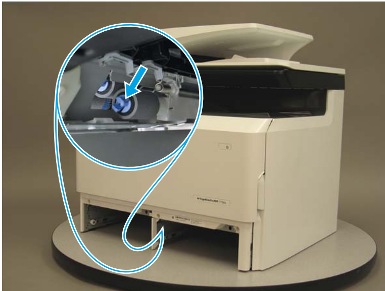
Figure 1-120 Remove the separation roller (A4 Tray 2)
