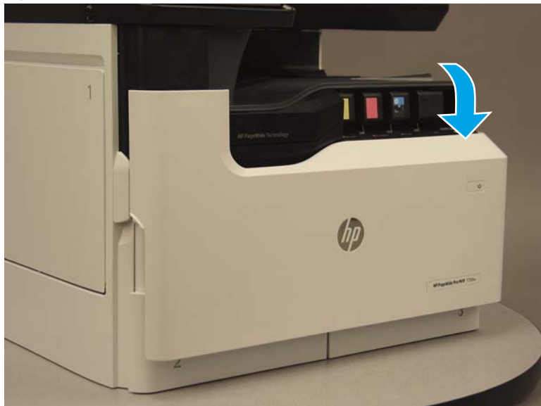
Figure 1-964 Open the cartridge door
