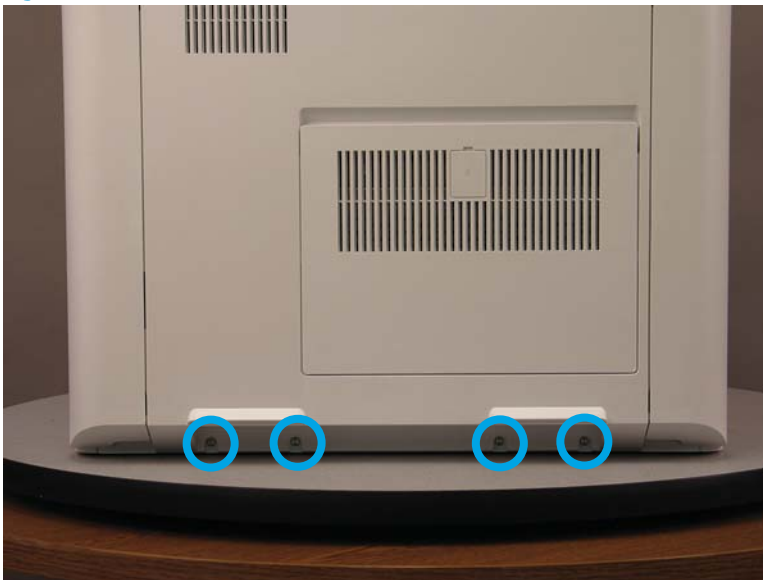
Figure 1-2275 Remove four screws
