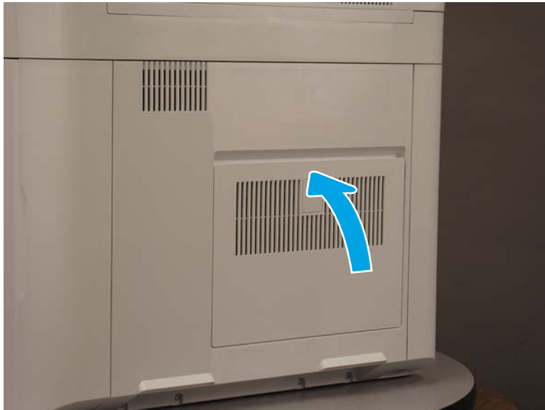
Figure 1-1336 Install the formatter cover
