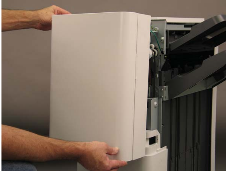
Figure 1-3473 Remove the front door assembly
