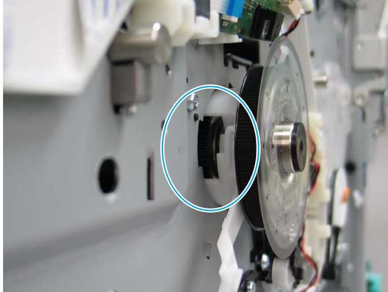
Figure 1-1085 Note the clip on the bearing surface
