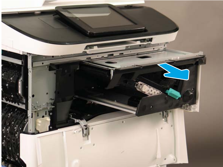
Figure 1-1742 Remove the bridge assembly
