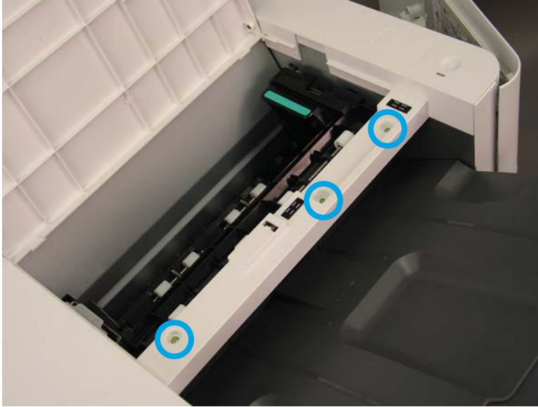
Figure 1-3744 Remove three screws (top side)
