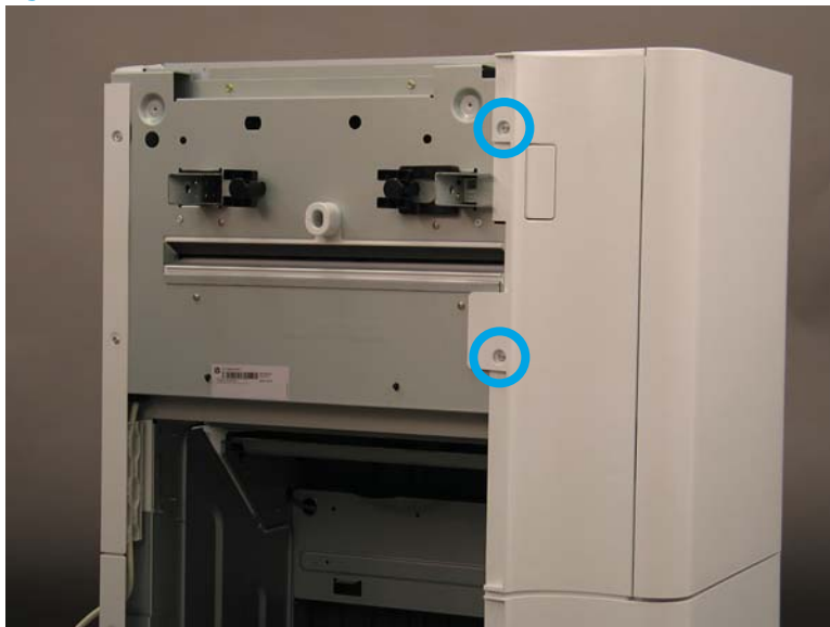
Figure 1-3771 Remove two screws (left side)
