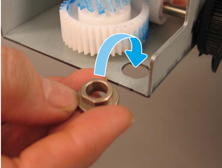
Figure 1-3935 Install the bushing
