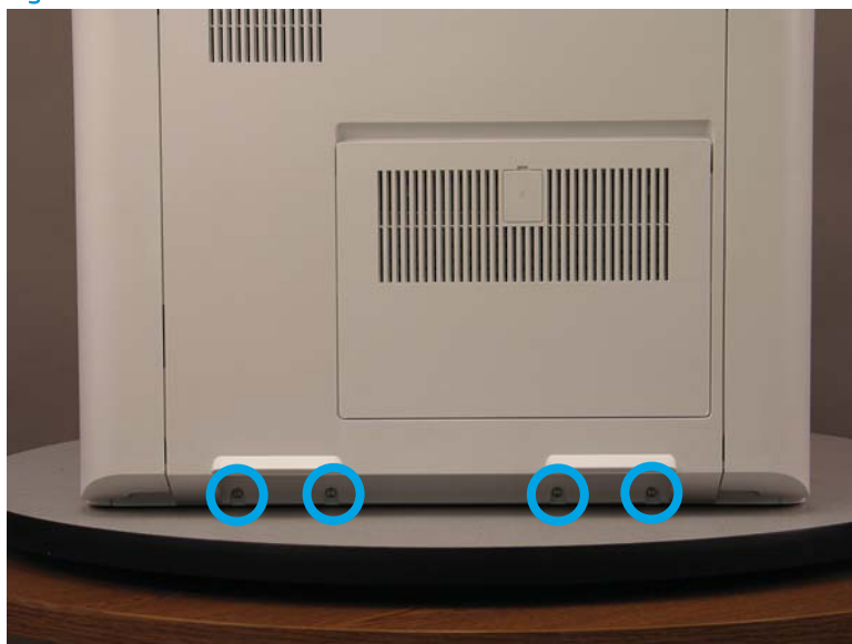
Figure 1-1394 Remove four screws
