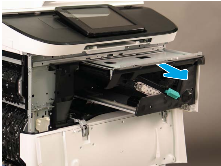
Figure 1-386 Remove the bridge assembly
