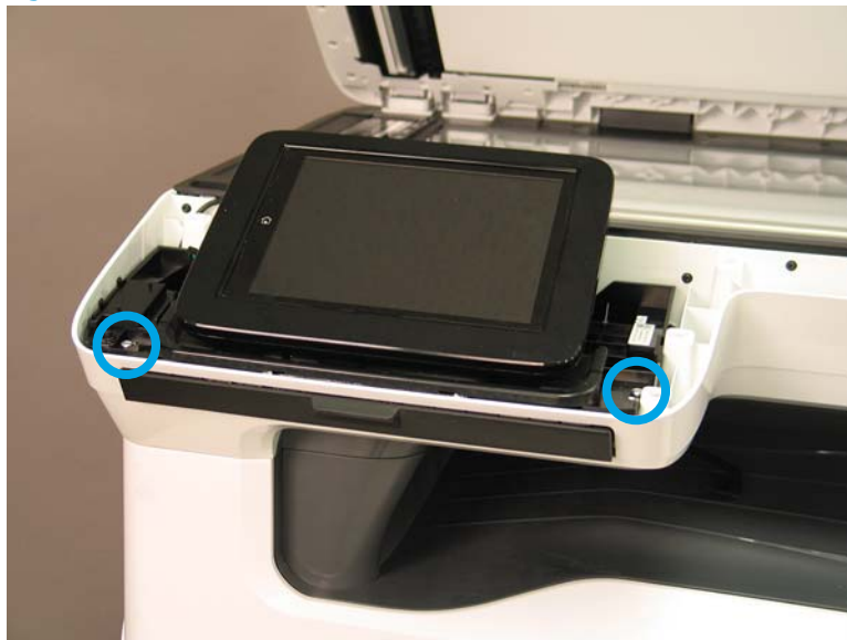
Figure 1-240 Remove two screws
