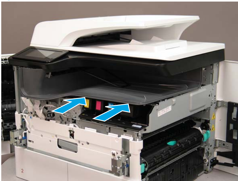
Figure 1-2054 Install the output bin
