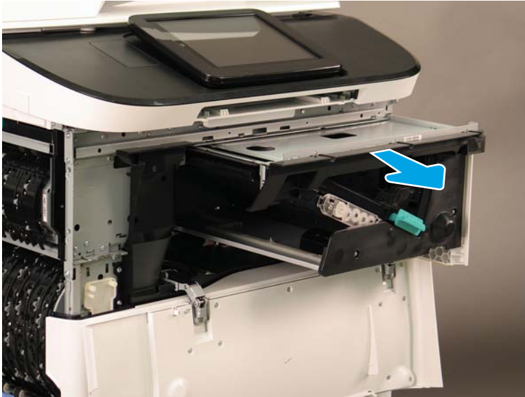
Figure 1-1837 Remove the bridge assembly
