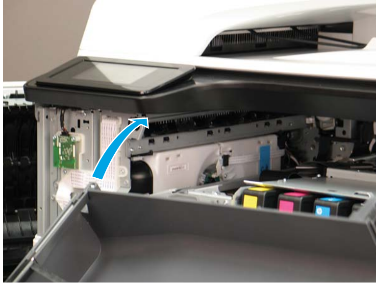
Figure 1-2107 Align the mounting rails
