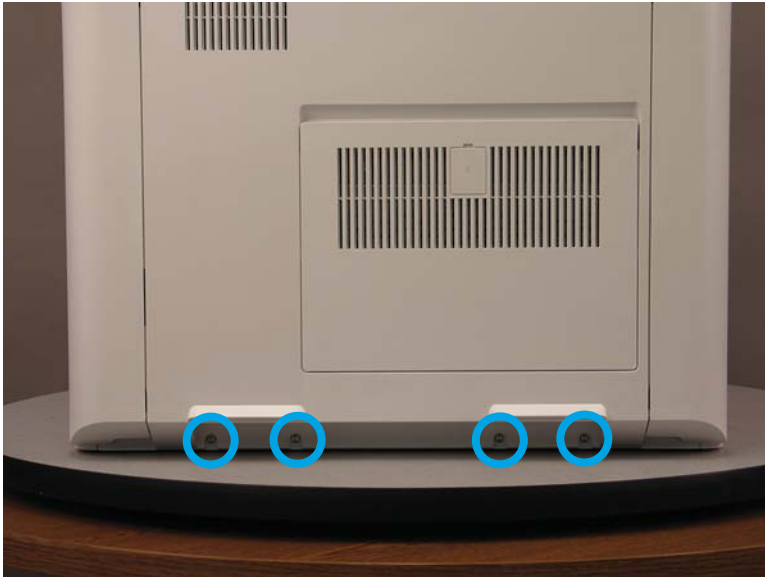
Figure 1-352 Remove four screws
