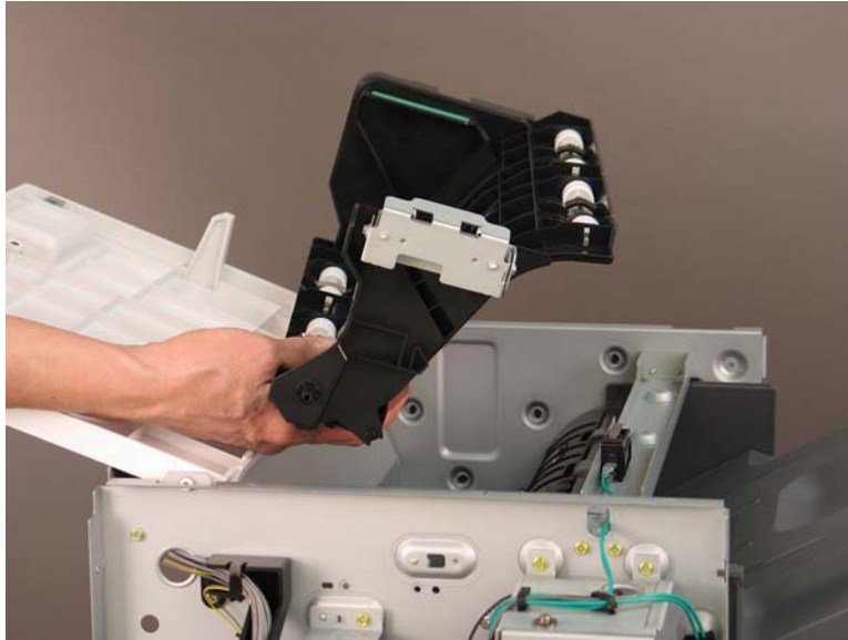
Figure 1-3540 Remove the top jam access cover
