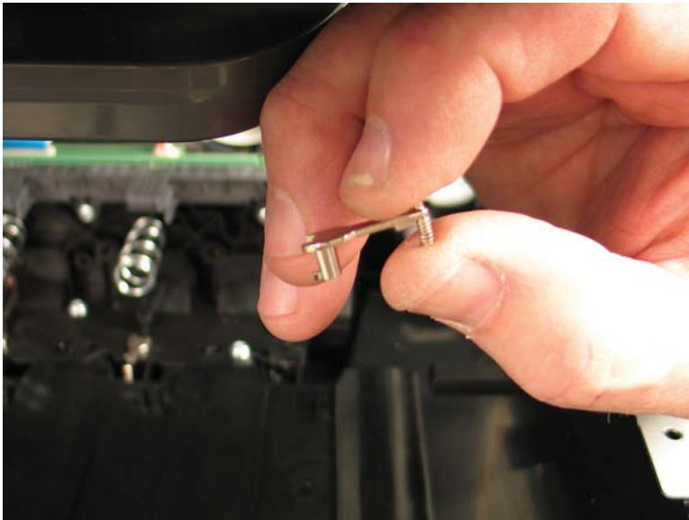
Figure 1-2061 Remove the cartridge latch(es) and spring(s)
