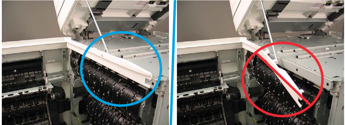
Figure 1-2903 Do not use the left-side cover as a hand hold
