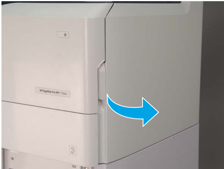
Figure 1-2573 Open the printer right door
