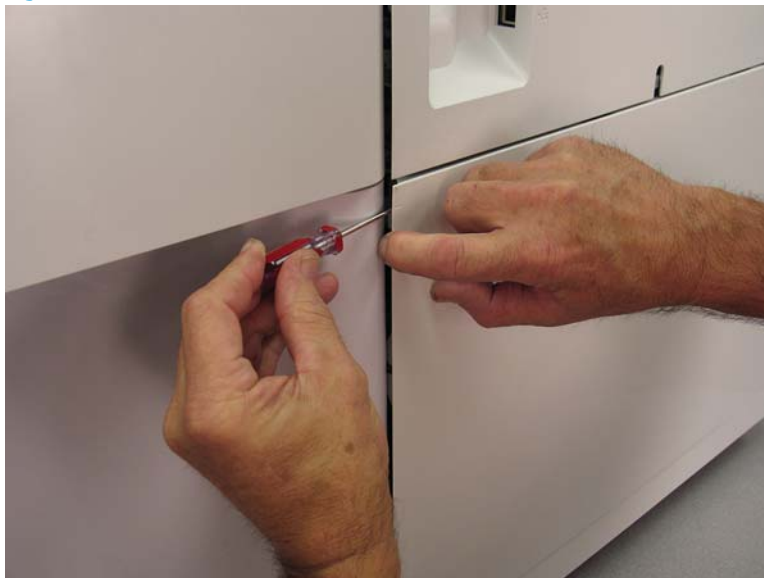
Figure 1-2550 Release the rear cover
