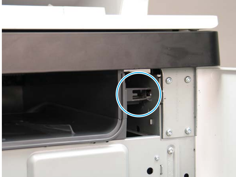
Figure 1-2111 Check the output bin installation
