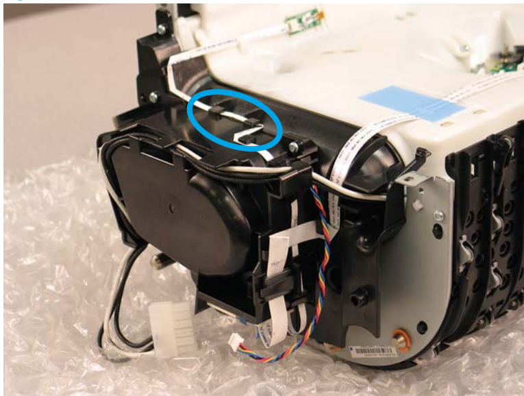
Figure 1-1895 Release the FFC
