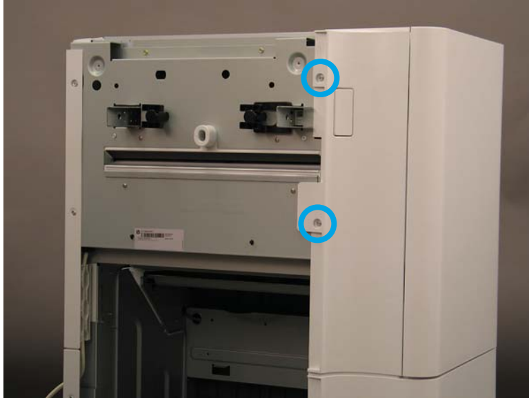
Figure 1-3497 Remove two screws (left side)
