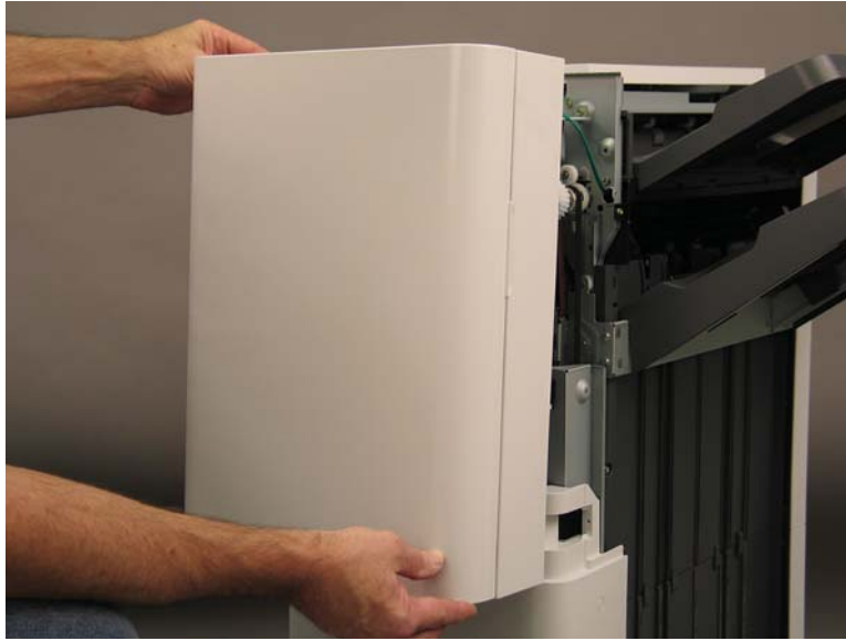
Figure 1-3213 Remove the front door assembly
