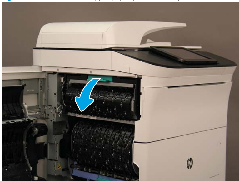
Figure 1-1763 Rotate the upper paper path assembly down
