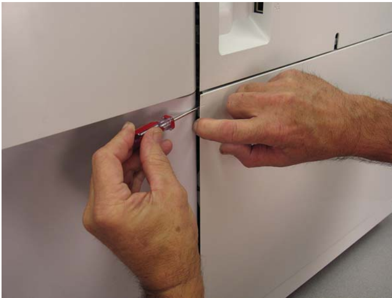
Figure 1-2636 Release the rear cover
