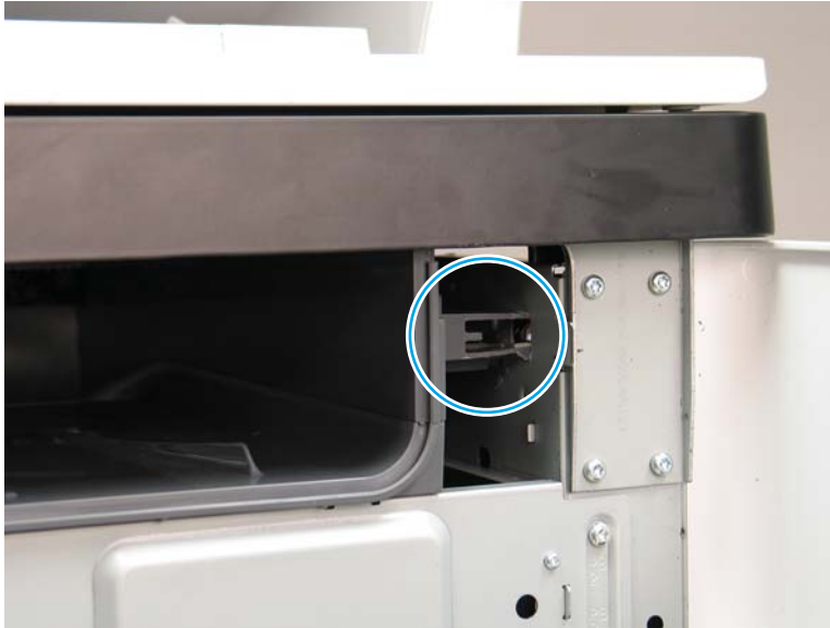
Figure 1-2252 Check the output bin installation
