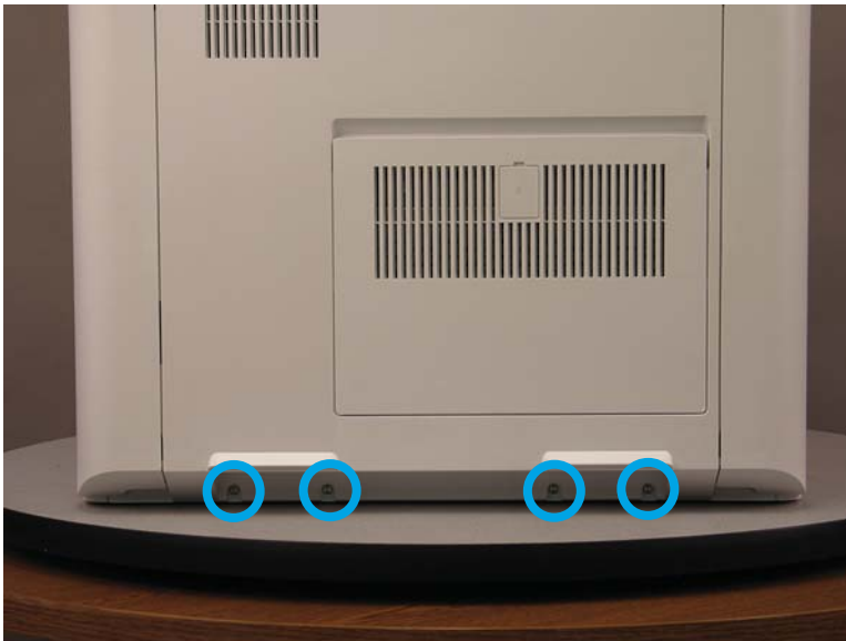
Figure 1-2214 Remove four screws
