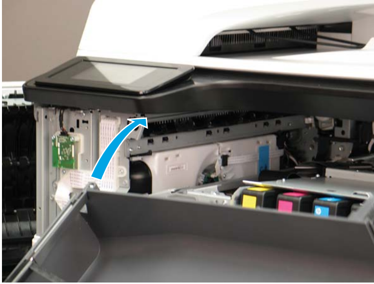
Figure 1-2309 Align the mounting rails
