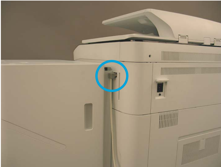
Figure 1-3168 Disconnect finisher connector
