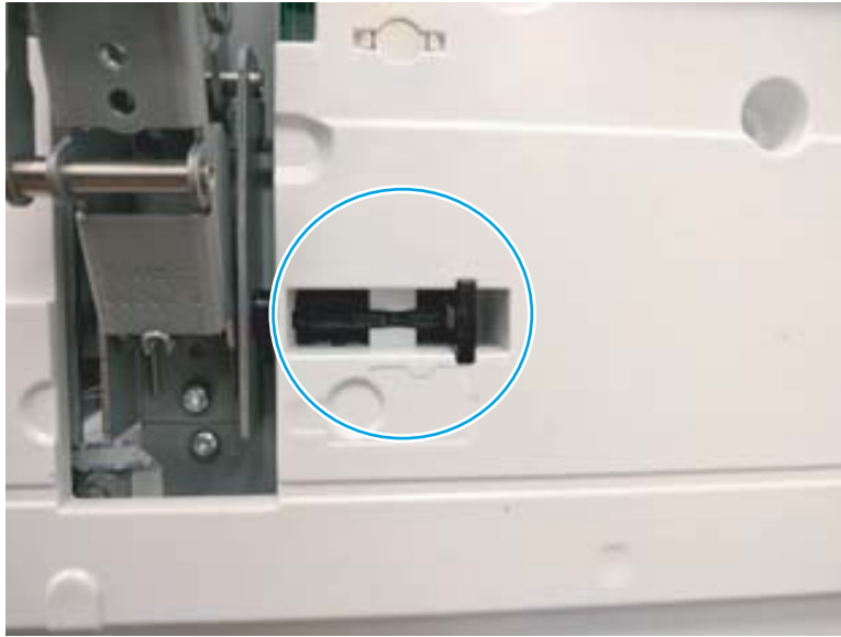
Figure 1-1039 Locate the cover lock feature
