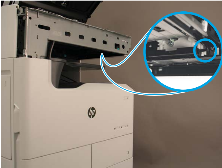
Figure 1-1688 Check the clamp drive bar and drive
