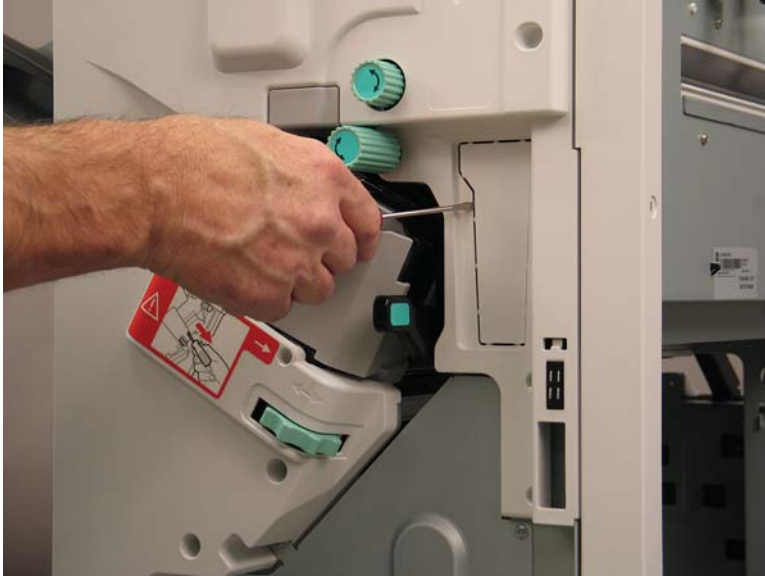
Figure 1-2458 Remove the blank cover
