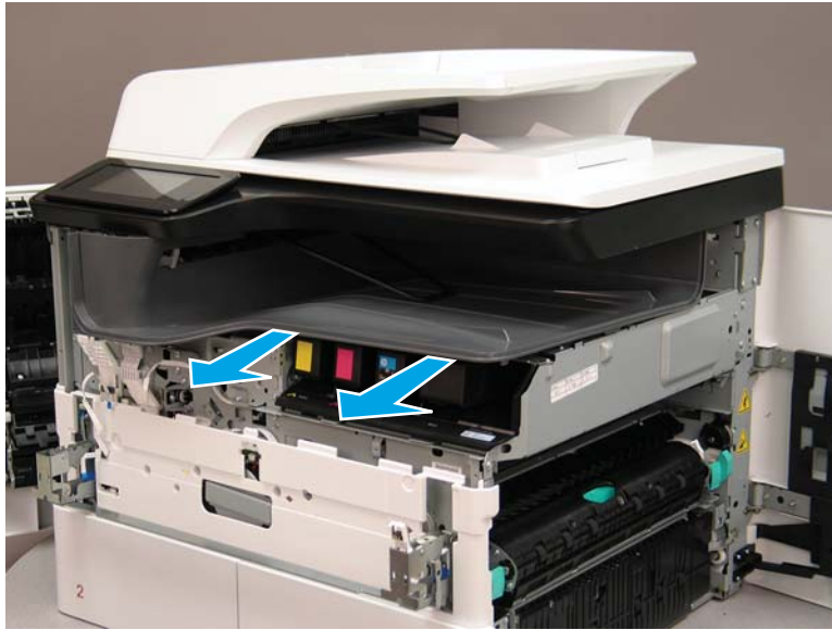
Figure 1-2047 Remove the output bin
