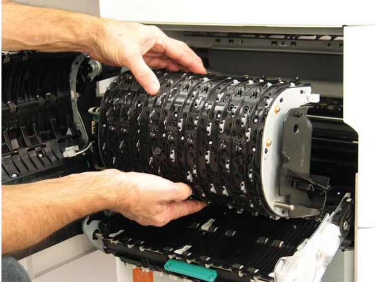
Figure 1-1892 Remove the airflow assembly
