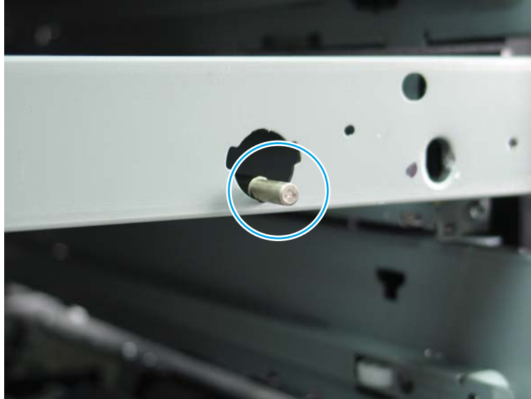
Figure 1-2561 Correct shaft install
