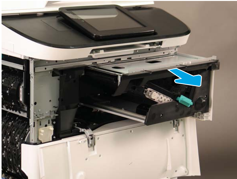
Figure 1-752 Remove the bridge assembly
