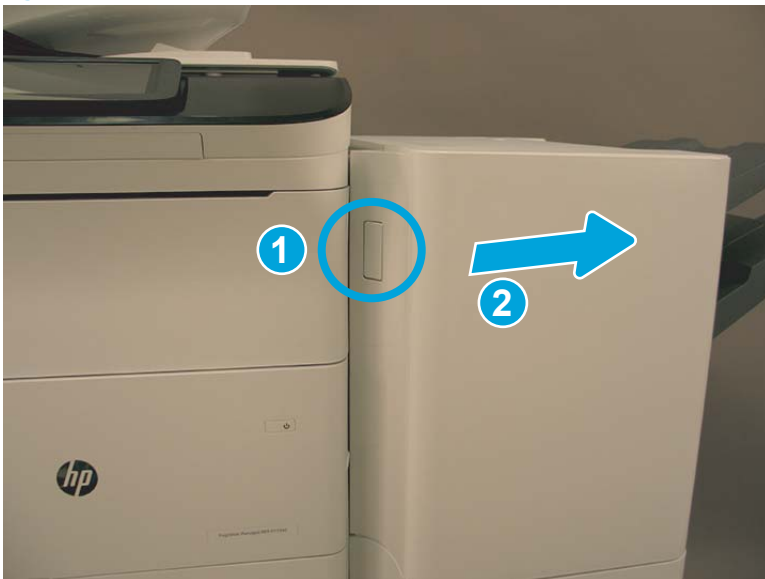
Figure 1-3916 Separate the finisher from the printer
