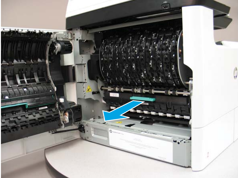
Figure 1-1885 Pull the service fluid container out
