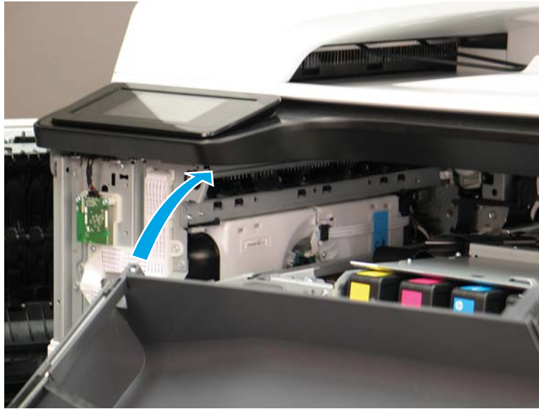
Figure 1-2051 Align the mounting rails
