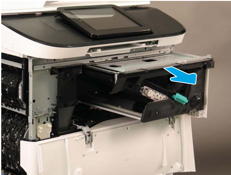
Figure 1-2042 Remove the bridge assembly
