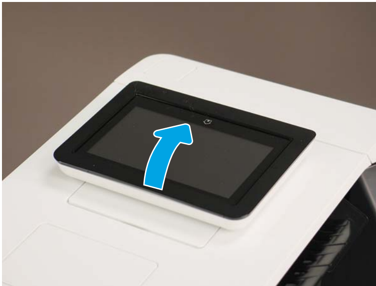
Figure 1-82 Tilt the control panel up (1 of 2)
