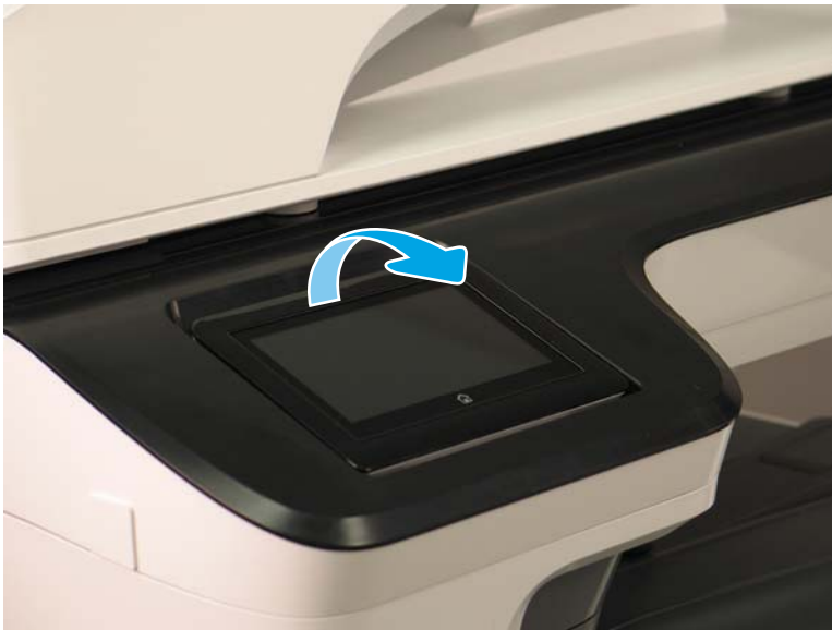
Figure 1-230 Tilt the control panel up
