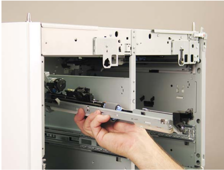
Figure 1-2618 Remove the separation assembly
