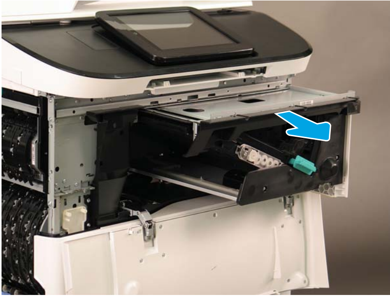
Figure 1-624 Remove the bridge assembly
