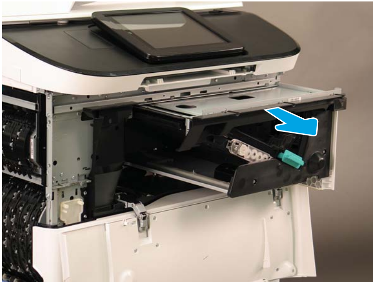
Figure 1-2374 Remove the bridge assembly
