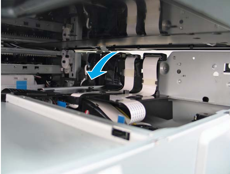
Figure 1-2000 Rotate the FFC guide down
