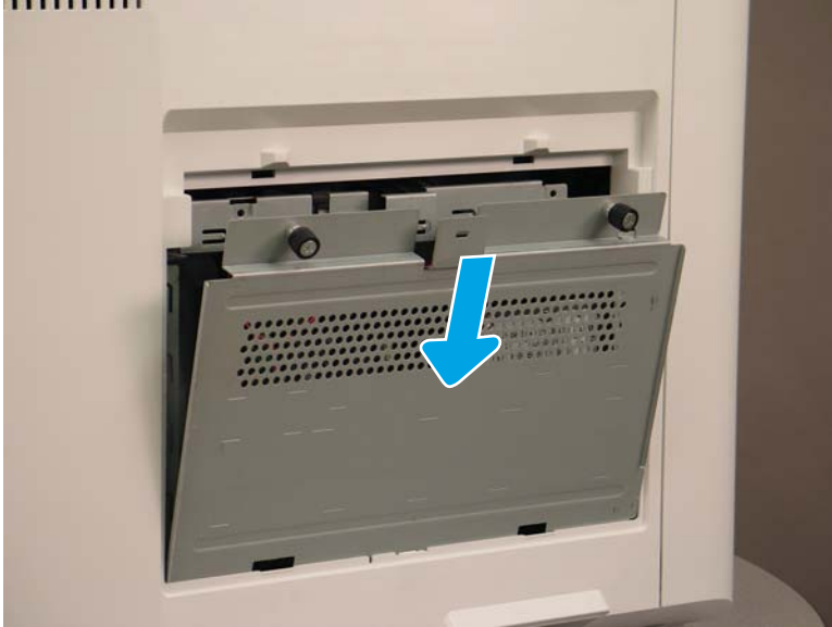
Figure 1-1333 Install the formatter cage cover
