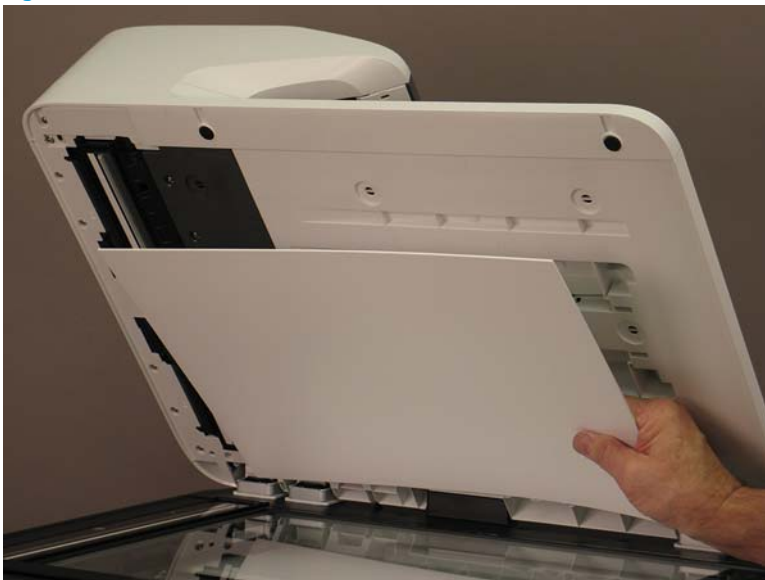
Figure 1-151 Remove the reflector
