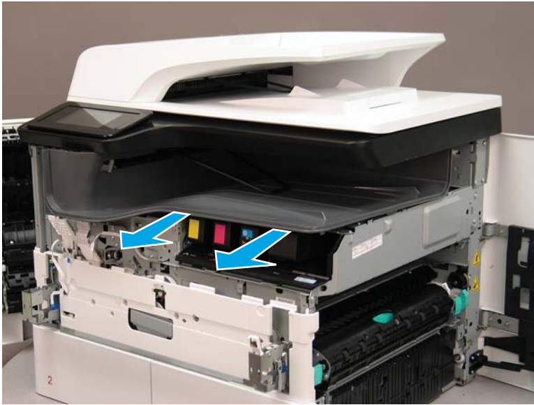
Figure 1-391 Remove the output bin
