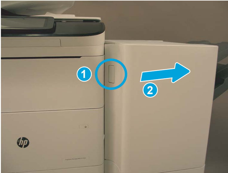
Figure 1-2439 Separate the finisher from the printer
