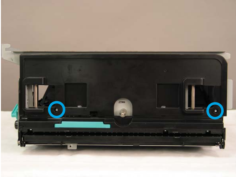
Figure 1-717 Remove two screws
