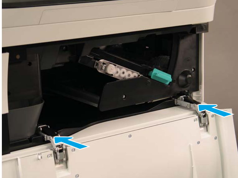
Figure 1-286 Release the door hinges
