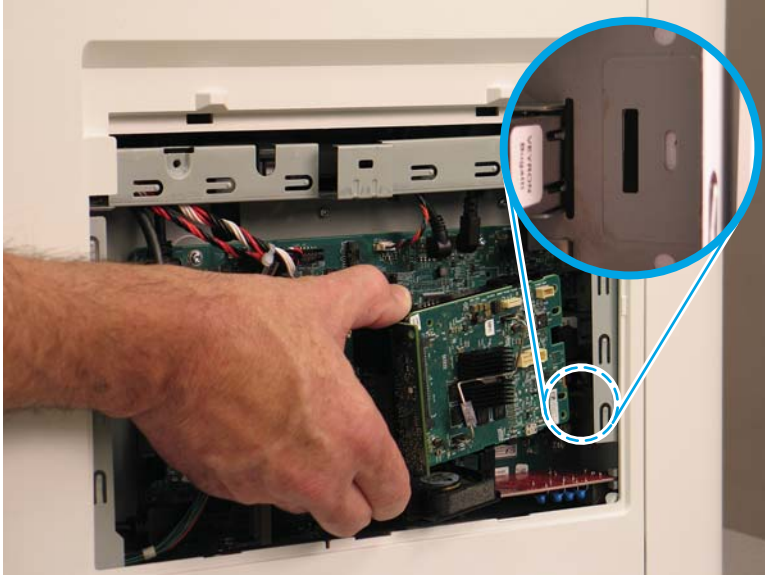
Figure 1-62 Locate the slot in the sheet metal
