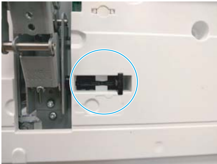
Figure 1-1104 Locate the cover lock feature
