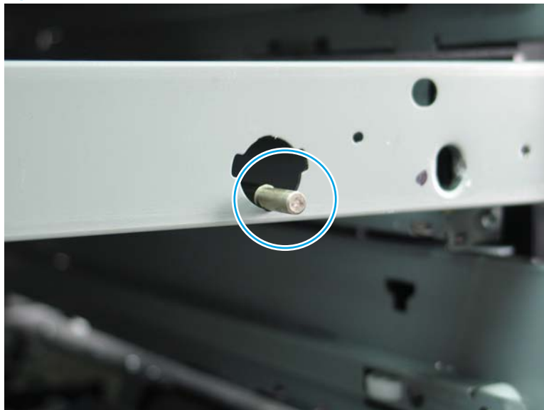
Figure 1-2547 Correct shaft install
