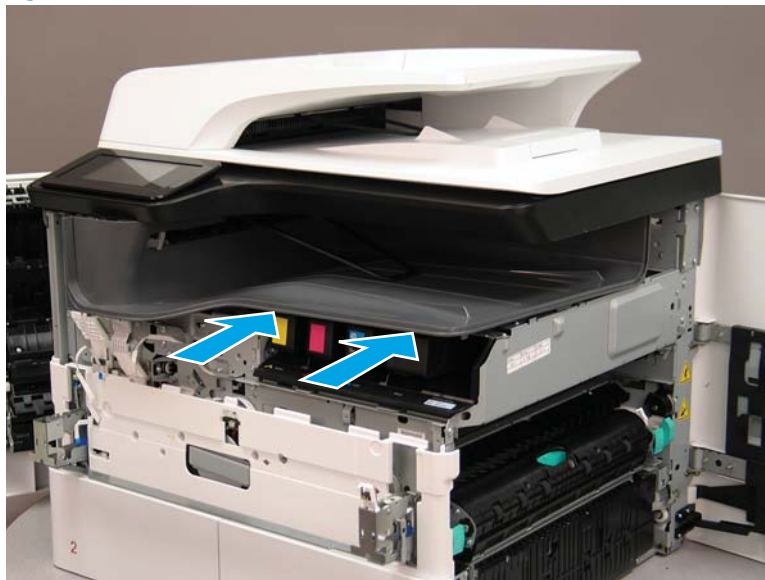
Figure 1-2192 Install the output bin
