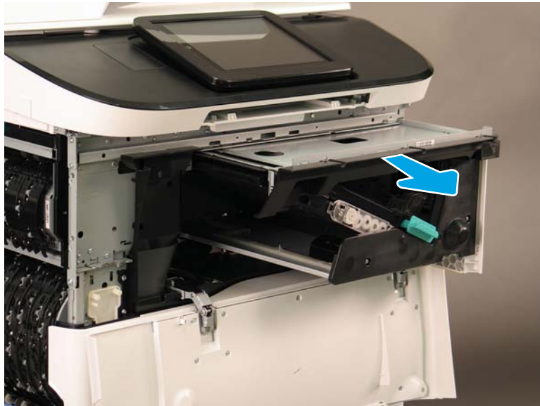
Figure 1-2180 Remove the bridge assembly
