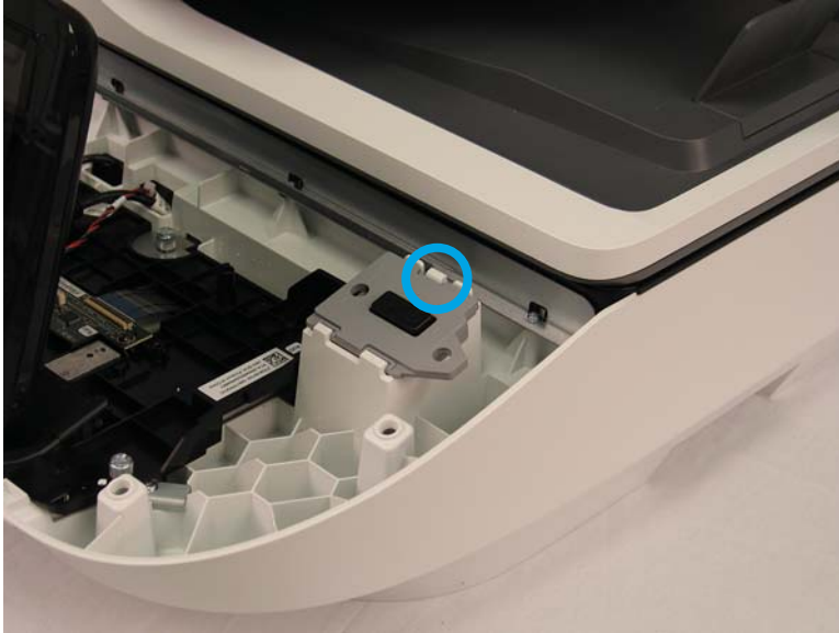
Figure 1-132 Remove the power button assembly (1 of 3)
