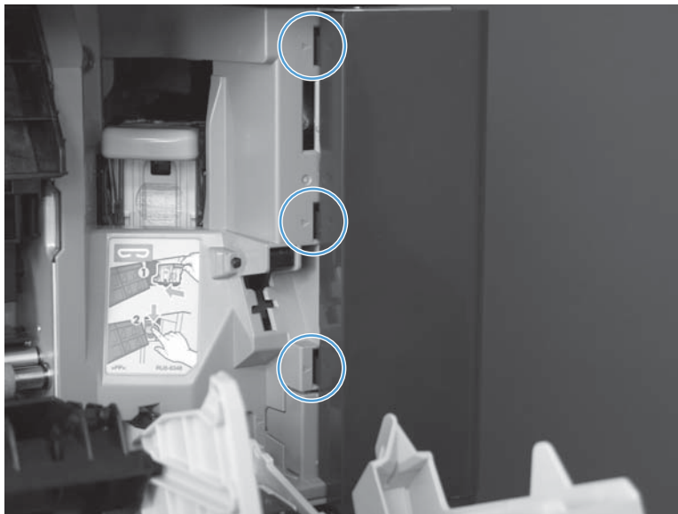
Figure 1-105 Remove the stapler/stacker rear cover (2 of 3)
