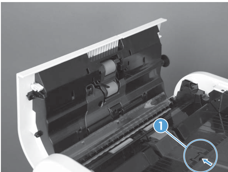
Figure 1-52 Remove the document feeder separation pad (2 of 3)
