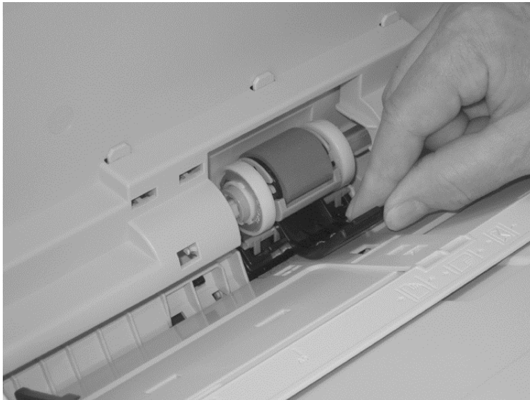
Figure 1-38 Remove the Tray 1 separation pad (4 of 4)
