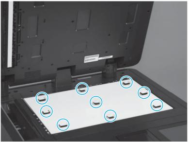
2. Make sure that the arrow on the replacement white backing is positioned in the upper-left corner of the scanner glass.
