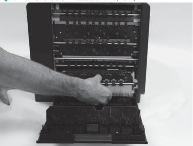
Figure 1-3 Remove the ink collection unit (2 of 2)
