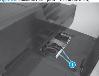
Figure 1-32 Remove the control panel — X585 models (2 of 4)
