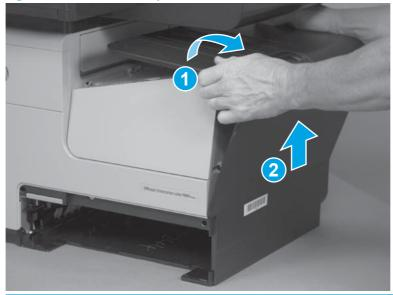
$-\frac{1}{2}$  **Reinstallation tip** Insert the tabs on the bottom edge first, and then snap the top edge into place.
