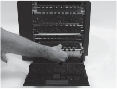
3. Unhook each restraining strap by twisting the bottom end of the strap away from the door.
