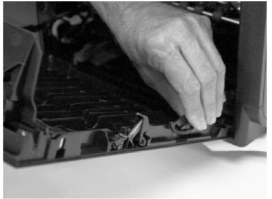
4. At the rear door hinge, the door is held in place by a retractable post. Insert a flat-blade screw driver between the door hinge and the chassis to push the post (callout 1) toward the product rear, and then pull that corner of the left door away from the product.
