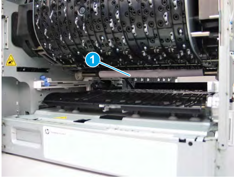
Figure 1-667 Paper wrapped around the feed shaft
