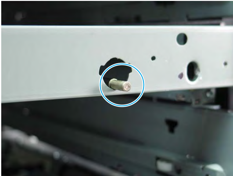
Figure 1-1764 Correct shaft install
