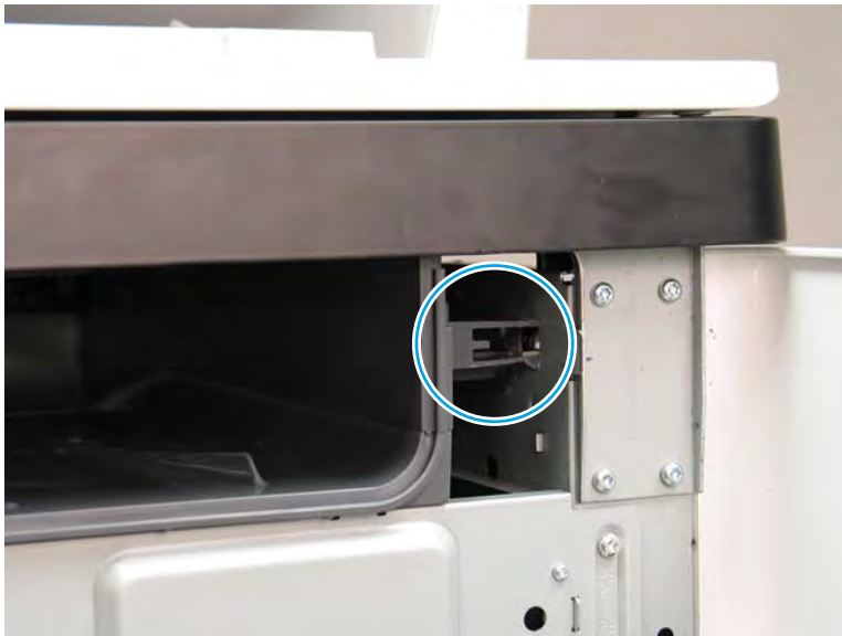
Figure 1-1664 Check the output bin installation
