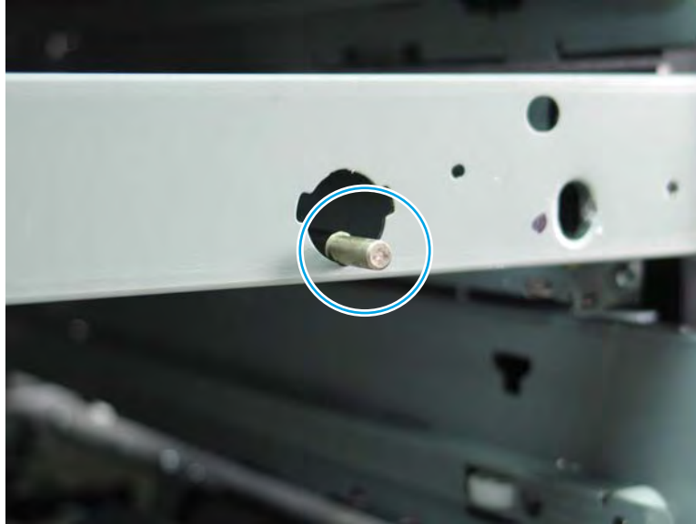
Figure 1-1772 Correct shaft install
