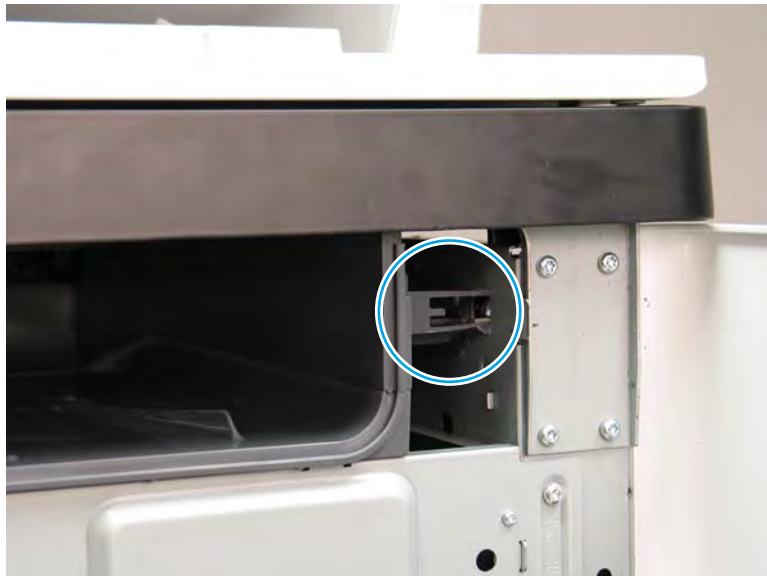
Figure 1-1605 Check the output bin installation
