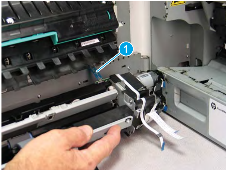
Figure 1-826 Disconnect one FFC and remove the Tray 1 separation assembly
