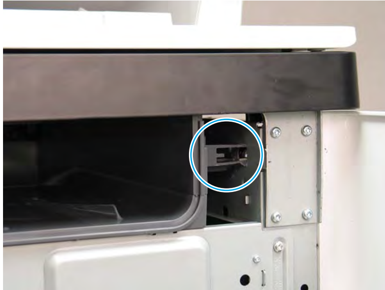
Figure 1-1421 Check the output bin installation
