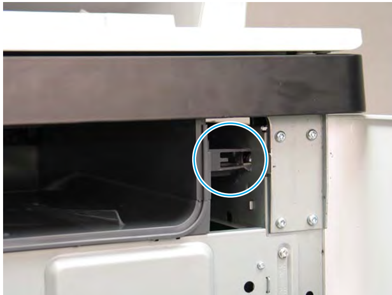
Figure 1-284 Check the output bin installation
