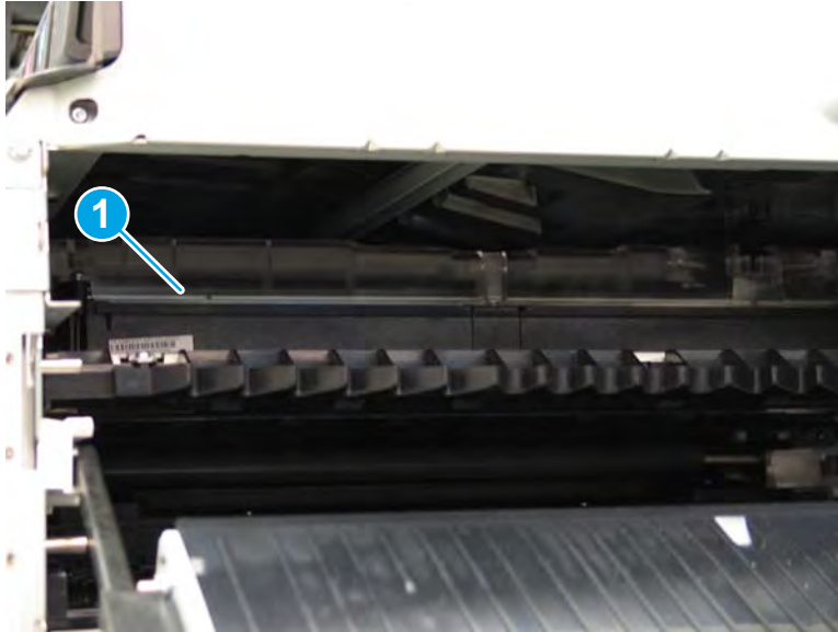
Figure 1-663 Printhead wiper in the home position
