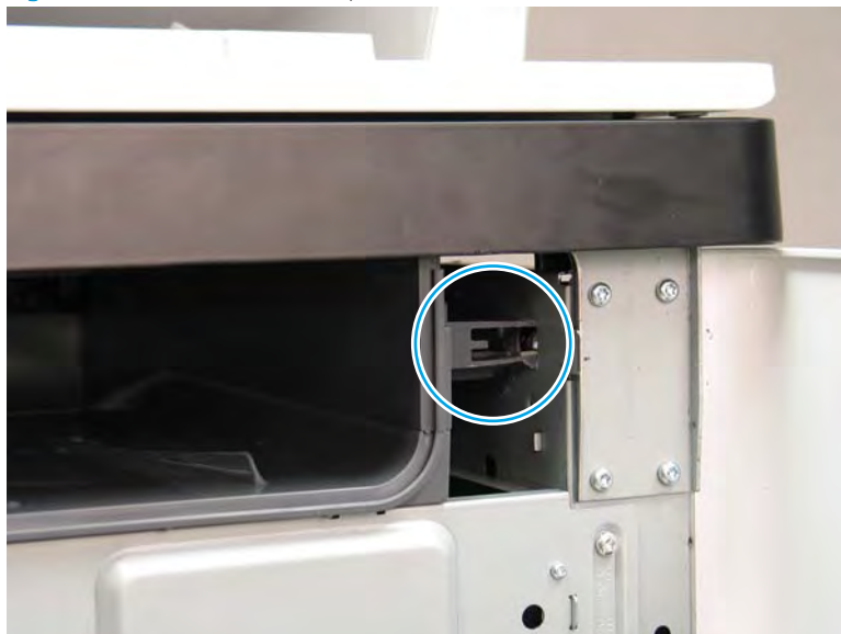
Figure 1-1551 Check the output bin installation
