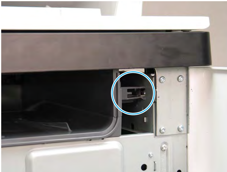
Figure 1-464 Check the output bin installation
