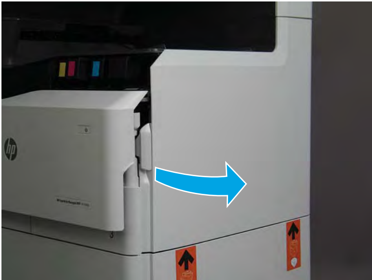
Figure 1-1085 Open the right door
