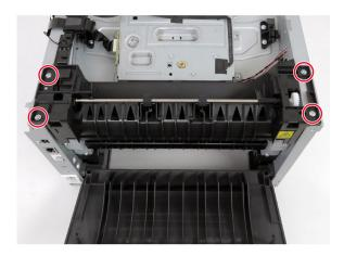
**6** Lift the redrive, and then disconnect the cable from the redrive.
