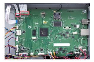
**6** Remove the three screws (A), remove the two cables (B) from the toroid (C), and then remove the printhead.
