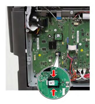
Installation note: Make sure that the connector is plugged.
