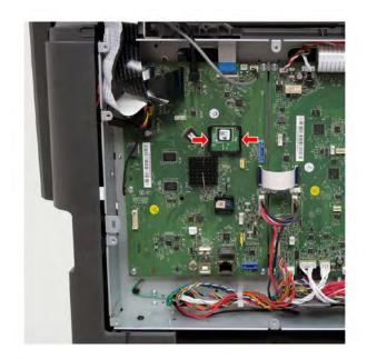
Installation note: Make sure that the connector is plugged.
