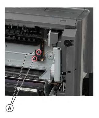
**3** Disconnect the cable (B), and then remove the sensor.
