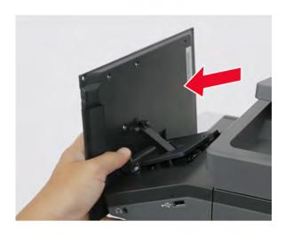
**4** Release the flat flex and ground cables from the control panel rear cover to remove the control panel base with rear cover.
