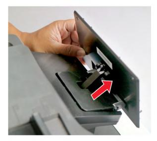
4 Release the FFC (B) from the control panel rear cover to remove the control panel base with rear cover.
