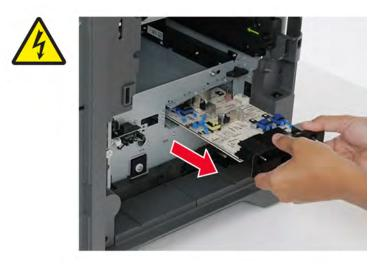
Installation note: Press on the side of the toner contacts (E) while removing the HVPS to fully release it.
