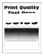
**Note:** Before performing this print quality check, print the Print Quality Test Pages. From the control panel, navigate to **Settings** > **Troubleshooting** > **Print Quality Test Pages**, and then perform the initial print quality check. See <u>"Initial print quality check" on page 35</u>.
