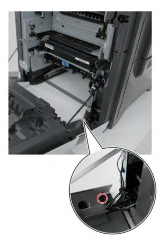
**2** Remove the two screws (A), and then remove the cable cover.
