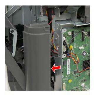
**9** Release the latch, remove the cable cover (D), and then remove the cables.
