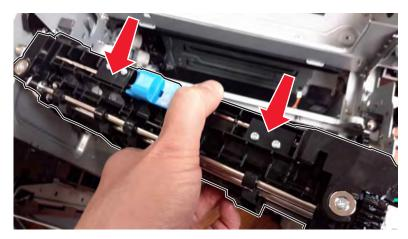
**13** Release the isolation unit cables from the printer.
