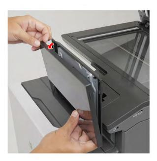
Unlock the clip, and then disconnect the cable.
