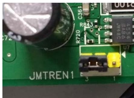
Interlock bypass disabled (default)
