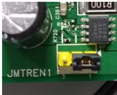
Interlock bypass enabled
