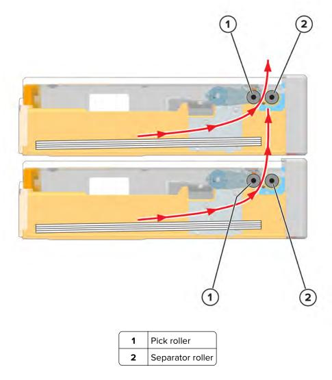
To prepare for feeding, the lift plate raises to push the paper against the pick roller. The lift plate stops pushing at the point where the pick roller is at the proper height for picking. After the pick roller is in position, it feeds the topmost paper to the separator roller. The separator roller rotates in a direction opposite to the pick roller to ensure that only one sheet is fed at a time.
