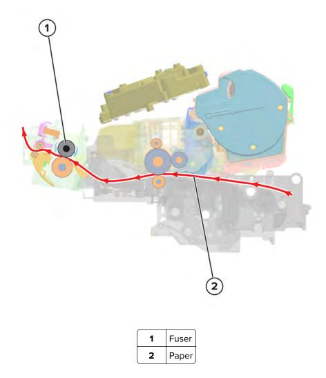
Even if the toner image is already on the paper, the toner particles are not yet permanently bonded to the surface. For the final part of printing, the paper is transported to the fuser where heat and pressure are applied to it. As a result, the toner particles melt and permanently fuse with the paper, completing the print process. The print cycle repeats for the succeeding pages.
