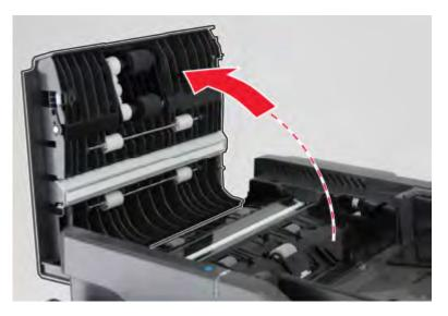
**2** Remove the restraint pad.
