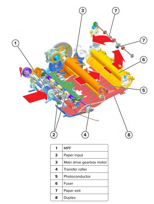
The gearbox provides mechanical power to the printer. Its motor transfer power through a number of gears to the following parts: MPF, paper input, transfer roll, photoconductor drum, fuser, paper exit, and duplex.
