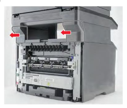
Installation note: Install the scanner rear covers first, and then the printer rear cover.
