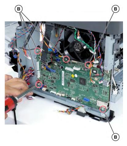
**7** Remove the controller board.
