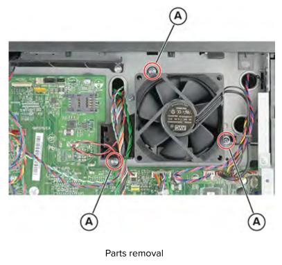
**4** Remove the two screws (B), and then remove the fan.
