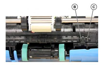
**Installation note:** When looping the isolation roller with the spring hook, make sure not to pierce the sleeve. Refer to the following illustrations:
