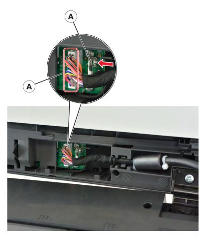
5 Release the cables off the assembly, and then remove the ADF.Installation note: Pay attention to the routing of the cables.
