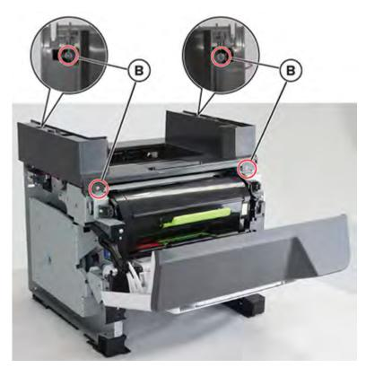
**7** Release the latch on the left and right sides of the cover.
