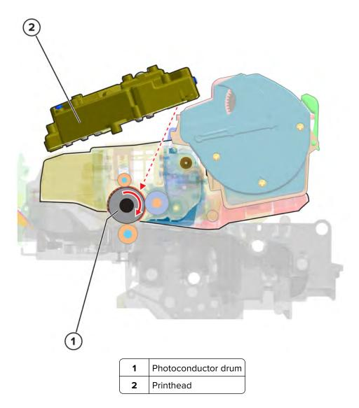
The printhead emits the light that contacts the surface of the photoconductor drum. The light turns on or off coinciding with the digital latent image. The light causes areas of the photoconductor drum surface to lose charge, resulting in a relative opposite polarity.
