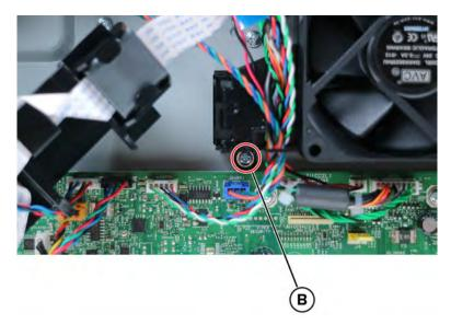
**5** Remove the two screws (C), and then remove the fan.
