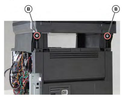
**6** Remove the flatbed scanner assembly.
