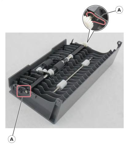
**3** Rotate the latches as shown, and then pull up to remove the roller.
