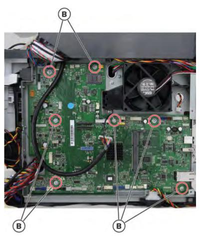
**8** Remove the controller board.
