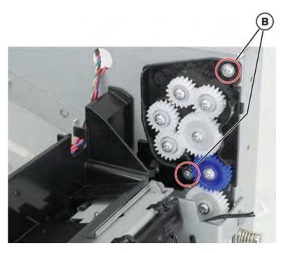
7 Remove the redrive gear assembly.
