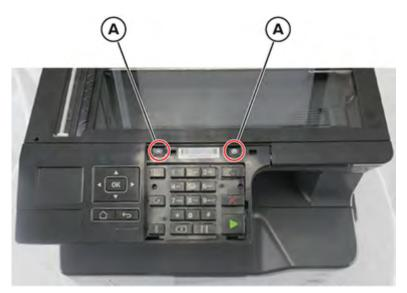
**4** Carefully disengage the assembly from the rear cover.
