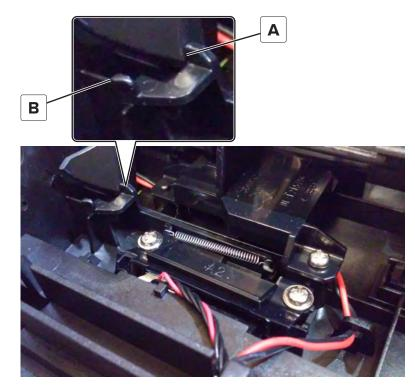
**5** Lift the pick roller assembly, and then place the bracket (M) in position.
