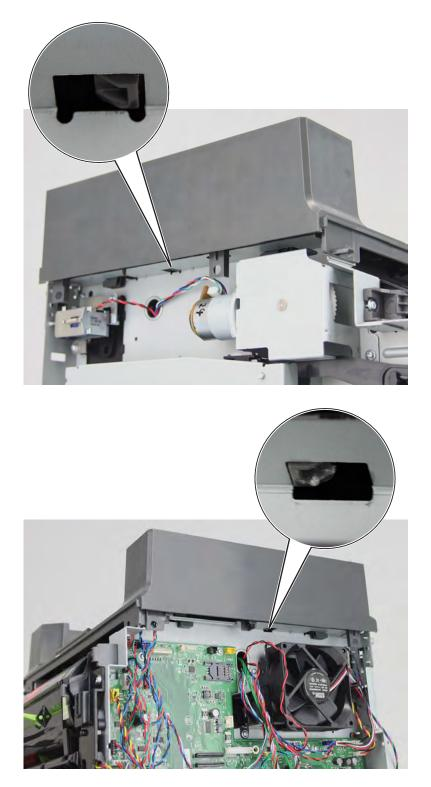
**8** Slide the cover to the front, and then pull up to remove.
