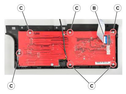
**4** Remove the control panel assembly.
