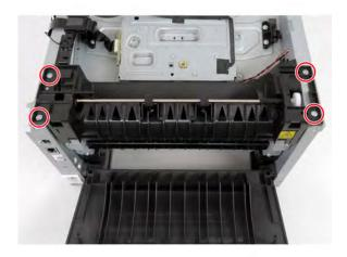
**5** Lift the redrive, and then disconnect the cable from the redrive.
