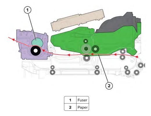
After the toner image is transferred to the paper, the toner particles are not yet permanently bonded to the paper. For the final step in the print process, paper is transported to the fuser where heat and pressure are applied to it. As a result, the toner particles melt and are permanently fused to the paper, completing the print process. The print cycle repeats for the succeeding pages.
