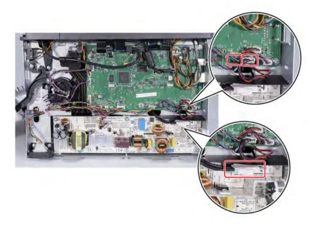
**3** Open the rear door, remove the four screws, and then remove the fuser.
