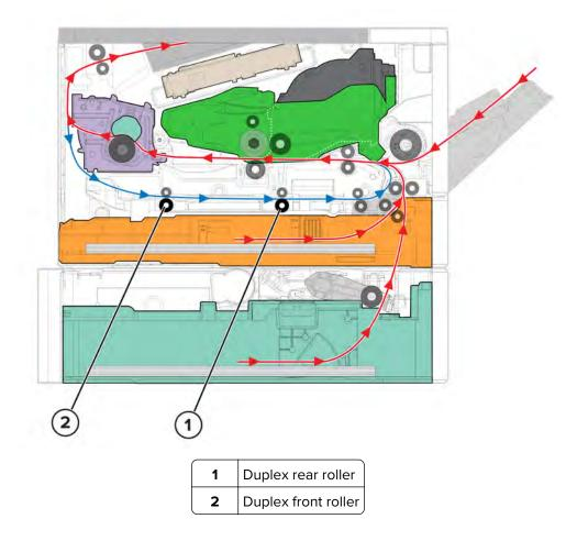
After the first side is printed, the paper stops at the output bin while still in the paper exit roller. The paper is fed again into the duplex paper path to have the opposite side printed.
