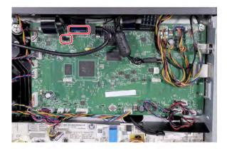
**5** Remove the three screws (A), remove the two cables (B) from the toroid (C), and then remove the printhead.
