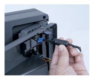
Release the three latches, and then remove the fax card.
