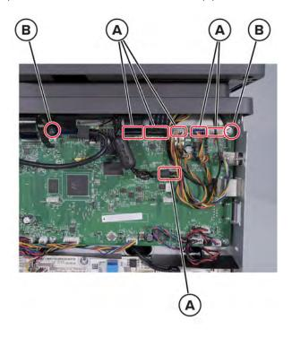
Remove the three screws from the printer frame.
