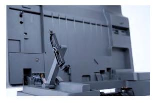
**3** Remove the two screws, and then remove the scanner pivot arm.
