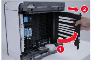
**Installation note:** Make sure that the duplex guide is properly inserted into the locating features inside the printer.
