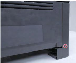
**2** Open the front door, and then release the left front door link.
