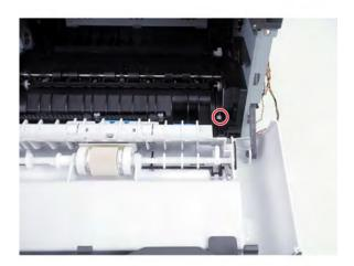
**3** Release the latches securing the sensor, and then disconnect the sensor cable.
