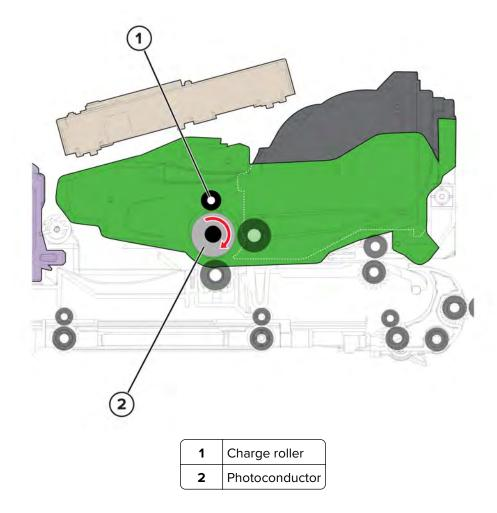
The charge roller applies a uniform negative electrical charge to the surface of the photoconductor. The insulative properties of the photoconductor allow it to hold a charge and its photoconductive properties allow it to discharge when exposed to light.
