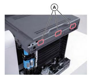
Release the latch at the front, and then remove the cover.
