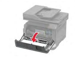
Locate the printer serial number behind the front door.
