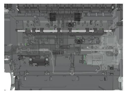
**e** Secure the cable at the pick/lift motor gearbox using cable ties. Cut off any excess cable tie.
