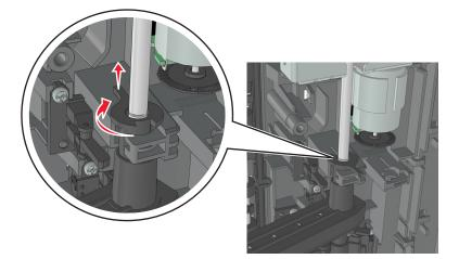
**9** Remove the ACM assembly along with its shaft.
