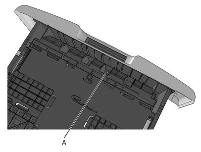
**2** Remove the E-clip, and then remove the gear.
