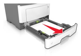
2 Firmly grasp the jammed paper on each side, and then gently pull it out.Note: Make sure all paper fragments are removed.
