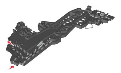
**c** Release the cartridge actuator. The cartridge lock should move back to its original position.
