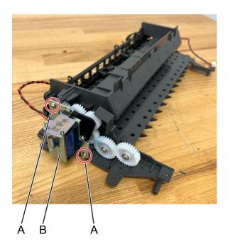
**b** Secure the solenoid to the screw holes (C) of the new redrive assembly.
