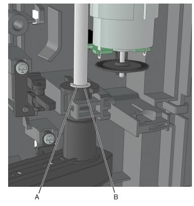
7 Remove the E-clip (A), and slide the washer (B) from the shaft.
