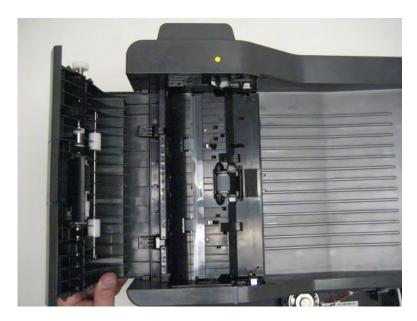
Release the cover by gently bending the ADF away from the top cover (1), and then lift the top cover (2) and remove.
