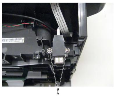
3 Remove the USB cable bracket.
