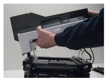
**Installation note:** After the new scanner assembly is installed, perform scanner manual registration, see <u>"Scanner manual registration" on page 244</u> and scanner calibration, see <u>"Scanner calibration" on page 221</u>.
