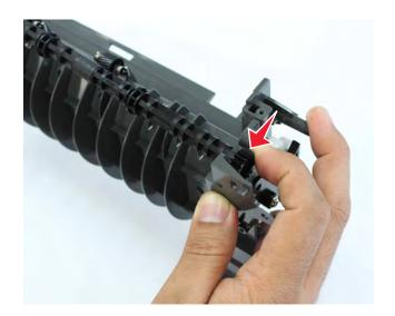
**8** If necessary, remove the bushing (B) from the redrive assembly.
