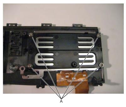
Remove the ground shield.
