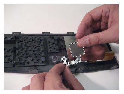
**5** Remove the light tube (B).
