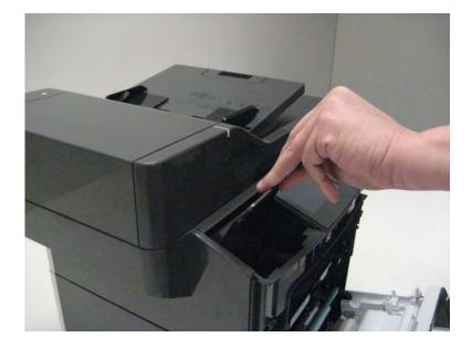
Lift the control panel to access the UICC underneath.
