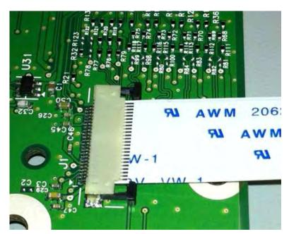
Slide the locking actuator towards the connector, locking the cable into place. The cable should not move when this step is performed. If the cable moves, open the actuator, reposition the cable, and then close the actuator to the down position.
