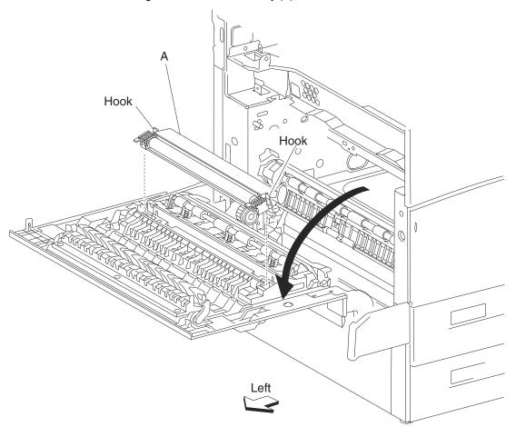
Note: Before reinstalling the transfer roll assembly (A), do not touch the roll surface.
