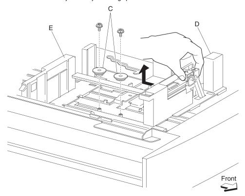
**Note:** Before reinstalling the pinion gears (C), slide the front media tray guide assembly (D) and the rear media guide (E) to their outward most positions. Ensure the media side guides slide smoothly.
