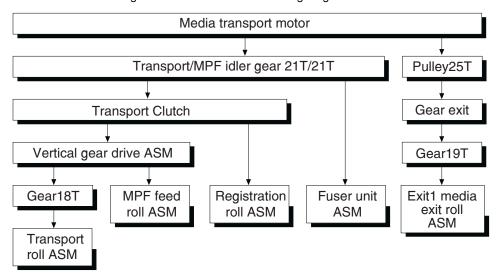
The driving force transmitted to the gear drives the transport roll assembly, multipurpose feeder (MPF) feed roll, registration roll assembly, fuser assembly, and exit 1 media exit roll assembly through the clutch and gears.
