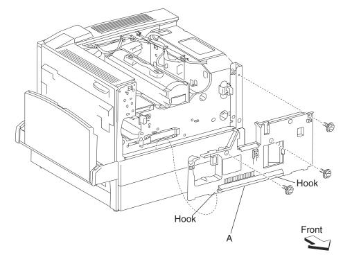
Note: To reinstall the front inner cover (A), start with the four plastic hooks on the bottom of the front inner cover.
