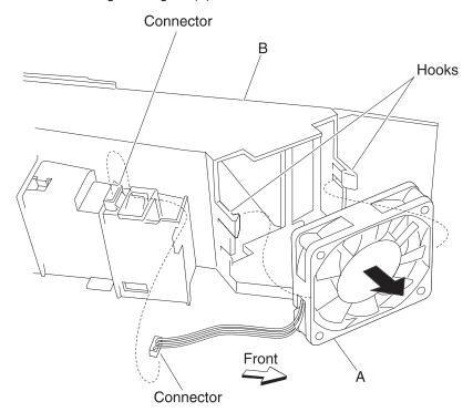
Note: Before reinstalling the PC cartridge cooling fan (A), ensure the fan blade is facing toward the front of the machine.
