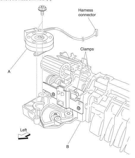
Note: Before reinstalling, secure the media shift motor (A) harness to the clamps on the exit 1 media shift assembly (B) to prevent damage.
