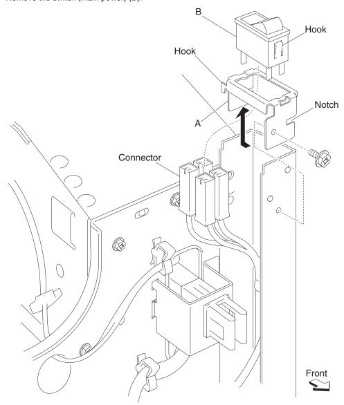
Note: Before reinstalling, ensure the four connectors are plugged into their proper location to prevent damage.
