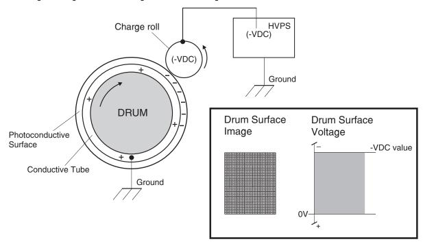
The charge roll is a conductive roll that is positioned slightly above the surface of the drum. The HVPS supplies the charge roll with two voltages; a negative DC charge voltage and an AC discharge voltage that is used for electrically cleaning the drum (discussed in Step 6. Clean).
