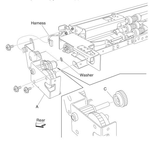
**Note:** Before reinstalling, ensure all gears and washers are securely attached to the bracket (A).
