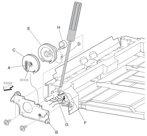
**9.** Remove the drive gear cam (E) and the drive stopper (H).
