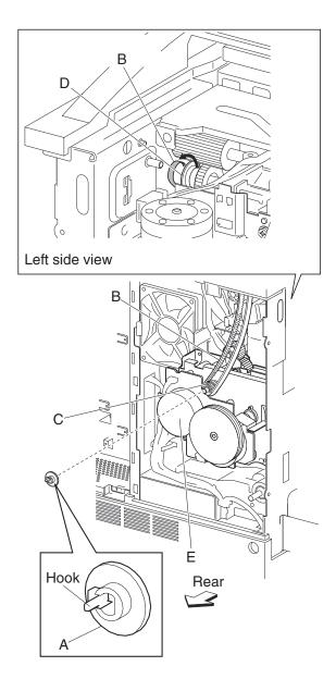
Note: Press on the exit 1 drive belt (B) while slowly turning the motor (E) by hand.
