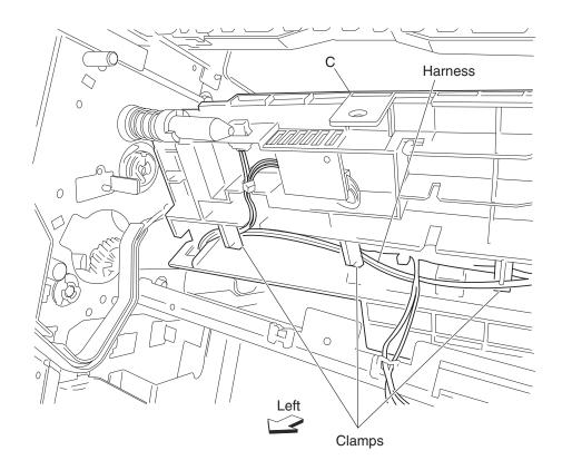
23. Lift the right side of the PC cartridge guide assembly (C). Remove the screw (G) securing the switch (PC cartridge interlock) (H) to the PC cartridge guide assembly (C). Remove the switch (PC cartridge interlock) (H).
