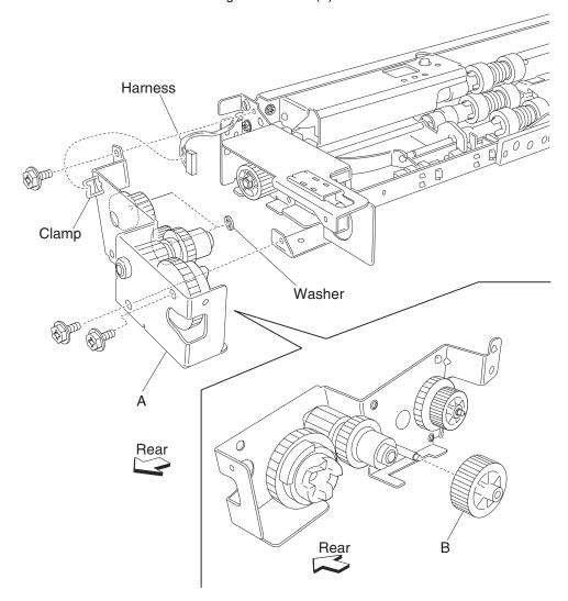
**6.** Remove the media feed unit drive gear - 29 tooth (B).
