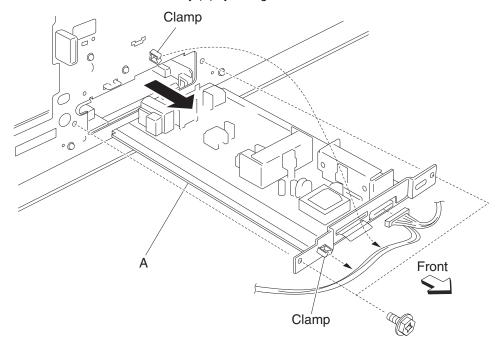
Note: Before reinstalling, ensure the HVPS (A) is inserted into the side slots properly.
