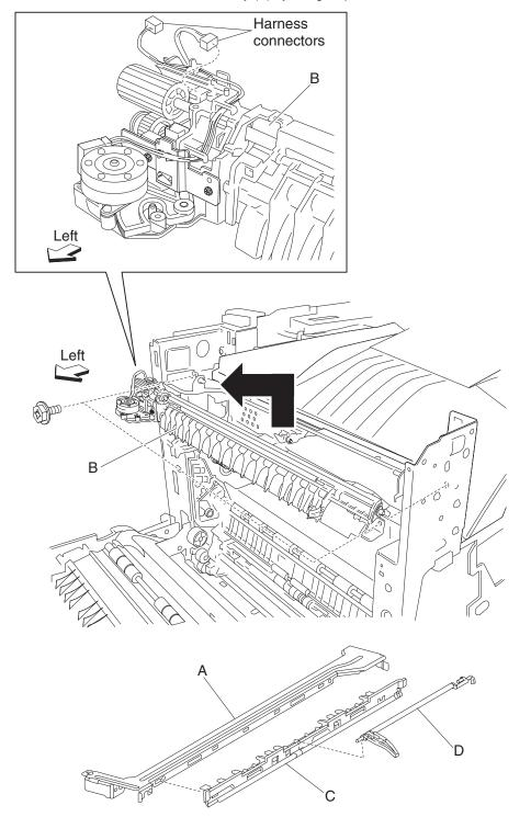
**Note:** When reinstalling the bracket (A), first release the hooks securing the plastic guide (C) that is attached to the bracket (A).
